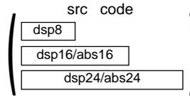
\*1 When src is indirectly addressed the code has 00001001 added at the beginning.
