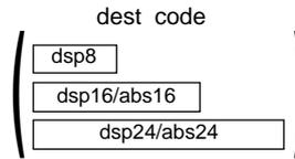
\*1 When dest is indirectly addressed, the code has 00001001 added at the beginning.
