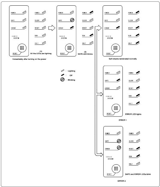
Figure 4.4 Self-check procedure
