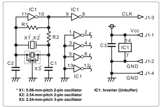
*Figure 3.7 Circuit of oscillator board (OSC-2)*
