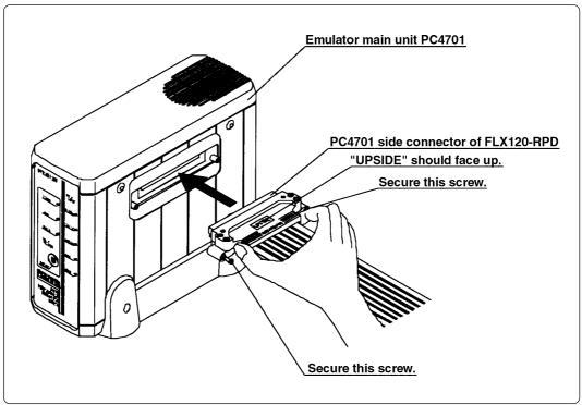
Figure 3.9 Connecting PC4701 and FLX120-RPD
