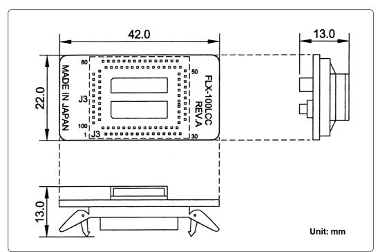
Figure 5.14 External dimensions of pitch converter board (FLX-100LCC)
