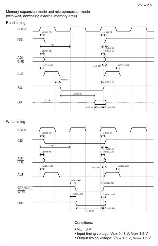
*Figure 5.7 Memory expansion mode and microprocessor mode (with wait)*
