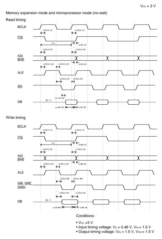
Figure 5.6 Memory expansion mode and microprocessor mode (no-wait)
