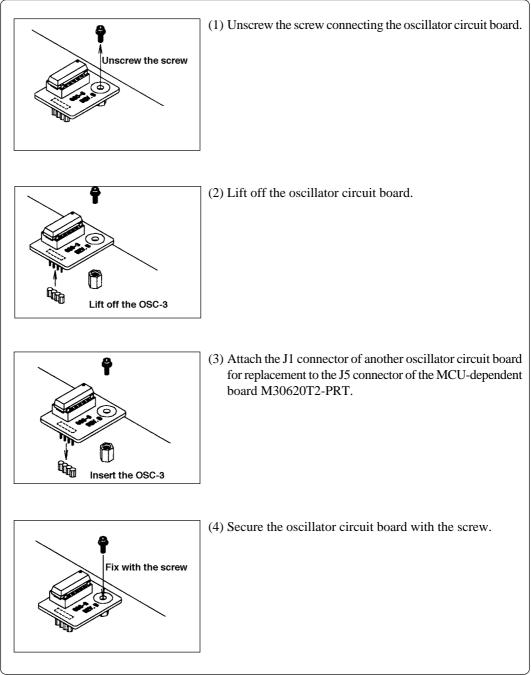
Figure 3.8 Replacing the oscillator circuit boards
