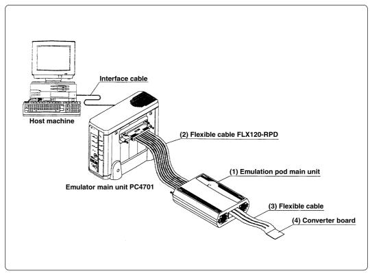
Figure 2.1 System configuration
