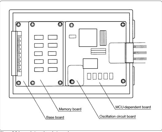
Figure 2.2 Internal view of emulation pod
