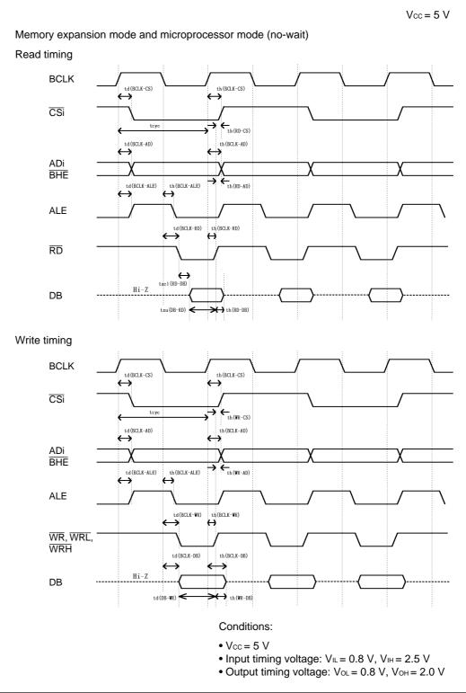
Figure 5.1 Memory expansion mode and microprocessor mode (no-wait)
