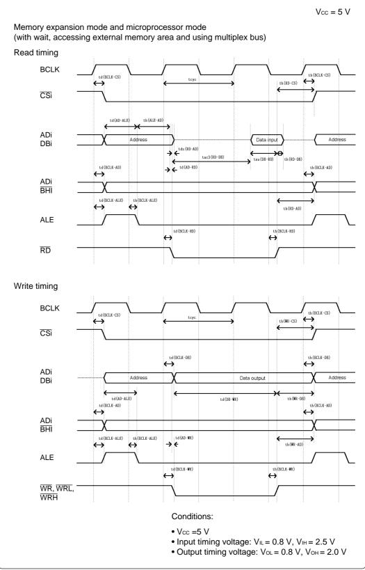
Figure 5.3 Memory expansion mode and microprocessor mode (with wait, multiplex bus)
