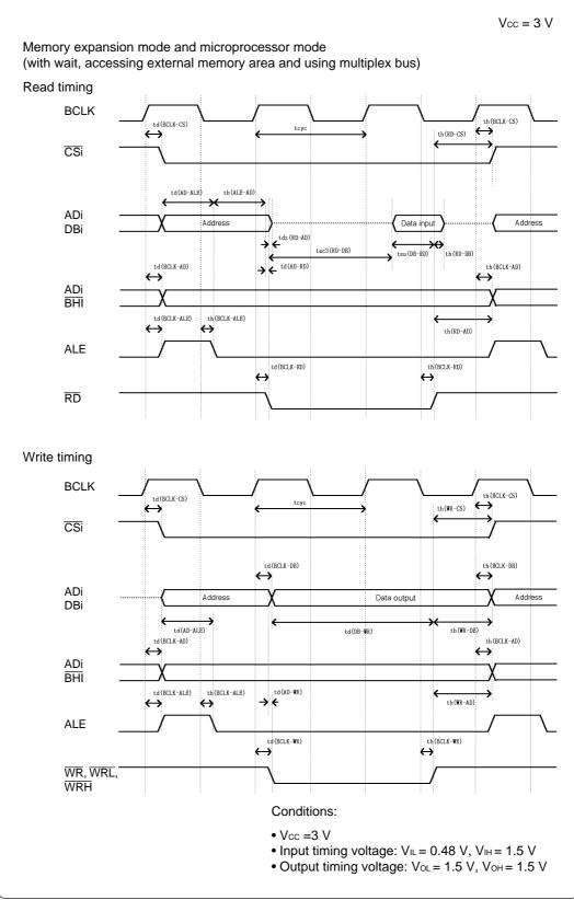
Figure 5.8 Memory expansion mode and microprocessor mode (with wait, multiplex bus)
