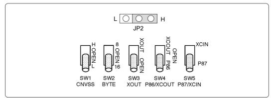
Figure 4.3 Switch settings when running the self-check (factory-settings)
