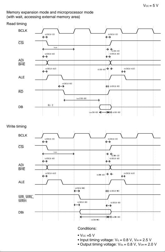
Figure 5.2 Memory expansion mode and microprocessor mode (with wait)
