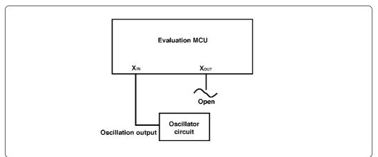
Figure 3.4 External oscillator circuit
