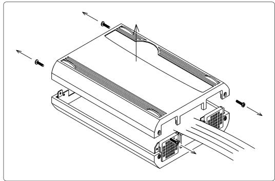
Figure 3.1 Removing the upper cover
