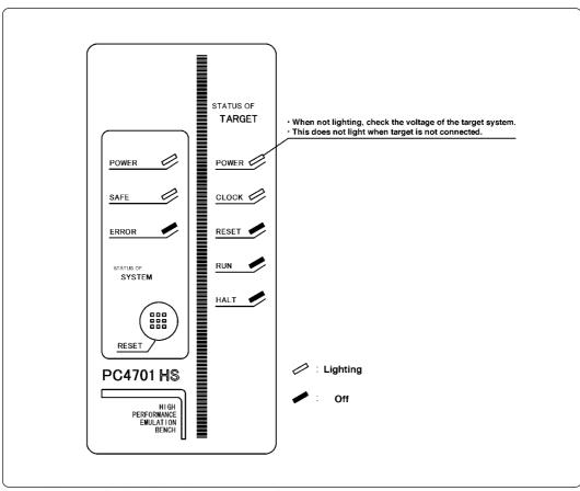
Figure 4.1 LED display when the power turned on
