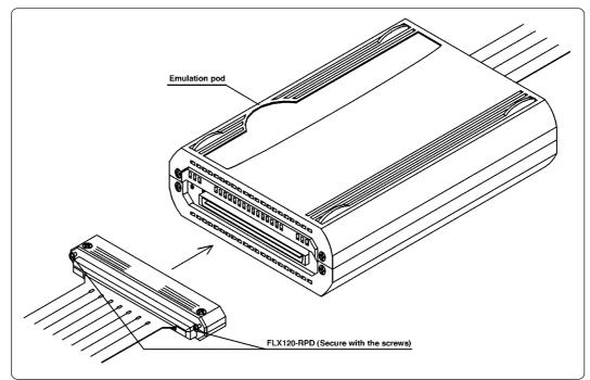
Figure 3.10 Connecting FLX120-RPD and emulation pod
