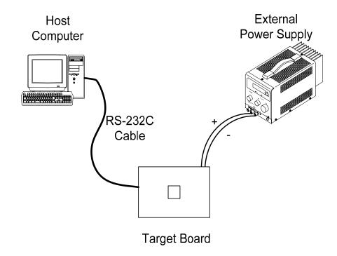
Figure 1 Connecting the Target Board to the User System
