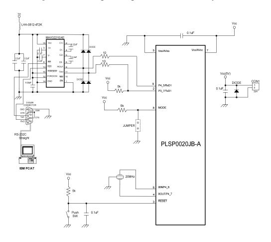
Figure 2 Circuit Using the RS-232C Cable (R8C/28, 29 Groups)
