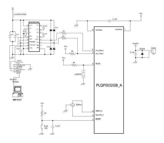
Figure 3 Circuit Using the RS-232C Cable (R8C/26, 27 Groups)
