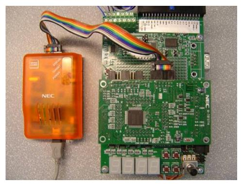
Figure 8-3 OCD Debugger Unit Connection
