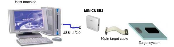
Figure 1-3 Example of ID78K0R-QB System Configuration [MINICUBE2]
