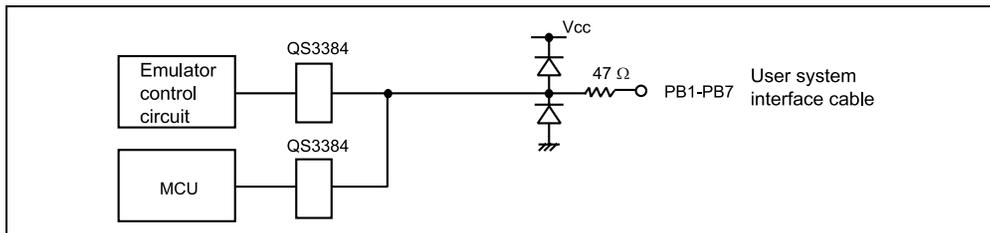
**Figure 7.5 User System Interface Circuit for PB1-PB7**
