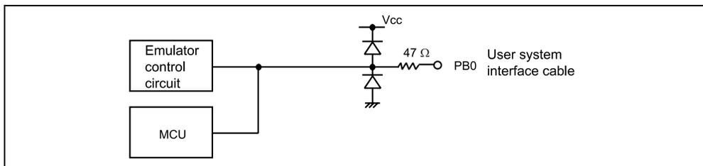
**Figure 7.4 User System Interface Circuit for PB0**
