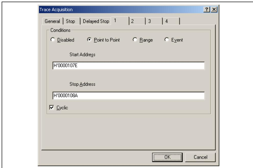
**Figure 5.73 Range Trace Setting (Point to Point)**
