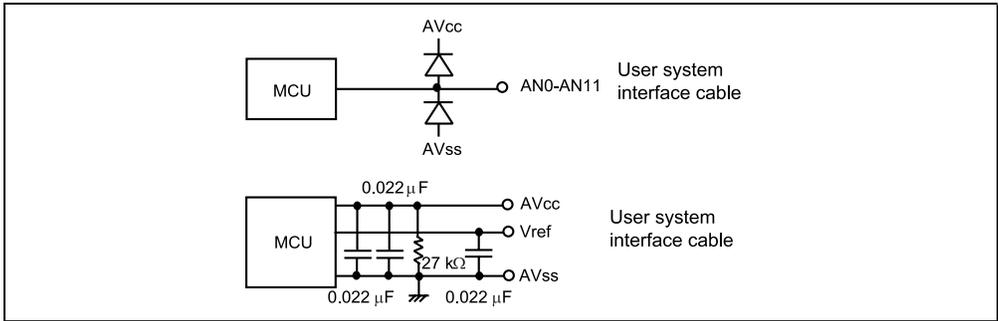
Figure 7.6 User System Interface Circuit for AN0-AN11, AVcc, AVss and Vref Signals
