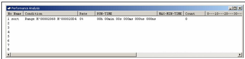
**Figure 6.67 [Performance Analysis] Dialog Box (Setting Completed)**
