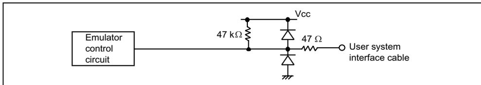
**Figure 7.3 User System Interface Circuit for RESET**
