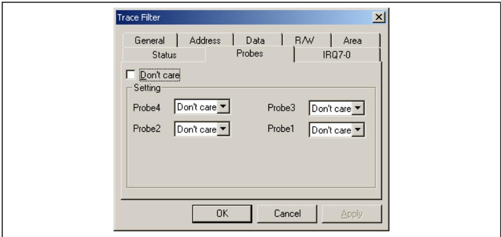
**Figure 5.91 [Trace Filter] Dialog Box ([Probes] Page)**
