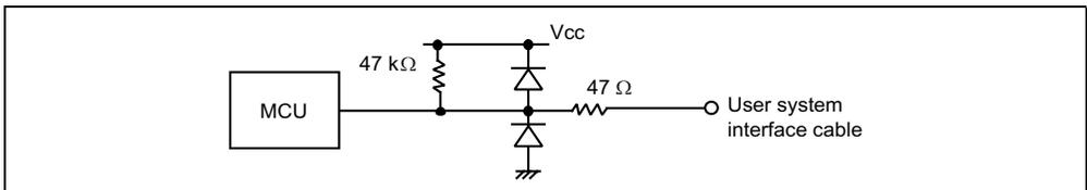
**Figure 7.1 Default User System Interface Circuit**
