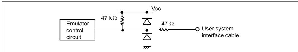
**Figure 7.2 User System Interface Circuit for MD2, MD1, MD0, NMI, WAIT, and STBY**
