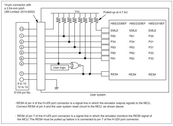
Figure 1.3 Example of E10A Emulator Connection
