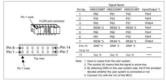
Figure 1.2 Pin Assignments of the H-UDI Port Connector
