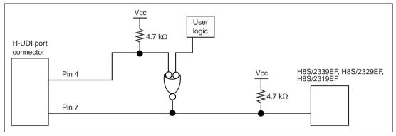
Figure 1.6 Connection of the RES# Pin
