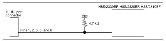
Figure 1.4 Connection of E10A Emulator and the MCU
