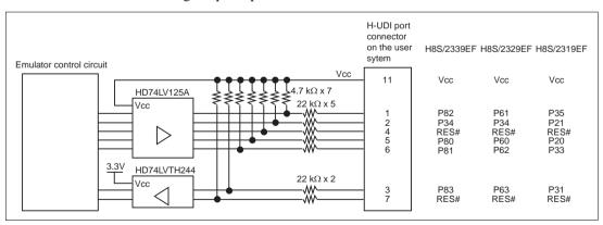
Figure 1.7 Interface Circuit in the Emulator (Reference)
