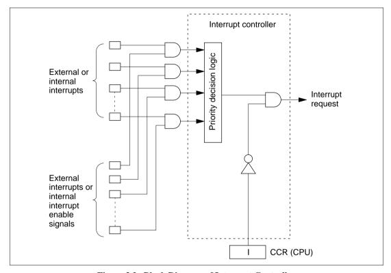
Figure 3.2 Block Diagram of Interrupt Controller
