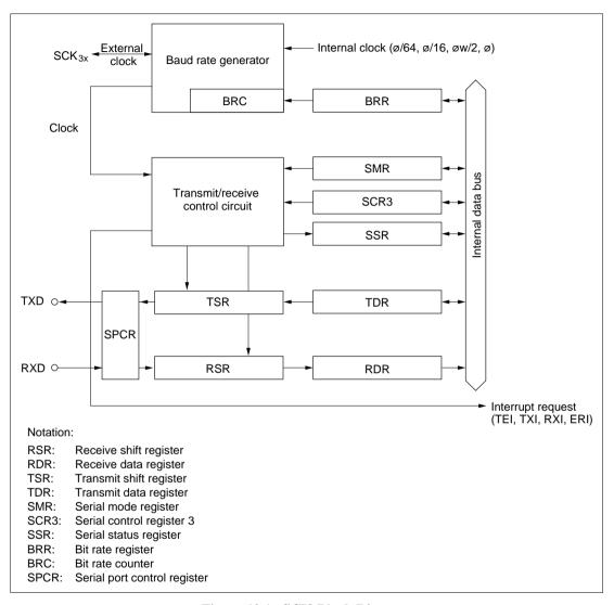
Figure 10.1 SCI3 Block Diagram
