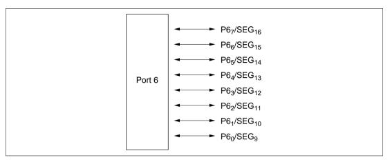
Figure 8.5 Port 6 Pin Configuration
