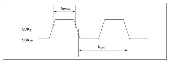
Figure 15.5 SCK3 Input Clock Timing
