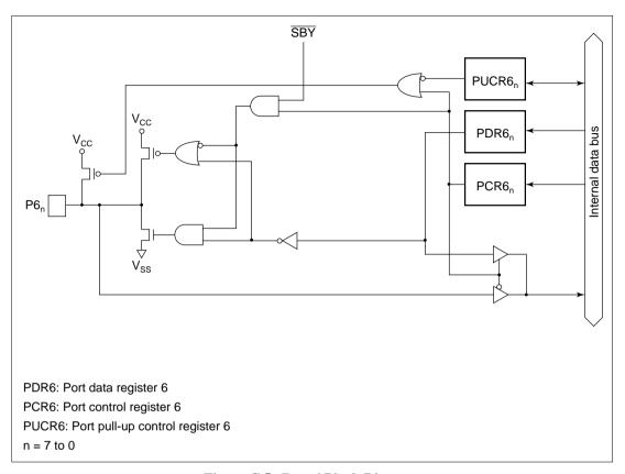
Figure C.5 Port 6 Block Diagram
