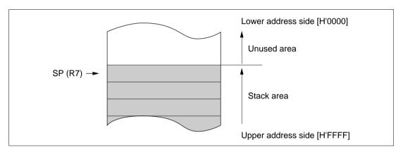
Figure 2.2 Stack Pointer
