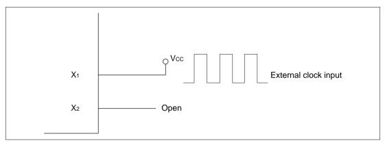
Figure 4.10 Pin Connection when Inputting External Clock
