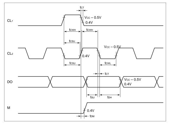
Figure 15.7 Segment Expansion Signal Timing
