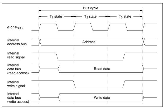
Figure 2.13 On-Chip Peripheral Module Access Cycle (3-State Access)
