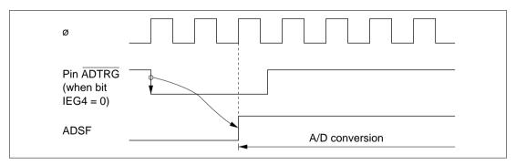
Figure 12.2 External Trigger Input Timing
