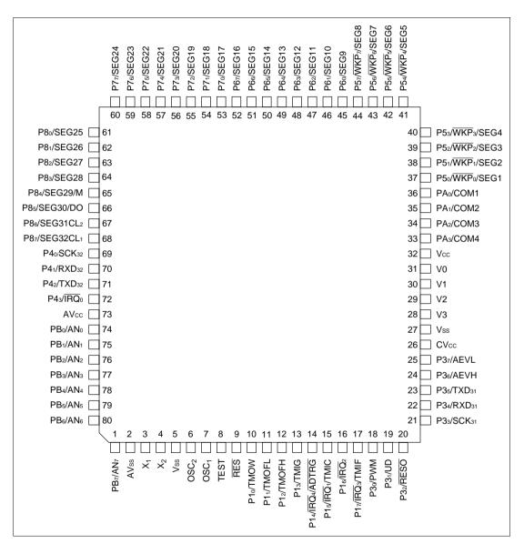
Figure 1.2 Pin Arrangement (FP-80A, TFP-80C: Top View)
