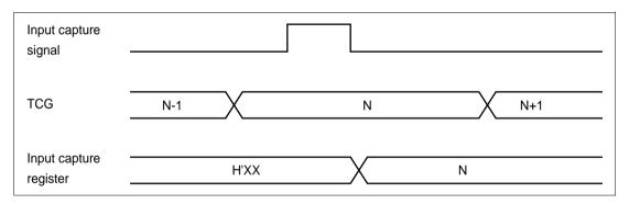
Figure 9.12 Timing of Input Capture by Input Capture Input
