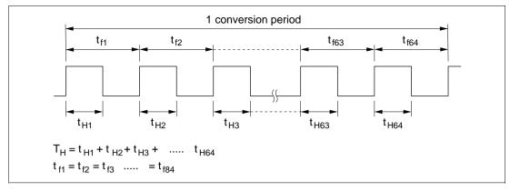
Figure 11.2 PWM Output Waveform
