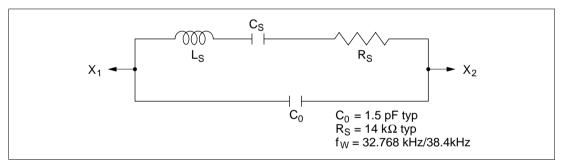
Figure 4.8 Equivalent Circuit of 32.768-kHz/38.4 kHz Crystal Oscillator
