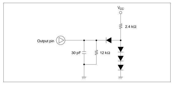
Figure 15.8 Output Load Condition
