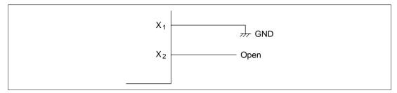
Figure 4.9 Pin Connection when not Using Subclock
