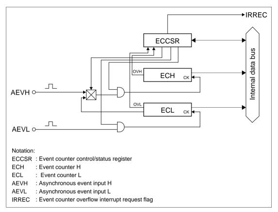
Figure 9.18 Block Diagram of Asynchronous Event Counter
