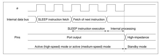
Figure 5.2 Standby Mode Transition and Pin States
