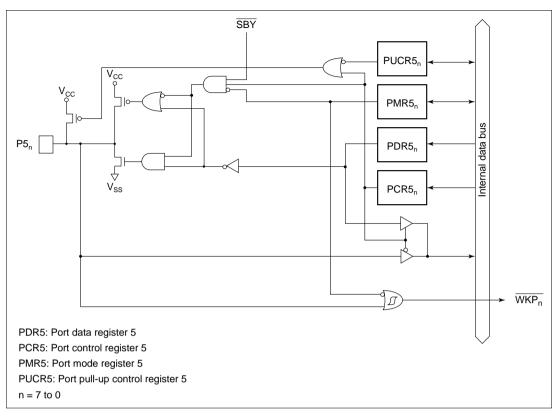
Figure C.4 Port 5 Block Diagram
