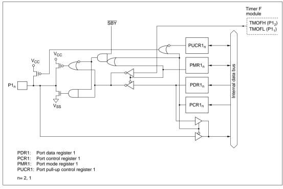
Figure C.1 (c) Port 1 Block Diagram (Pin P1<sub>2</sub>, P1<sub>1</sub>)
