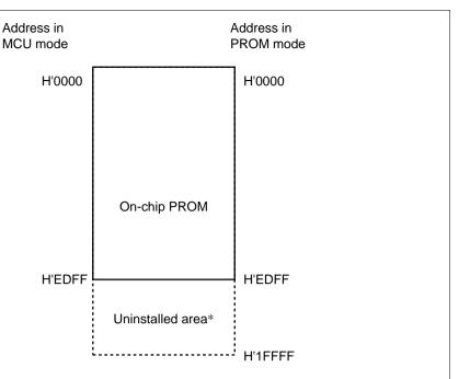
Note: \* The output data is not guaranteed if this address area is read in PROM mode. Therefore, when programming with a PROM programmer, be sure to specify addresses from H'0000 to H'EDFF. If programming is inadvertently performed from H'EE00 onward, it may not be possible to continue PROM programming and verification.
