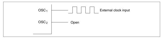
Figure 4.6 External Clock Input (Example)
