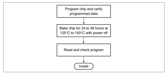
Figure 6.6 Recommended Screening Procedure
