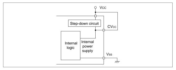
Figure 14.2 Power Supply Connection when Internal Step-Down Circuit Is Not Used
