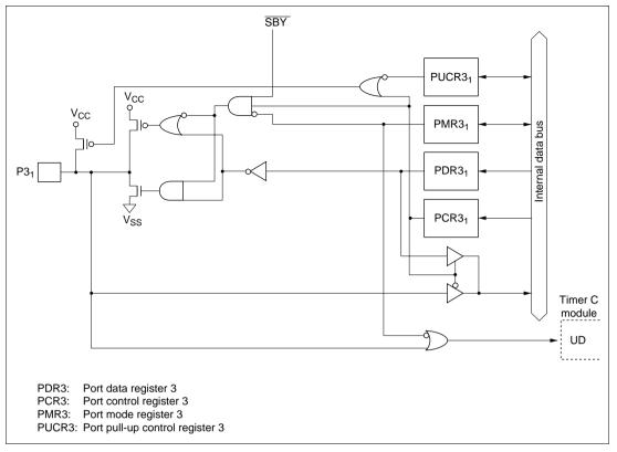
Figure C.2 (f) Port 3 Block Diagram (Pin P3<sub>1</sub>)
