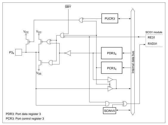
Figure C.2 (c) Port 3 Block Diagram (Pin P3<sub>4</sub>)
