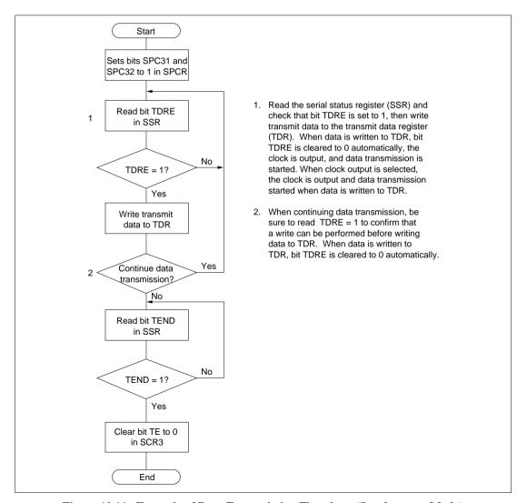
Figure 10.11 Example of Data Transmission Flowchart (Synchronous Mode)
