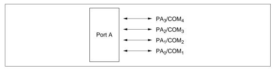
Figure 8.8 Port A Pin Configuration
