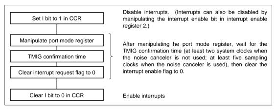
Figure 9.14 Port Mode Register Manipulation and Interrupt Enable Flag Clearing Procedure
