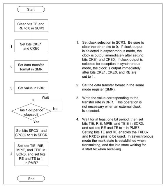
Figure 10.5 Example of SCI3 Initialization Flowchart
