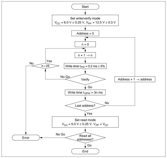
Figure 6.4 High-Speed, High-Reliability Programming Flow Chart
