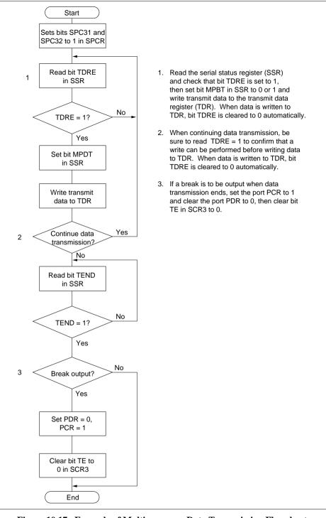
Figure 10.17 Example of Multiprocessor Data Transmission Flowchart
