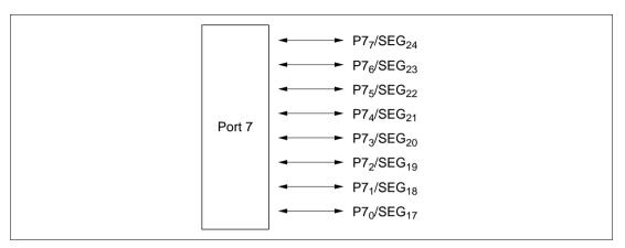
Figure 8.6 Port 7 Pin Configuration
