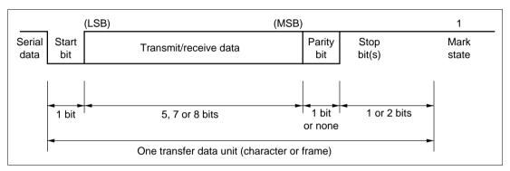
Figure 10.3 Data Format in Asynchronous Communication
