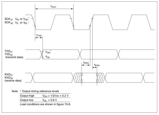
Figure 15.6 SCI3 Synchronous Mode Input/Output Timing
