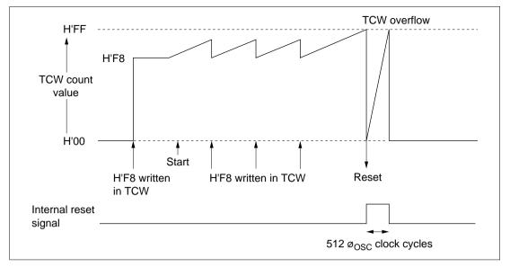
Figure 9.17 Typical Watchdog Timer Operations (Example)
