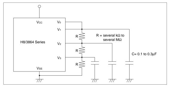
Figure 13.17 Connection of External Split-Resistance
