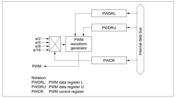
Figure 11.1 Block Diagram of the 14 bit PWM
