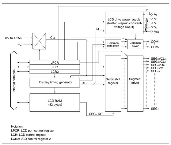
Figure 13.1 Block Diagram of LCD Controller/Driver
