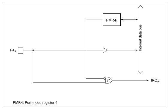
Figure C.3 (a) Port 4 Block Diagram (Pin P4<sub>3</sub>)
