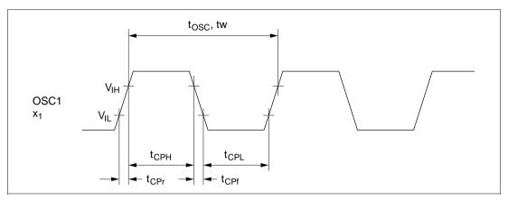
Figure 15.1 Clock Input Timing
