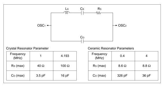
Figure 15.9 Resonator Equivalent Circuit
