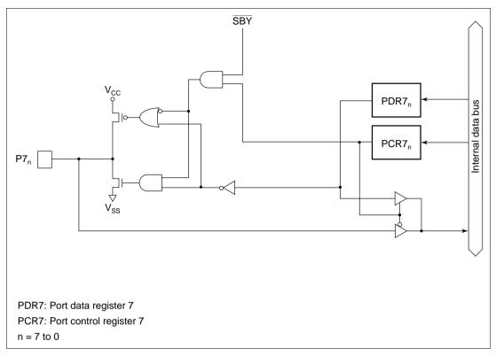
Figure C.6 Port 7 Block Diagram
