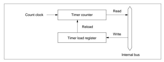
Figure 2.18 Timer Configuration Example
