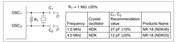
Figure 4.2 Typical Connection to Crystal Oscillator
