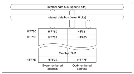
Figure 7.1 RAM Block Diagram (H8/3864 and H8/3824)
