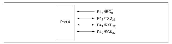
Figure 8.3 Port 4 Pin Configuration
