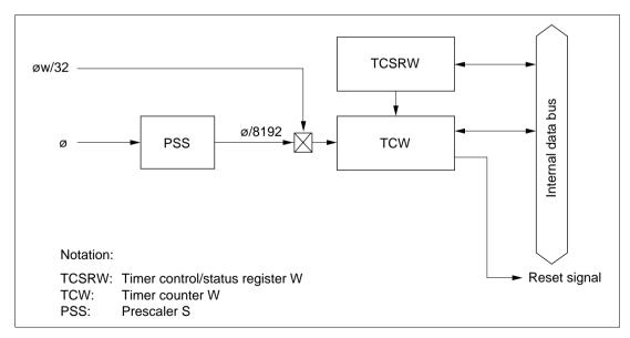
Figure 9.16 Block Diagram of Watchdog Timer
