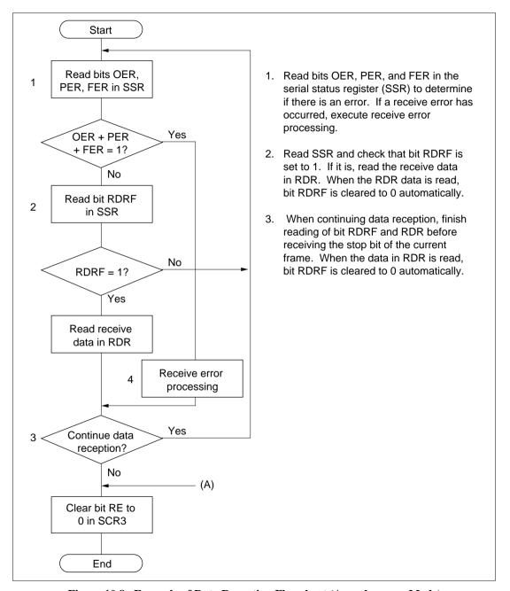
Figure 10.8 Example of Data Reception Flowchart (Asynchronous Mode)
