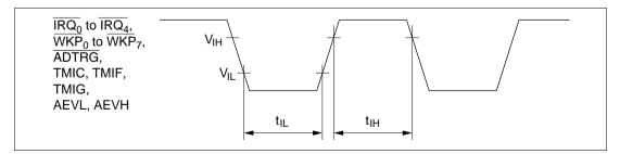
Figure 15.3 Input Timing
