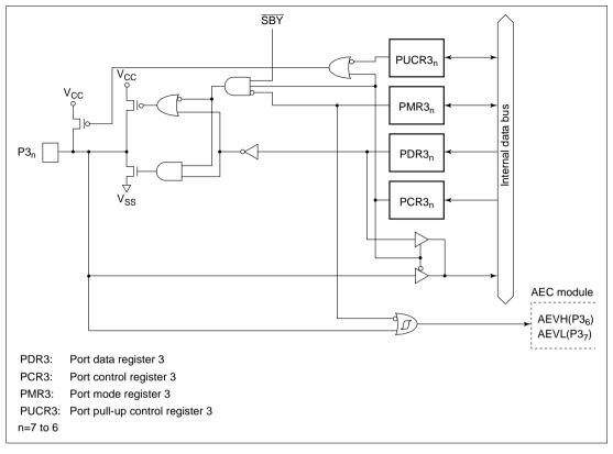
Figure C.2 (a) Port 3 Block Diagram (Pin P3<sub>7</sub> to P3<sub>6</sub>)
