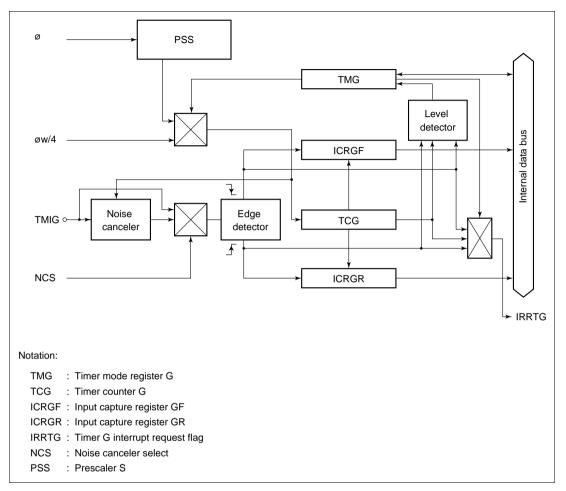
Figure 9.7 Block Diagram of Timer G
