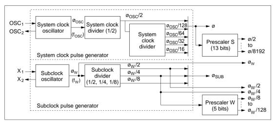
Figure 4.1 Block Diagram of Clock Pulse Generators
