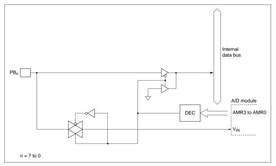
Figure C.9 Port B Block Diagram
