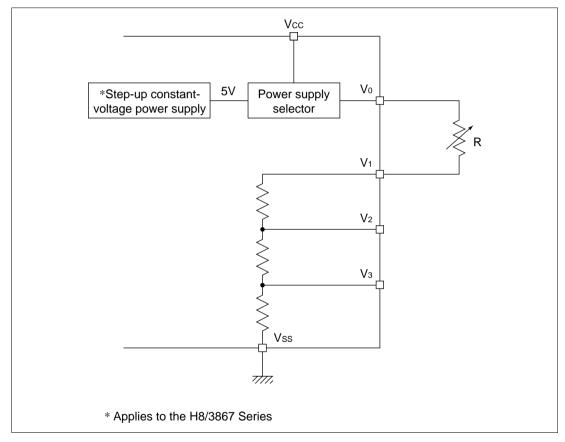
Figure 13.13 LCD Drive Power Supply Unit
