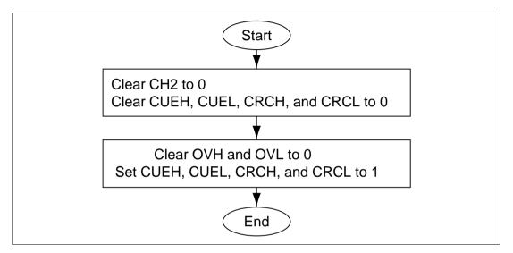
Figure 9.19 Example of Software Processing when Using ECH and ECL as 16-Bit Event Counter
