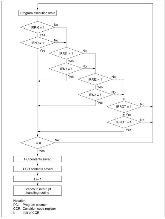
Figure 3.3 Flow up to Interrupt Acceptance
