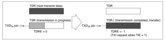
Figure 10.2 (b) TDRE Setting and TXI Interrupt
