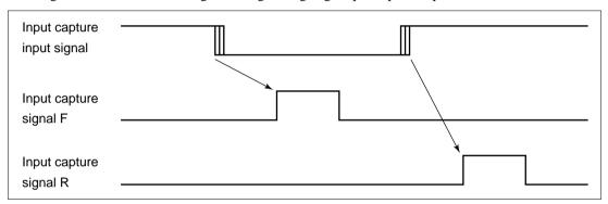
Figure 9.10 Input Capture Input Timing (without Noise Cancellation Function)
