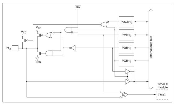
Figure C.1 (b) Port 1 Block Diagram (Pin P1<sub>3</sub>)
