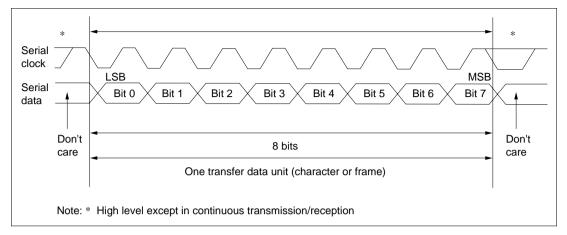
Figure 10.10 Data Format in Synchronous Communication
