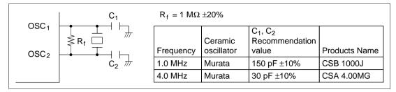
Figure 4.4 Typical Connection to Ceramic Oscillator
