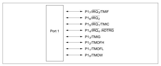
Figure 8.1 Port 1 Pin Configuration
