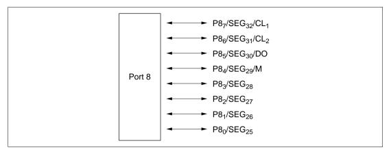
Figure 8.7 Port 8 Pin Configuration
