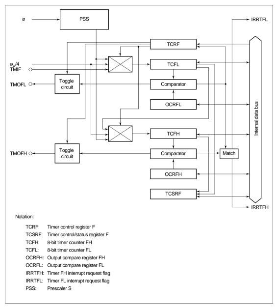
Figure 9.3 Block Diagram of Timer F
