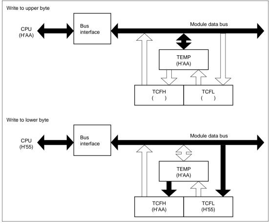
Figure 9.4 Write Access to TCR (CPU Æ TCF)
