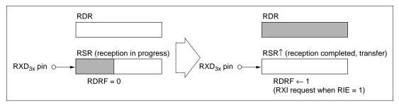
Figure 10.2 (a) RDRF Setting and RXI Interrupt
