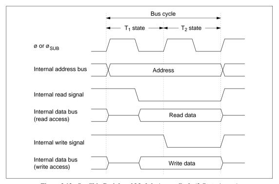
Figure 2.12 On-Chip Peripheral Module Access Cycle (2-State Access)
