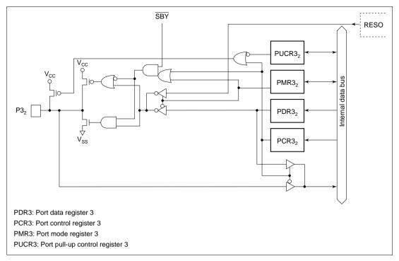
Figure C.2 (e) Port 3 Block Diagram (Pin P3<sub>2</sub>)
