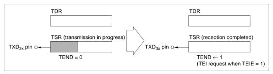
Figure 10.2 (c) TEND Setting and TEI Interrupt
