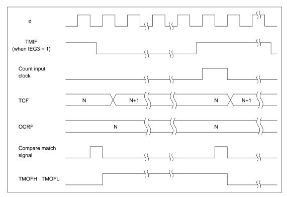
Figure 9.6 TMOFH/TMOFL Output Timing
