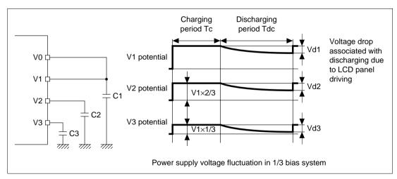
Figure 13.14 Example of Low-Power-Consumption LCD Drive Operation
