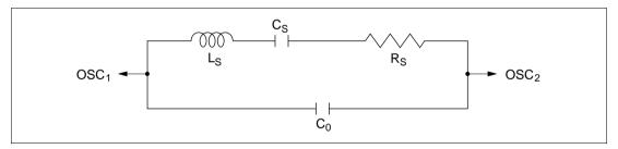
Figure 4.3 Equivalent Circuit of Crystal Oscillator
