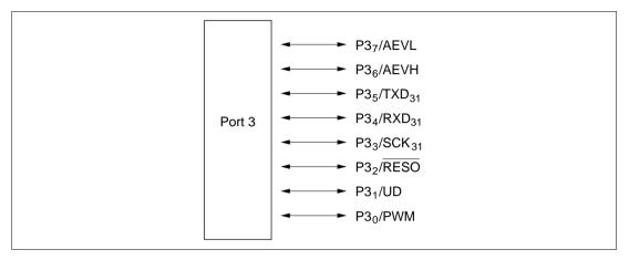
Figure 8.2 Port 3 Pin Configuration
