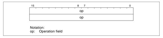
Figure 2.10 Block Data Transfer Instruction Code
