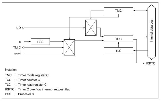
Figure 9.2 Block Diagram of Timer C
