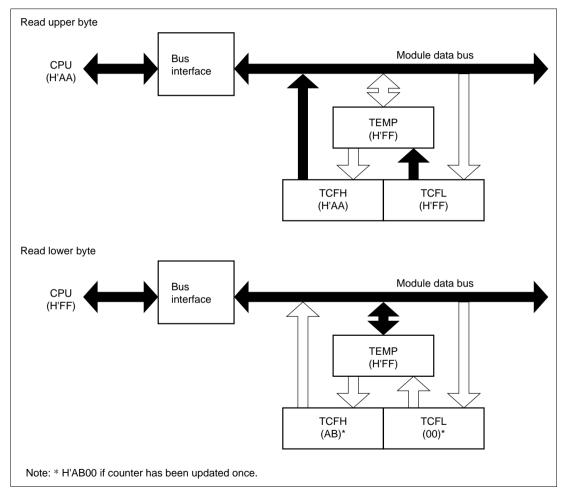
Figure 9.5 Read Access to TCF (TCF Æ CPU)
