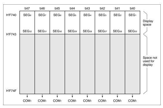
Figure 13.8 LCD RAM Map when Not Using Segment External Expansion (Static Mode)
