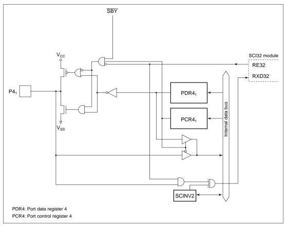
Figure C.3 (c) Port 4 Block Diagram (Pin P4<sub>1</sub>)
