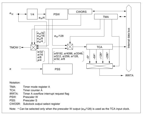
Figure 9.1 Block Diagram of Timer A
