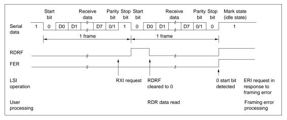
Figure 10.9 Example of Operation when Receiving in Asynchronous Mode (8-bit data, parity, 1 stop bit)
