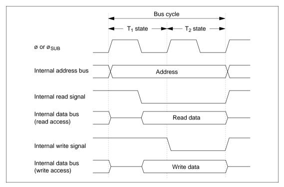
Figure 2.11 On-Chip Memory Access Cycle
