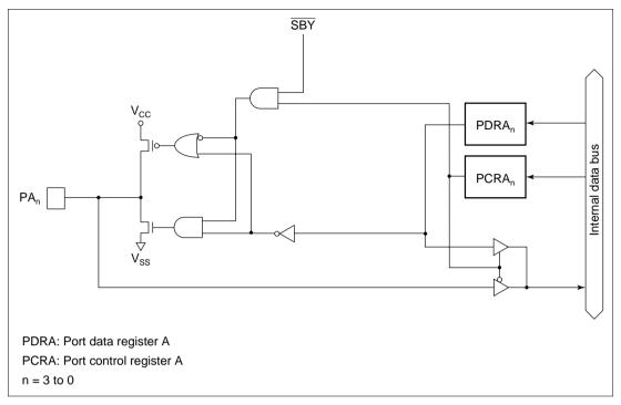
Figure C.8 Port A Block Diagram
