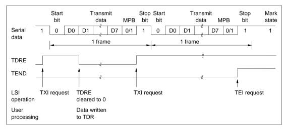
Figure 10.18 Example of Operation when Transmitting using Multiprocessor Format (8-bit data, multiprocessor bit, 1 stop bit)
