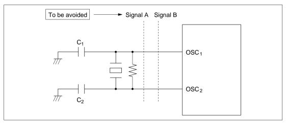
Figure 4.5 Board Design of Oscillator Circuit
