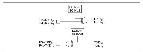
Figure 8.10 Input/Output Data Inversion Function
