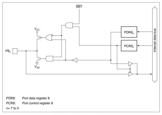
Figure C.7 Port 8 Block Diagram
