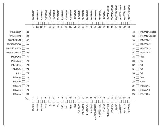
Figure 1.3 Pin Arrangement (FP-80B: Top View)
