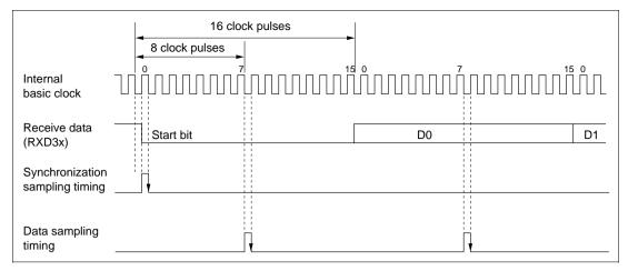
Figure 10.21 Receive Data Sampling Timing in Asynchronous Mode
