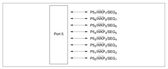
Figure 8.4 Port 5 Pin Configuration
