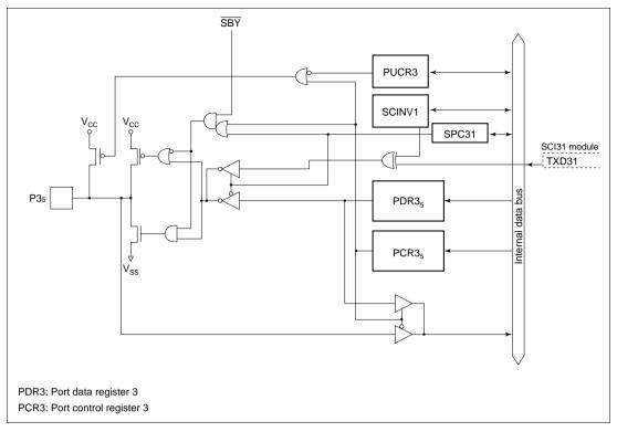
Figure C.2 (b) Port 3 Block Diagram (Pin P3<sub>5</sub>)
