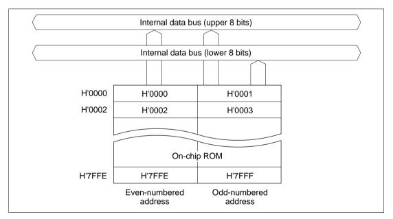
Figure 6.1 ROM Block Diagram (H8/3864 and H8/3824)
