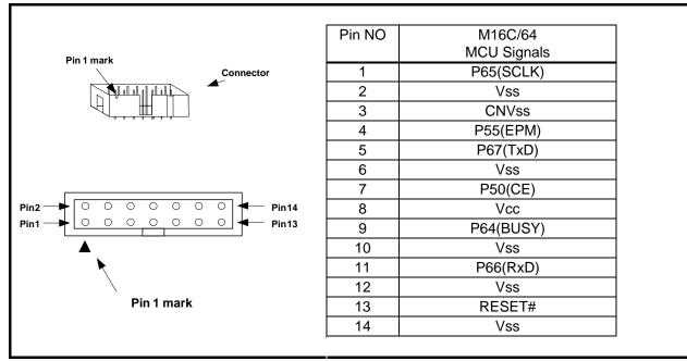
Figure 3.2 E8a Connecting Connector Pin Assignments
