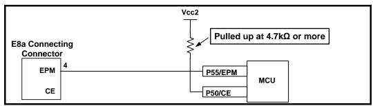
Figure 4.8 Connection of E8a Emulator and Pins P50 and P55 (Dual Power Supply and Single-chip Mode)
