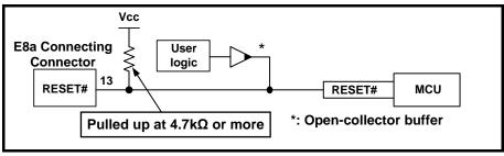
Figure 4.11 Example of a Reset Circuit
