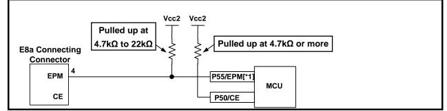
Figure 4.9 Connection of E8a Emulator and Pins P50 and P55 (Dual Power Supply and Memory Expansion Mode)
