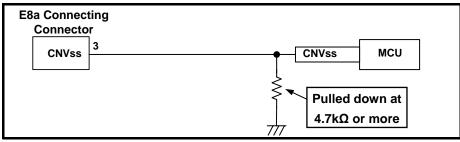
Figure 4.10 E8a Emulator and CNVss Pin Connection
