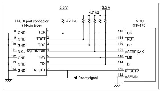
Figure 4.2 Recommended Circuit for Connection between the H-UDI Port Connector and MCU (14-Pin Type)
