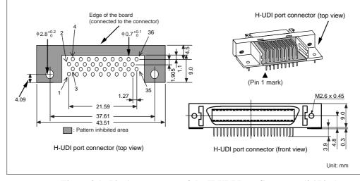
Figure 3.1 Pin Arrangement of the H-UDI Port Connector (36 Pins)
