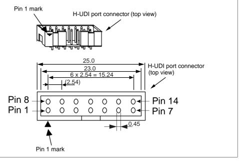
Figure 3.2 Pin Arrangement of the H-UDI Port Connector (14 Pins)
