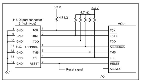
Figure 4.2 Recommended Circuit for Connection between the H-UDI Port Connector and the MCU when Using the Emulator (14-Pin Type)
