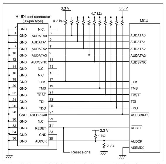
Figure 4.1 Recommended Circuit for Connection between the H-UDI Port Connector and the MCU when Using the Emulator (36-Pin Type)
