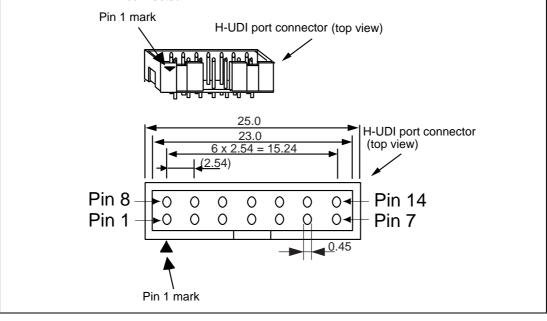
Figure 3.2 Pin Arrangement of the H-UDI Port Connector (14 Pins)
