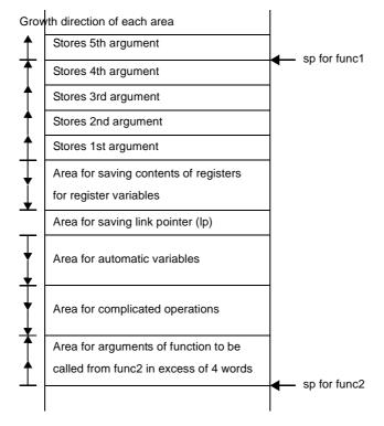
Figure 3-22. Stack Growth Direction of Each Area of Stack Frame
