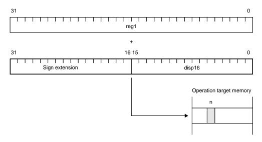
**Remark** n: Bit position specified with 3-bit data (bit#3) (n = 0 to 7)
