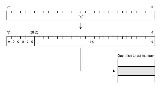
Figure 4-14. Register Addressing (JMP [reg1]) [V850E2]
