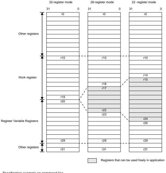
Figure 3-9. Register Modes and Usable Registers
