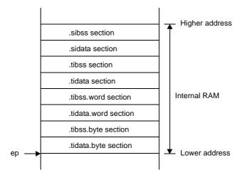
Figure 4-19. Memory Location Image of Internal RAM
