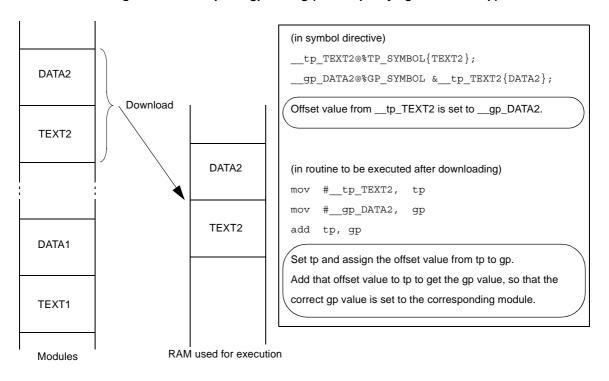
Figure 5-7. Example of gp Setting (When Specifying Offset from tp)
