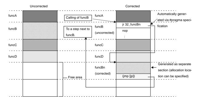
Figure 3-16. Image of Smart Correction Memory
