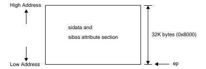
Data with initial values is allocated to the sidata attribute section, and data without initial values is allocated to sibss attribute section. If variables that exceed the upper limit of the sdata and sbss attribute sections that can be accessed from gp with 1 instruction, but which need to be accessed with 1 instruction still exist, they can be allocated in the range that can be accessed with 1 instruction using ep.
