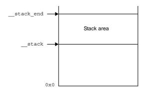
The size of the \_\_stack symbol is specified in the startup module and should therefore be defined in C source in an array as follows.
