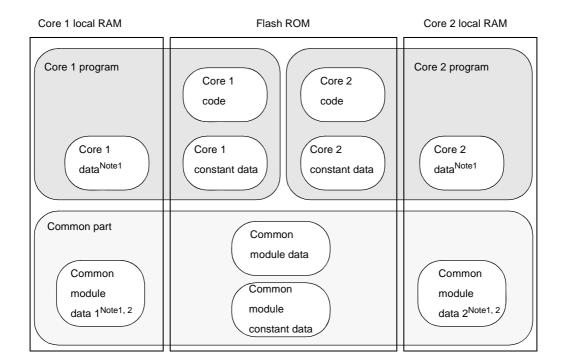
Figure 2-2. Sample Structure of a Multi-core Program
