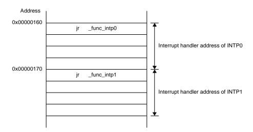
Figure 3-15. Image of Interrupt Handler Address
