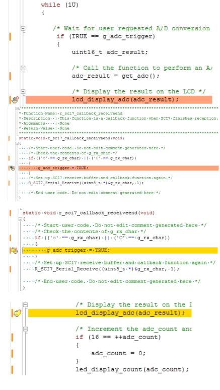
The program proceeds to display the result of the A/D conversion on the LCD and in the terminal window. In addition, the running count of A/D conversions performed is displayed in binary form using LEDs 0-3 on the RSK+. Adjust the potentiometer and press SW3 on the RSK+ and an additional A/D conversion will be performed.
