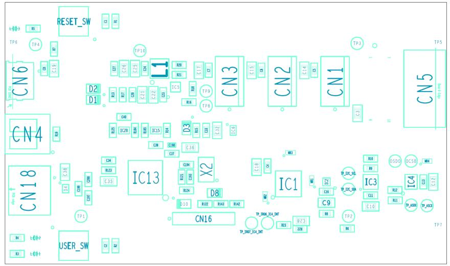
Figure 3-1 : Component Positions on Top Side of Board
