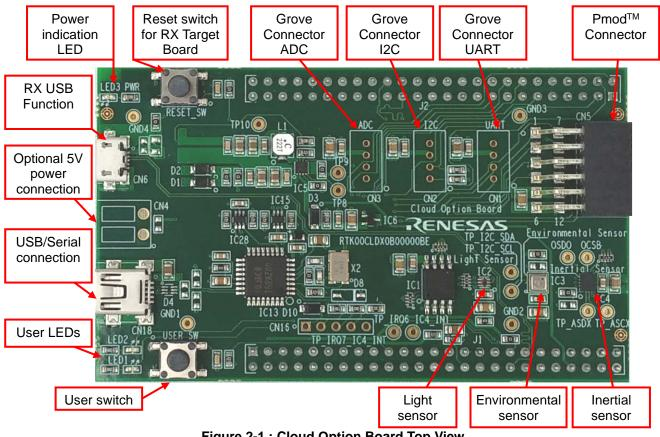
Figure 2-1 : Cloud Option Board Top View
