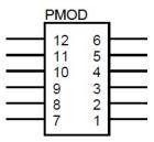
Figure 4-2: Pmod<sup>™</sup> Connector Pin Assignment (Top View)
