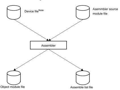
Figure 1-6 Assembler Function
