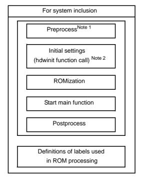
Figure8-1 Overview of Startup Routines
