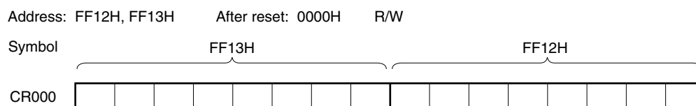
Figure 6-3. Format of 16-Bit Timer Capture/Compare Register 000 (CR000)
