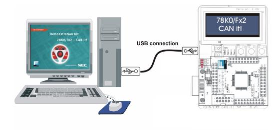
Figure 1: 78K0/Fx2 – CAN it! system configuration
