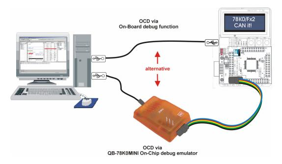
Figure 5: 78K0/Fx2 – CAN it! configuration for On-Chip debugging
