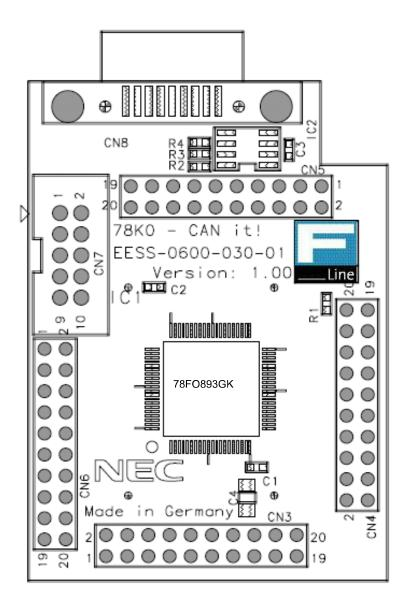
Figure 4: 78K0/Fx2 - CAN it! CPU module components
