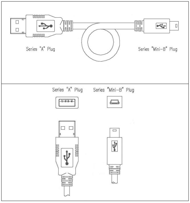
Figure 77: USB interface cable (Mini-B type)
