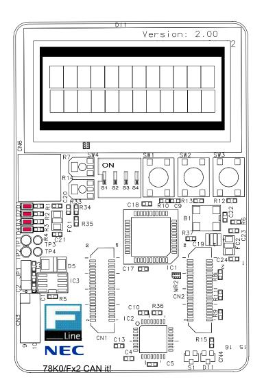
Figure 2: 78K0/Fx2 - CAN it! baseboard connectors, switches and LED's
