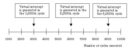
As shown above, virtual interrupts (in this case, timer A0 interrupt) can be generated in any desired cycle.
