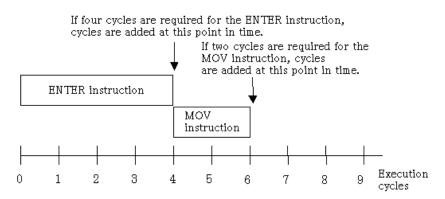
In the above example, no cycles are added while the ENTER or MOV instruction is being executed. The cycles required for each instruction are added after instruction execution. Note that the virtual port input/output and virtual interrupt functions are processed after instruction execution is completed.
