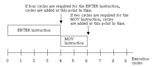
In the above example, no cycles are added while the ENTER or MOV instruction is being executed. The cycles required for each instruction are added after instruction execution. Note that the virtual port input/output and virtual interrupt functions are processed after instruction execution is completed.
