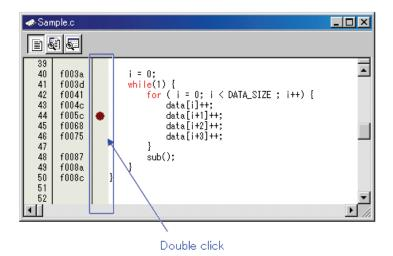
You can delete the break point by double-clicking again in the break point setting area ("S/W breakpoints" column).
