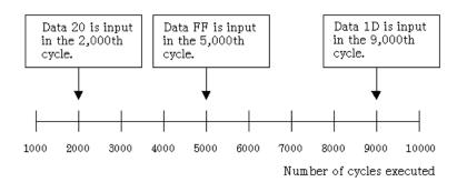
As shown above, data can be input to memory address 3E0 in any desired cycle as specified by the user.
