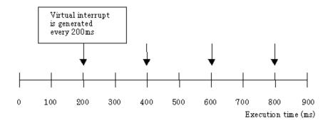
As shown above, virtual interrupts (in this case, timer A0 interrupt) can be generated in interval-synchronized.
