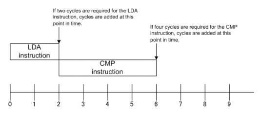
In the above example, no cycles are added while the LDA or CMP instruction is being executed. The cycles required for each instruction are added after instruction execution. Note that the virtual port input/output and virtual interrupt functions are processed after instruction execution is completed. Target program execution time measurement
