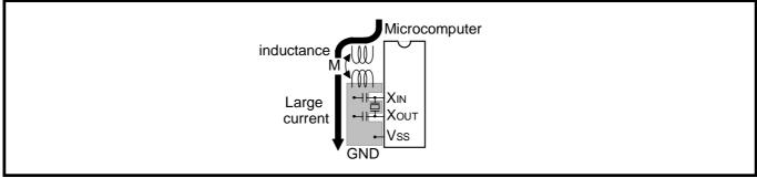
Fig. 3.3.8 Wiring for a large current signal line
