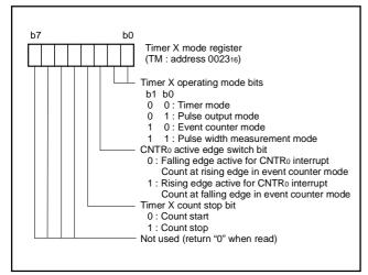
Fig. 16 Structure of timer X mode register
