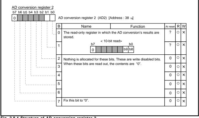
Fig. 2.8.4 Structure of AD conversion register 2
