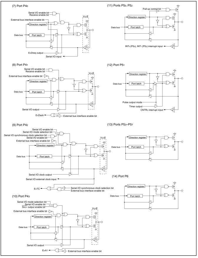
Fig. 11 Port block diagram (2)
