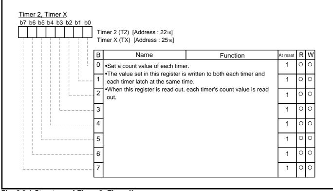
Fig. 2.3.4 Structure of Timer 2, Timer X
