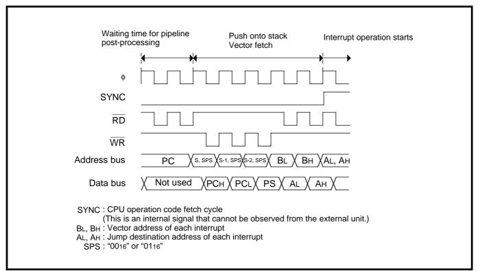
Fig. 2.2.10 Timing chart after acceptance of interrupt request
