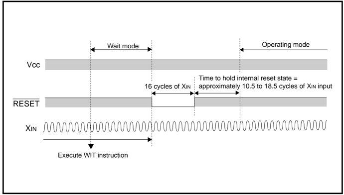
Fig. 2.13.5 Reset input time
