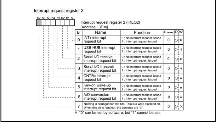
Fig. 2.2.3 Structure of Interrupt request register 2
