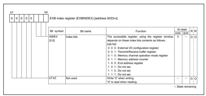
Fig. 111 Structure of EXB index register
