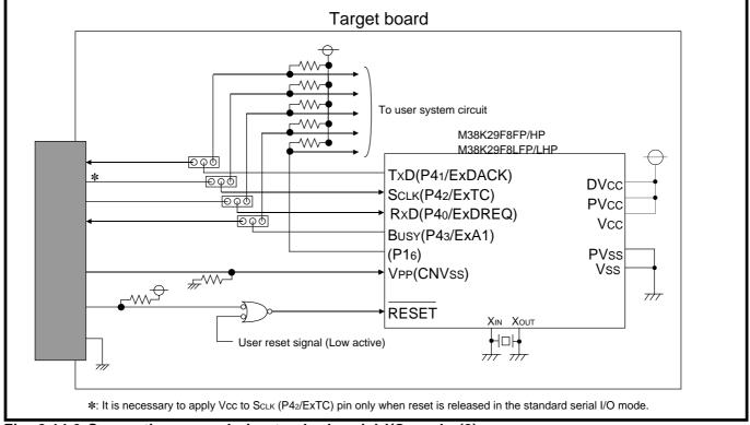
Fig. 2.14.6 Connection example in standard serial I/O mode (2)
