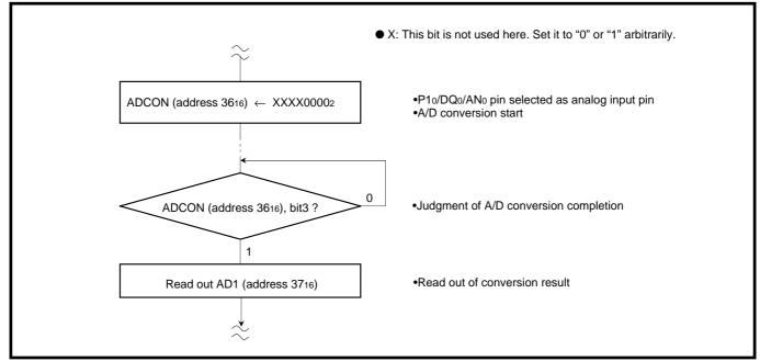
Fig. 2.8.9 Control procedure for 8-bit read
