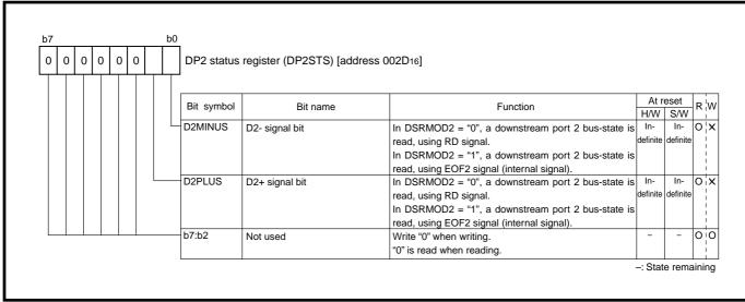
Fig. 3.4.64 Structure of DP2 status register
