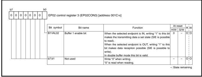
Fig. 3.4.32 Structure of EP02 control register 3
