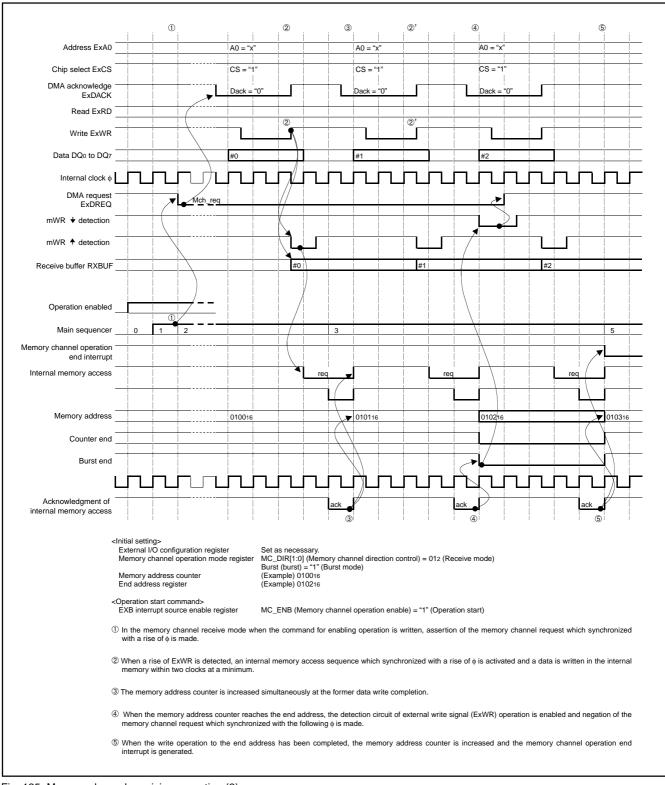
Fig. 125 Memory channel receiving operation (2)
