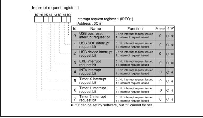
Fig. 2.3.6 Structure of Interrupt request register 1
