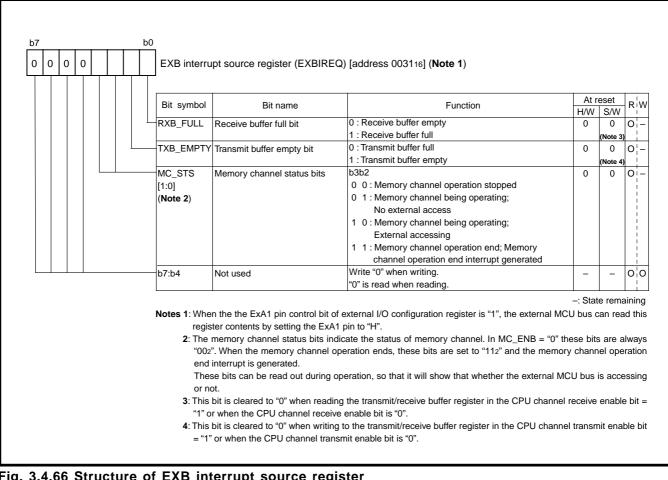
Fig. 3.4.66 Structure of EXB interrupt source register
