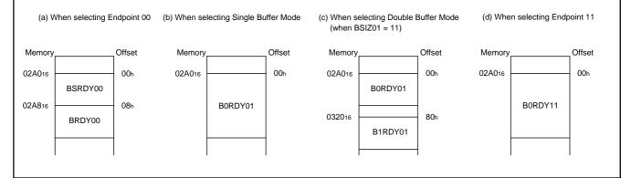
Fig. 28 Examples of interrupt source dependant buffer area offset address
