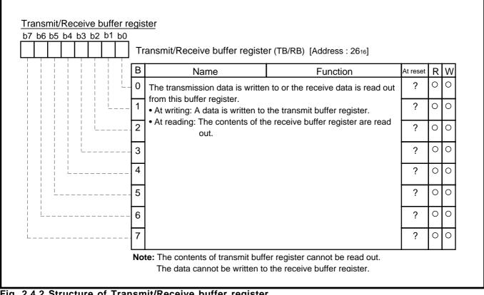
Fig. 2.4.2 Structure of Transmit/Receive buffer register
