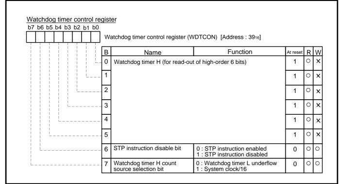
Fig. 3.4.81 Structure of Watchdog timer control register
