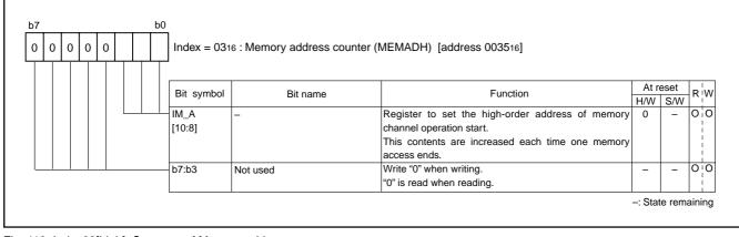
Fig. 119 Index03[high]; Structure of Memory address counter
