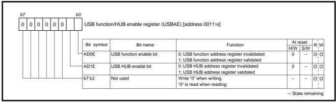
Fig. 3.4.4 Structure of USB function/HUB enable register
