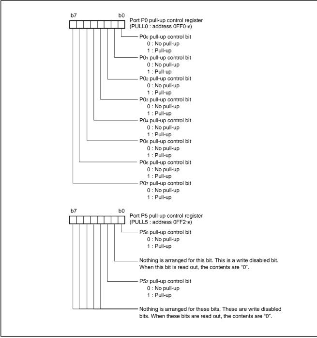
Fig. 12 Structure of port I/O-related registers
