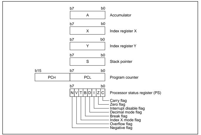
Fig. 5 740 Family CPU register structure
