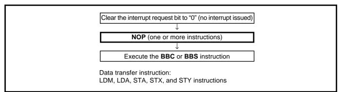
Fig. 2.2.16 Sequence of check of interrupt request bit
