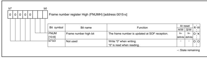
Fig. 36 Structure of Frame number register High
