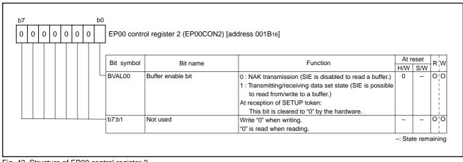
Fig. 42 Structure of EP00 control register 2
