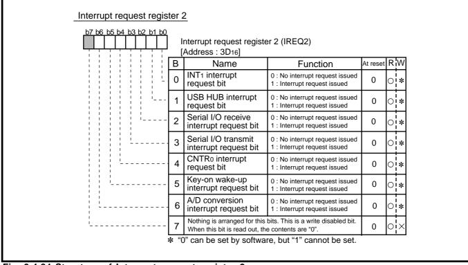
Fig. 3.4.84 Structure of Interrupt request register 2
