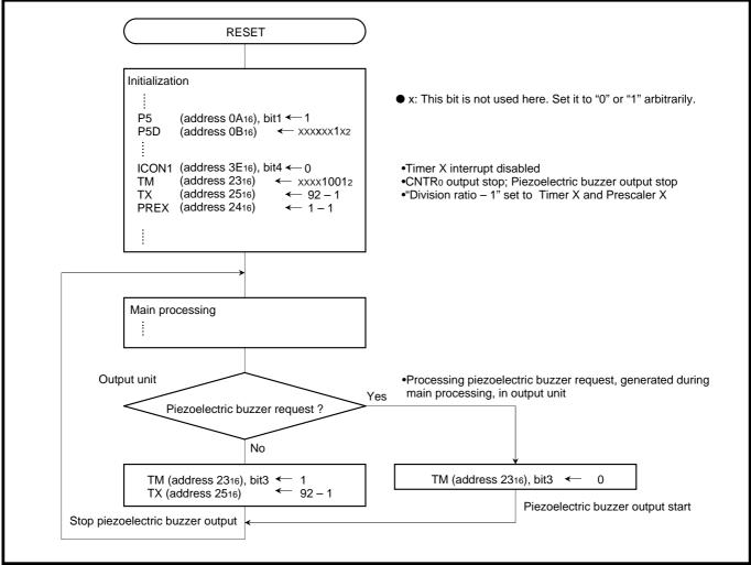
Fig. 2.3.16 Control procedure
