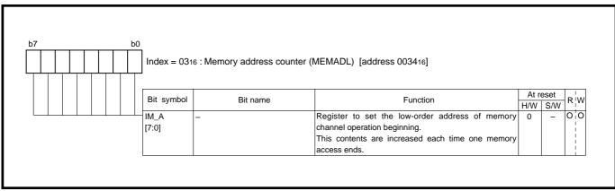
Fig. 3.4.72 Index03[low]; Structure of Memory address counter
