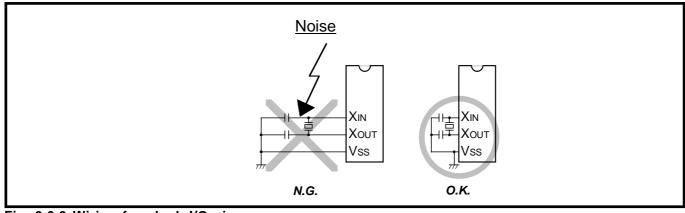
Fig. 3.3.3 Wiring for clock I/O pins
