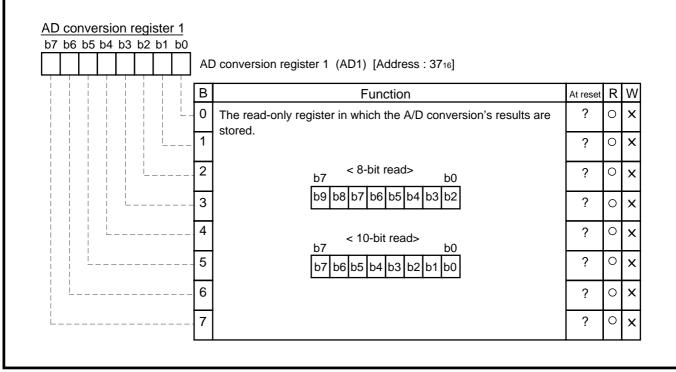
Fig. 3.4.79 Structure of AD conversion register 1
