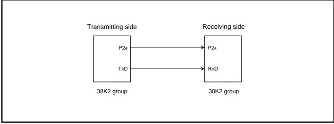
Fig. 2.4.29 Connection diagram (Communication using UART)
