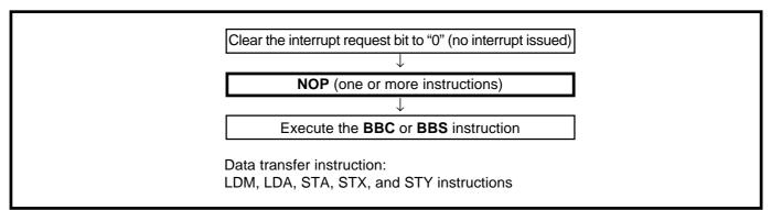
Fig. 3.2.2 Sequence of check of interrupt request bit
