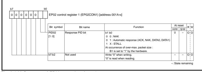
Fig. 3.4.20 Structure of EP02 control register 1
