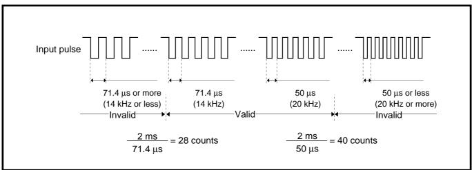
Fig. 2.3.17 Judgment method of valid/invalid of input pulses
