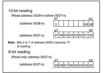
Fig. 133 10-bit/8-bit reading
