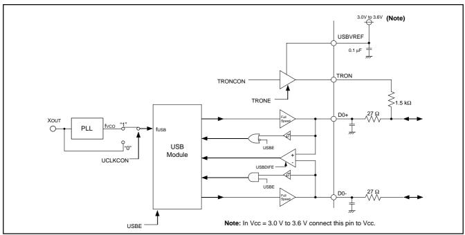
Fig. 26 USB port external circuit (D0+, D0-, USBVREF, TrON) block diagram  $(3.0V \le Vcc \le 4.0V)$
