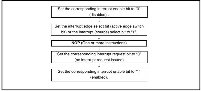
Fig. 2.2.15 Sequence of changing relevant register
