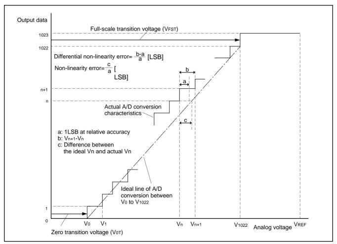
Fig. 167 Definition of A/D conversion accuracy
