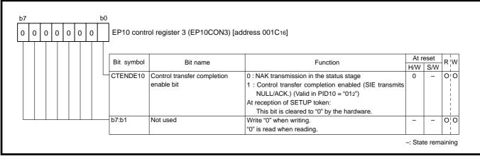
Fig. 3.4.34 Structure of EP10 control register 3
