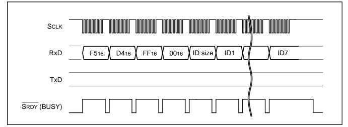
Fig. 163 Timing for ID check
