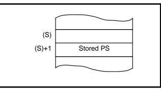
Fig. 3.2.6 Stack memory contents after PHP instruction execution
