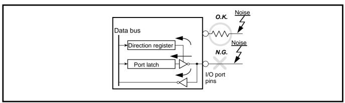
Fig. 3.3.11 Setup for I/O ports
