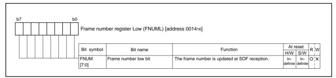
Fig. 35 Structure of Frame number register Low
