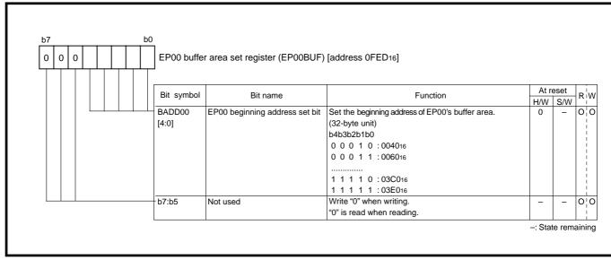
Fig. 3.4.93 Structure of EP00 buffer area set register
