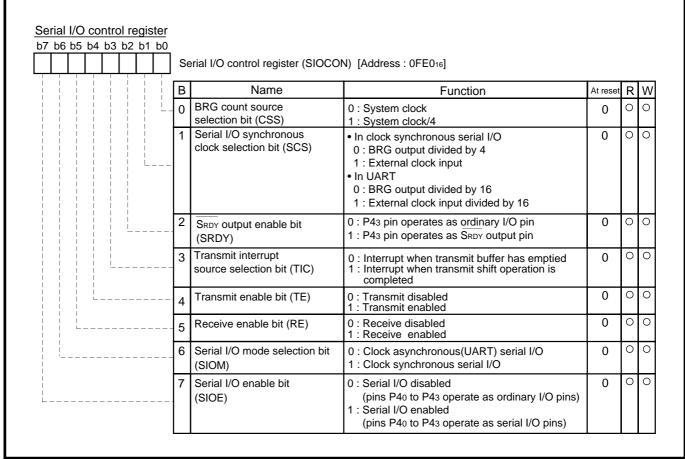
Fig. 3.4.87 Structure of Serial I/O control register
