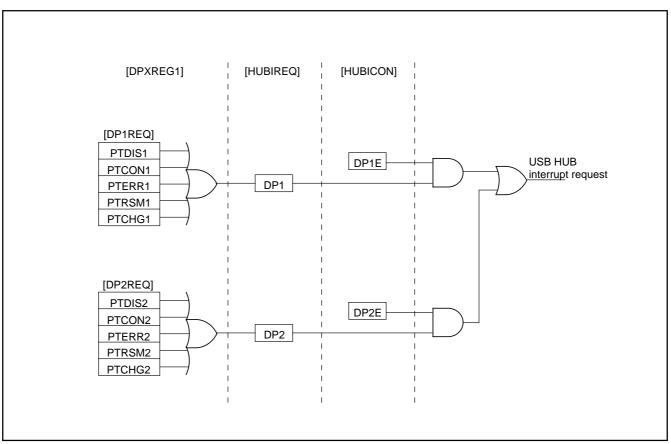
Fig. 91 USB HUB interrupt control
