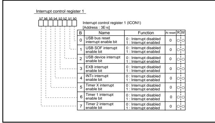
Fig. 3.4.85 Structure of Interrupt control register 1
