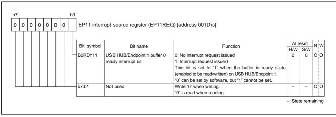
Fig. 84 Structure of EP11 interrupt source register
