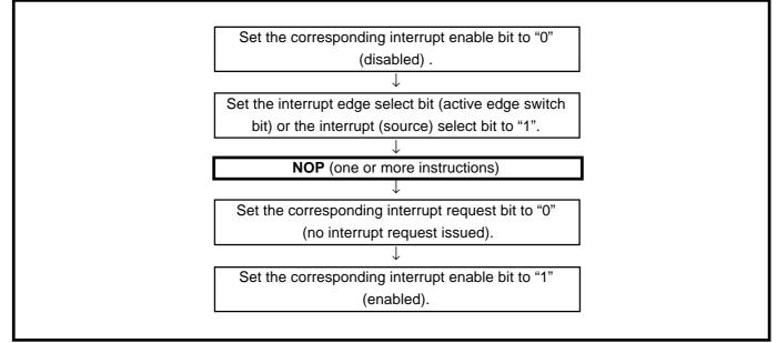
Fig. 3.2.1 Sequence of changing relevant register
