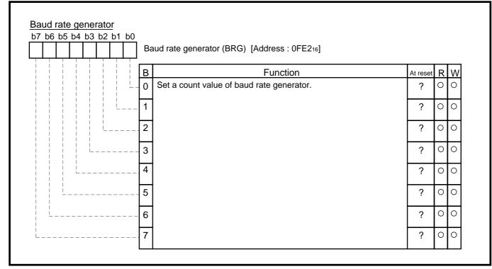
Fig. 3.4.89 Structure of Baud rate generator
