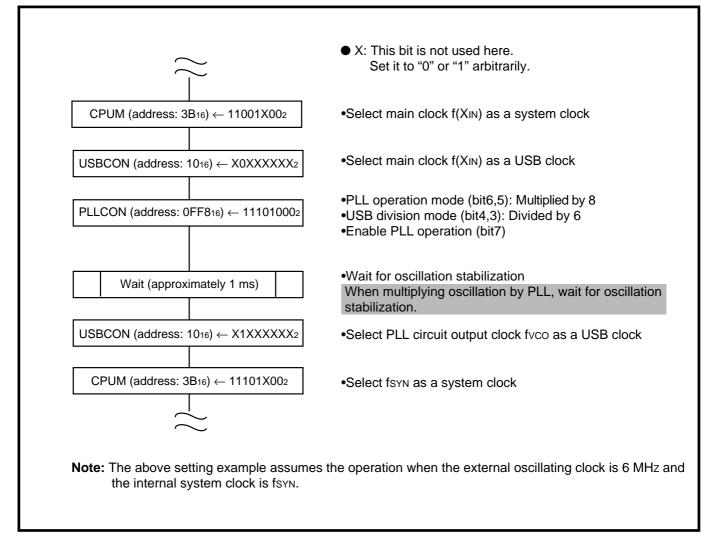
Fig. 2.11.6 Related registers setting when hardware reset
