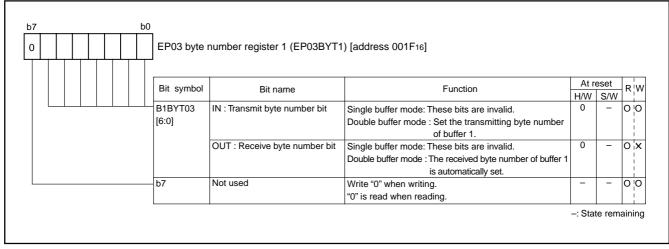
Fig. 71 Structure of EP03 byte number register 1
