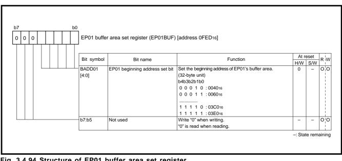
Fig. 3.4.94 Structure of EP01 buffer area set register
