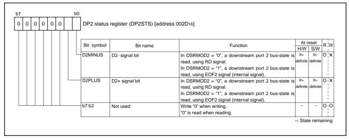
Fig. 101 Structure of DP2 status register
