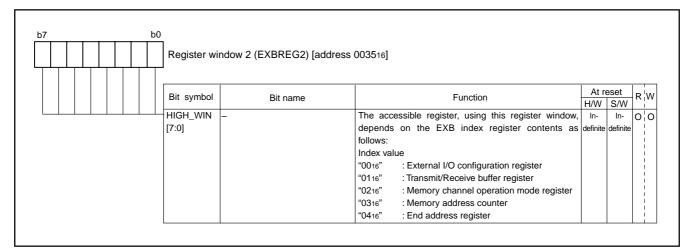
Fig. 113 Structure of Register window 2
