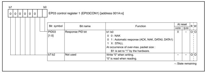
Fig. 66 Structure of EP03 control register 1
