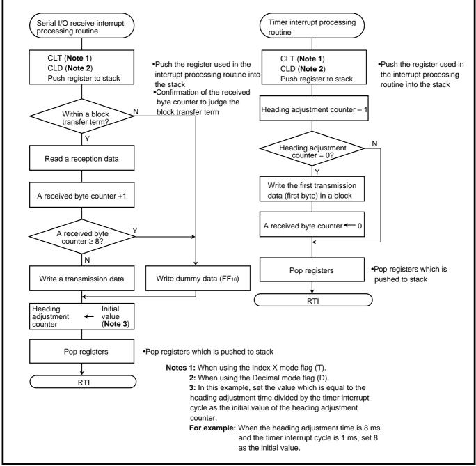
Fig. 2.4.28 Control procedure of slave unit
