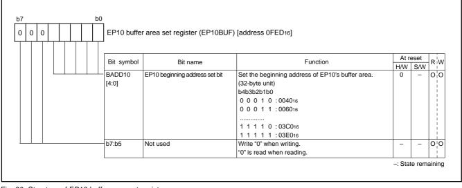
Fig. 80 Structure of EP10 buffer area set register
