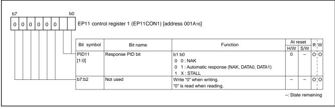
Fig. 82 Structure of EP11 control register 1
