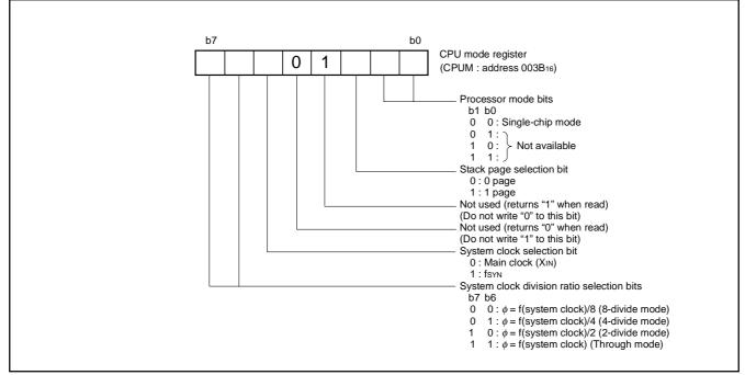
Fig. 7 Structure of CPU mode register
