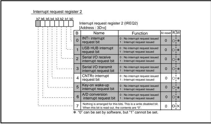
Fig. 2.3.7 Structure of Interrupt request register 2
