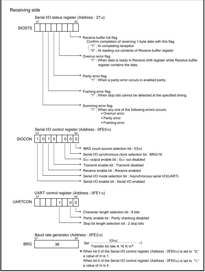
Fig. 2.4.32 Registers setting related to receiving side
