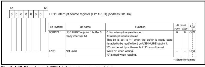
Fig. 3.4.40 Structure of EP11 interrupt source register
