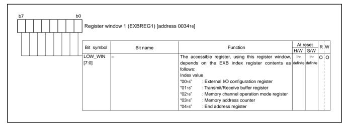
Fig. 112 Structure of Register window 1
