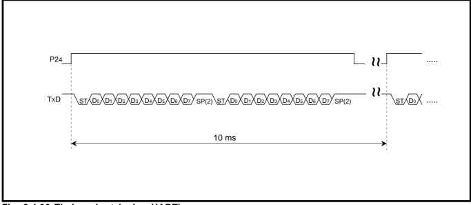
Fig. 2.4.30 Timing chart (using UART)
