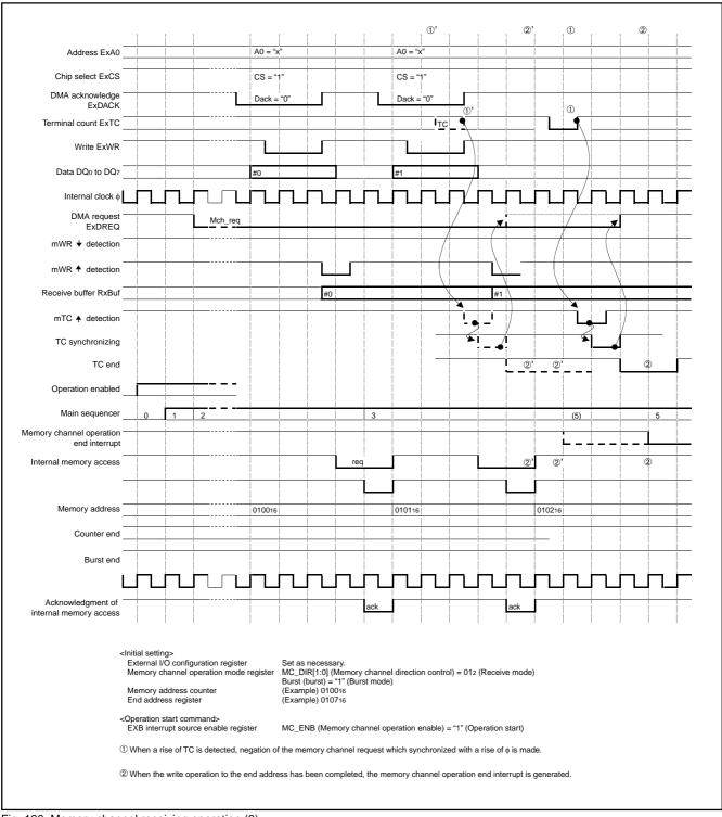
Fig. 126 Memory channel receiving operation (3)
