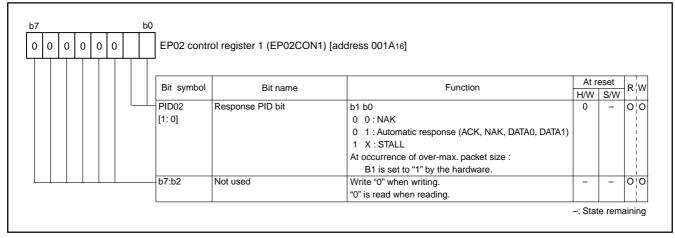
Fig. 57 Structure of EP02 control register 1
