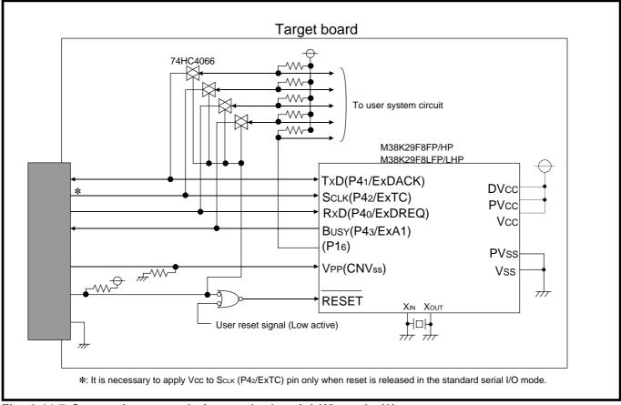
Fig. 2.14.7 Connection example in standard serial I/O mode (3)
