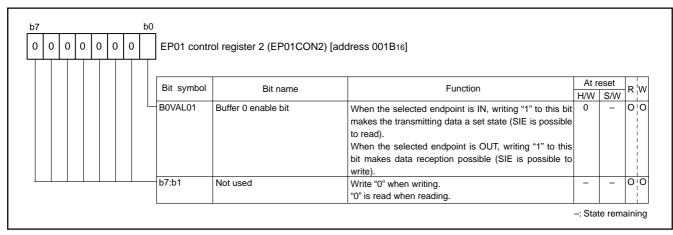
Fig. 49 Structure of EP01 control register 2
