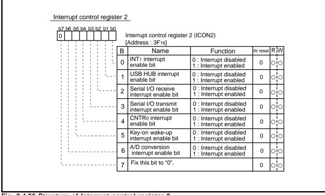
Fig. 3.4.86 Structure of Interrupt control register 2
