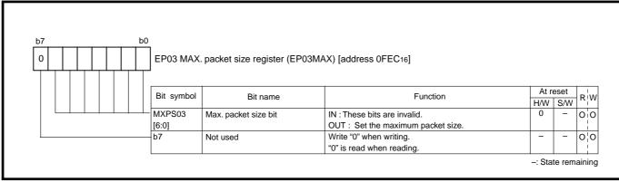
Fig. 3.4.92 Structure of EP03 MAX. packet size register
