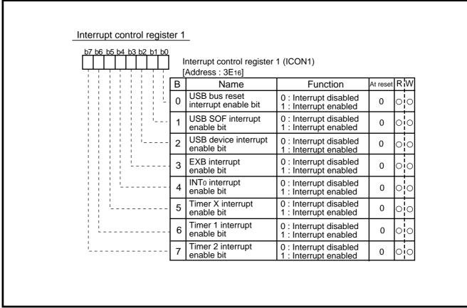
Fig. 2.2.4 Structure of Interrupt control register 1
