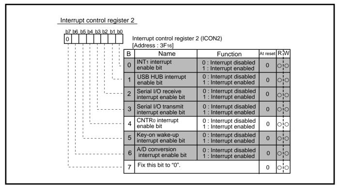
Fig. 2.3.9 Structure of Interrupt control register 2
