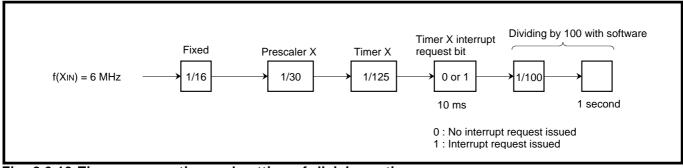
Fig. 2.3.10 Timers connection and setting of division ratios
