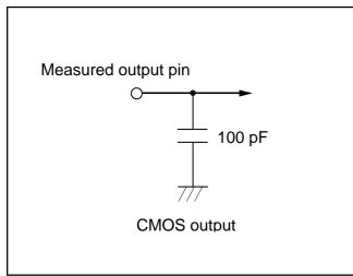
Fig. 3.1.1 Output switching characteristics measurement circuit
