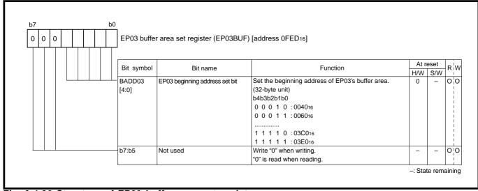
Fig. 3.4.96 Structure of EP03 buffer area set register
