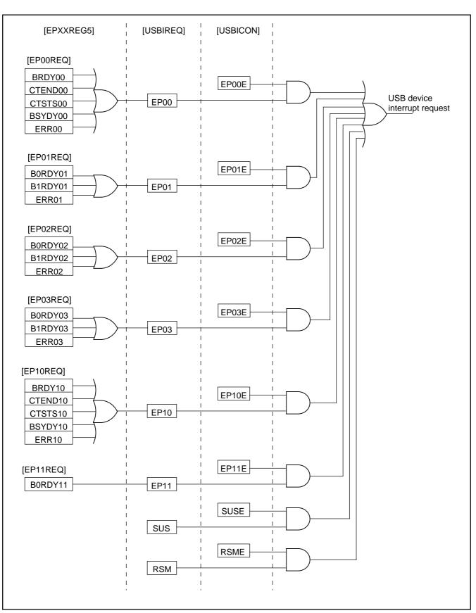
Fig. 29 USB device interrupt control
