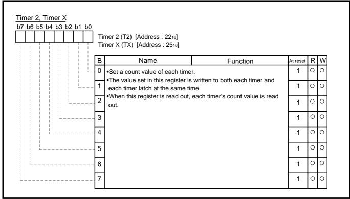
Fig. 3.4.52 Structure of Timer 2, Timer X
