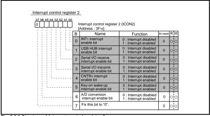
Fig. 2.8.6 Structure of Interrupt control register 2
