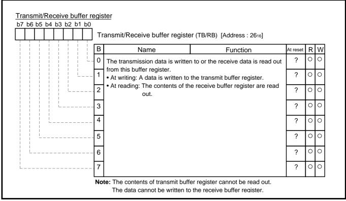
Fig. 3.4.54 Structure of Transmit/Receive buffer register
