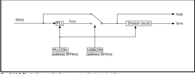
Fig. 2.11.5 Block diagram for frequency synthesizer circuit
