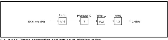
Fig. 2.3.14 Timers connection and setting of division ratios
