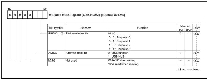
Fig. 39 Structure of Endpoint index register
