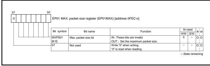
Fig. 3.4.90 Structure of EP01 MAX. packet size register
