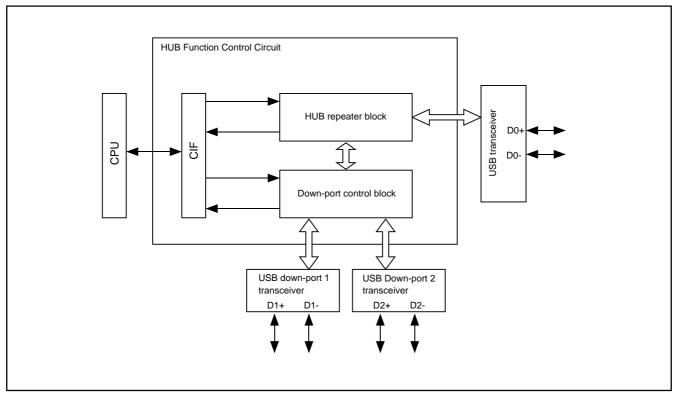
Fig. 88 HUB function control circuit block diagram
