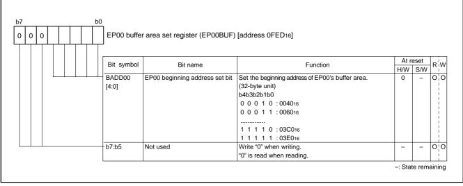
Fig. 46 Structure of EP00 buffer area set register
