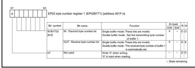
Fig. 3.4.48 Structure of EP02 byte number register 1
