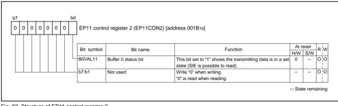
Fig. 83 Structure of EP11 control register 2
