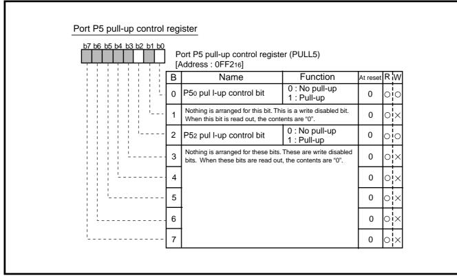
Fig. 3.4.100 Structure of Port P5 pull-up control register
