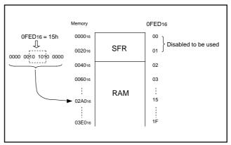
Fig. 27 Example setting of buffer area beginning address
