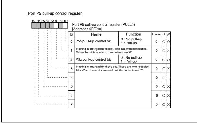
Fig. 2.1.5 Structure of Port P5 pull-up control register
