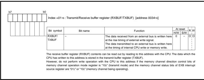
Fig. 3.4.70 Index01[low]; Structure of Transmit/Receive buffer register
