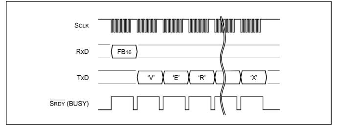
Fig. 161 Timing for version information output
