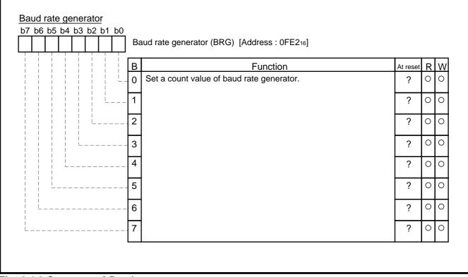
Fig. 2.4.6 Structure of Baud rate generator
