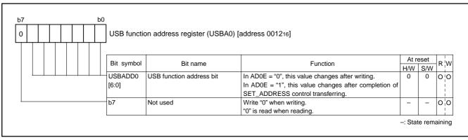
Fig. 33 Structure of USB function address register
