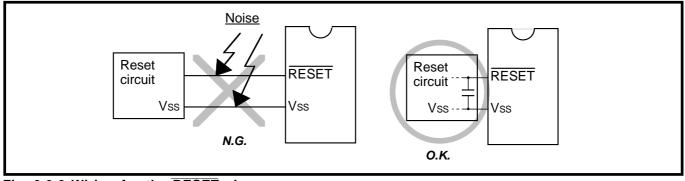
Fig. 3.3.2 Wiring for the RESET pin
