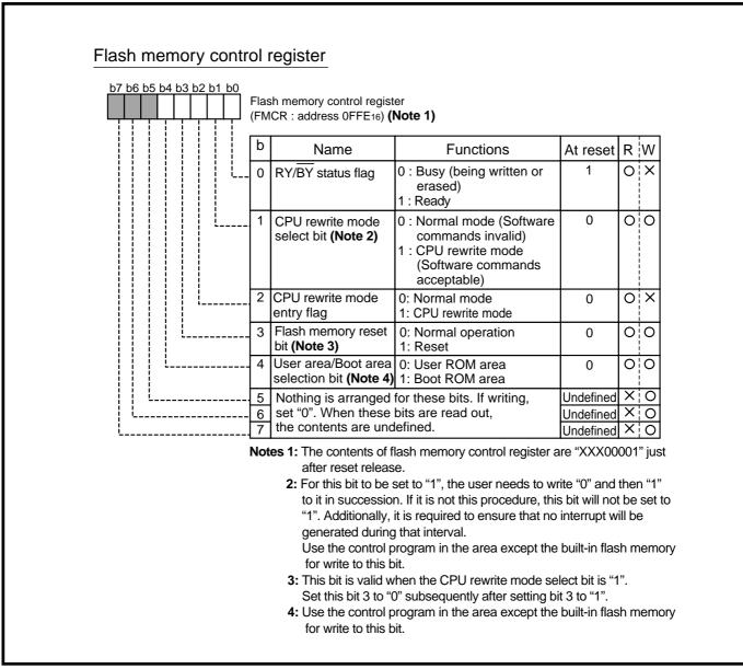
Fig. 2.14.3 Structure of Flash memory control register
