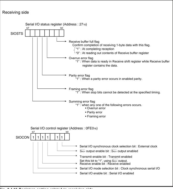
Fig. 2.4.16 Registers setting related to receiving side
