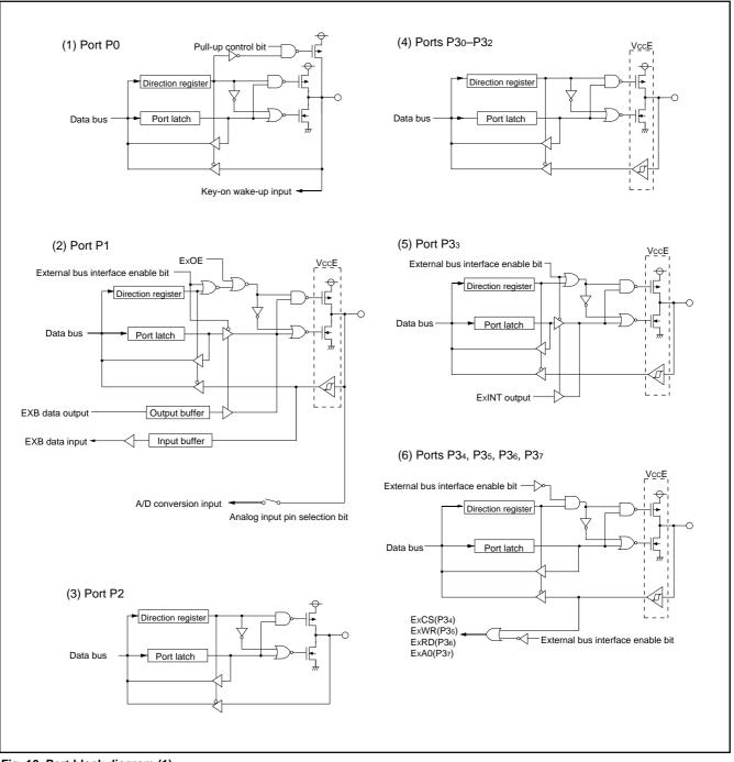
Fig. 10 Port block diagram (1)
