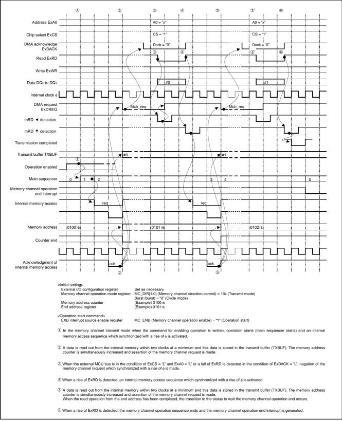
Fig. 127 Memory channel tranmitting operation (1)
