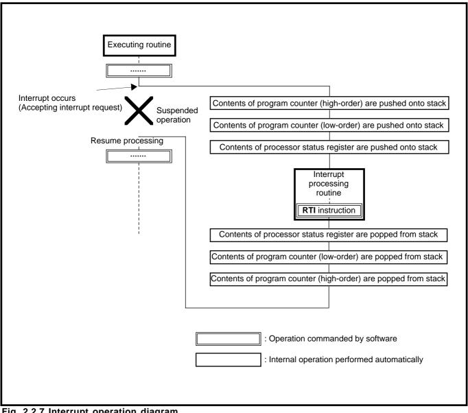
Fig. 2.2.7 Interrupt operation diagram
