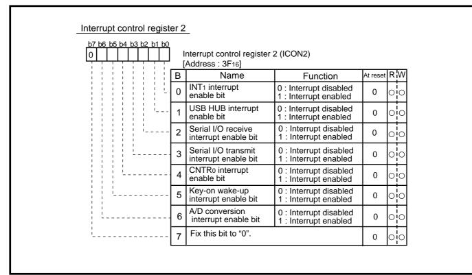
Fig. 2.2.5 Structure of Interrupt control register 2
