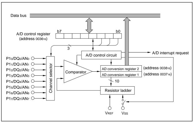
Fig. 134 A/D converter block diagram
