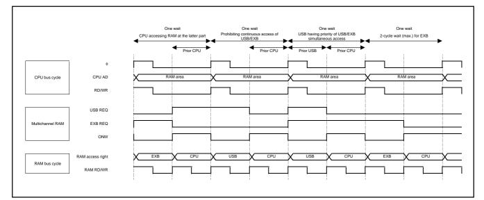
Fig. 130 Multichannel RAM timing diagram (one wait)
