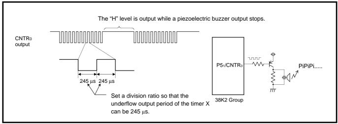
Fig. 2.3.13 Peripheral circuit example
