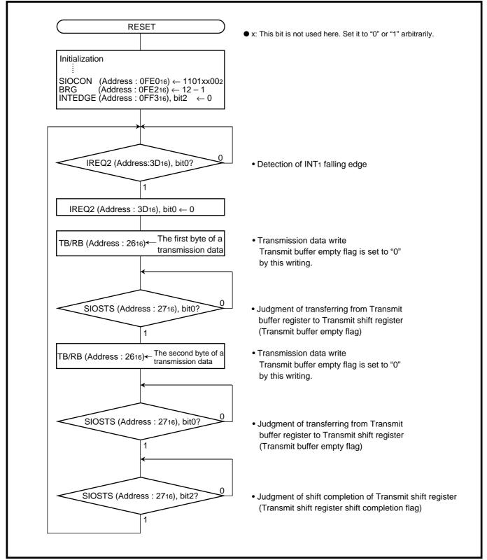
Fig. 2.4.17 Control procedure of transmitting side
