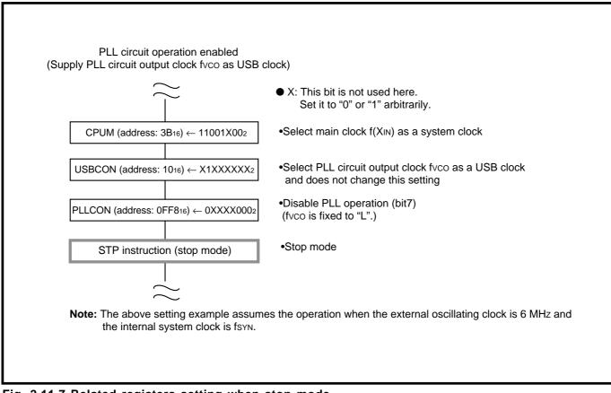
Fig. 2.11.7 Related registers setting when stop mode
