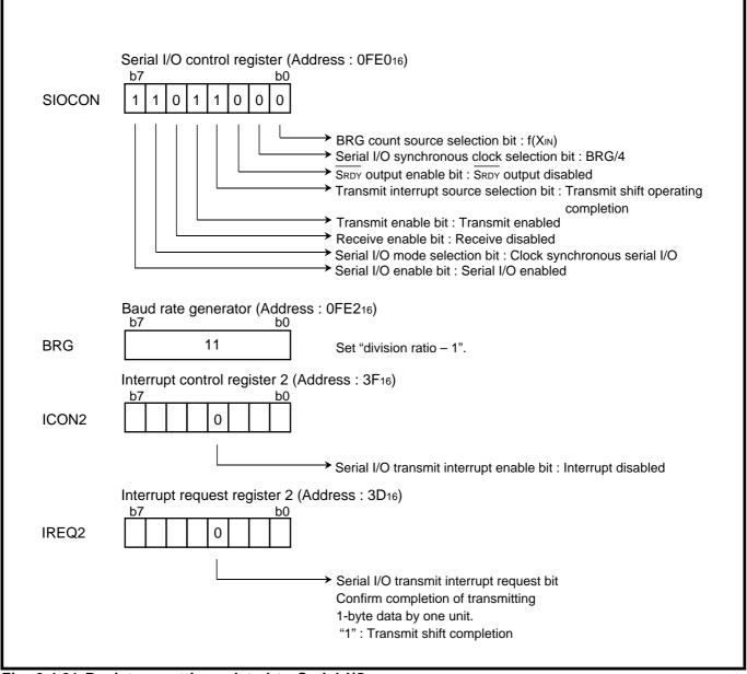
Fig. 2.4.21 Registers setting related to Serial I/O
