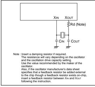
Fig. 141 Ceramic resonator or quartz-crystal oscilltor circuit
