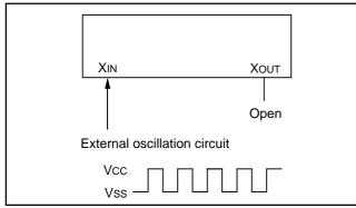
Fig. 142 External clock input circuit
