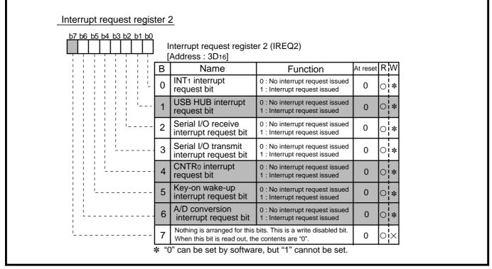
Fig. 2.4.8 Structure of Interrupt request register 2
