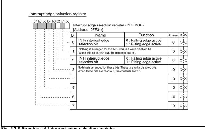
Fig. 2.2.6 Structure of Interrupt edge selection register
