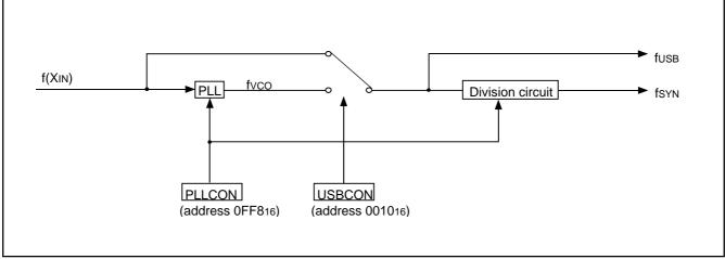
Fig. 139 Block diagram of PLL circuit
