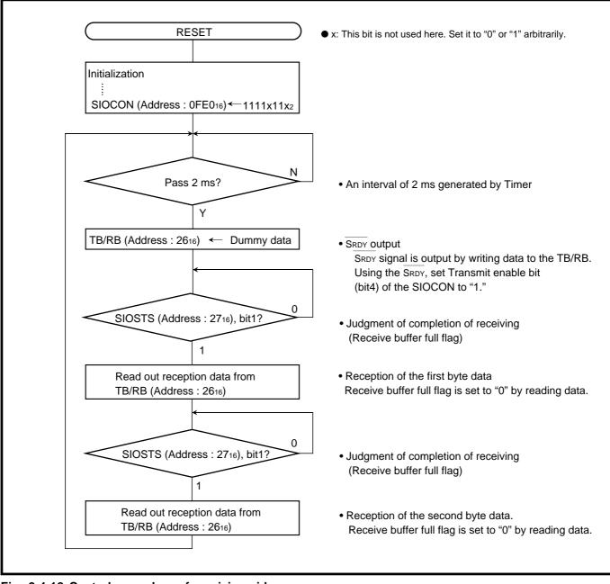
Fig. 2.4.18 Control procedure of receiving side
