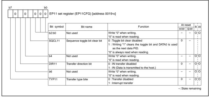
Fig. 81 Structure of EP11 set register
