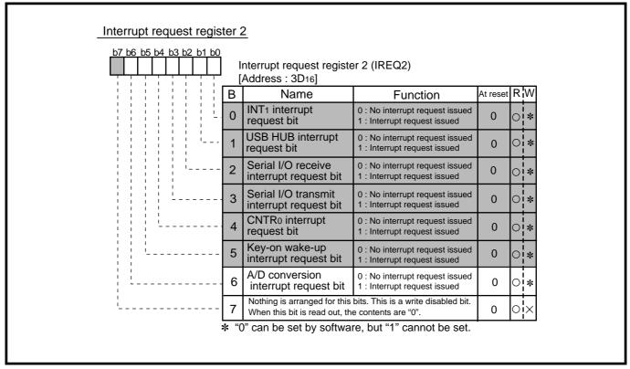
Fig. 2.8.5 Structure of Interrupt request register 2
