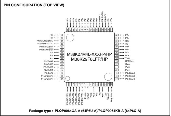
Fig. 1 Pin configuration of 38K2 group
