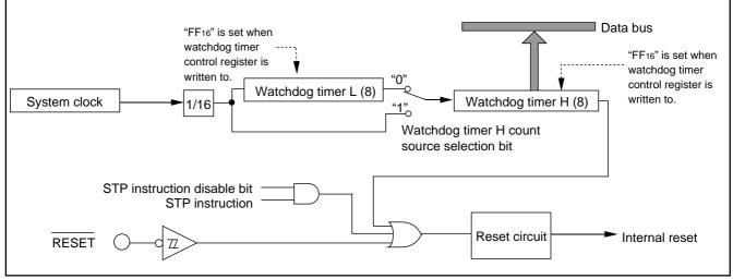
Fig. 135 Block diagram of Watchdog timer
