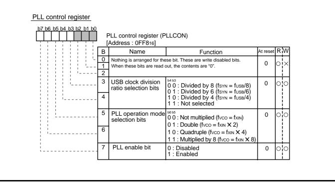
Fig. 3.4.102 Structure of PLL control register
