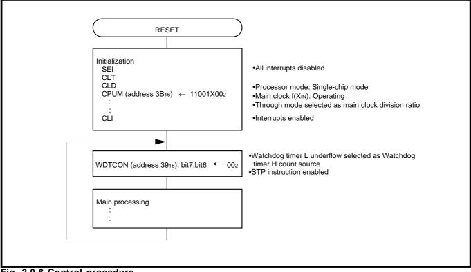
Fig. 2.9.6 Control procedure
