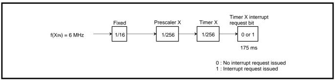
Fig. 2.3.20 Timers connection and setting of division ratios
