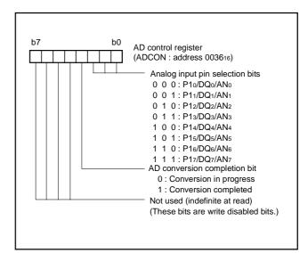
Fig. 132 Structure of AD control register
