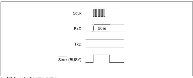
Fig. 157 Timing for clear status register
