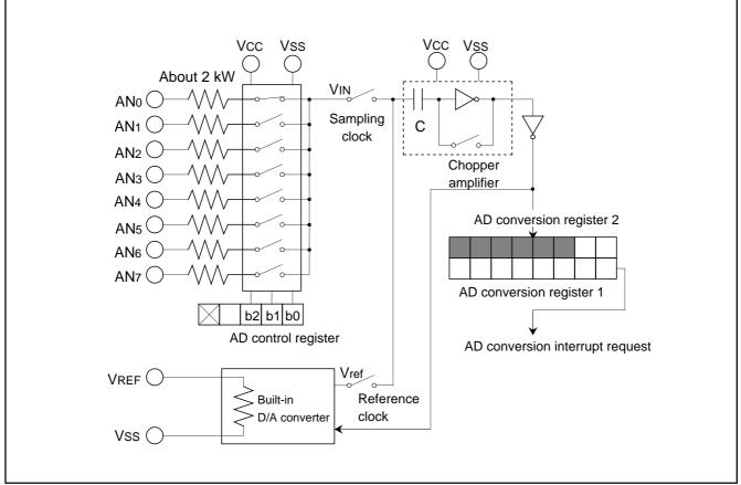
Figures 168 shows the A/D conversion equivalent circuit, and Figure 169 shows the A/D conversion timing chart.
