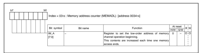
Fig. 118 Index03[low]; Structure of Memory address counter
