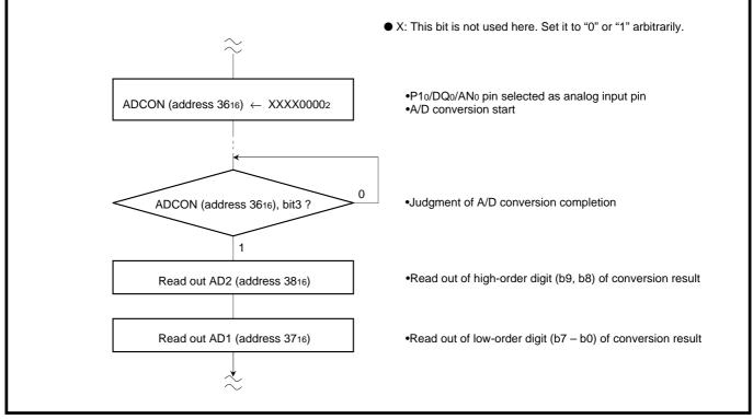
Fig. 2.8.10 Control procedure for 10-bit read
