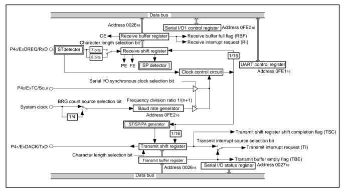
Fig. 20 Block diagram of UART serial I/O
