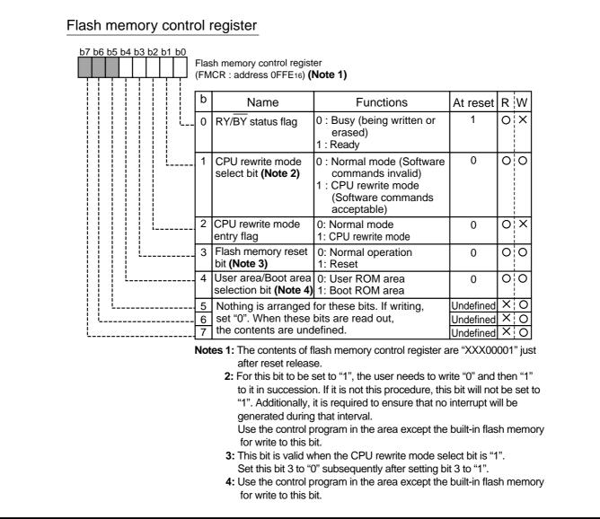
Fig. 3.4.105 Structure of Flash memory control register
