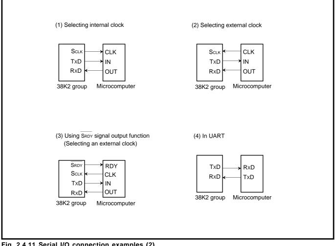
Fig. 2.4.11 Serial I/O connection examples (2)
