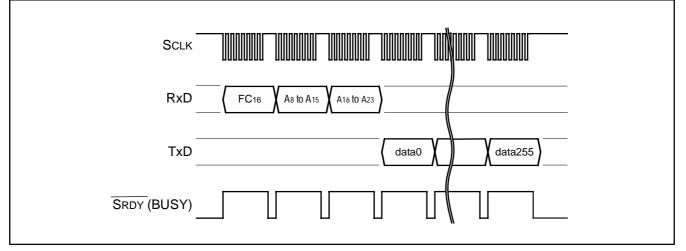
Fig. 162 Timing for Boot ROM area output
