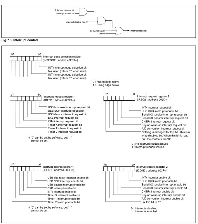
Fig. 14 Structure of interrupt-related registers
