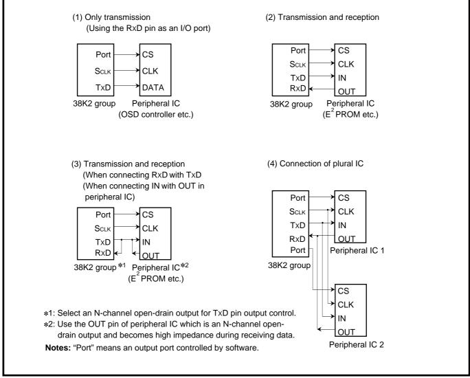
Fig. 2.4.10 Serial I/O connection examples (1)
