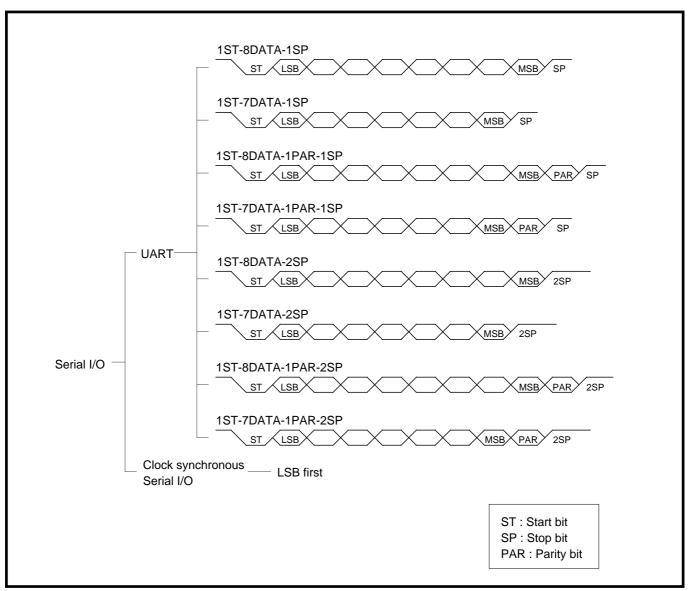
Fig. 2.4.12 Serial I/O transfer data format
