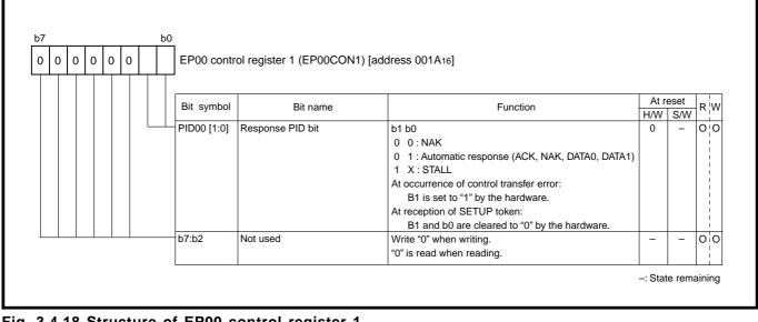
Fig. 3.4.18 Structure of EP00 control register 1
