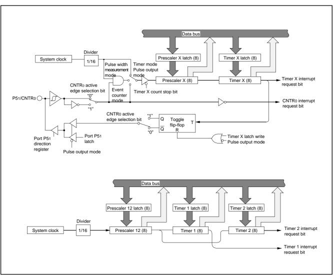
Fig. 17 Timer block diagram
