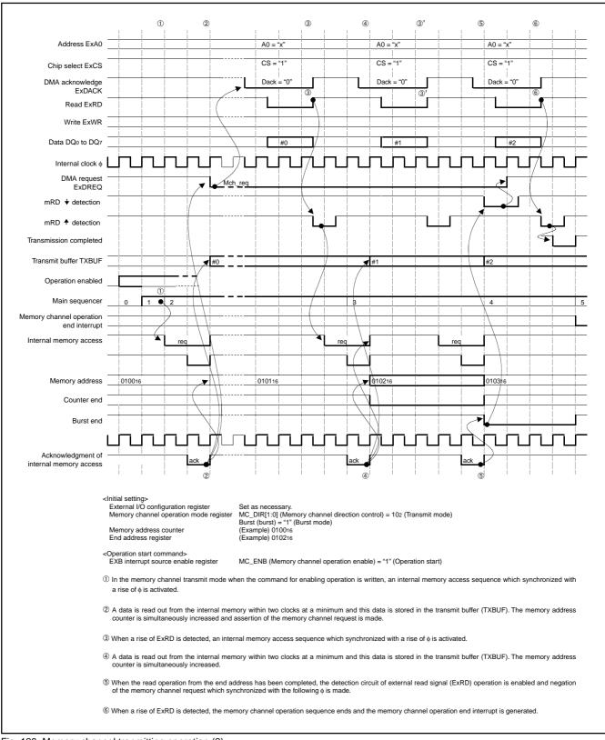
Fig. 128 Memory channel tranmitting operation (2)
