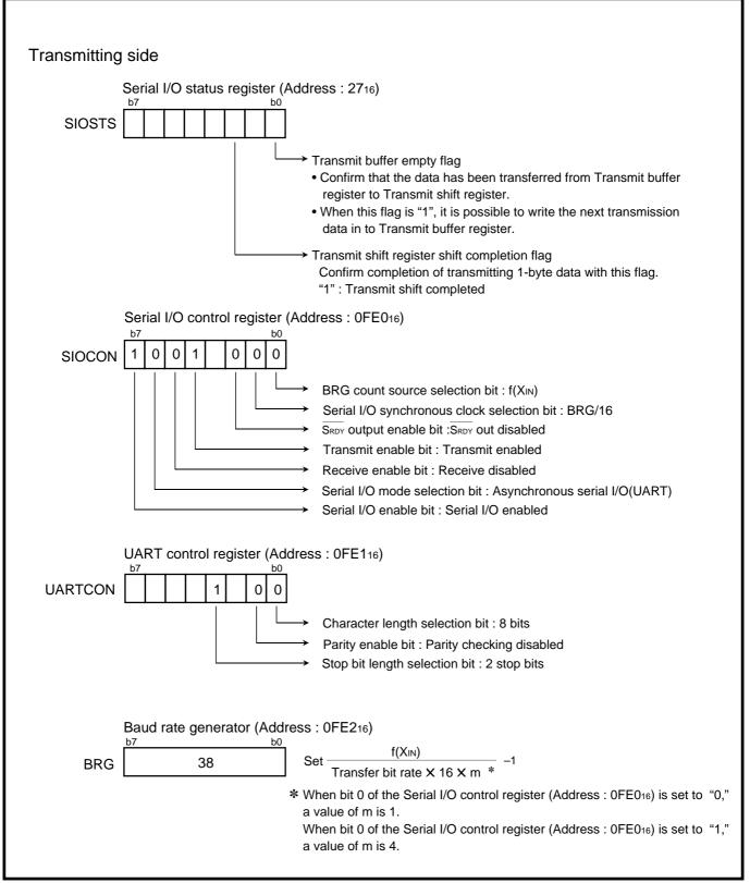
Fig. 2.4.31 Registers setting related to transmitting side
