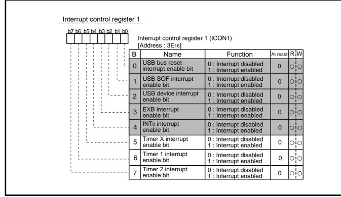
Fig. 2.3.8 Structure of Interrupt control register 1
