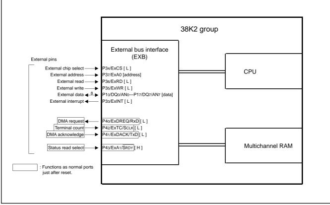
Fig. 105 External bus interface (EXB) pin assignment
