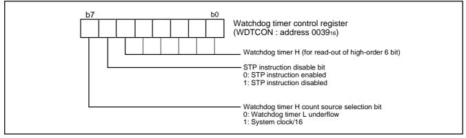
Fig. 136 Structure of Watchdog timer control register
