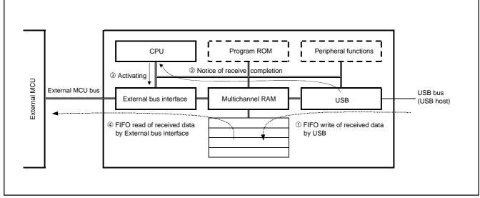
Fig. 131 Multichannel RAM operation example
