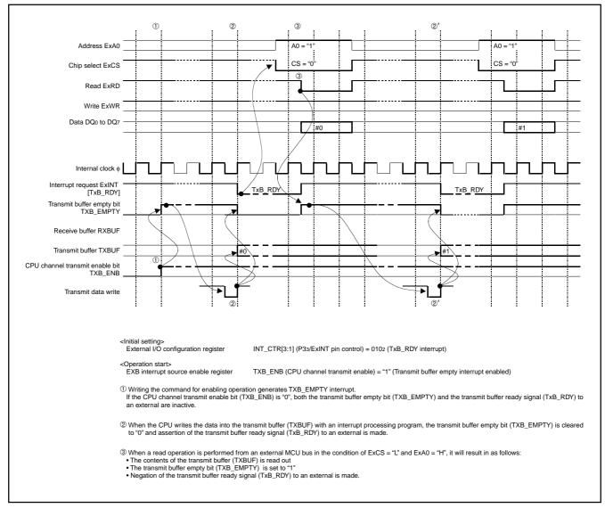
Fig. 123 CPU channel tranmitting operation
