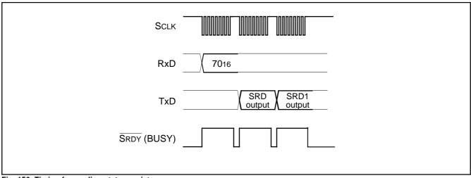
Fig. 156 Timing for reading status register
