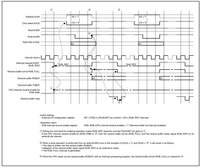
Fig. 122 CPU channel receiving operation
