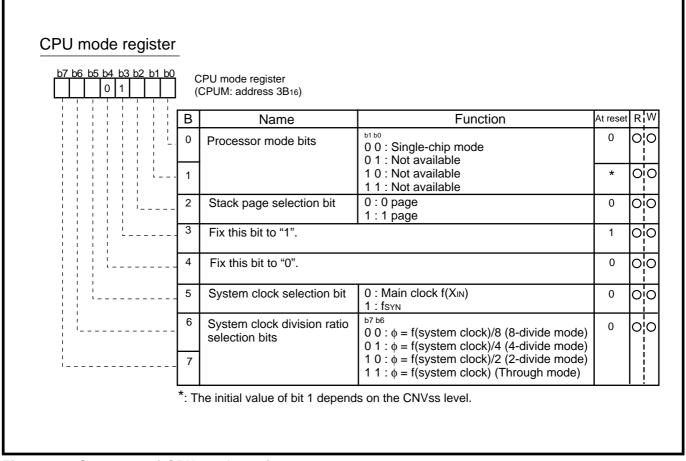
Fig. 3.4.82 Structure of CPU mode register
