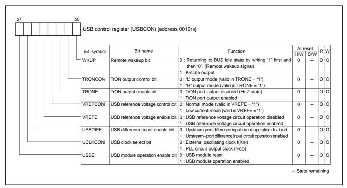
Fig. 31 Structure of USB control register
