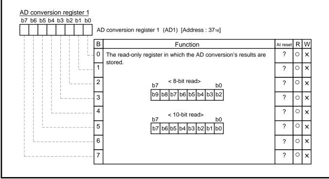
Fig. 2.8.3 Structure of AD conversion register 1
