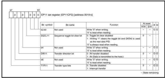
Fig. 3.4.17 Structure of EP11 set register
