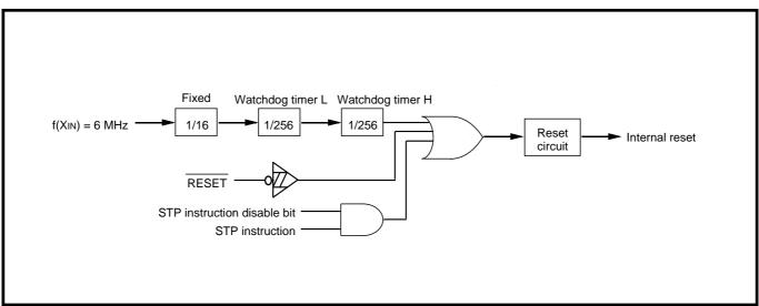
Fig. 2.9.4 Watchdog timer connection and division ratio setting
