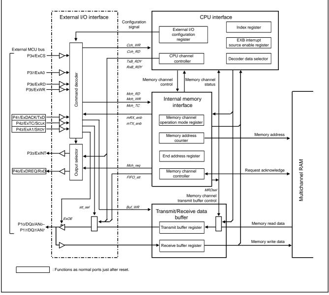
Fig. 106 Block diagram of external bus interface (EXB)
