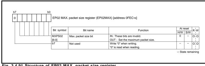
Fig. 3.4.91 Structure of EP02 MAX. packet size register
