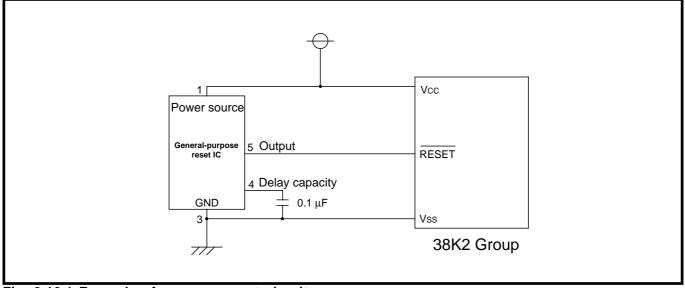
Fig. 2.10.1 Example of poweron reset circuit
