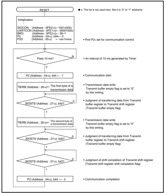
Fig. 2.4.33 Control procedure of transmitting side
