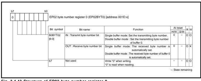
Fig. 3.4.43 Structure of EP02 byte number register 0
