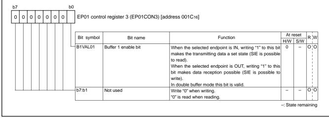
Fig.50 Structure of EP01 control register 3
