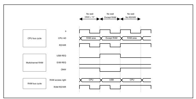
Fig. 129 Multichannel RAM timing diagram (no wait)
