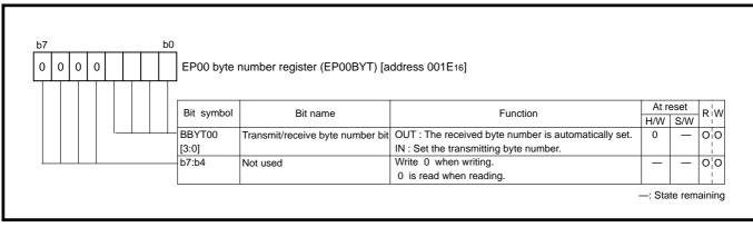
Fig. 3.4.41 Structure of EP00 byte number register
