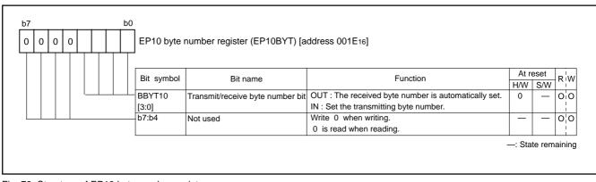
Fig. 79 Structure of EP10 byte number register
