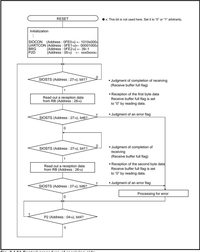
Fig. 2.4.34 Control procedure of receiving side
