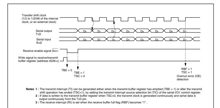
Fig. 19 Operation of clock synchronous serial I/O function
