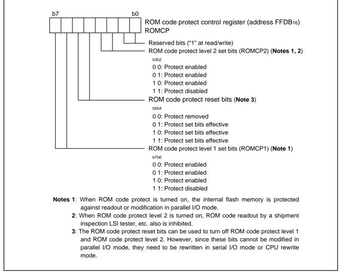
Fig. 152 Structure of ROM code protect control register
