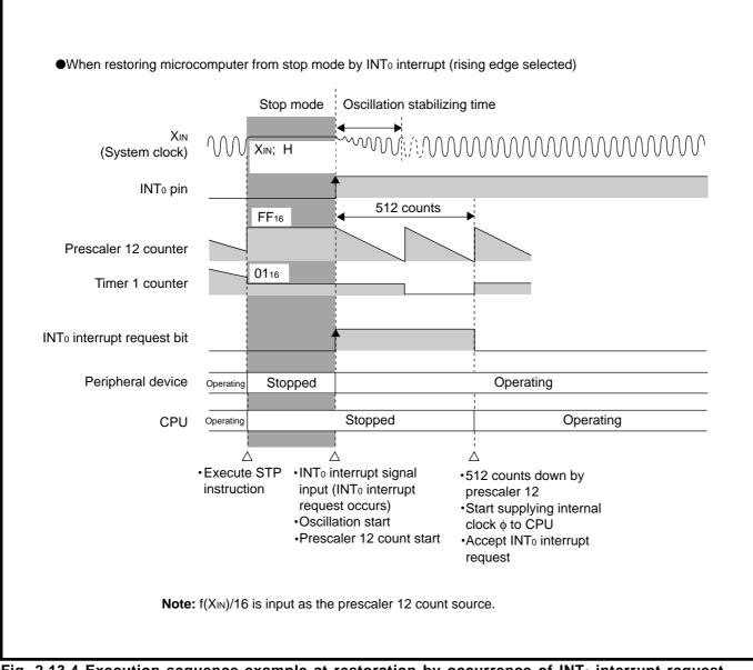
Fig. 2.13.4 Execution sequence example at restoration by occurrence of INT<sub>0</sub> interrupt request
