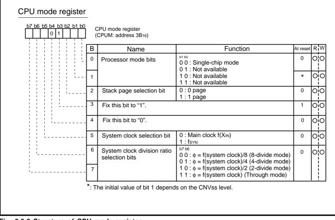
Fig. 2.9.3 Structure of CPU mode register
