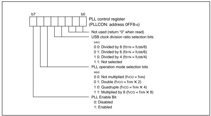
Fig. 140 Structure of PLL control register
