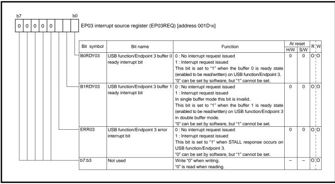
Fig. 3.4.38 Structure of EP03 interrupt source register
