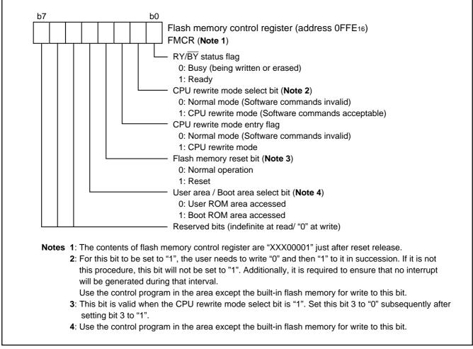
Fig. 147 Structure of flash memory control register
