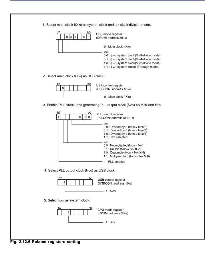
**Note:** When selecting f<sub>SYN</sub> as an internal system clock, refer to "2.11 Frequency synthesizer (PLL)" for details concerning how to generate f<sub>USB</sub> (USB clock) from f(X<sub>IN</sub>) and the notes on PLL circuit.
