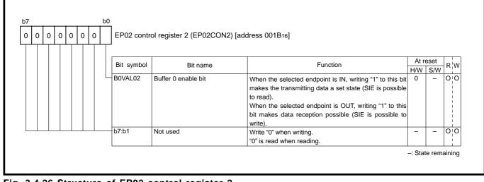
Fig. 3.4.26 Structure of EP02 control register 2
