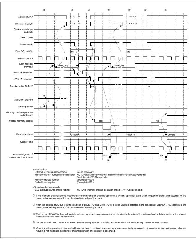
Fig. 124 Memory channel receiving operation (1)
