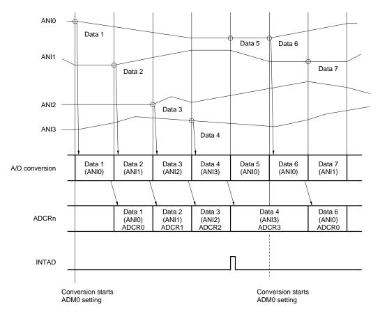
Figure 11-8. Operation Timing Example of Scan Mode: 4-Channel Scan (ANI0 to ANI3)
