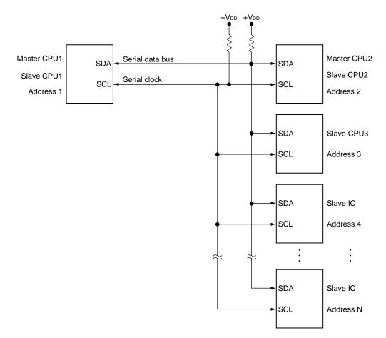
Figure 10-8. Serial Bus Configuration Example Using I<sup>2</sup>C Bus
