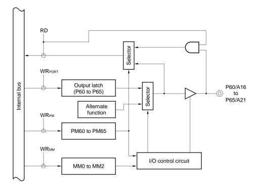
Figure 16-33. Block Diagram of P60 to P65
