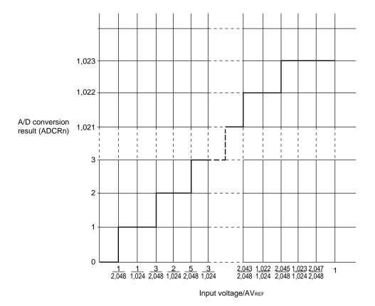
Figure 11-5. Relation between Analog Input Voltage and A/D Conversion Result
