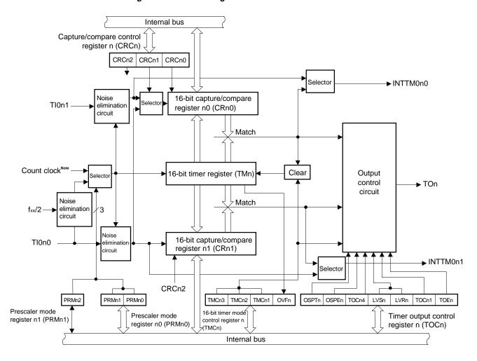
Figure 7-50. Block Diagram of TM0 and TM1
