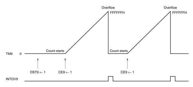
Figure 7-35. Operation after Occurrence of Overflow (When OST9 = 1)
