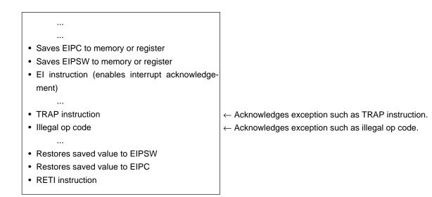
Priorities 0 to 7 (0 is the highest) can be programmed for each maskable interrupt request for multiple interrupt processing control. To set a priority level, write values to the xxPRn0 to xxPRn2 bits of the interrupt request control register (xxICn) corresponding to each maskable interrupt request. At reset, the interrupt request is masked by the xxMKn bit, and the priority level is set to 7 by the xxPRn0 to xxPRn2 bits.
