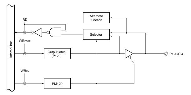
Figure 16-51. Block Diagram of P120
