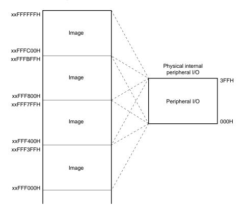
Figure 3-9. Internal Peripheral I/O Area
