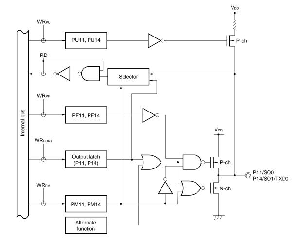
Figure 16-12. Block Diagram of P11 and P14
