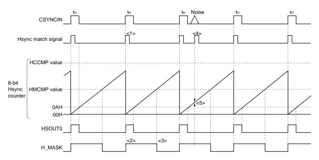
Figure 15-9. Hsync Signal Mask Operation
