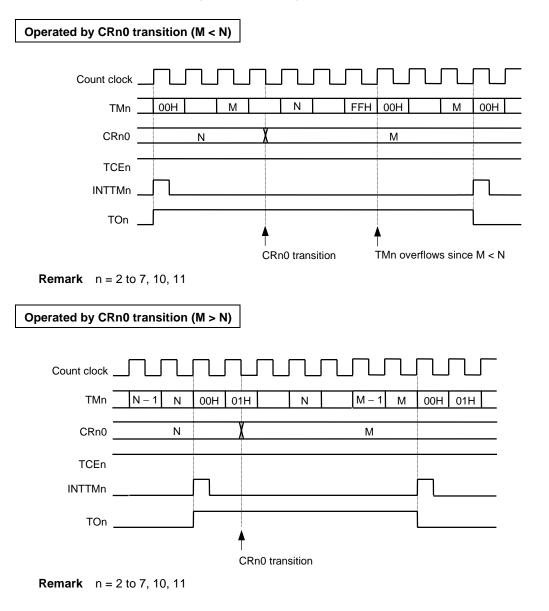
Figure 7-91. Timing of Interval Timer Operation (3/3)
