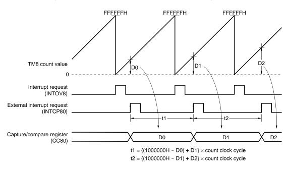
Figure 7-47. Example of Frequency Measurement Timing (Timer 8)
