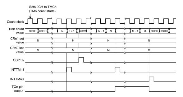
Figure 7-78. Timing of One-Shot Pulse Output Operation with Software Trigger
