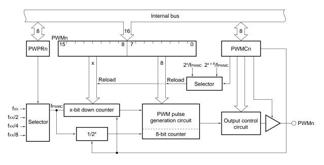
Figure 14-1. Block Diagram of PWM Function
