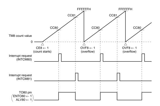
Figure 7-33. Example of TM8 Compare Operation (Set/Reset Output Mode)
