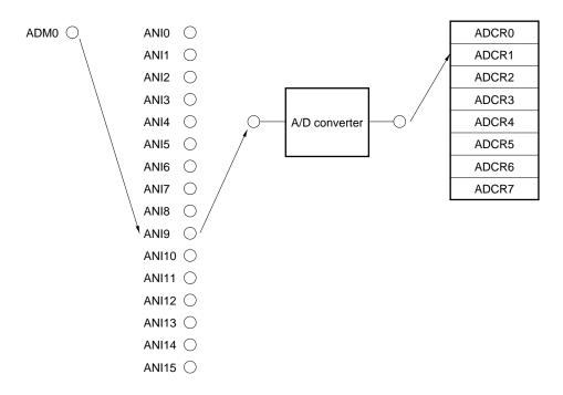
Figure 11-9. Example of 1-Buffer Mode (A/D Trigger Select 1-Buffer) Operation (ANI9)
