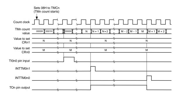
Figure 7-80. Timing of One-Shot Pulse Output Operation with External Trigger (with Rising Edge Specified)
