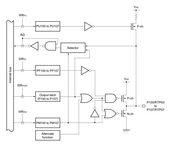
Figure 16-44. Block Diagram of P100 to P107
