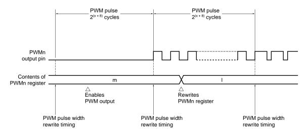
Figure 14-10. Example 1 of PWM Output Timing (PWM Pulse Width Rewrite Cycle 2<sup>(x+8)</sup>/fpwmc)
