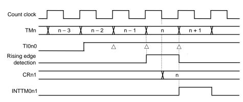
Figure 7-66. CRn1 Capture Operation with Rising Edge Specified
