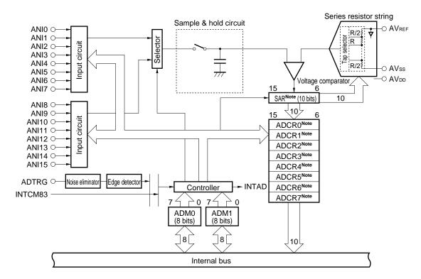
Figure 11-1. Block Diagram of A/D Converter
