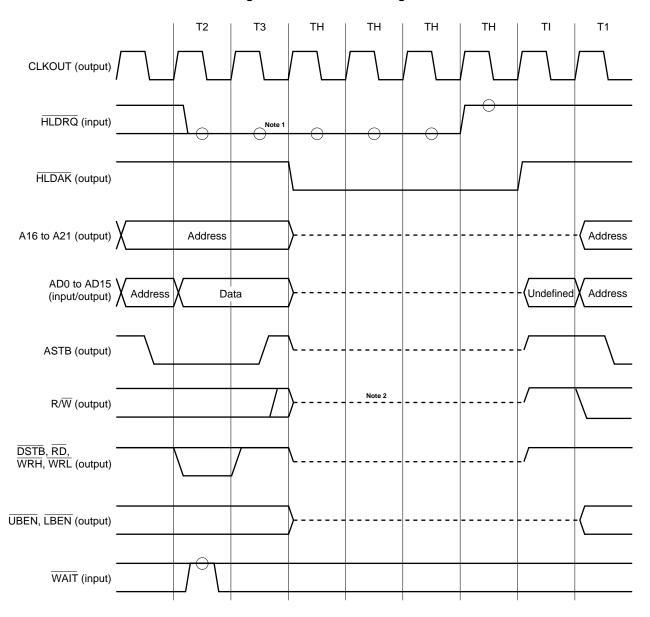
Figure 4-16. Bus Hold Timing
