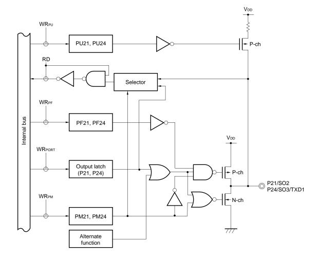
Figure 16-19. Block Diagram of P21 and P24
