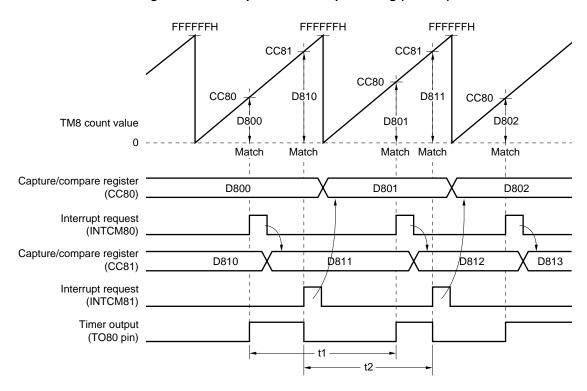
Figure 7-44. Example of PWM Output Timing (Timer 8)
