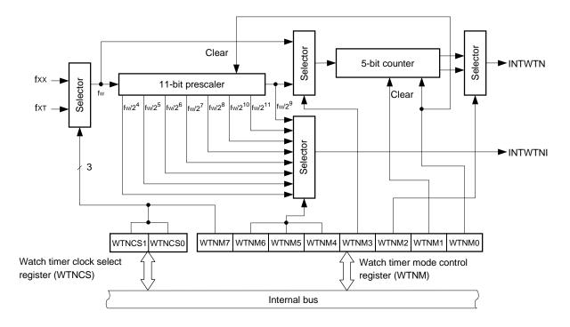
Figure 8-1. Block Diagram of Watch Timer
