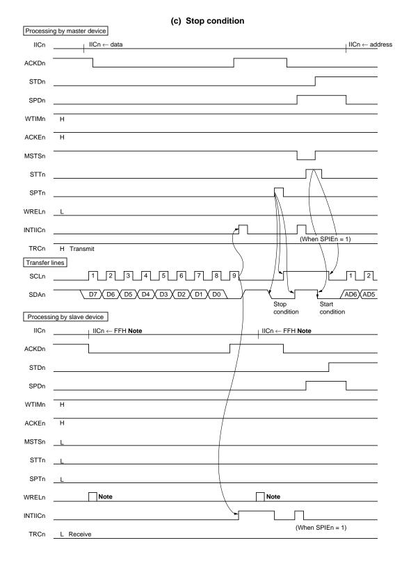
Figure 10-29. Example of Master to Slave Communication (When 9-Clock Wait Is Selected for Both Master and Slave) (3/3)
