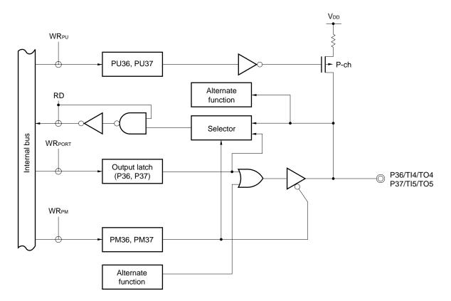
Figure 16-27. Block Diagram of P36 and P37
