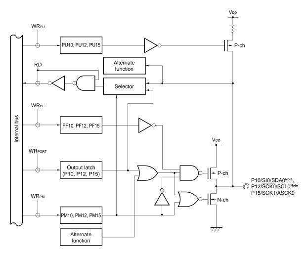
Figure 16-11. Block Diagram of P10, P12, and P15
