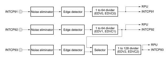
Figure 7-19. INTCP9n Inputs (n = 1 to 3)
