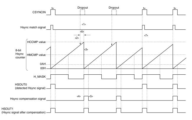
Figure 15-10. Hsync Signal Self-Generation
