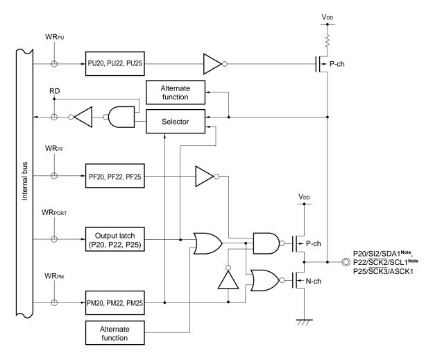
Figure 16-18. Block Diagram of P20, P22, and P25
