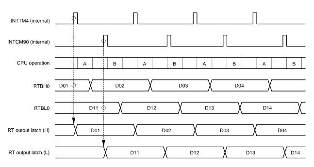
Figure 13-5. Example of Operation Timing of RTO (When EXTR0 = 0, BYTE0 = 0)
