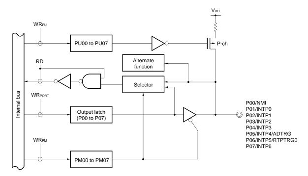
Figure 16-6. Block Diagram of P00 to P07
