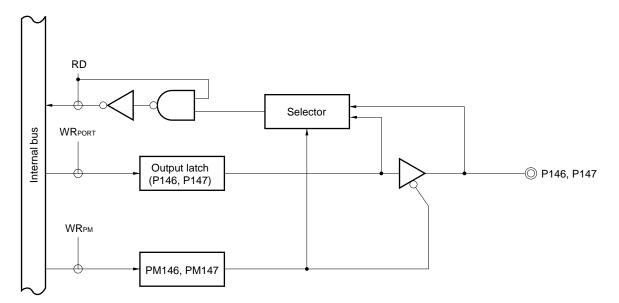
Figure 16-67. Block Diagram of P146 and P147
