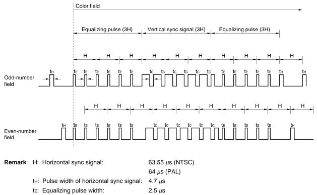
tc: Serrated pulse width:  $4.4 \,\mu s$
