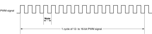
Figure 14-5. Basic Operations of PWM
