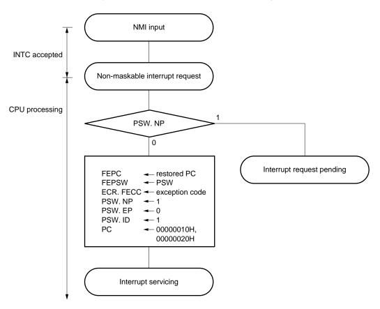
Figure 5-1. Non-Maskable Interrupt Servicing
