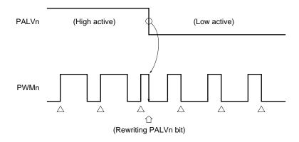
Figure 14-9. Setting of Active Level of PWM Output
