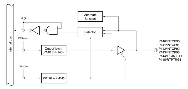
Figure 16-66. Block Diagram of P140 to P145
