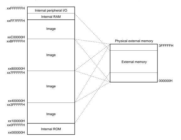
Figure 3-11. External Memory Area (When Expanded to 4 Mbytes)
