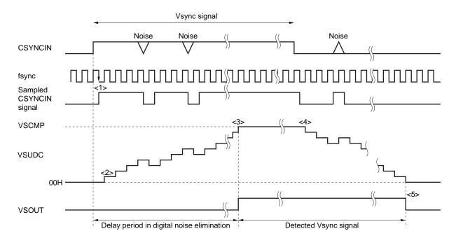
Figure 15-7. Vsync Signal Separation
