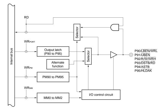
Figure 16-38. Block Diagram of P90 to P95
