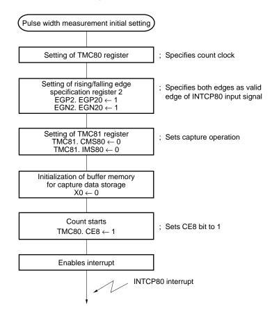
Figure 7-42. Example of Setting Procedure for Pulse Width Measurement (Timer 8)
