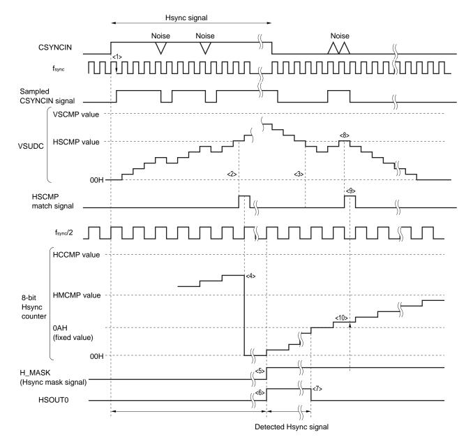
Figure 15-8. Hsync Signal Separation
