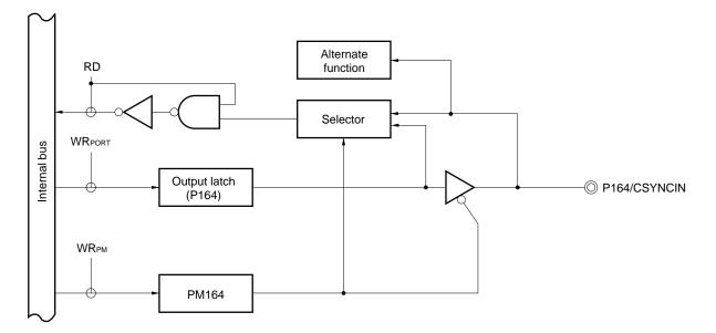
Figure 16-74. Block Diagram of P164
