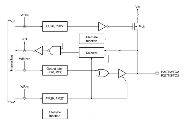
Figure 16-21. Block Diagram of P26 and P27
