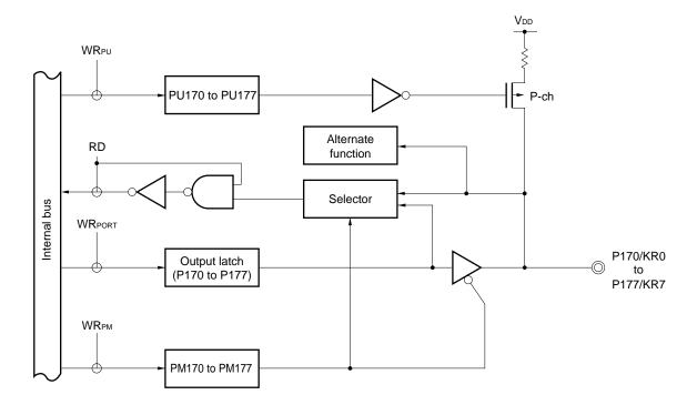
Figure 16-78. Block Diagram of P170 to P177
