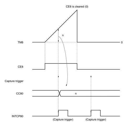
Figure 7-30. Example of TM8 Capture Operation
