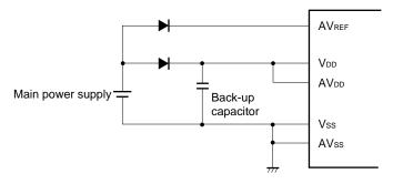
Figure 11-19. Handling of AVDD Pin
