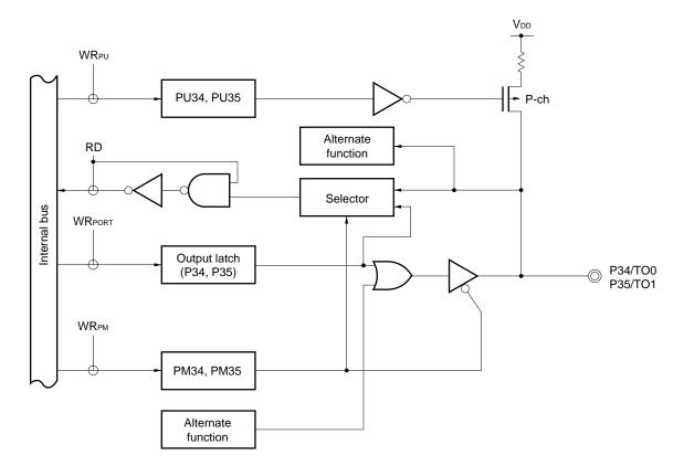
Figure 16-26. Block Diagram of P34 and P35
