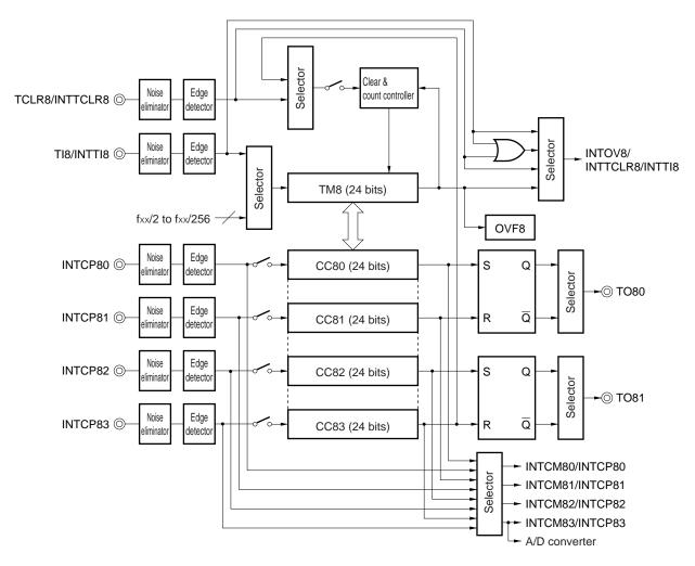
Figure 7-1. Block Diagram of TM8
