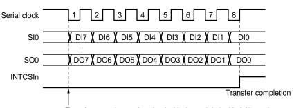
Figure 10-6. Timing of 3-Wire Serial I/O Mode
