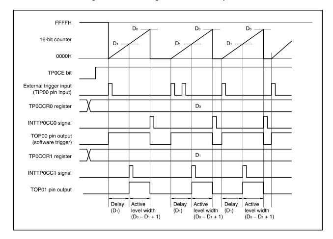
Figure 7-21. Basic Timing in One-Shot Pulse Output Mode
