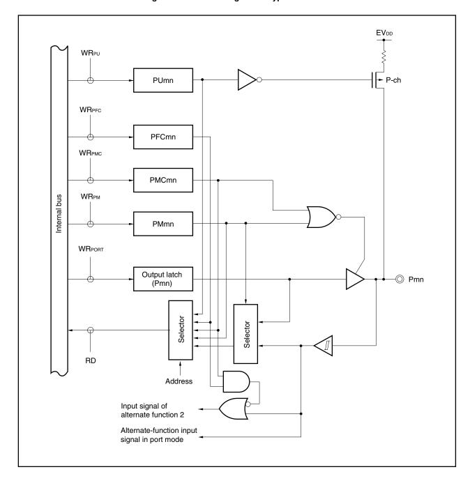
Figure 4-20. Block Diagram of Type Ex1-SUHT
