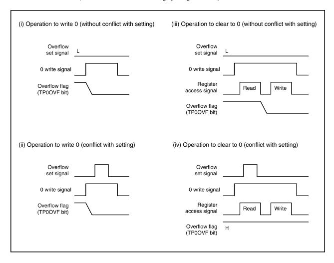
To clear the overflow flag to 0, read the overflow flag to check if it is set to 1, and clear it with the CLR instruction. If 0 is written to the overflow flag without checking if the flag is 1, the set information of overflow may be erased by writing 0 ((ii) in the above chart). Therefore, software may judge that no overflow has occurred even when an overflow actually has occurred.
