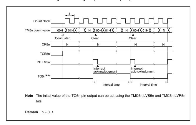
Figure 9-4. Timing of Square-Wave Output Operation
