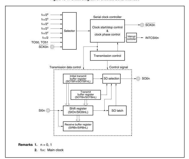
Figure 16-1. Block Diagram of Clocked Serial Interface
