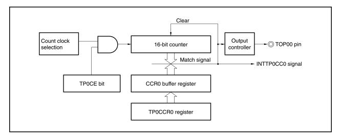
Figure 7-2. Configuration of Interval Timer
