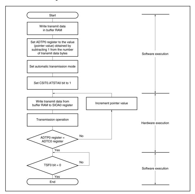
Figure 17-9. Automatic Transmission Mode Flowchart
