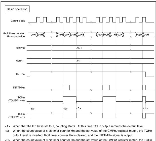
Figure 10-5. Operation Timing in PWM Output Mode (1/4)
