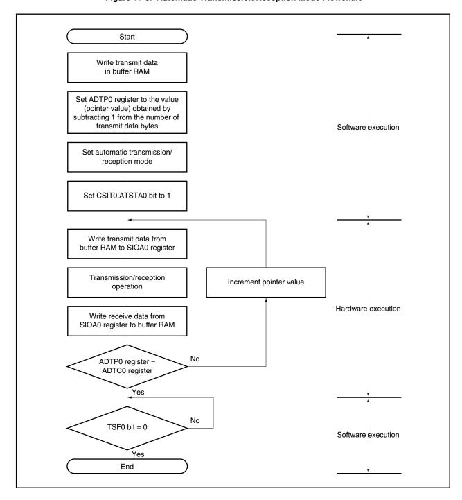
Figure 17-6. Automatic Transmission/Reception Mode Flowchart
