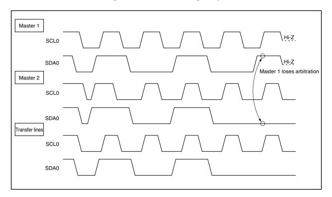
Figure 18-11. Arbitration Timing Example
