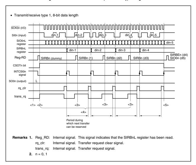
Figure 16-4. Continuous Transfer (Receive-Only) Timing Chart
