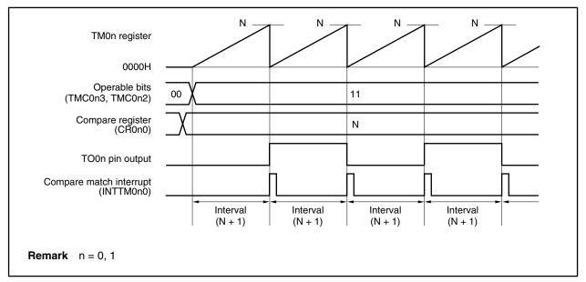
Figure 8-8. Example of Register Settings for Square Wave Output Operation
