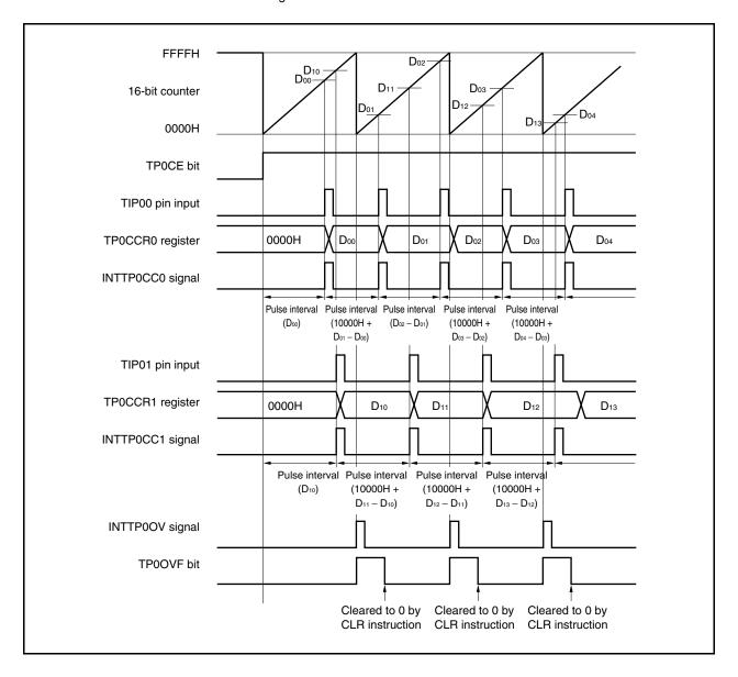
When executing pulse width measurement in the free-running timer mode, two pulse widths can be measured with one channel.
