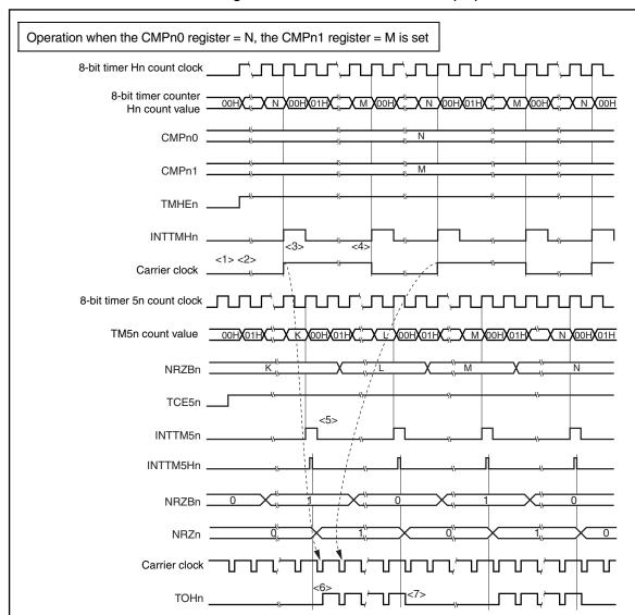
Figure 10-8. Carrier Generator Mode (2/3)
