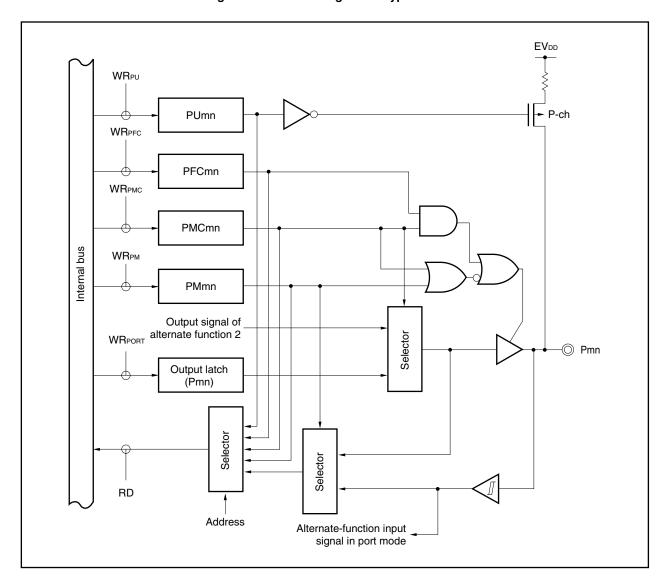
Figure 4-18. Block Diagram of Type Ex0-SUT
