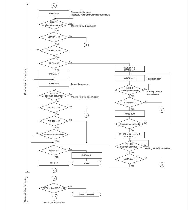
Figure 18-16. Master Operation in Multimaster System (3/3)
