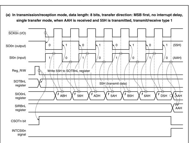
Figure 16-3. Timing Chart in Single Transfer Mode (1/2)
