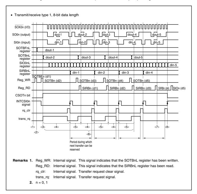
Figure 16-5. Continuous Transfer (Transmission/Reception) Timing Chart
