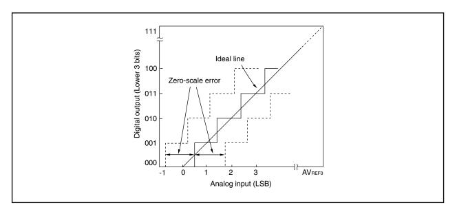
Figure 14-14. Zero-Scale Error
