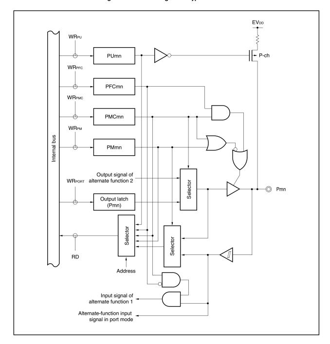
Figure 4-16. Block Diagram of Type E10-SULT
