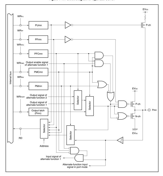
Figure 4-17. Block Diagram of Type E20-SUFLT
