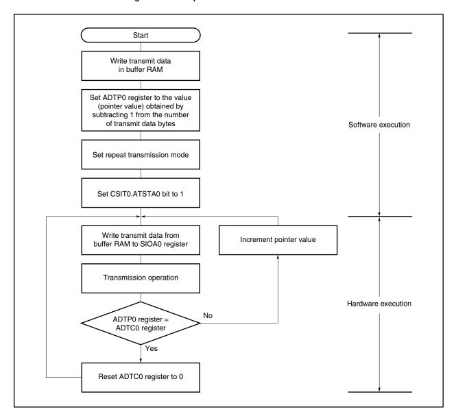
Figure 17-12. Repeat Transmission Mode Flowchart
