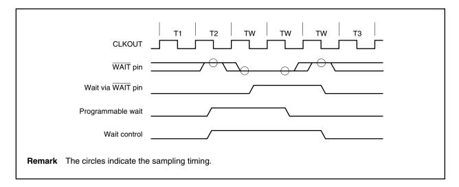
Figure 5-3. Example of Inserting Wait States
