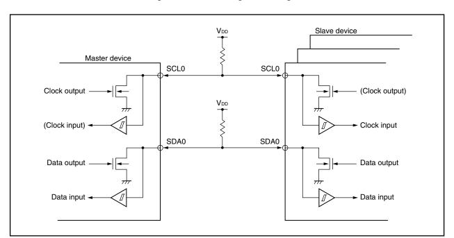
Figure 18-3. Pin Configuration Diagram
