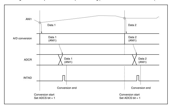
Figure 14-4. Example of Select Mode Operation Timing (ADS.ADS2 to ADS.ADS0 Bits = 001B)
