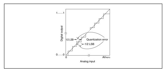
Figure 14-13. Quantization Error
