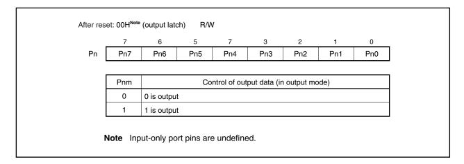
Writing to and reading from the Pn register are executed as follows depending on the setting of each register.
