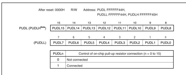
**Note** When reading from or writing to bits 8 to 15 of the PUDL register in 8-bit or 1-bit units, specify these bits as bits 0 to 7 of the PUDLH register.
