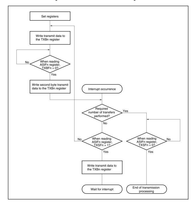
Figure 15-4. Continuous Transmission Processing Flow
