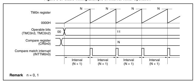
Figure 8-4. Example of Register Settings for Interval Timer Operation
