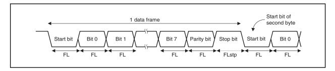
Representing the 1-bit data length by FL, the stop bit length by FLstp, and the base clock frequency by fuclk yields the following equation.
