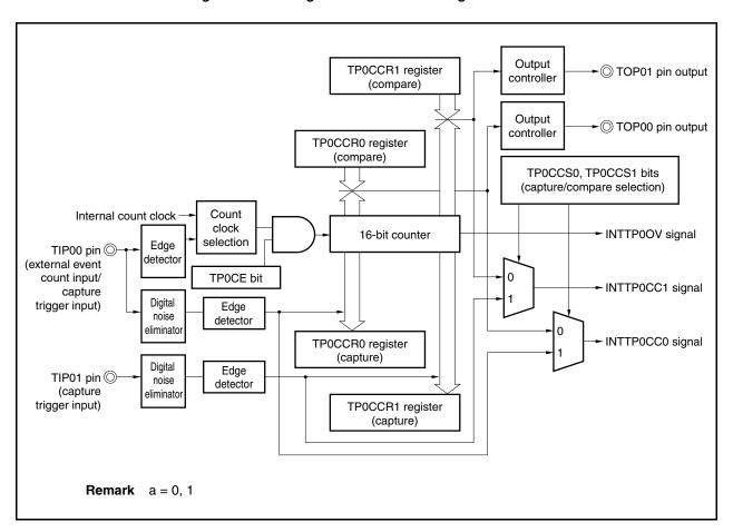
Figure 7-28. Configuration in Free-Running Timer Mode
