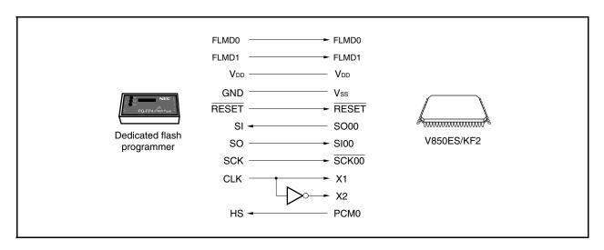
The dedicated flash programmer outputs the transfer clock, and the V850ES/KF2 operates as a slave.
