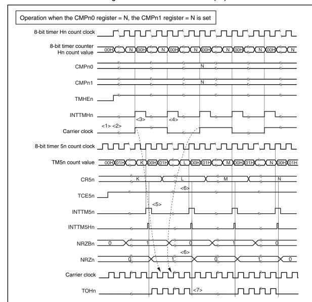
Figure 10-8. Carrier Generator Mode (1/3)
