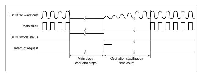
Figure 21-2. Oscillation Stabilization Time
