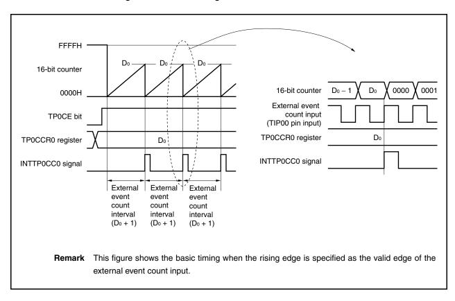
When the TP0CE bit is set to 1, the value of the 16-bit counter is cleared from FFFFH to 0000H. The counter counts each time the valid edge of external event count input is detected. Additionally, the set value of the TP0CCR0 register is transferred to the CCR0 buffer register.
