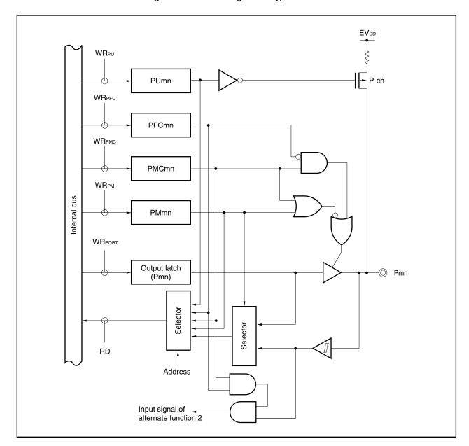
Figure 4-22. Block Diagram of Type Ex1-SUL
