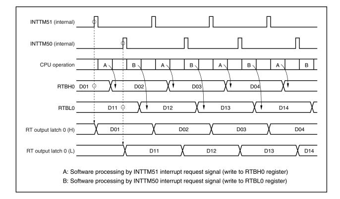
Figure 13-2. Example of Operation Timing of RTO0 (When EXTR0 and BYTE0 Bits = 00)
