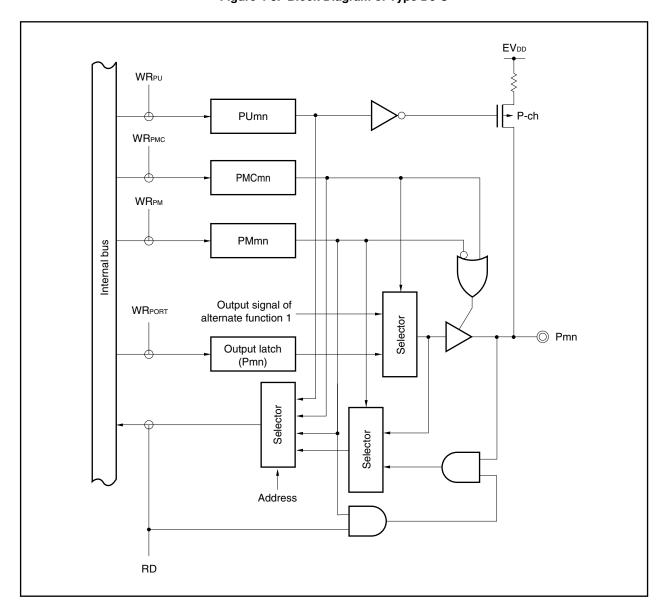
Figure 4-3. Block Diagram of Type D0-U
