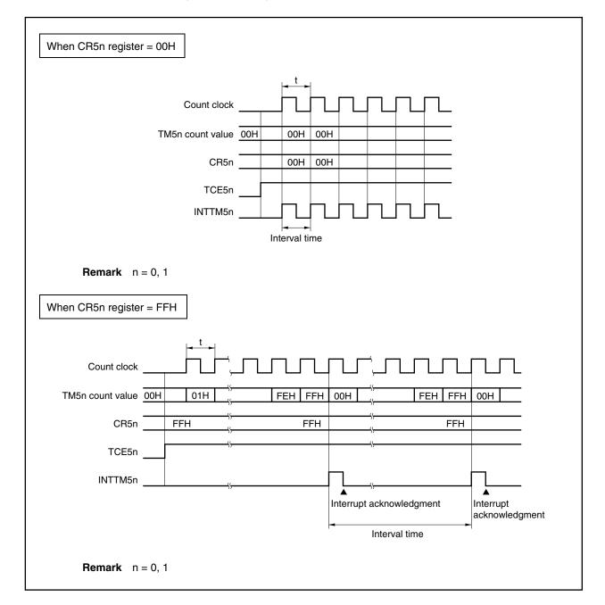
Figure 9-2. Timing of Interval Timer Operation (2/2)
