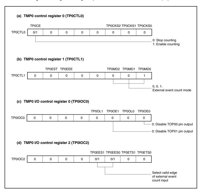
Figure 7-11. Register Setting for Operation in External Event Count Mode (2/2)
