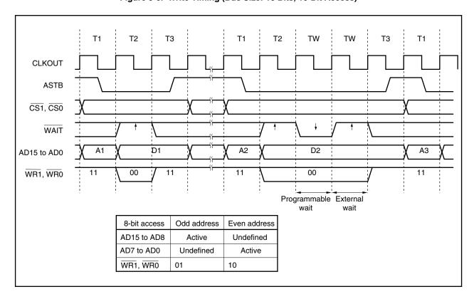
Figure 5-6. Write Timing (Bus Size: 16 Bits, 16-Bit Access)
