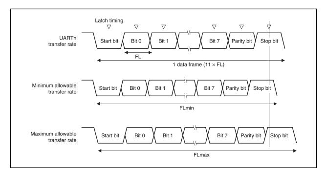
Figure 15-13. Allowable Baud Rate Range During Reception
