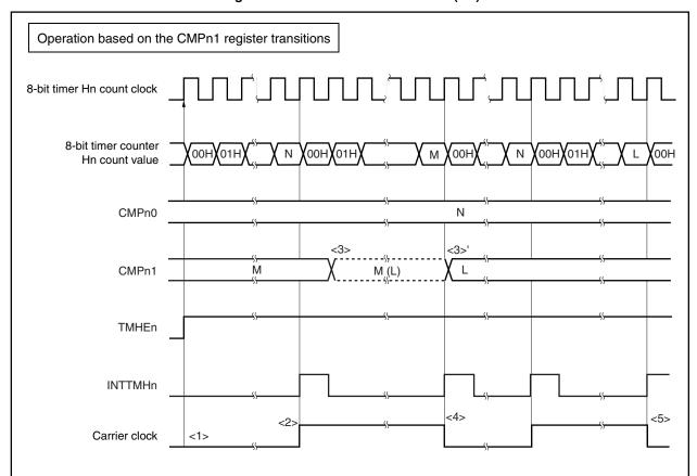
Figure 10-8. Carrier Generator Mode (3/3)
