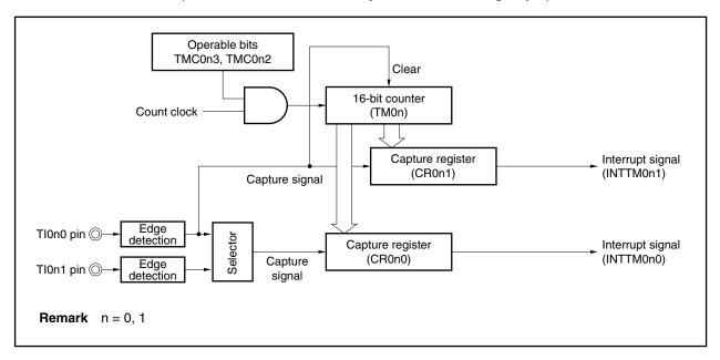
A pulse width can be measured in the following three ways.
