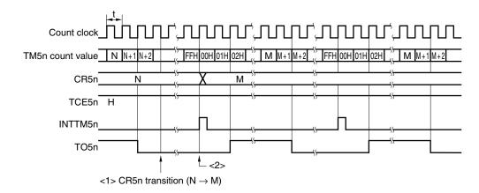
When the value of the CR5n register changes from N to M after the rising edge of the FFH clock
