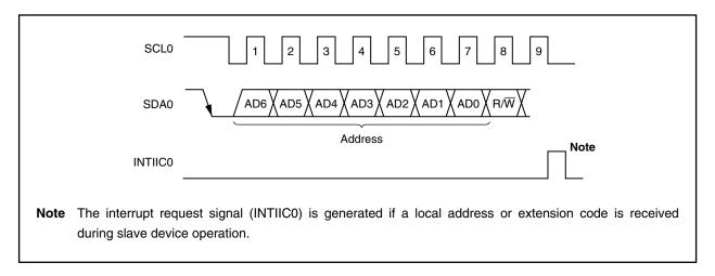
The slave address and the eighth bit, which specifies the transfer direction as described in **18.5.3 Transfer** direction specification below, are together written to the IIC0 register and are then output. Received addresses are written to the IIC0 register.
