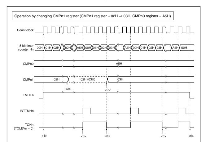
Figure 10-5. Operation Timing in PWM Output Mode (4/4)
