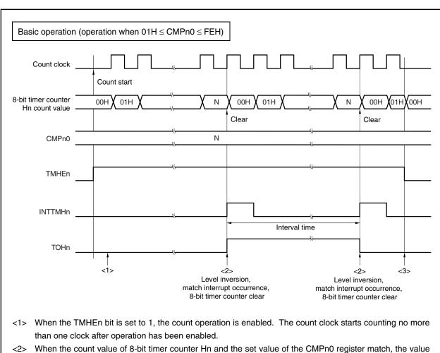
Figure 10-3. Timing of Interval Timer/Square Wave Output Operation (1/2)
