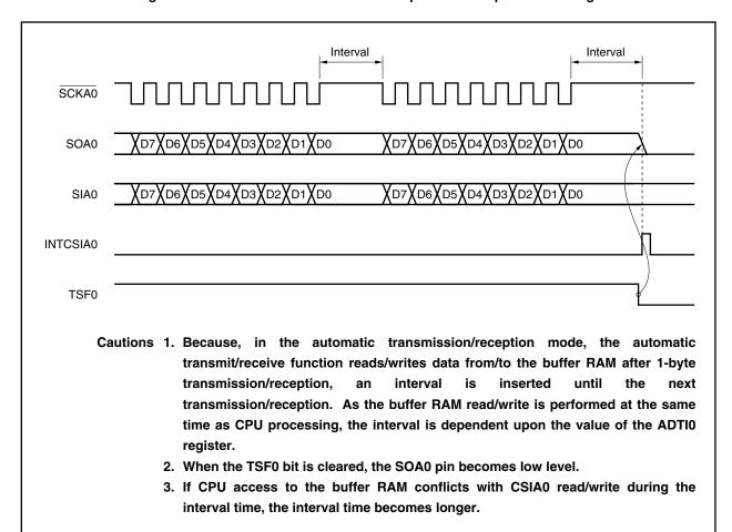
Figure 17-5. Automatic Transmission/Reception Mode Operation Timings
