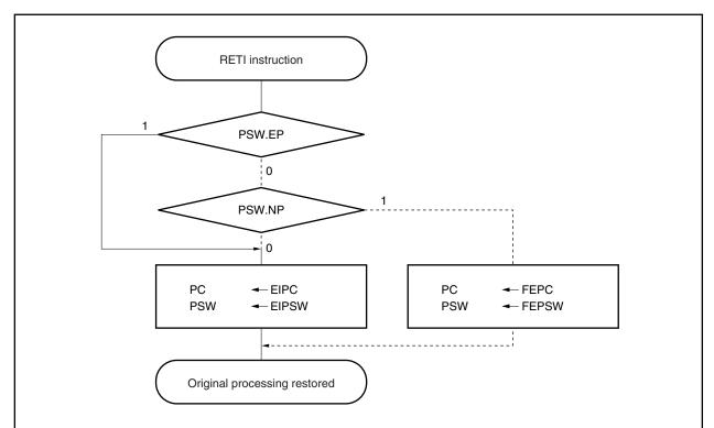
Caution When the EP bit and the NP bit are changed by the LDSR instruction during software exception processing, in order to restore the PC and PSW correctly during restoring by the RETI instruction, it is necessary to set the EP bit back to 1 using the LDSR instruction immediately before the RETI instruction.
