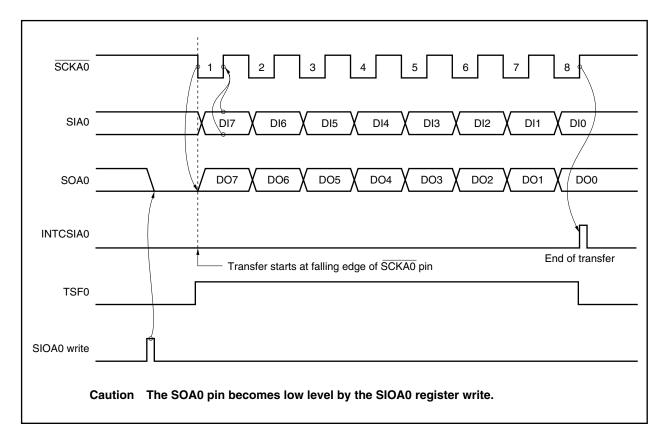
Figure 17-2. 3-Wire Serial I/O Mode Timing
