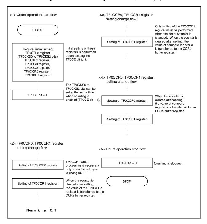
Figure 7-27. Software Processing Flow in PWM Output Mode (2/2)
