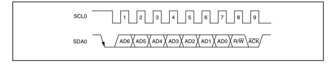
When the local address is received,  $\overline{ACK}$  is automatically generated regardless of the value of the ACKE0 bit. No  $\overline{ACK}$  is generated if the received address is not a local address (NACK).
