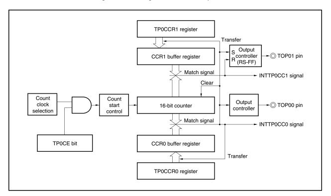
Figure 7-24. Configuration in PWM Output Mode
