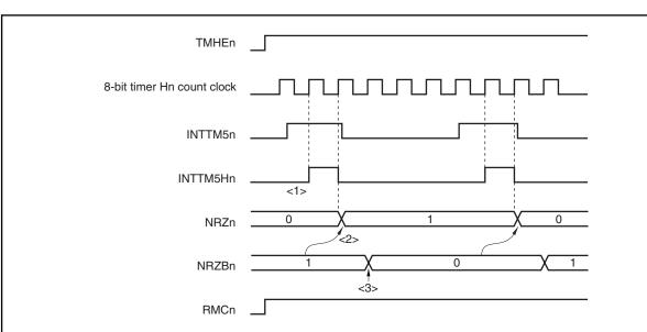
Figure 10-6. Transfer Timing
