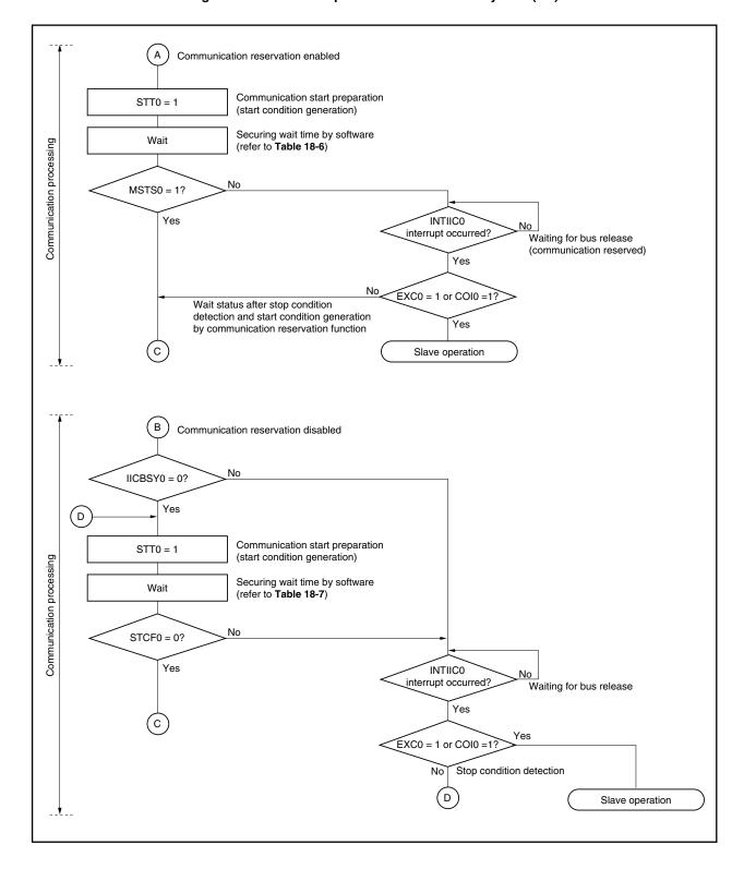
Figure 18-16. Master Operation in Multimaster System (2/3)
