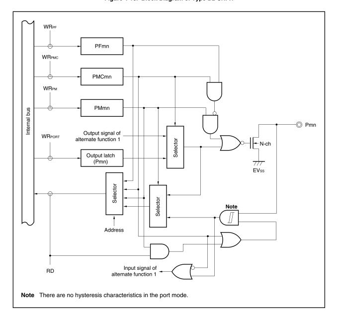
Figure 4-10. Block Diagram of Type D2-SNFH
