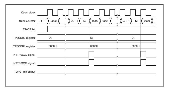
To output a 100% waveform, set a value of (set value of TP0CCR0 register + 1) to the TP0CCR1 register. If the set value of the TP0CCR0 register is FFFFH, 100% output cannot be produced.
