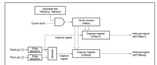
**Remarks 1.** If both the CR0n0 and CR0n1 registers are used as capture registers in the free-running timer mode, the output level of the TO0n pin is not inverted.
