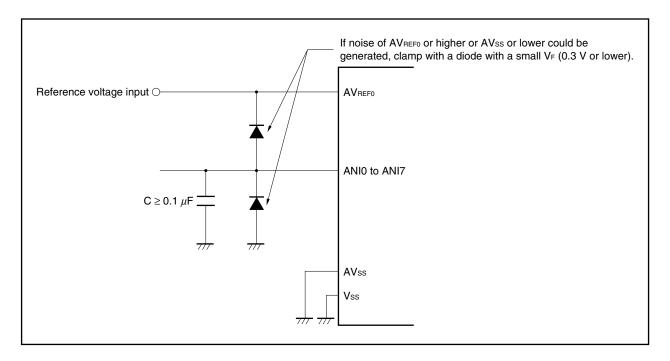
Figure 14-8. Handling of Analog Input Pins
