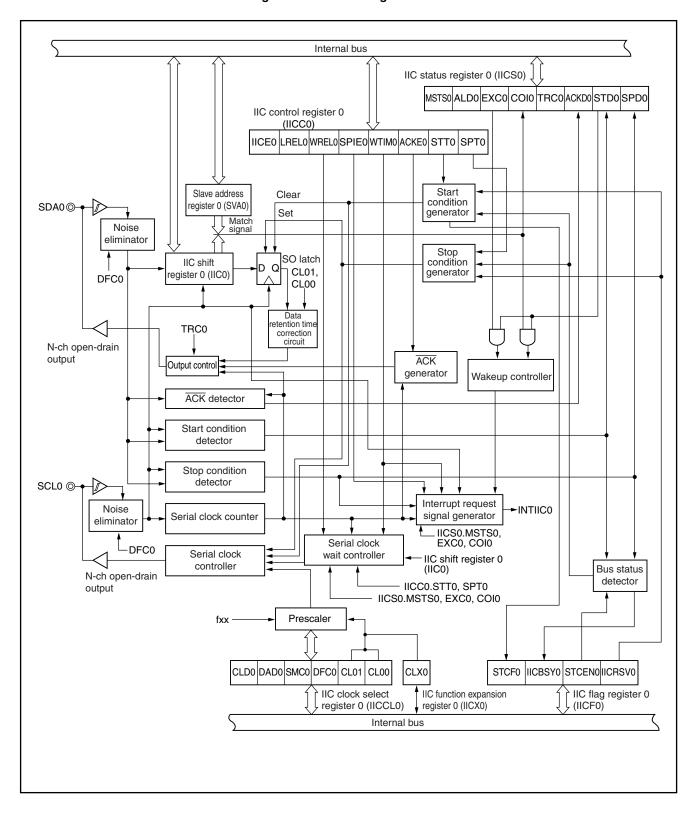
Figure 18-1. Block Diagram of I<sup>2</sup>C0
