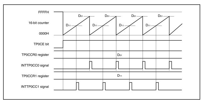
If the set value of the TP0CCR1 register is greater than the set value of the TP0CCR0 register, the INTTP0CC1 signal is not generated because the count value of the 16-bit counter and the value of the TP0CCR1 register do not match.
