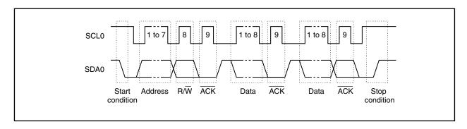
Figure 18-4. I<sup>2</sup>C Bus's Serial Data Transfer Timing
