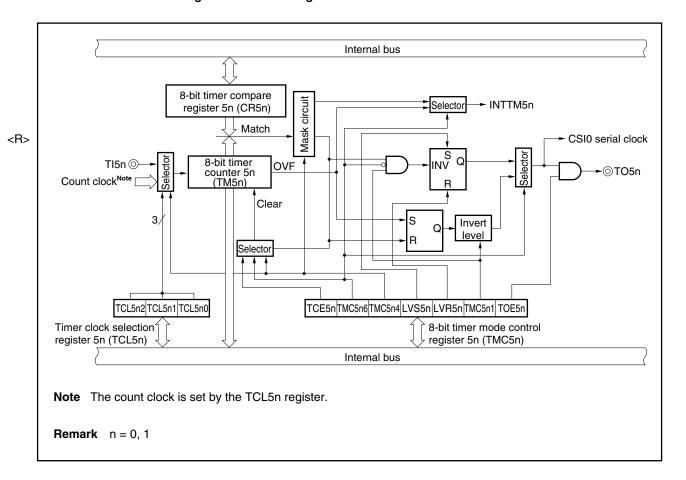
Figure 9-1. Block Diagram of 8-Bit Timer/Event Counter 5n
