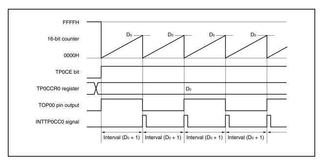
When the TPOCE bit is set to 1, the value of the 16-bit counter is cleared from FFFFH to 0000H in synchronization with the count clock, and the counter starts counting. At this time, the output of the TOP00 pin is inverted. Additionally, the set value of the TP0CCR0 register is transferred to the CCR0 buffer register.
