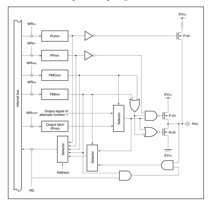
Figure 4-4. Block Diagram of Type D0-UF
