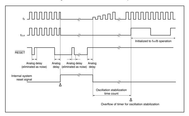
Figure 22-2. Hardware Status on RESET Input
