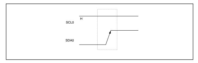
A stop condition is generated when the IICC0.SPT0 bit is set to 1. When the stop condition is detected, the IICS0.SPD0 bit is set to 1 and the interrupt request signal (INTIIC0) is generated when the IICC0.SPIE0 bit is set to 1.
