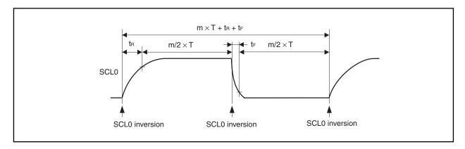
The selection clock is set using a combination of the IICCL0.SMC0, IICCL0.CL01, and IICCL0.CL00 bits and the IICX0.CLX0 bit.
