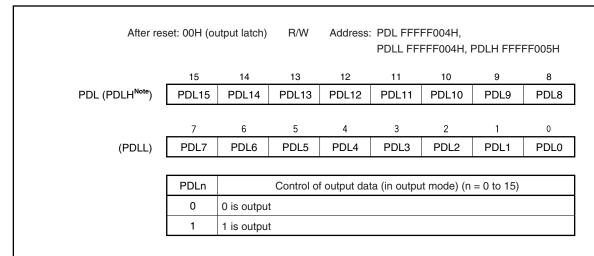
**Note** When reading from or writing to bits 8 to 15 of the PDL register in 8-bit or 1-bit units, specify these bits as bits 0 to 7 of the PDLH register.
