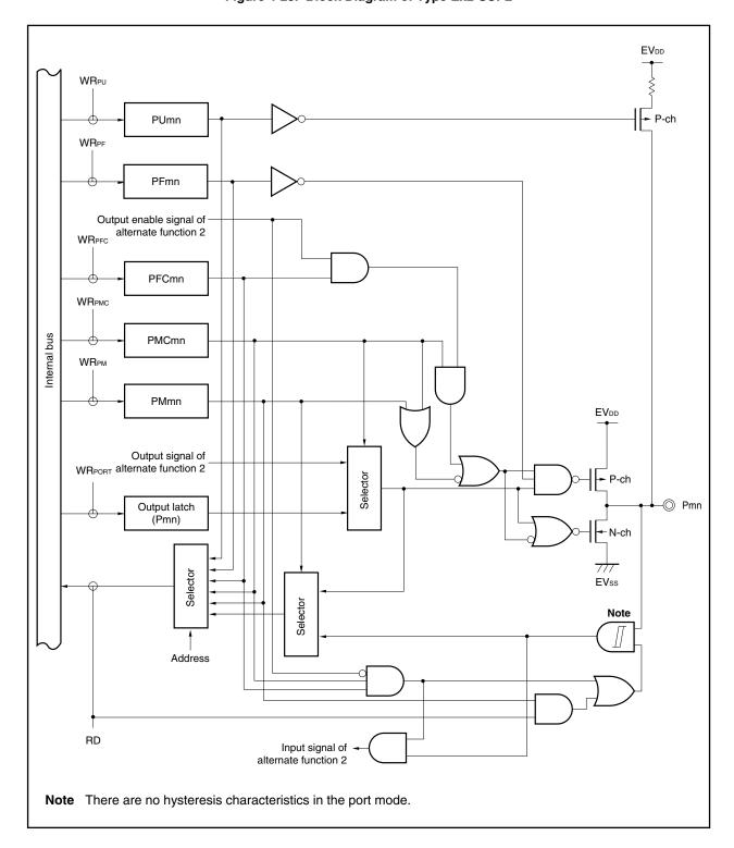
Figure 4-23. Block Diagram of Type Ex2-SUFL
