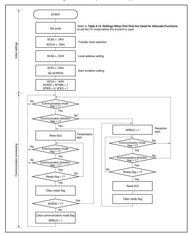
Figure 18-18. Slave Operation Flowchart (1)
