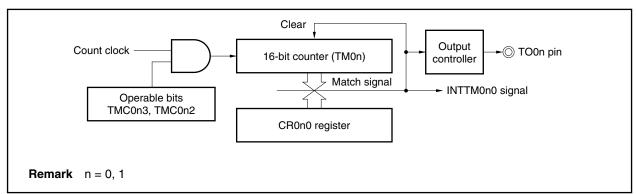
Figure 8-6. Block Diagram of Square Wave Output Operation
