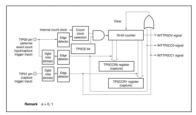
Figure 7-34. Configuration in Pulse Width Measurement Mode
