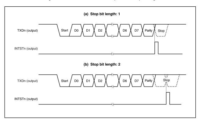
Figure 15-3. UARTn Transmission Completion Interrupt Timing
