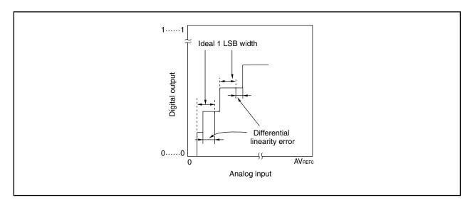
Figure 14-16. Differential Linearity Error
