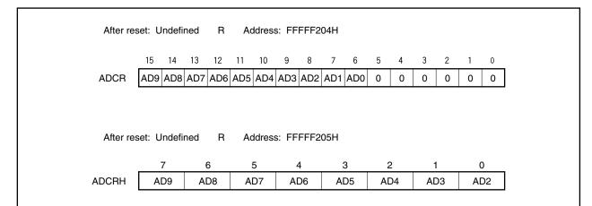
Caution Do not access the ADCR and ADCRH registers when the main clock is stopped and the subclock is operating. For details, refer to 3.4.8 (2) Access to special on-chip peripheral I/O register.
