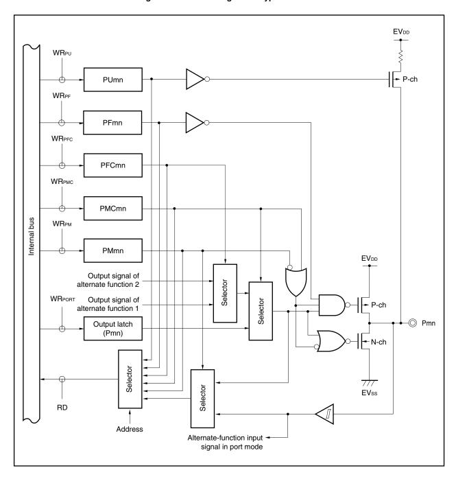
Figure 4-13. Block Diagram of Type E00-SUFT
