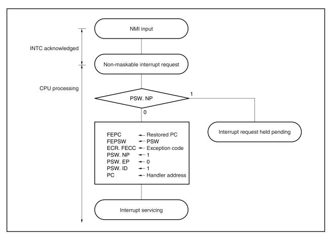
Figure 19-2. Non-Maskable Interrupt Servicing
