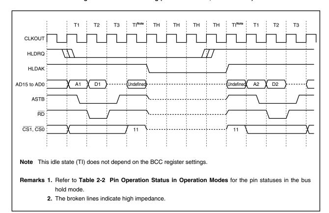
Figure 5-8. Bus Hold Timing (Bus Size: 16 Bits, 16-Bit Access)
