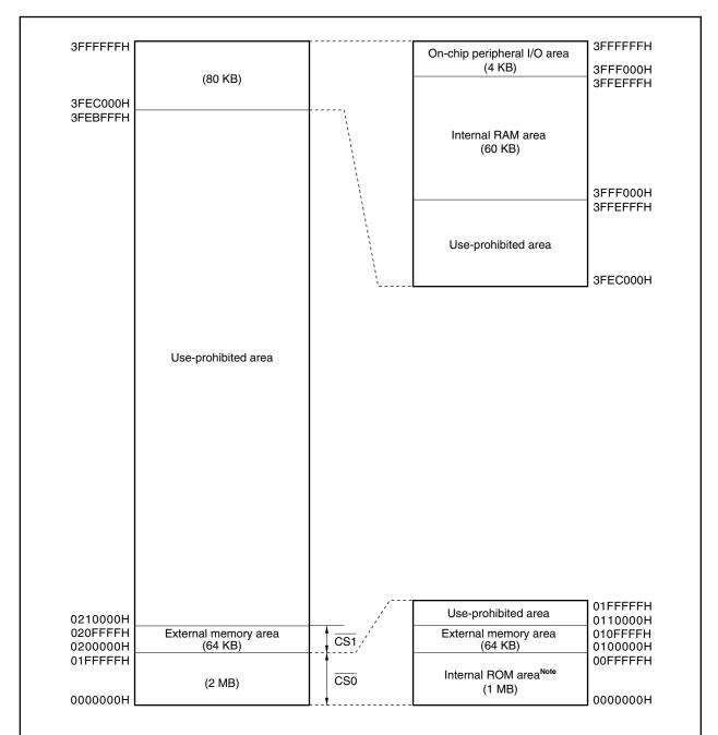
**Note** Fetch access and read access to addresses 0000000H to 00FFFFH is performed for the internal ROM area, but in the case of data write access, it is performed for an external memory area.
