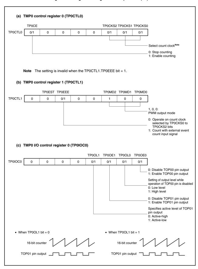
Figure 7-26. Register Setting in PWM Output Mode (2/2)
