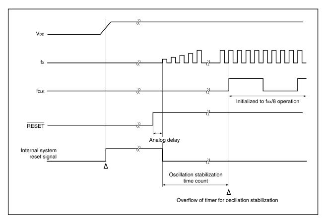
Figure 22-4. Timing of Reset Operation by Watchdog Timer 1
