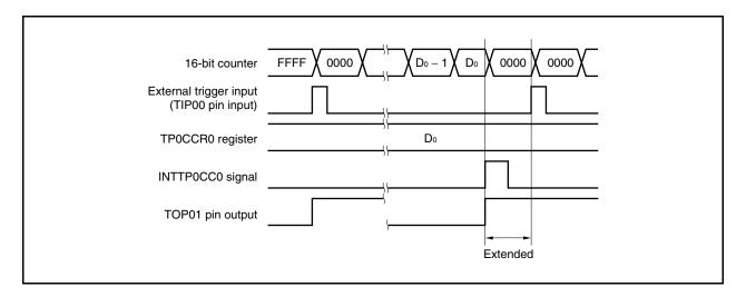
If the trigger is detected immediately before the INTTPOCC0 signal is generated, the INTTPOCC0 signal is not generated. The 16-bit counter is cleared to 0000H, the TOP01 pin is asserted, and the counter continues counting. Consequently, the inactive period of the PWM waveform is shortened.
