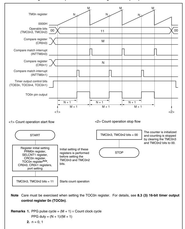
Figure 8-33. Example of Software Processing for PPG Output Operation
