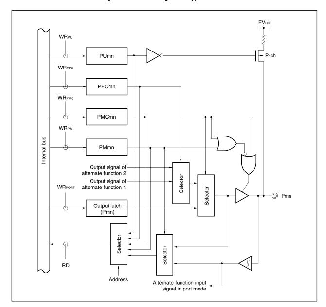
Figure 4-14. Block Diagram of Type E00-SUT
