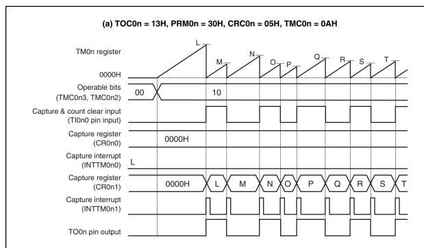
This is an application example where the count value is captured to the CR0n1 register, the TM0n register is cleared, and the TO0n pin output is inverted when the rising or falling edge of the Tl0n0 pin is detected. When the edge of the Tl0n1 pin is detected, an interrupt signal (INTTM0n0) is generated. Mask the INTTM0n0 signal when it is not used.
