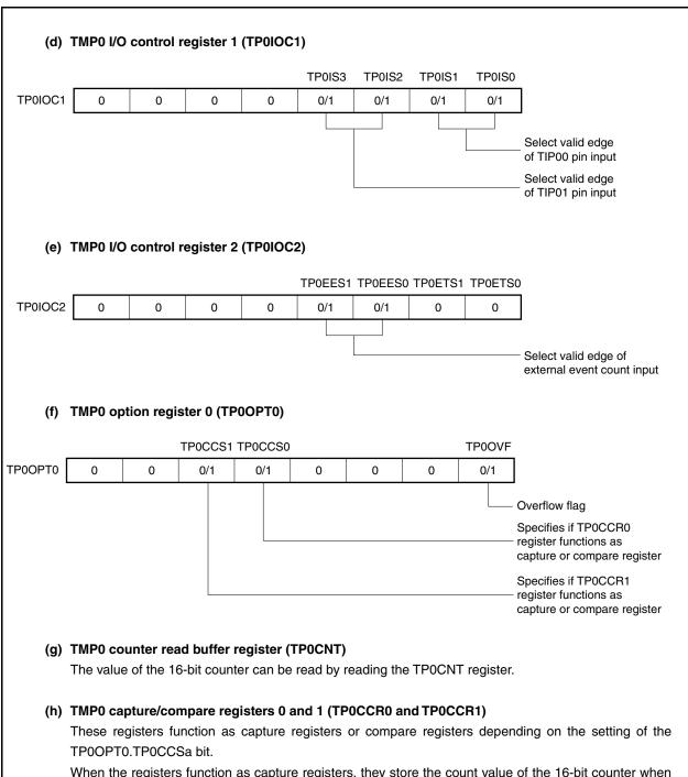
When the registers function as capture registers, they store the count value of the 16-bit counter when the valid edge input to the TIP0a pin is detected.
