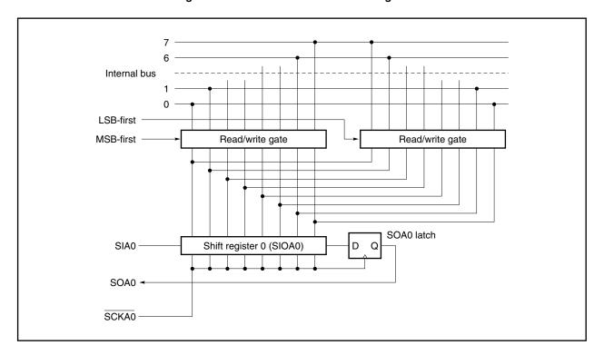
Figure 17-4. Transfer Bit Order Switching Circuit
