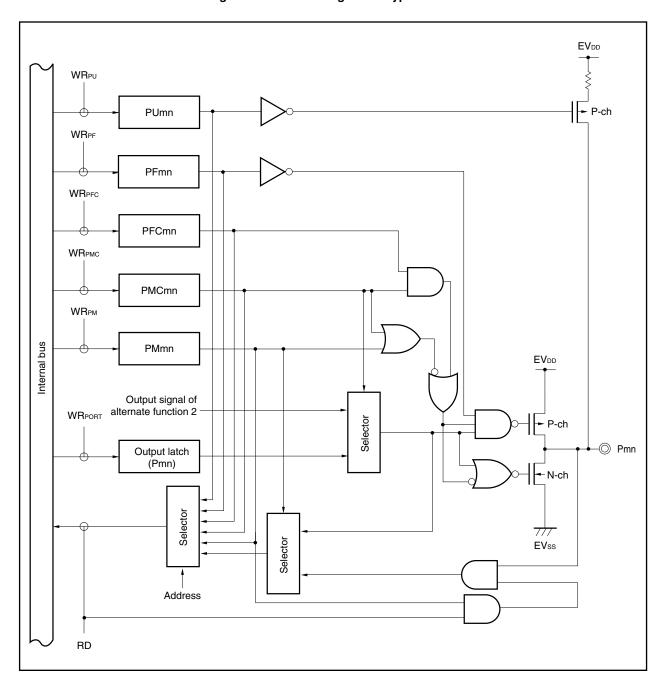
Figure 4-19. Block Diagram of Type Ex0-UF
