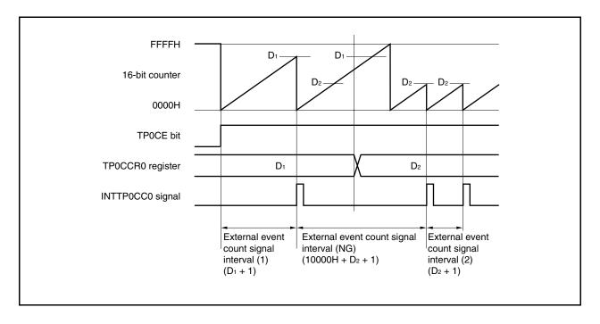
If the value of the TP0CCR0 register is changed from  $D_1$  to  $D_2$  while the count value is greater than  $D_2$  but less than  $D_1$ , the count value is transferred to the CCR0 buffer register as soon as the TP0CCR0 register has been rewritten. Consequently, the value that is compared with the 16-bit counter is  $D_2$ .
