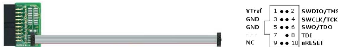
Figure 34. J-Link 9-pin Cortex-M Adapter
