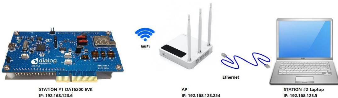
**Figure 47. Throughput test environment**
