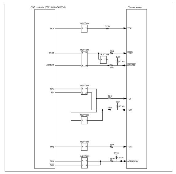
Figure 6.8 User System Interface Circuit of the H-UDI Pin in the Emulator (HS7660KCI02H) (Model Name: HS0005KCI04H)
