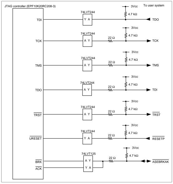
Figure 6.7 User System Interface Circuit in the Emulator (HS7660KCI01H) (Model Name: HS0005KCI03H)
