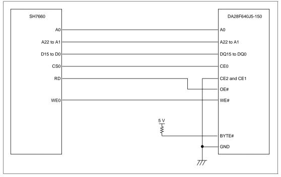
Figure 6.17 Example of Connecting the Flash Memory
