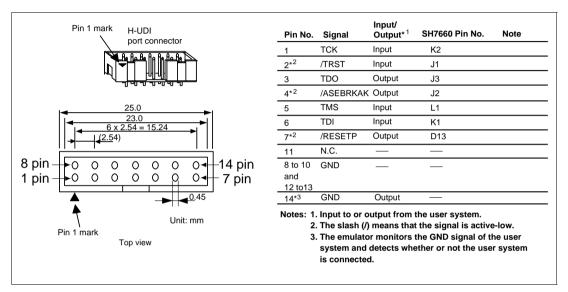
Figure 6.2 Pin Arrangement of the H-UDI Port Connector (14 Pins)
