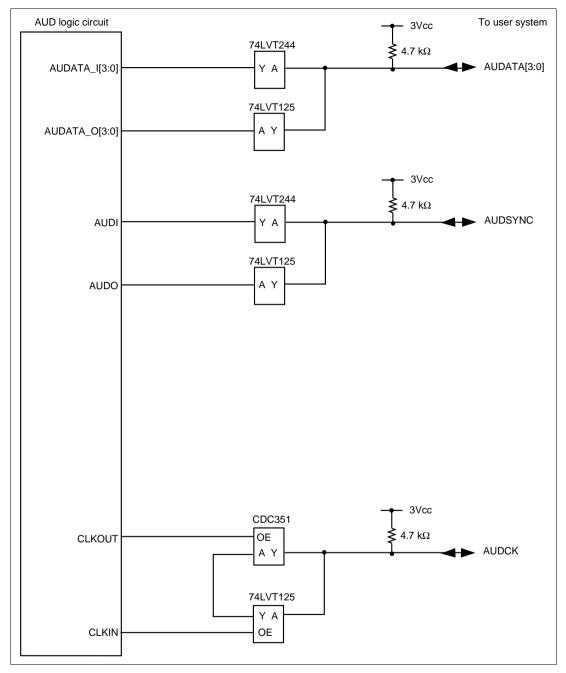
Figure 6.9 User System Interface Circuit of the AUD Pin in the Emulator (HS7660KCI02H) (Model Name: HS0005KCI04H)
