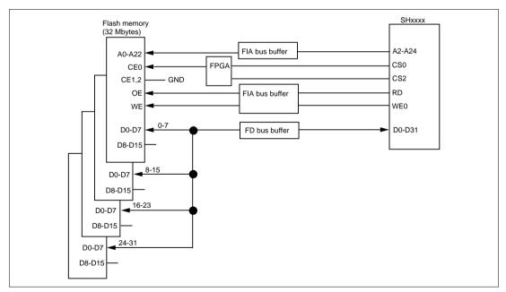
Figure 3.69 Flash Memory Wiring
