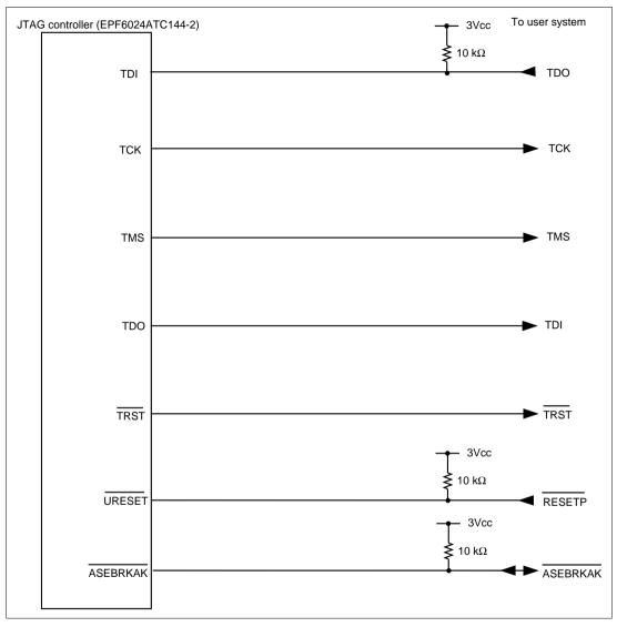
Figure 6.5 User System Interface Circuit of the H-UDI Pin in the Emulator (HS7660KCM02H) (Model Name: HS0005KCM04H)
