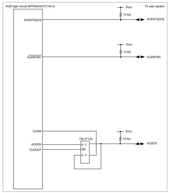
Figure 6.6 User System Interface Circuit of the AUD Pin in the Emulator (HS7660KCM02H) (Model Name: HS0005KCM04H)
