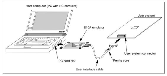
Figure 6.1 Connecting Ferrite Core
