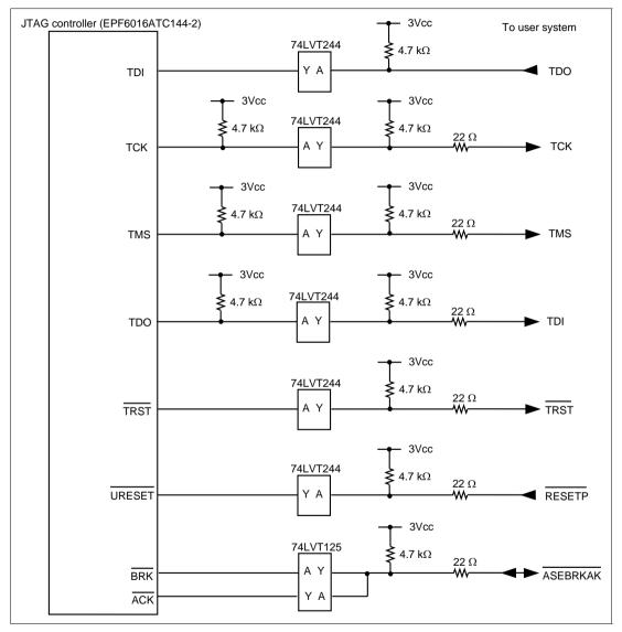
Figure 6.4 User System Interface Circuit in the Emulator (HS7660KCM01H) (Model Name: HS0005KCM03H)
