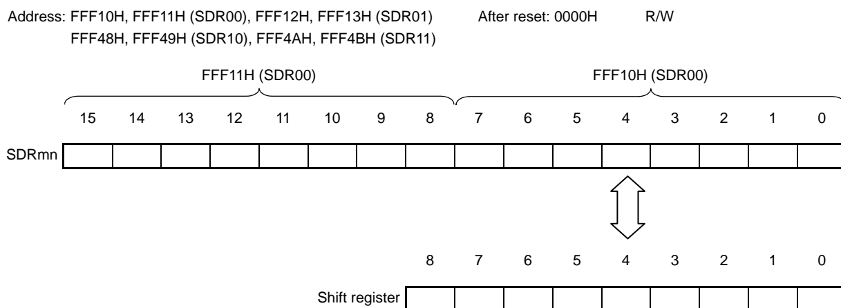
Figure 15 - 3 Format of Serial data register mn (SDRmn) (mn = 00, 01, 10, 11)
