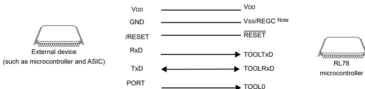
**Note** Connect REGC pin to ground via a capacitor (0.47 to 1 μF).
