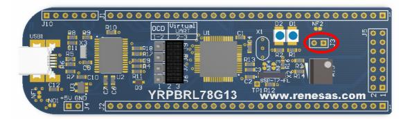
Figure 44: Current Measurement Connector
