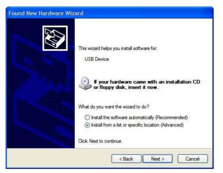
Figure 8: Install from a Specific Location (Windows XP)
