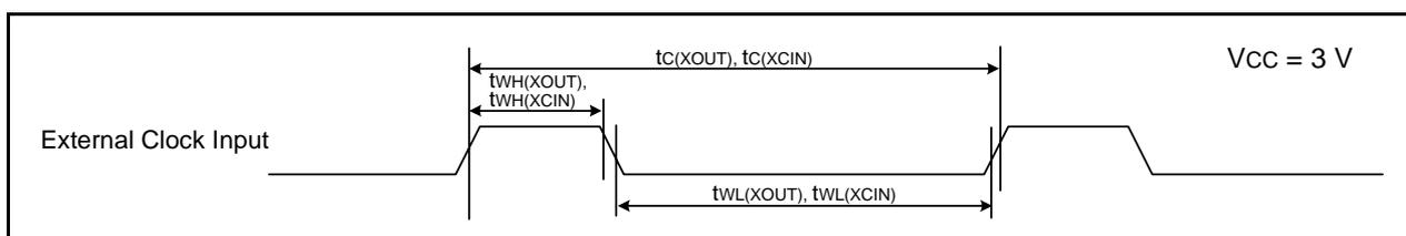
**Figure 26.8 External Clock Input Timing Diagram when  $V_{CC} = 3\text{ V}$** **Table 26.22 TRAIO Input**
