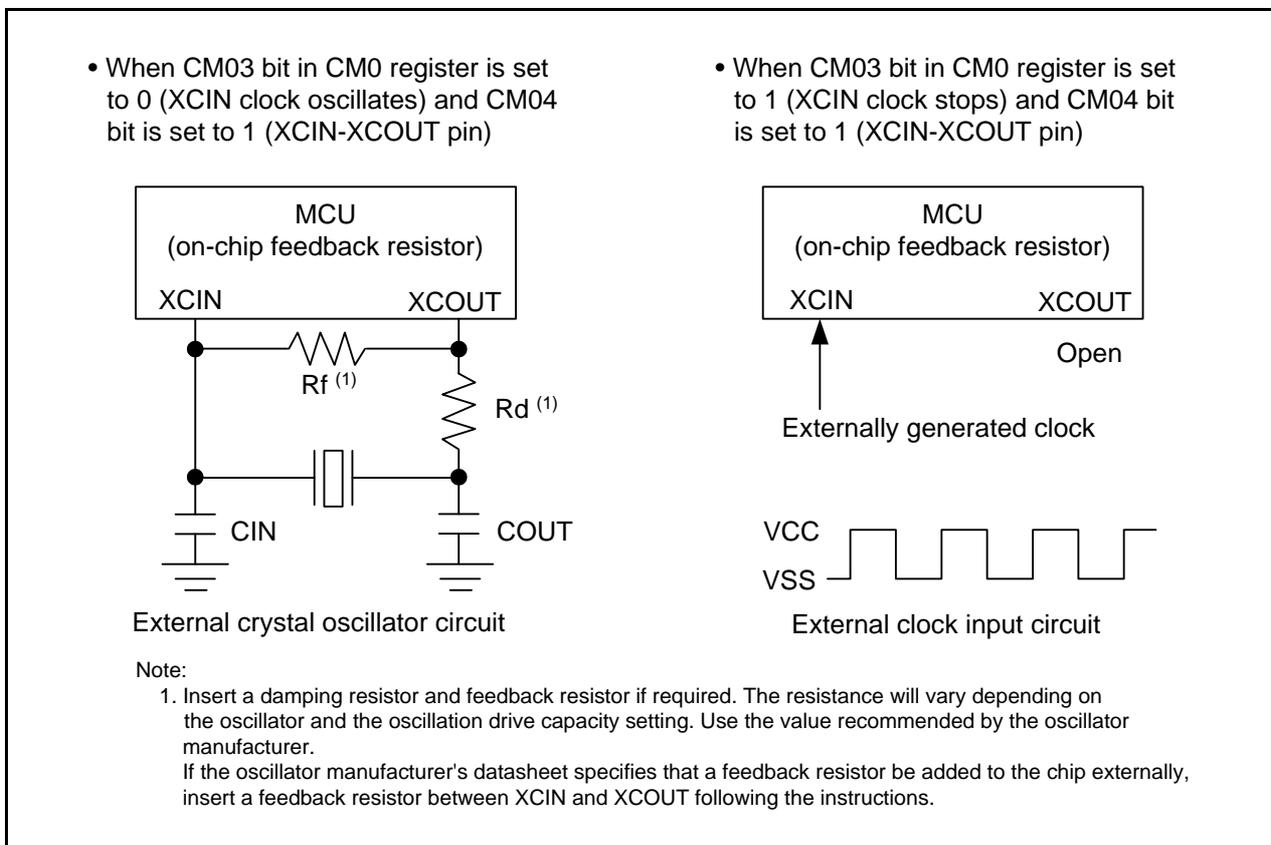
**Figure 9.5** Examples of XCIN Clock Connection Circuits
