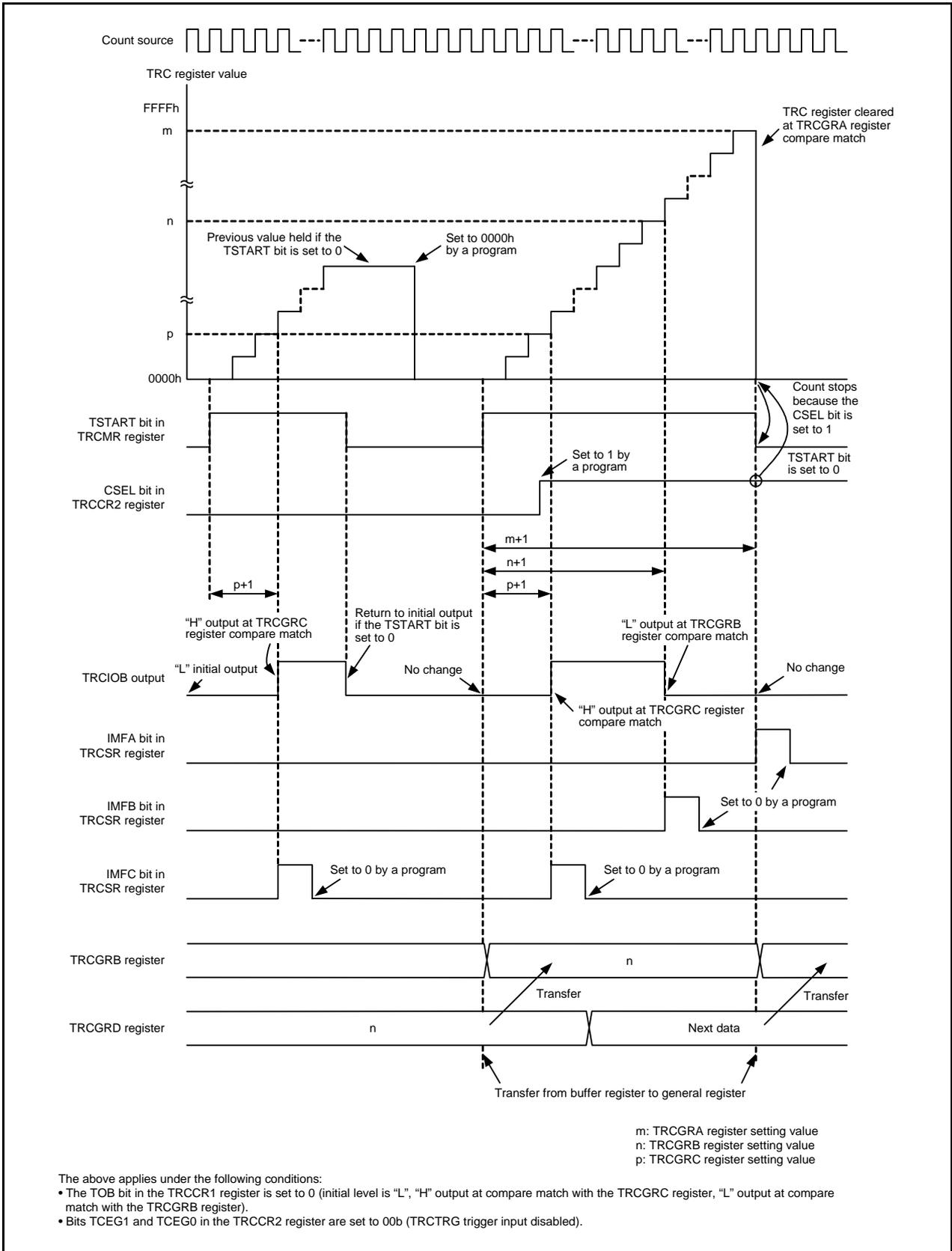
Figure 18.17 Operating Example of PWM2 Mode (TRCTRГ Trigger Input Disabled)
