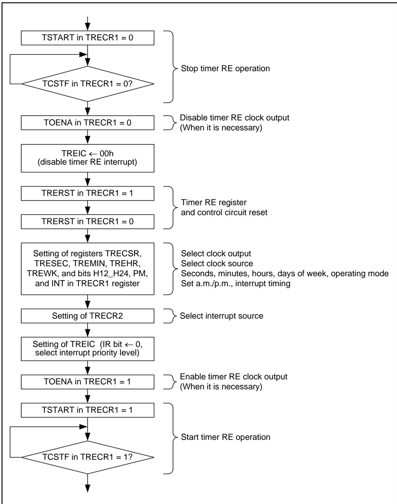
Figure 27.2 Setting Example in Real-Time Clock Mode
