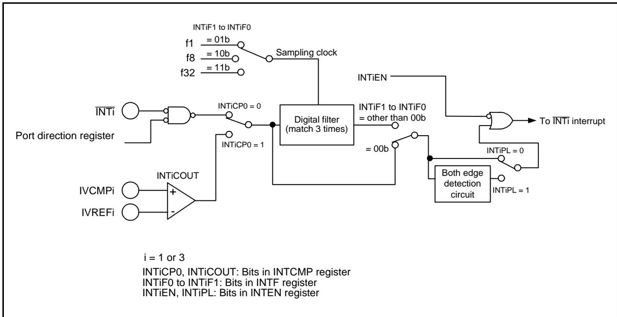
Figure 23.3 Configuration of Comparator Bi Digital Filter
