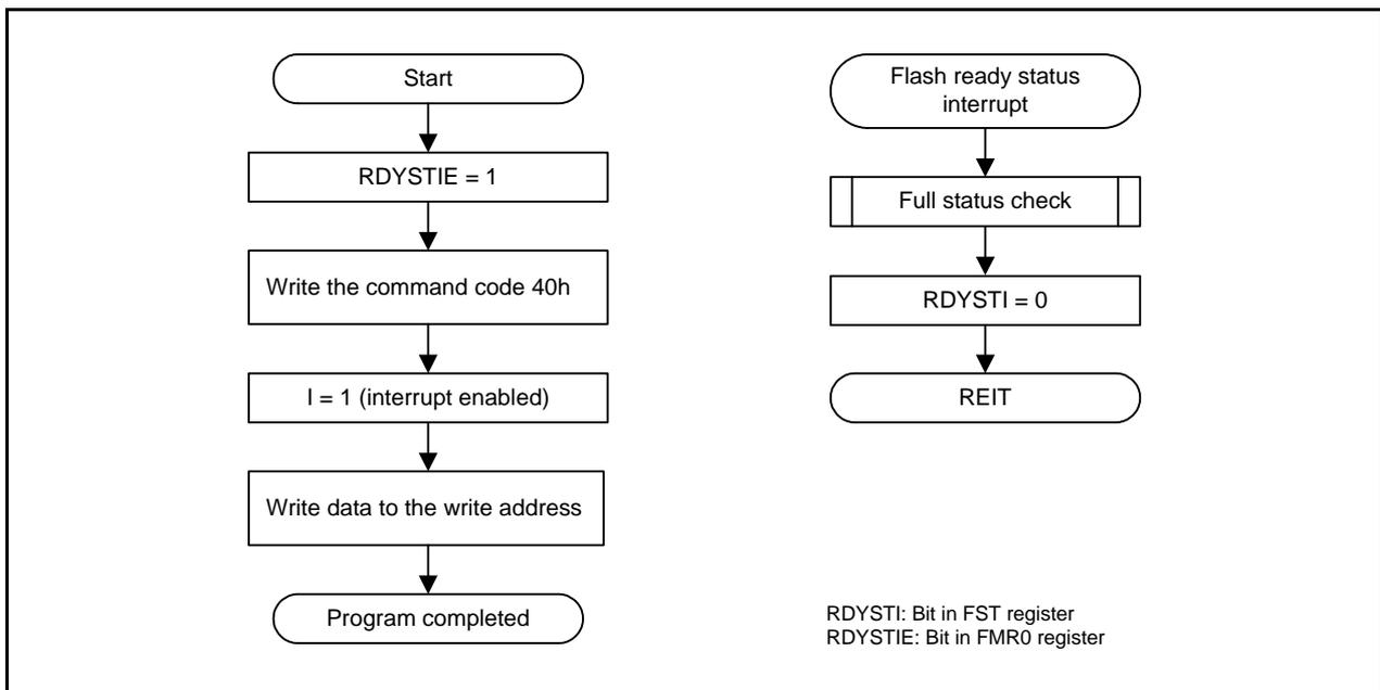
Figure 24.8 Program Flowchart (Flash Ready Status Interrupt Enabled)
