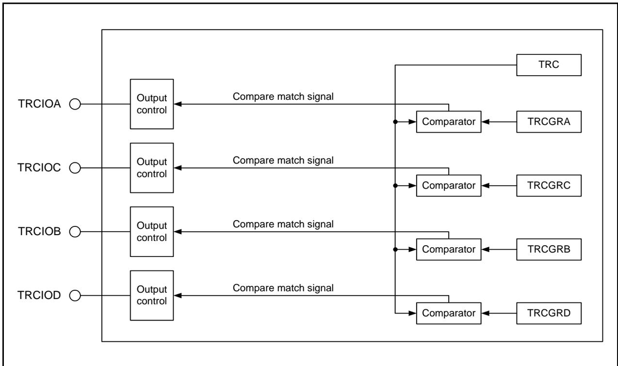
Figure 18.9 Block Diagram of Output Compare Function
