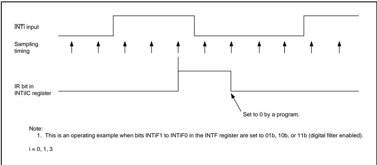
Figure 11.10 Operating Example of  $\overline{\text{INT}}_i$  Input Filter
