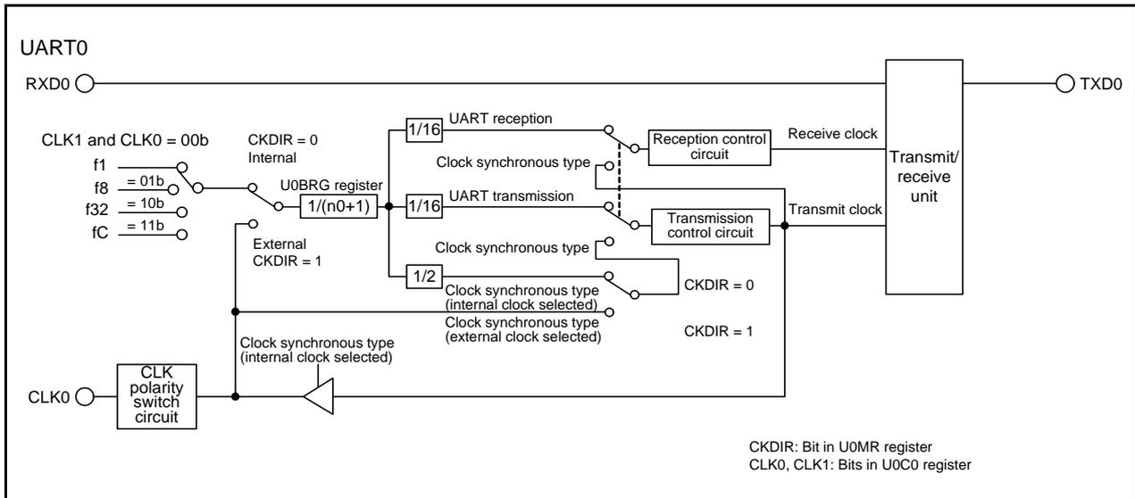
Figure 20.1 UART0 Block Diagram
