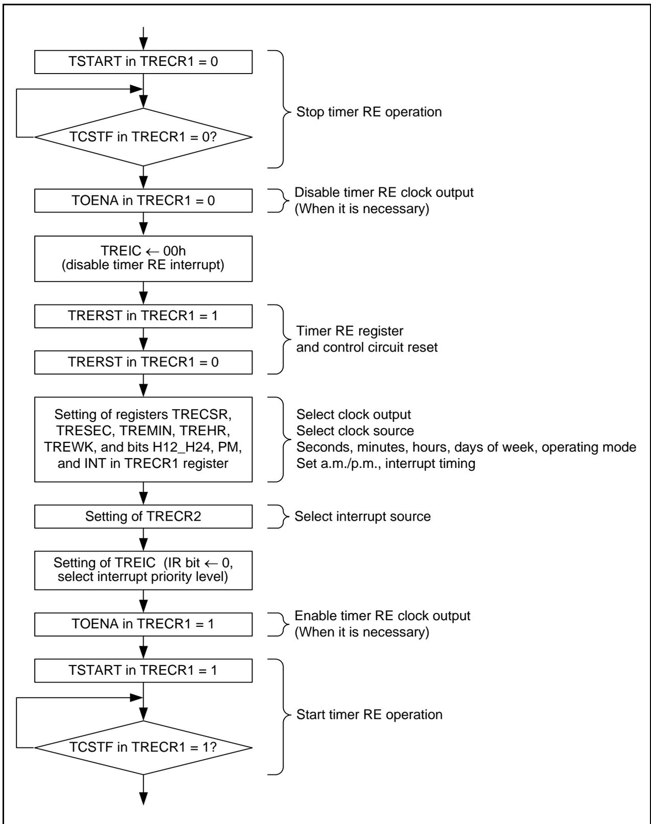
Figure 19.6 Setting Example in Real-Time Clock Mode
