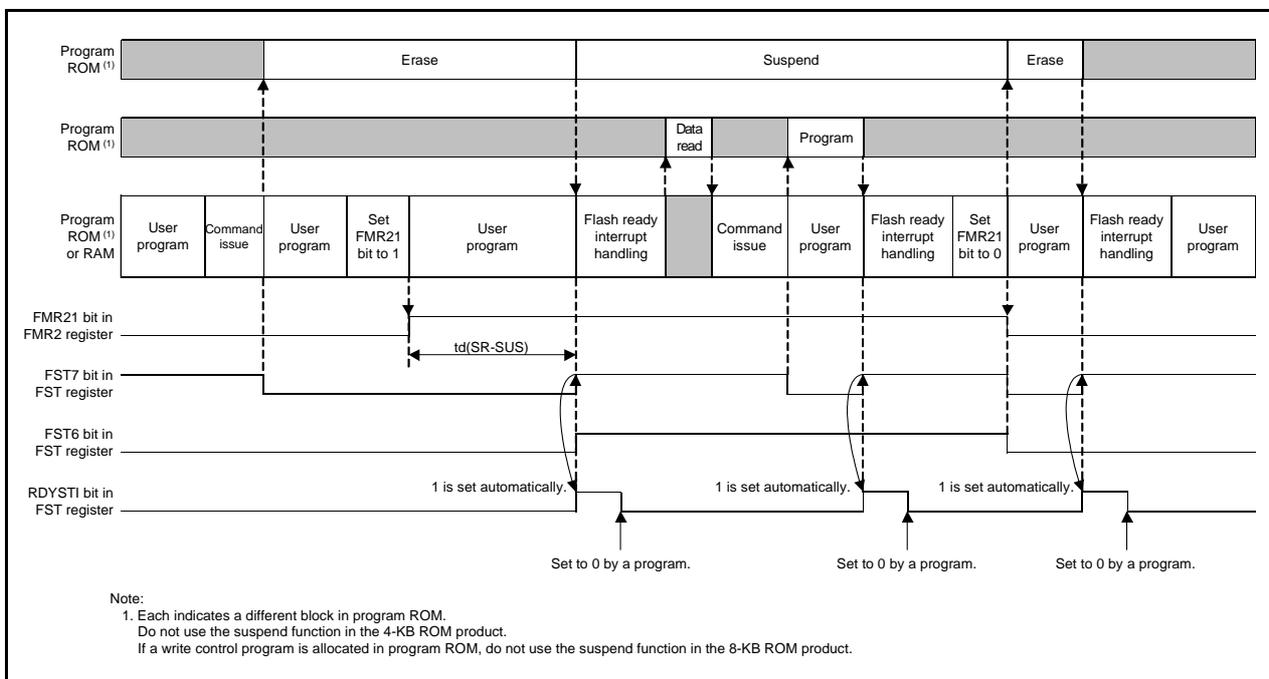
**Figure 24.3 Suspend Operation Timing**
