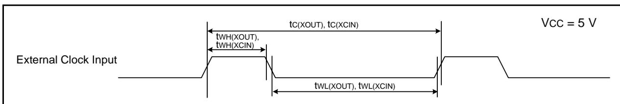
**Figure 26.4 External Clock Input Timing Diagram when  $V_{CC} = 5\text{ V}$**
