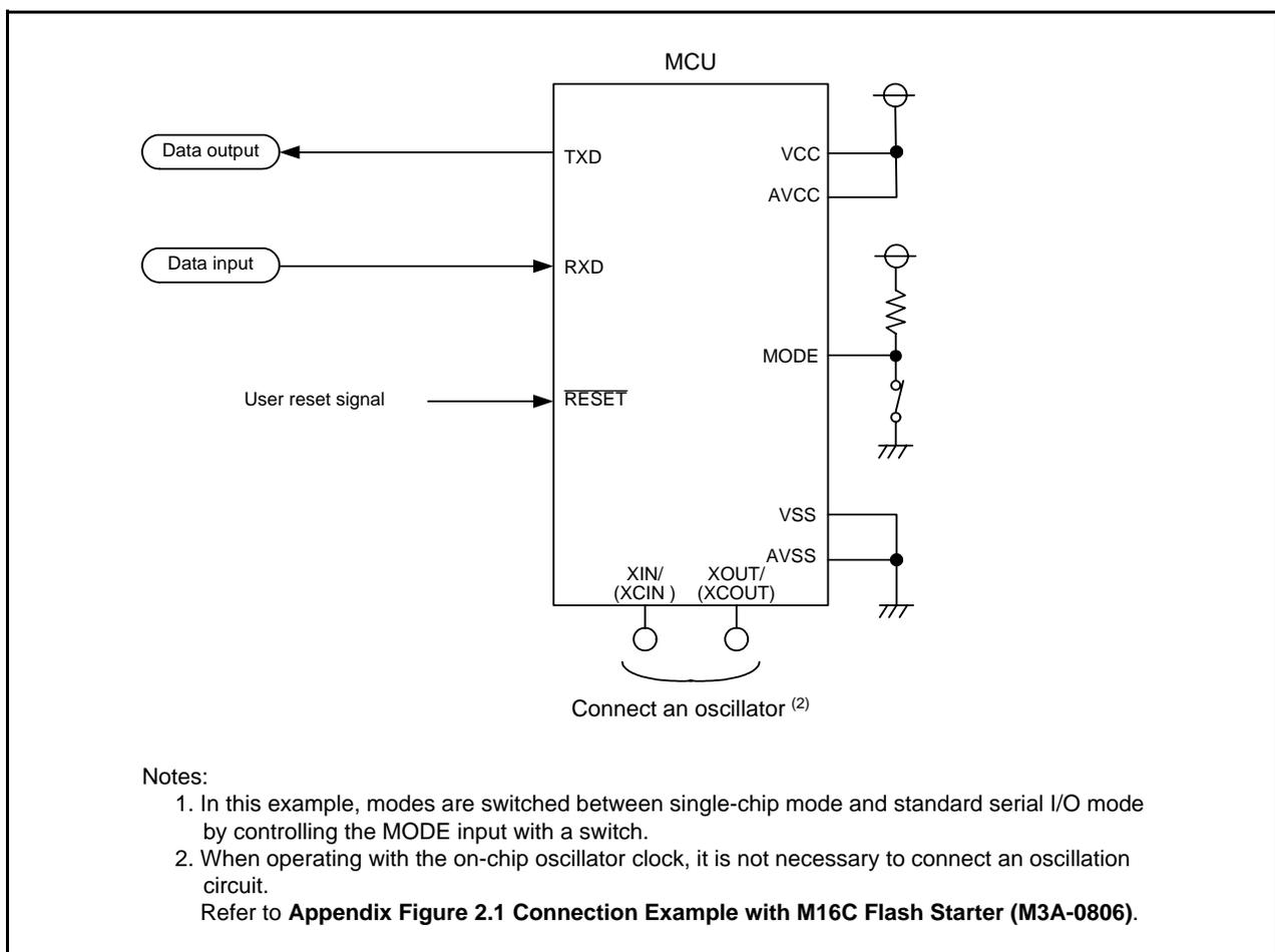
**Figure 24.16 Pin Handling in Standard Serial I/O Mode 2**
