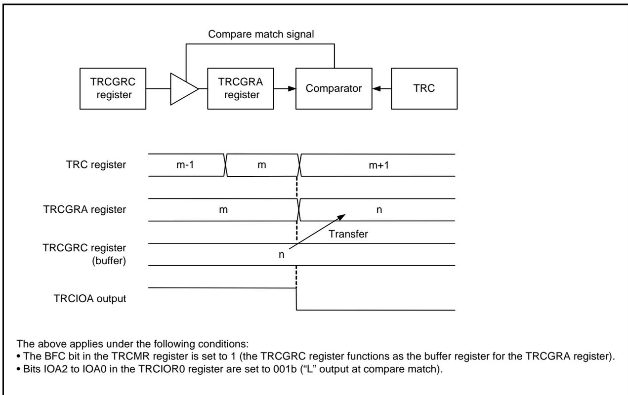
**Figure 18.4 Buffer Operation for Output Compare Function**
