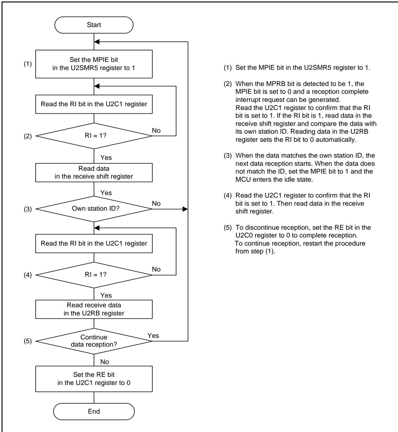
Figure 21.20 Sample Flowchart of Multiprocessor Data Reception
