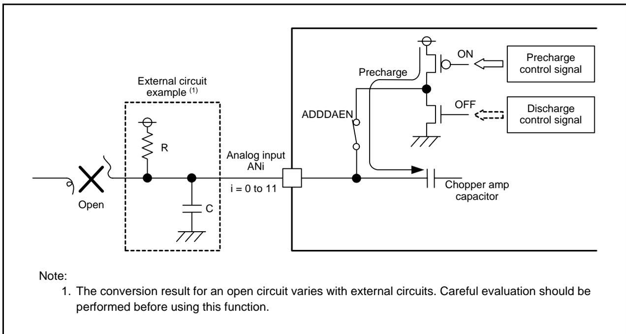
**Figure 22.5 A/D Open-Circuit Detection Example on AVCC Side (Precharge before Conversion Selected)**
