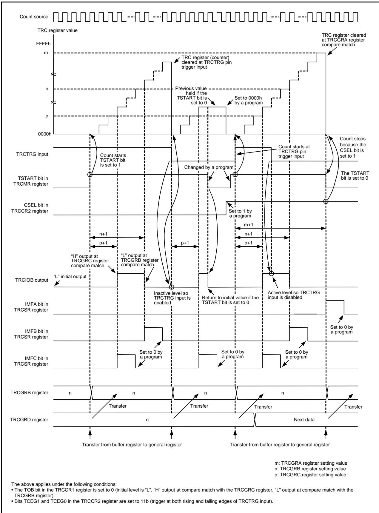
Figure 18.18 Operating Example of PWM2 Mode (TRCTRГ Trigger Input Enabled)
