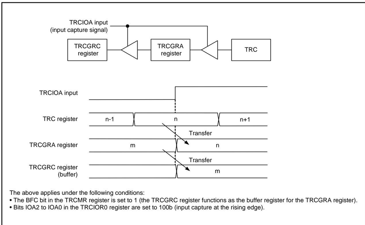
**Figure 18.3 Buffer Operation for Input Capture Function**
