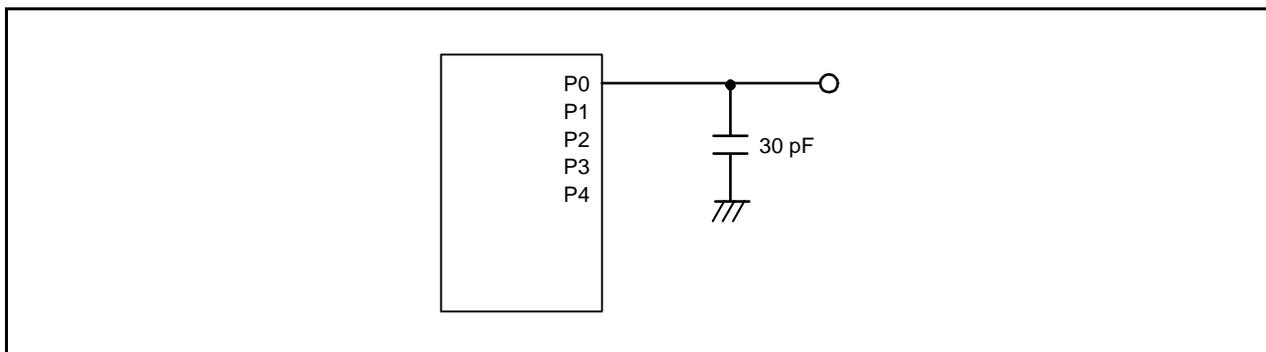
Figure 26.1 Ports P0 to P4 Timing Measurement Circuit
