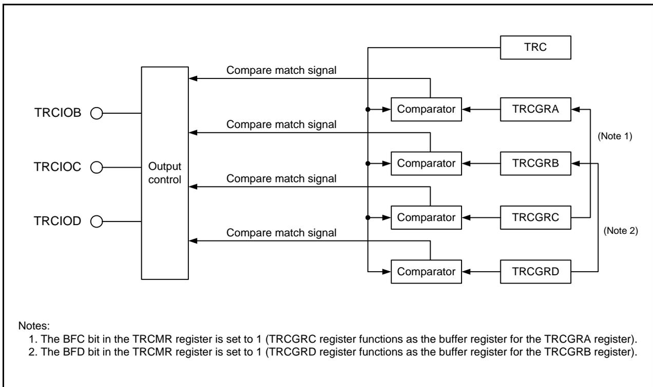
Figure 18.13 PWM Mode Block Diagram
