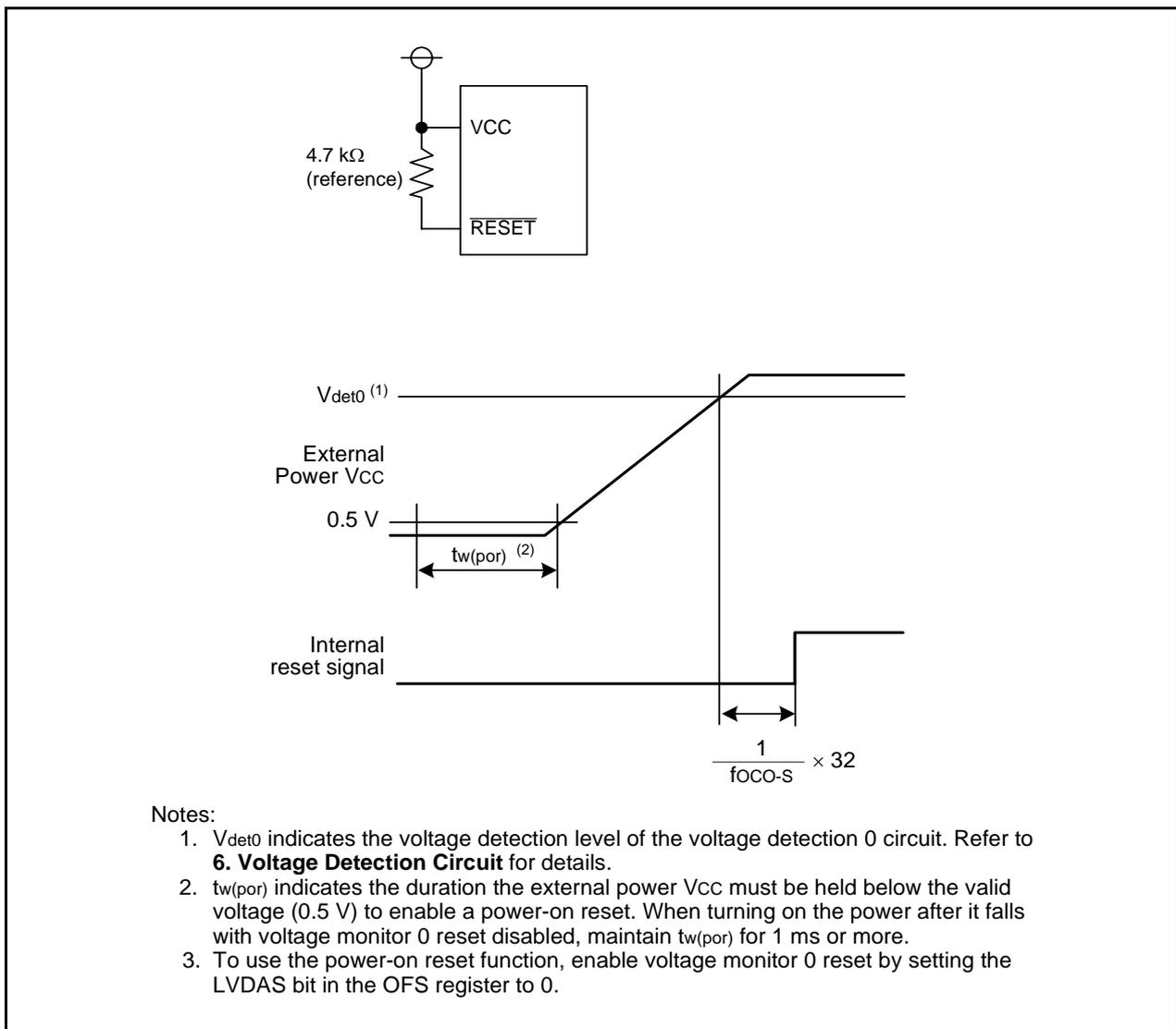
**Figure 5.6** Example of Power-On Reset Circuit and Operation
