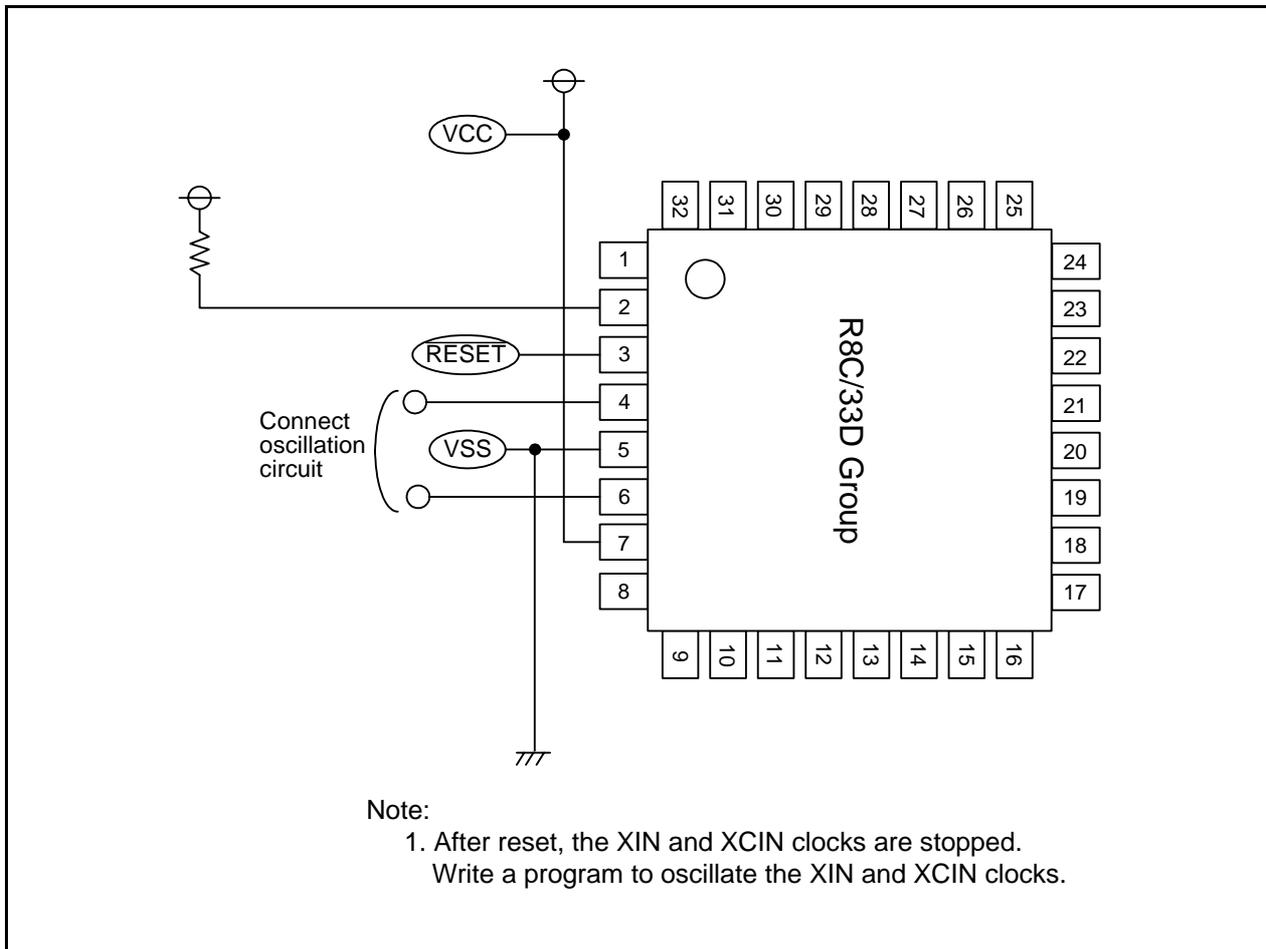
Appendix Figure 3.1 Example of Oscillation Evaluation Circuit
