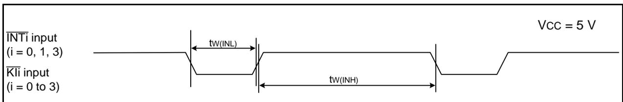
**Figure 26.7 Input Timing for External Interrupt  $\overline{INTi}$  and Key Input Interrupt  $\overline{Kli}$  when Vcc = 5 V**
