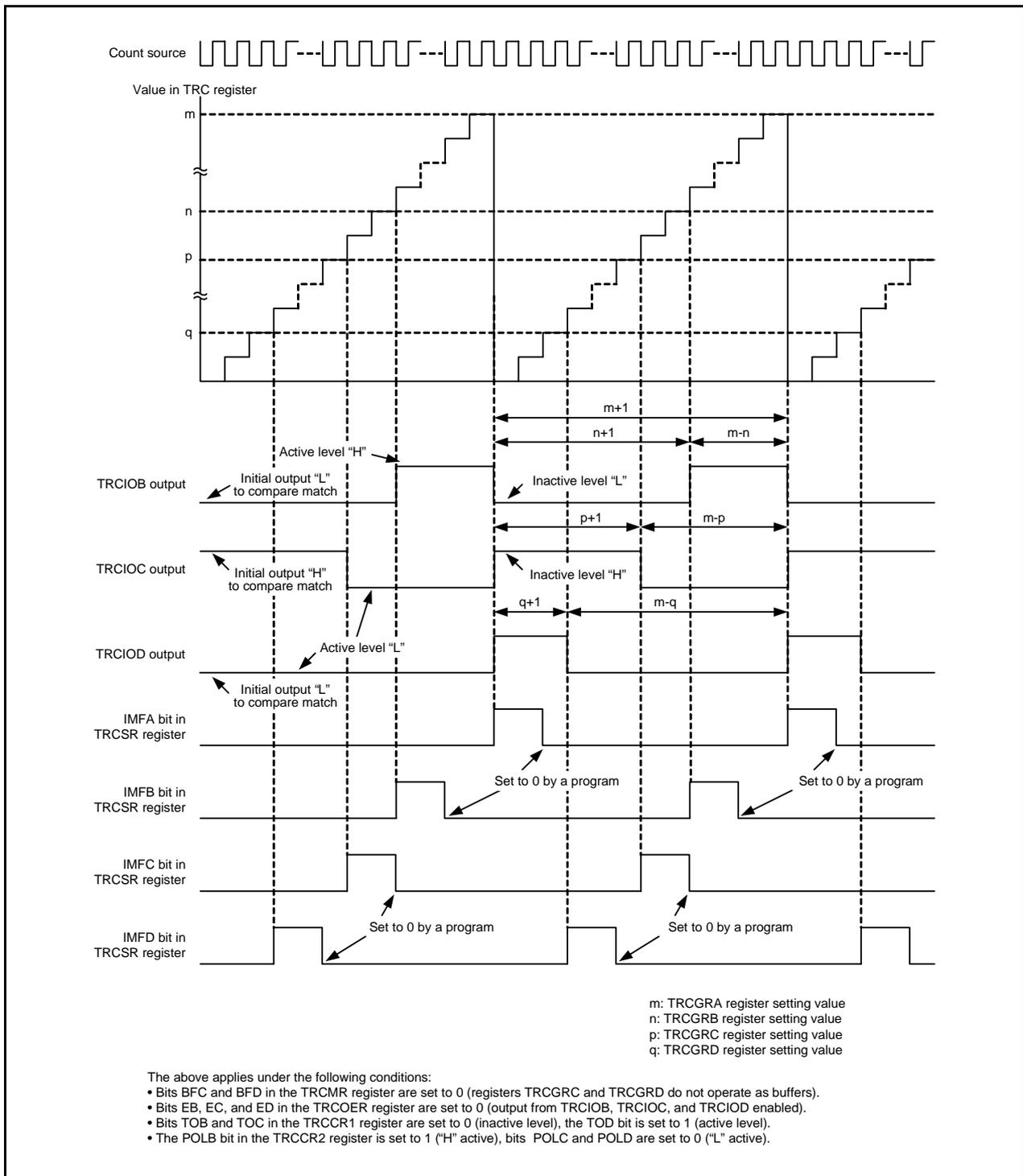
Figure 18.14 Operating Example of PWM Mode
