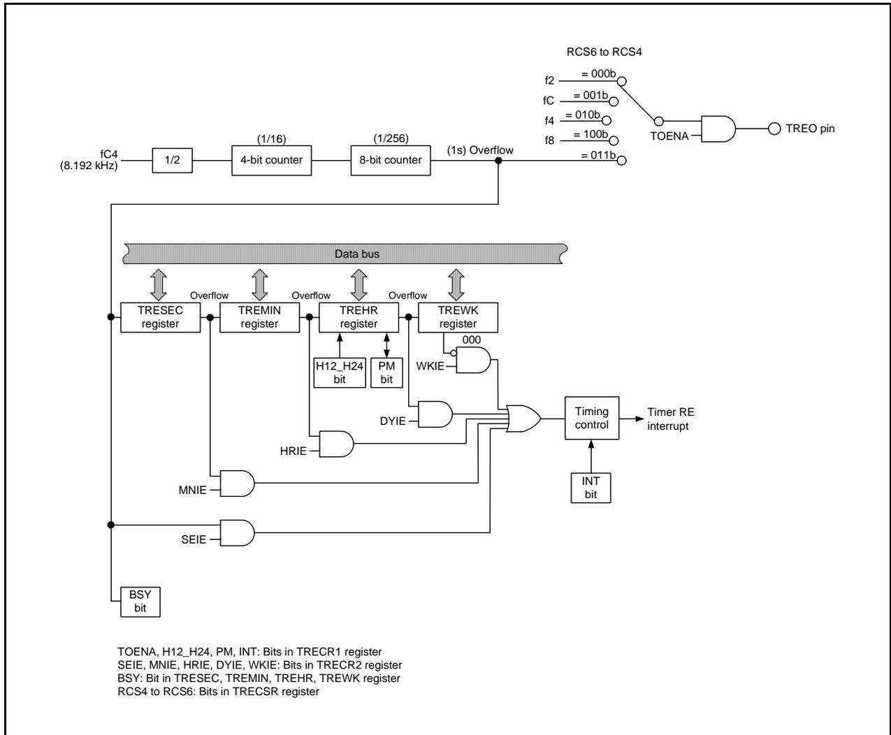
Figure 19.1 Block Diagram of Real-Time Clock Mode
