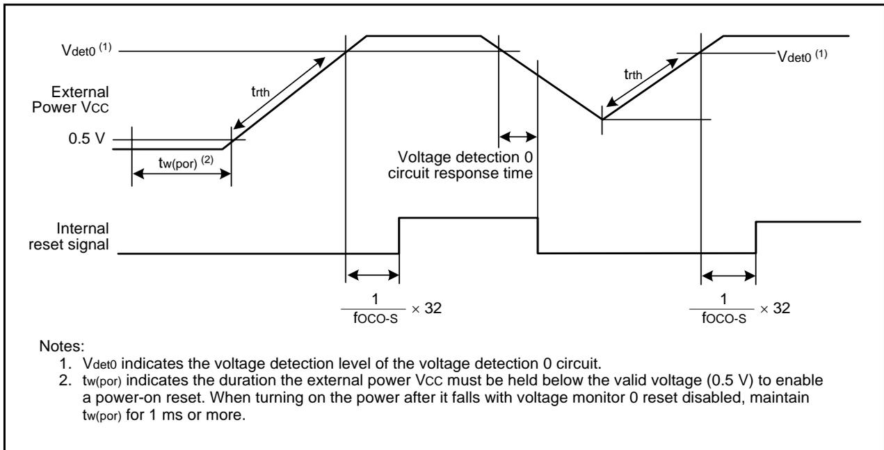
**Figure 26.3 Power-on Reset Circuit Electrical Characteristics**
