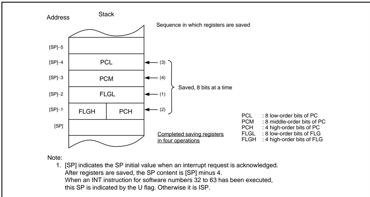
**Figure 11.6 Register Saving Operation**
