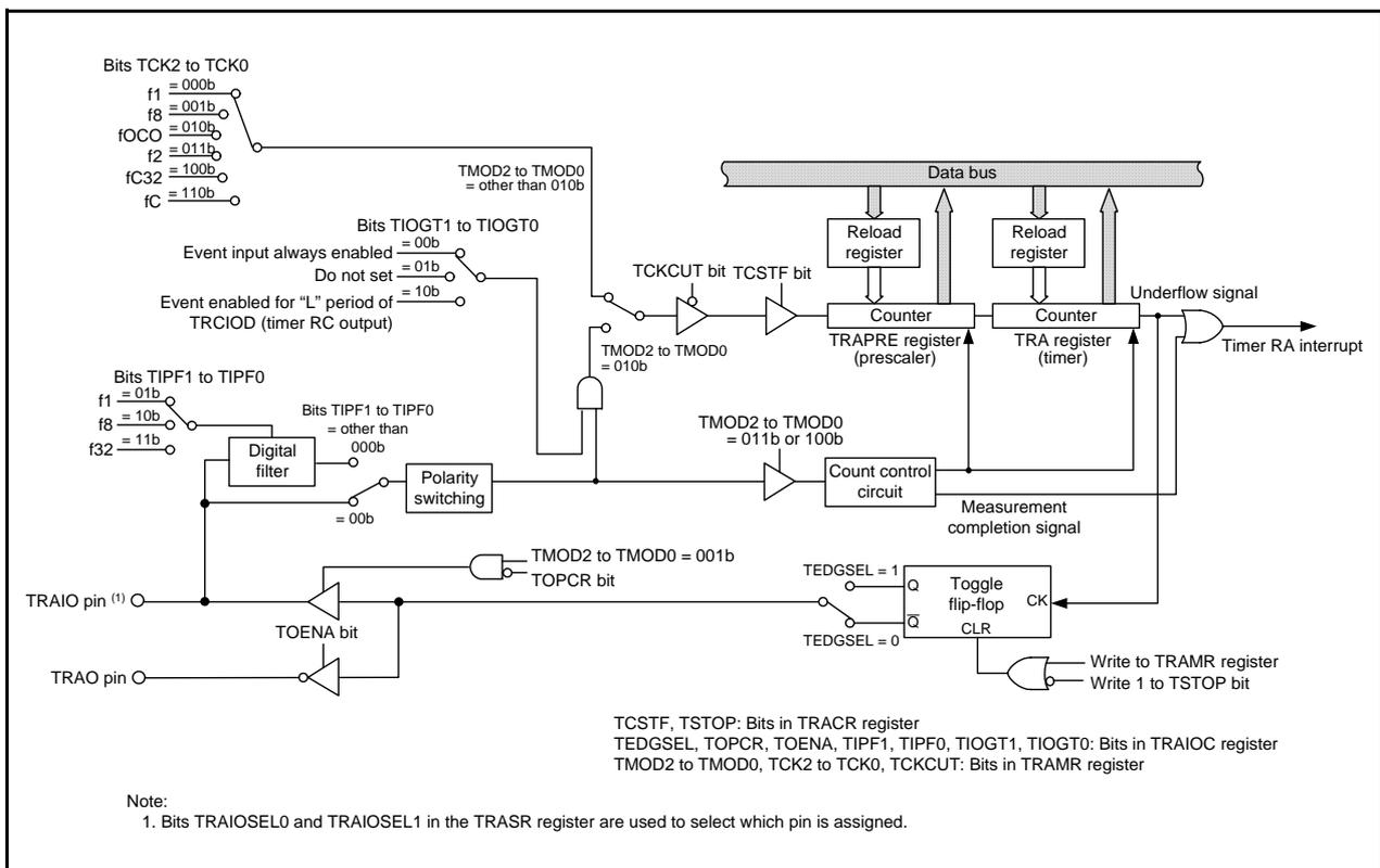
Figure 16.1 Timer RA Block Diagram
