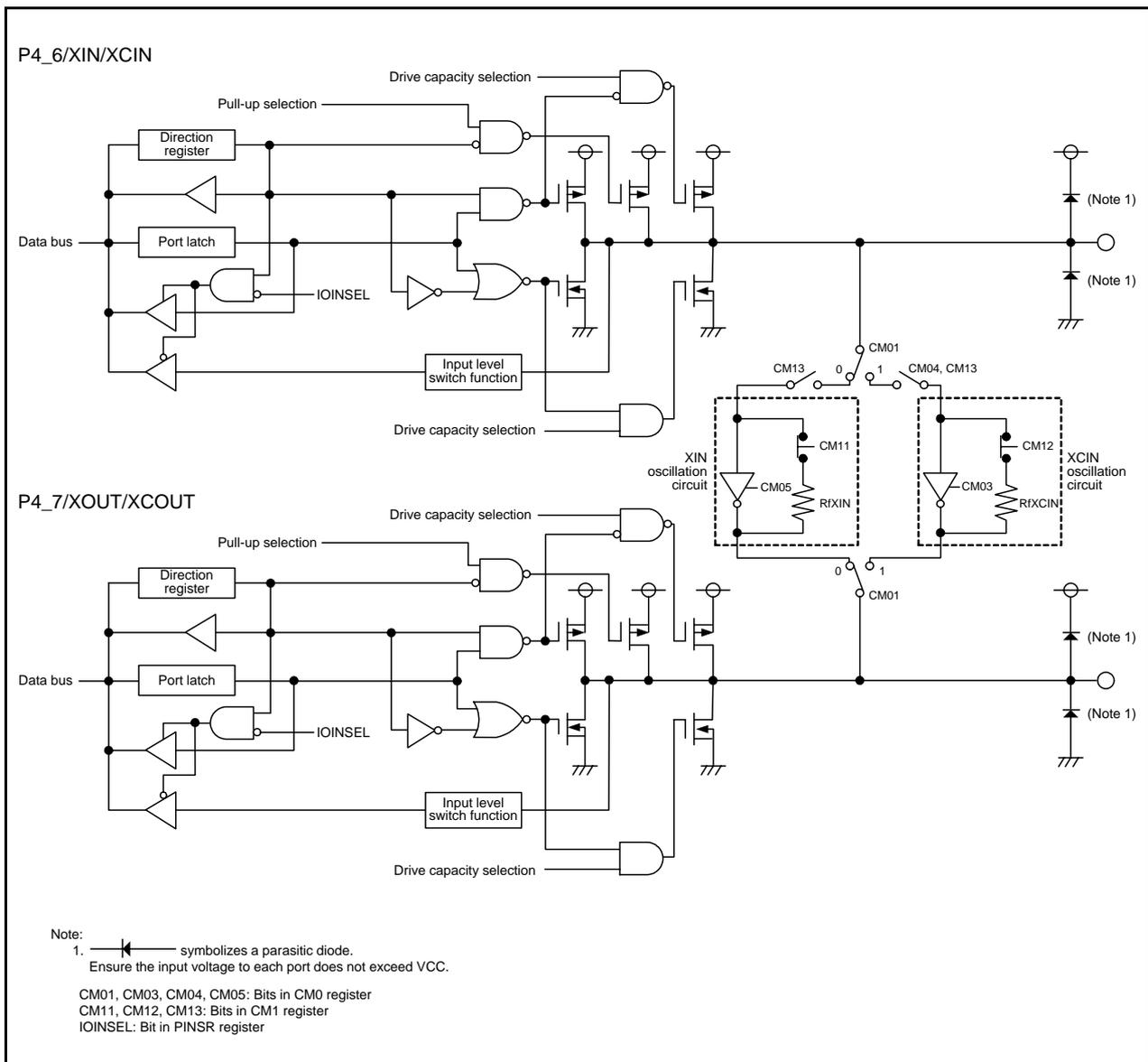
**Figure 7.10 Configuration of I/O Ports (10)**
