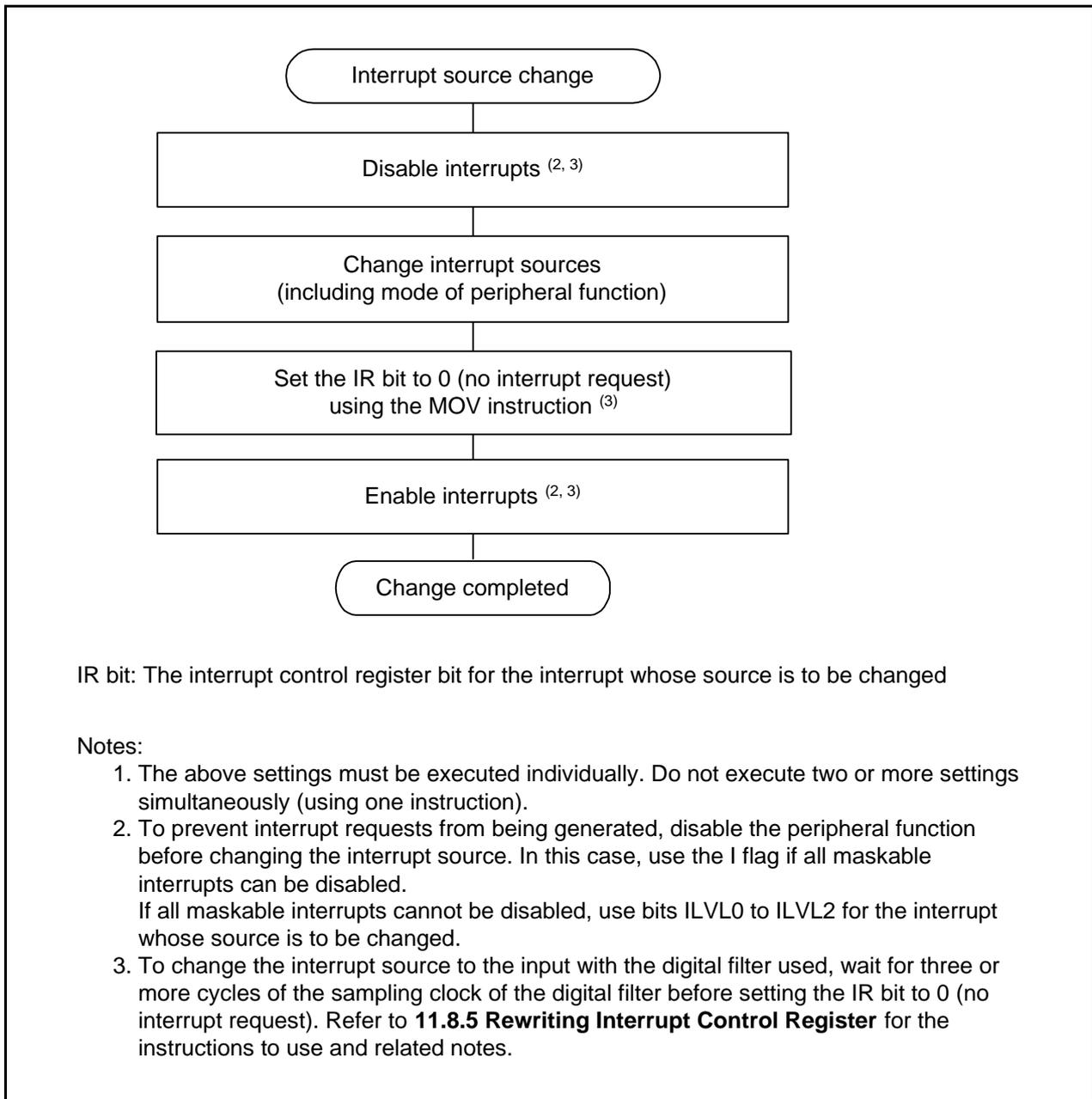
Figure 11.12 Procedure Example for Changing Interrupt Sources
