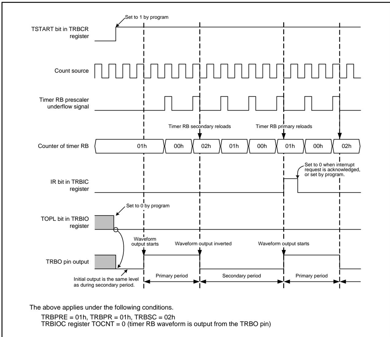
**Figure 17.3 Operating Example of Timer RB in Programmable Waveform Generation Mode**
