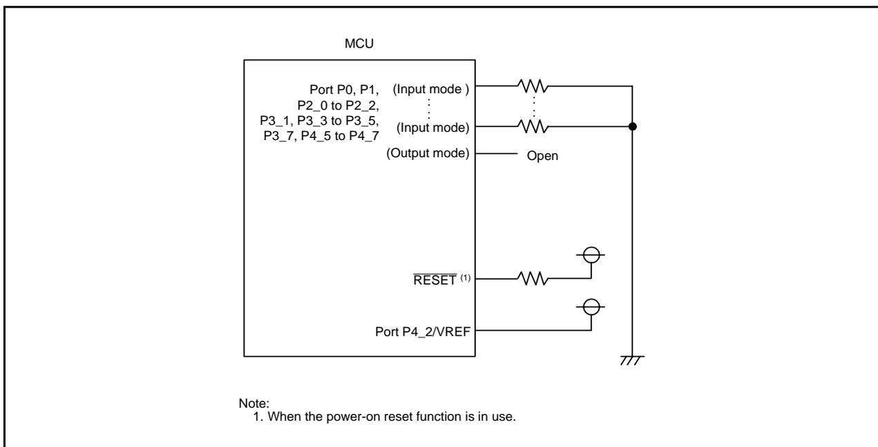
**Figure 7.12 Unassigned Pin Handling**
