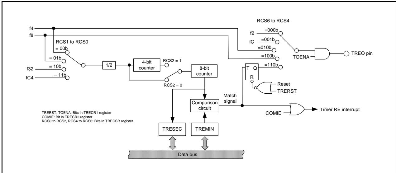
Figure 19.4 Block Diagram of Output Compare Mode
