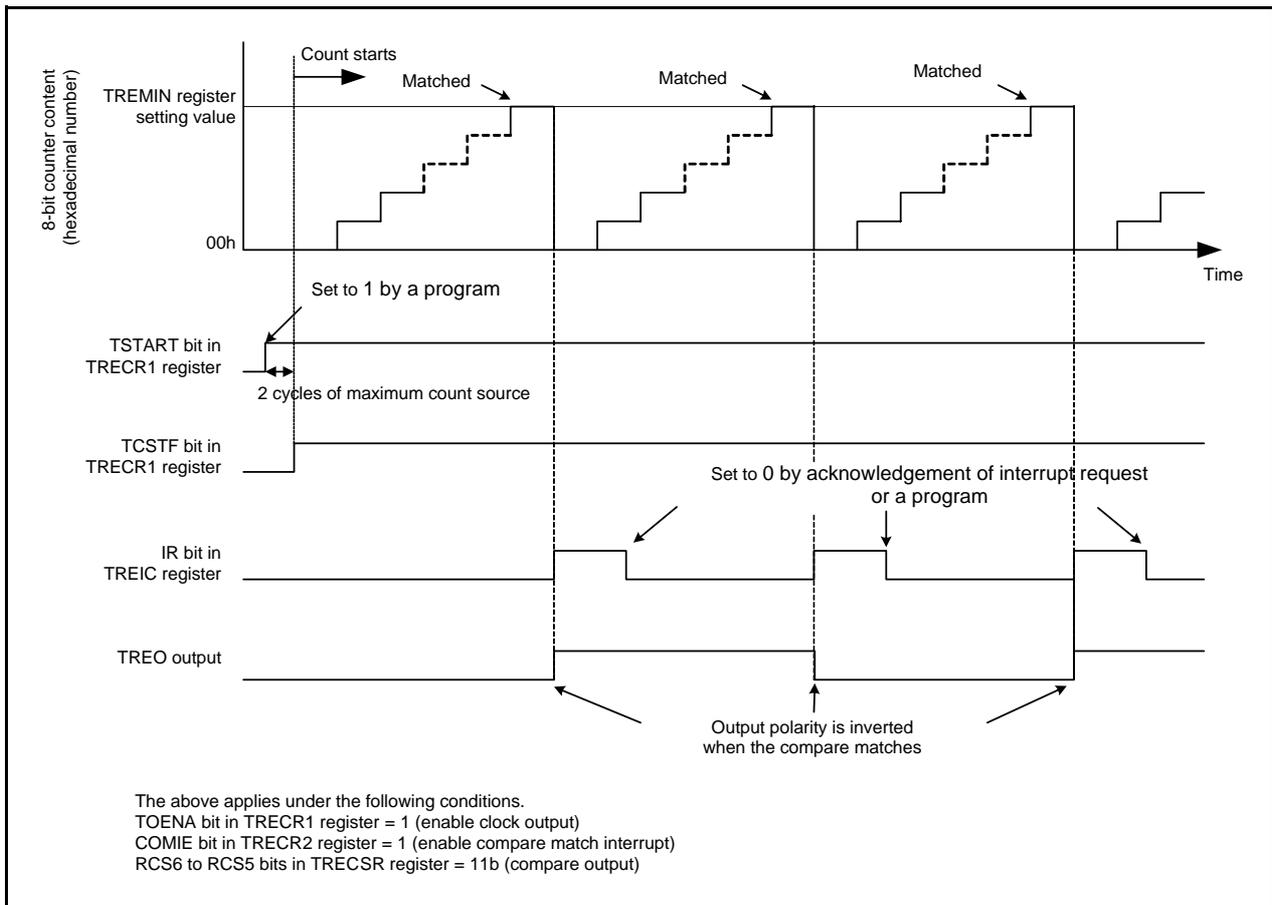
Figure 19.5 Operating Example in Output Compare Mode
