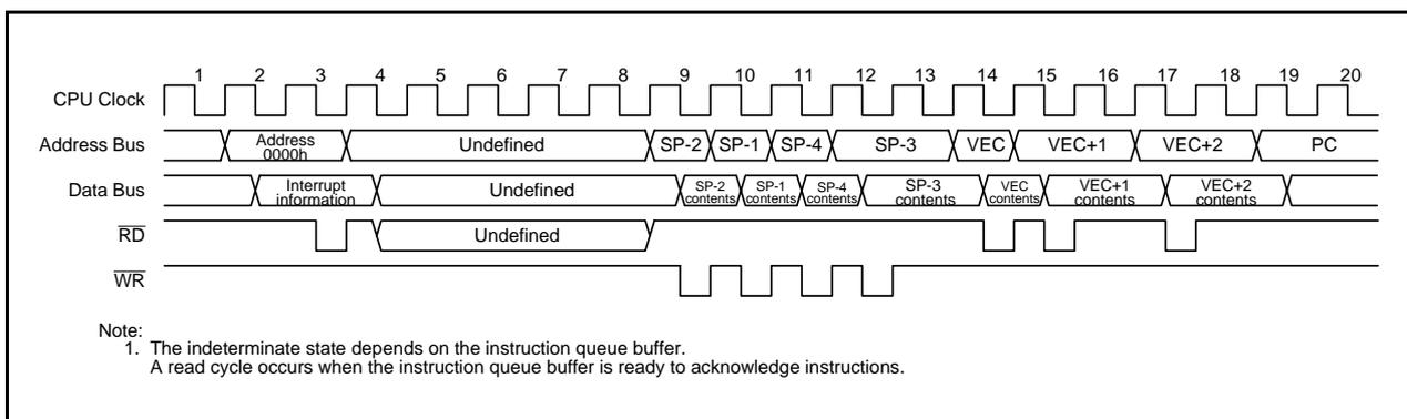
**Figure 11.3 Time Required for Executing Interrupt Sequence**
