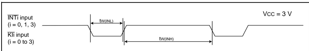
**Figure 26.11 Input Timing for External Interrupt  $\overline{INTi}$  and Key Input Interrupt  $\overline{Kli}$  when Vcc = 3 V**
