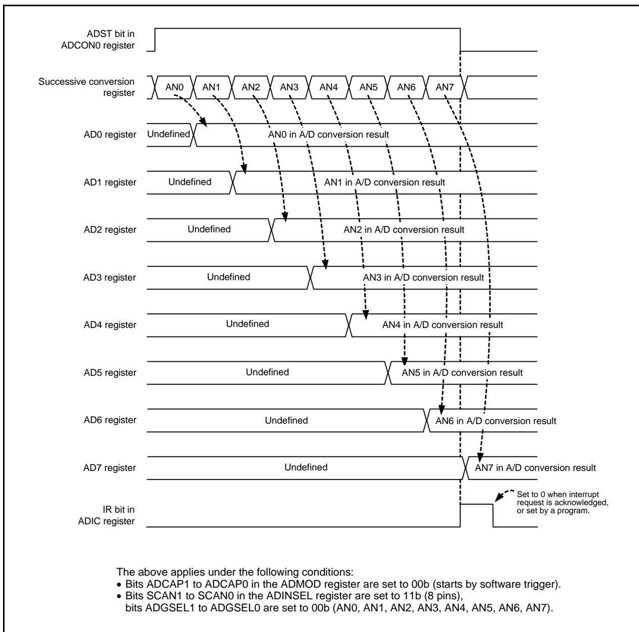
**Figure 22.8** Operating Example of Single Sweep Mode
