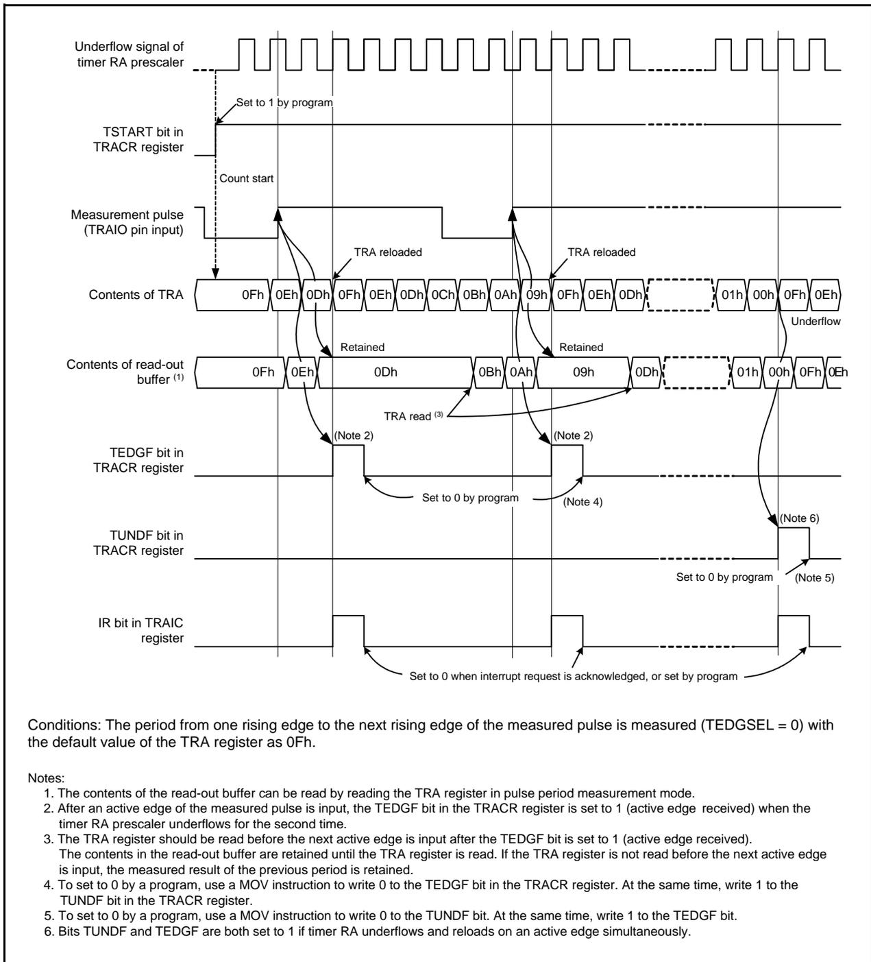
Figure 16.4 Operating Example of Pulse Period Measurement Mode
