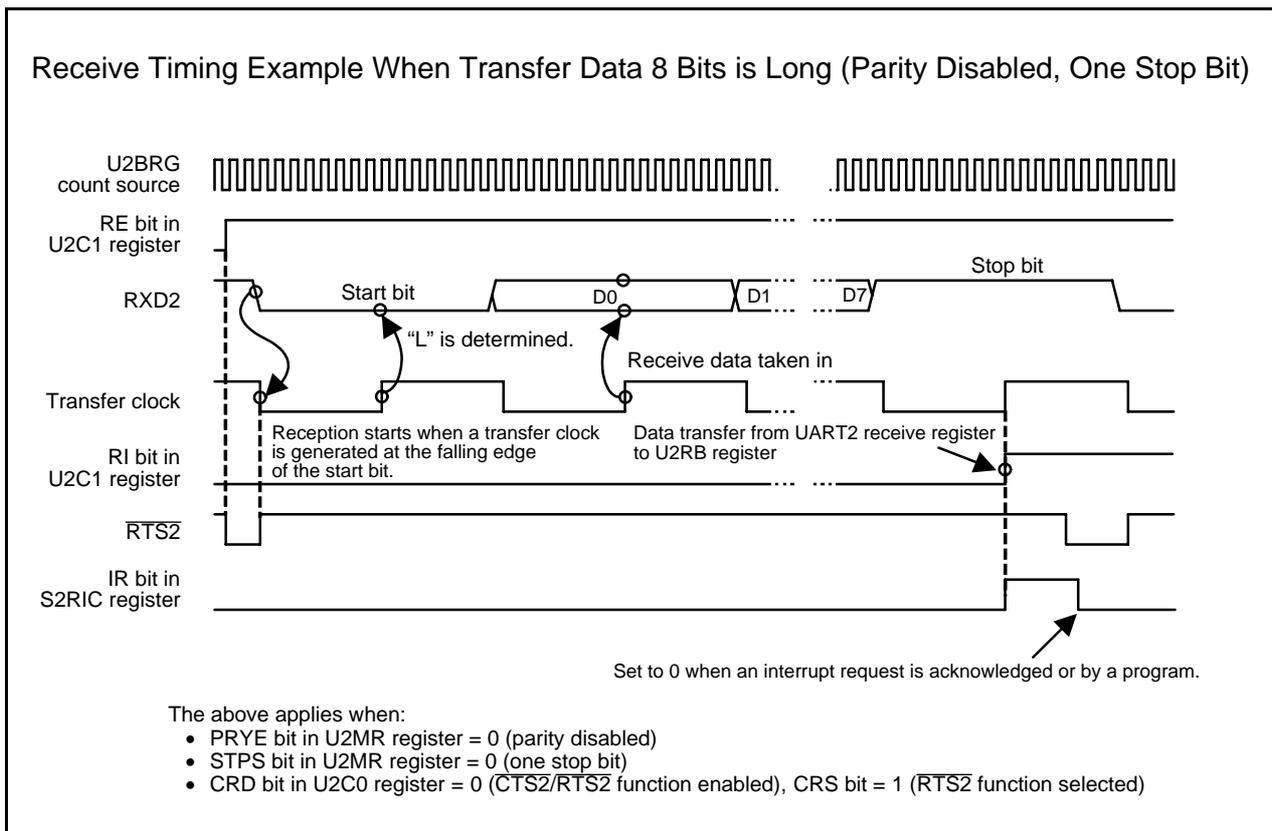
**Figure 21.8 Receive Timing in UART Mode**
