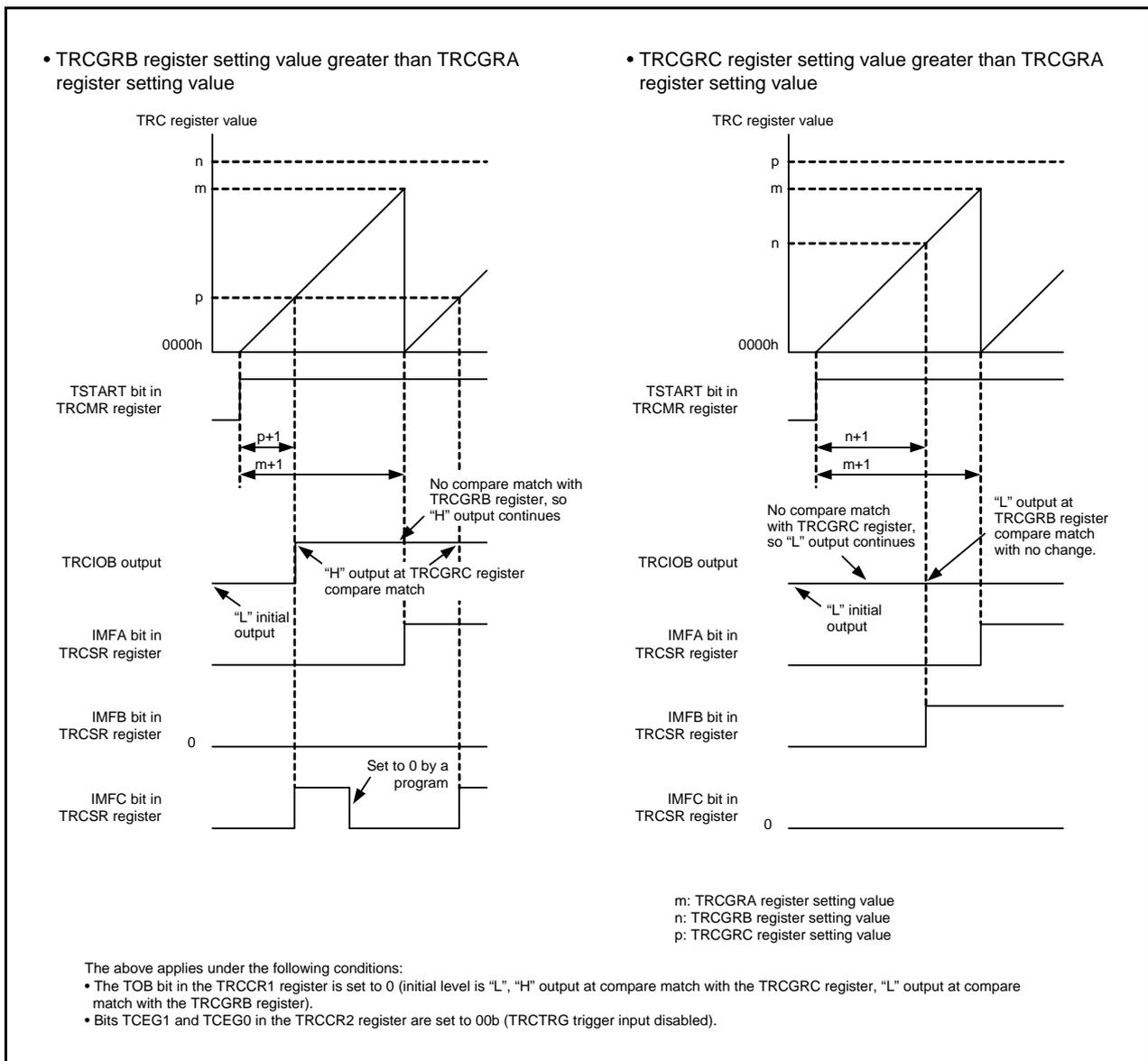
**Figure 18.19 Operating Example of PWM2 Mode (Duty 0% and Duty 100%)**
