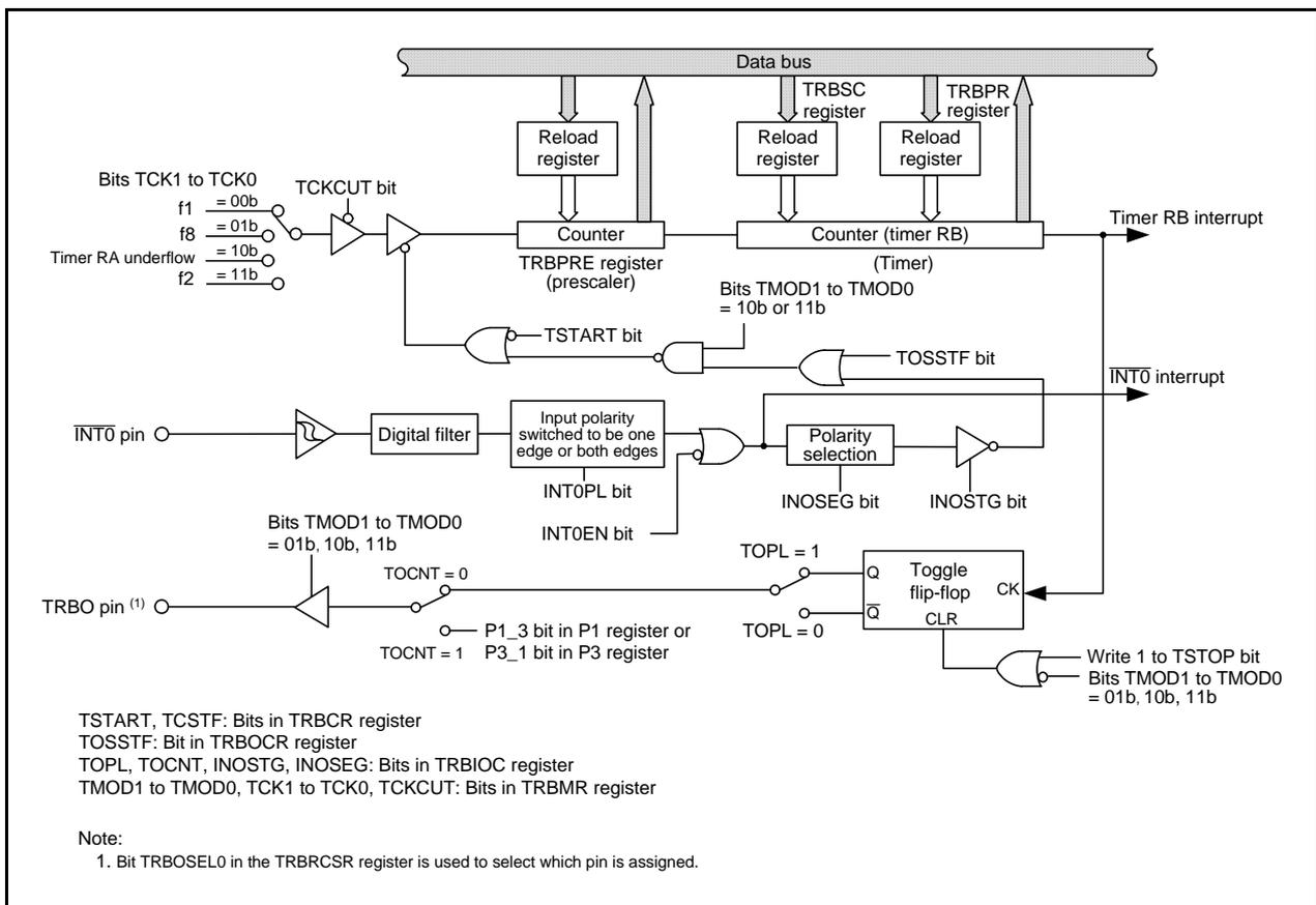
Figure 17.1 Timer RB Block Diagram
