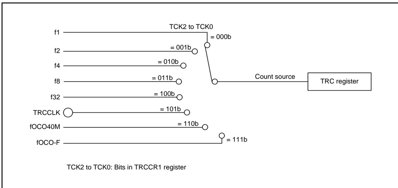
**Figure 18.2 Count Source Block Diagram**
