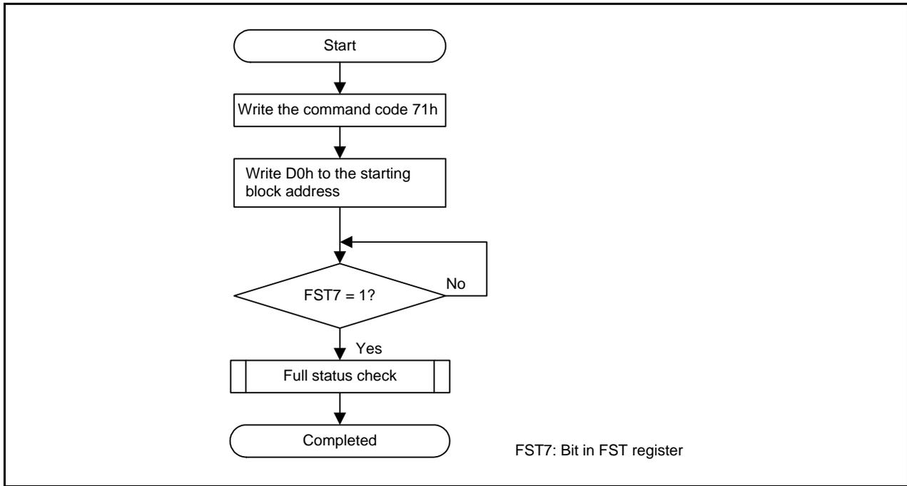
Figure 24.13 Read Lock Bit Status Flowchart
