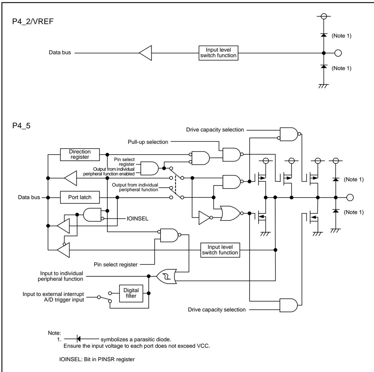
**Figure 7.9 Configuration of I/O Ports (9)**
