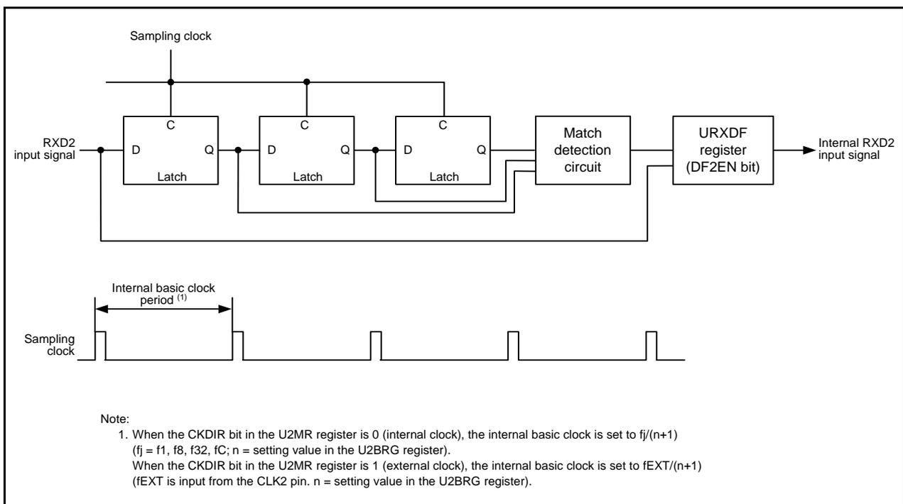
Figure 21.12 Block Diagram of RXD2 Digital Filter Circuit
