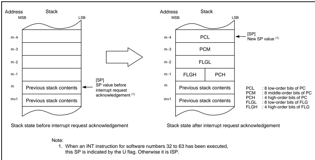
**Figure 11.5 Stack State Before and After Acknowledgement of Interrupt Request**
