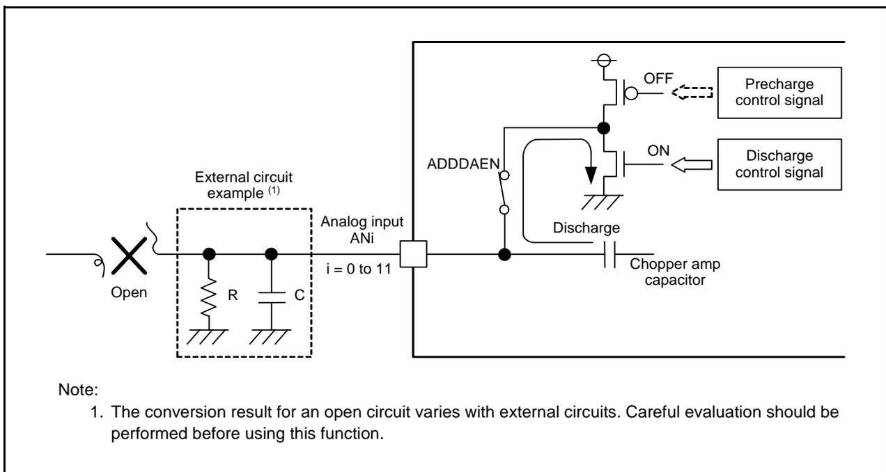
**Figure 22.6 A/D Open-Circuit Detection Example on AVSS Side (Discharge before Conversion Selected)**
