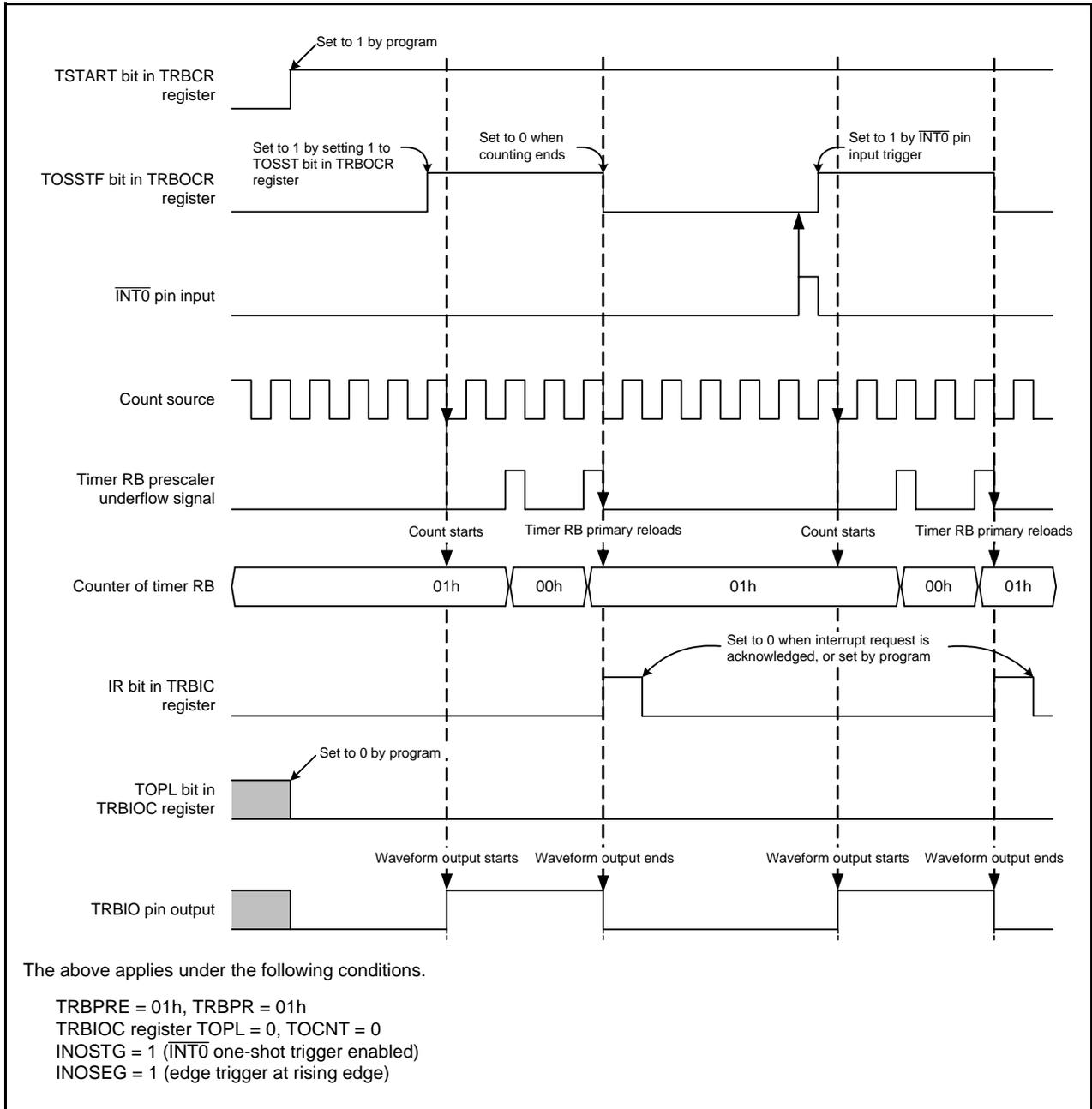
Figure 17.4 Operating Example of Programmable One-Shot Generation Mode
