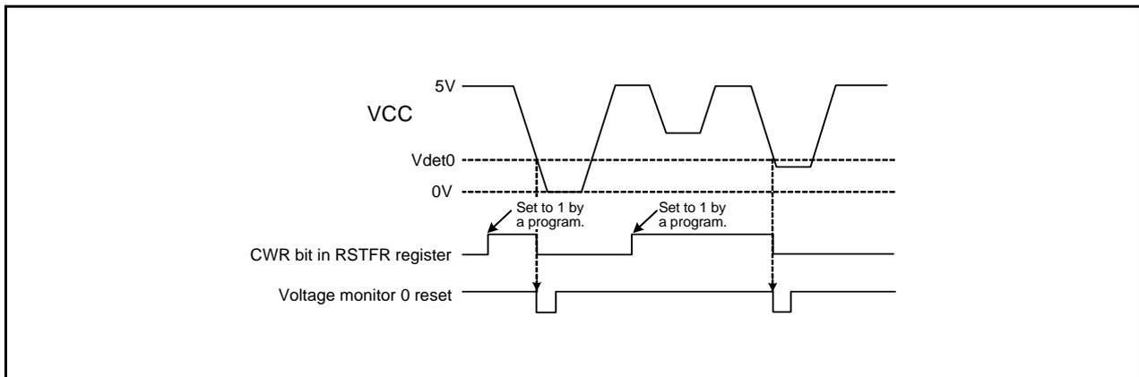
Figure 5.8 Operating Example of Cold Start-Up/Warm Start-Up Function
