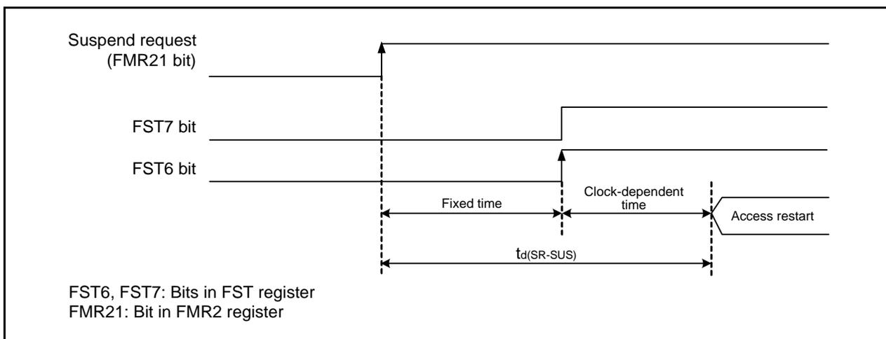
**Figure 26.2 Time delay until Suspend**
