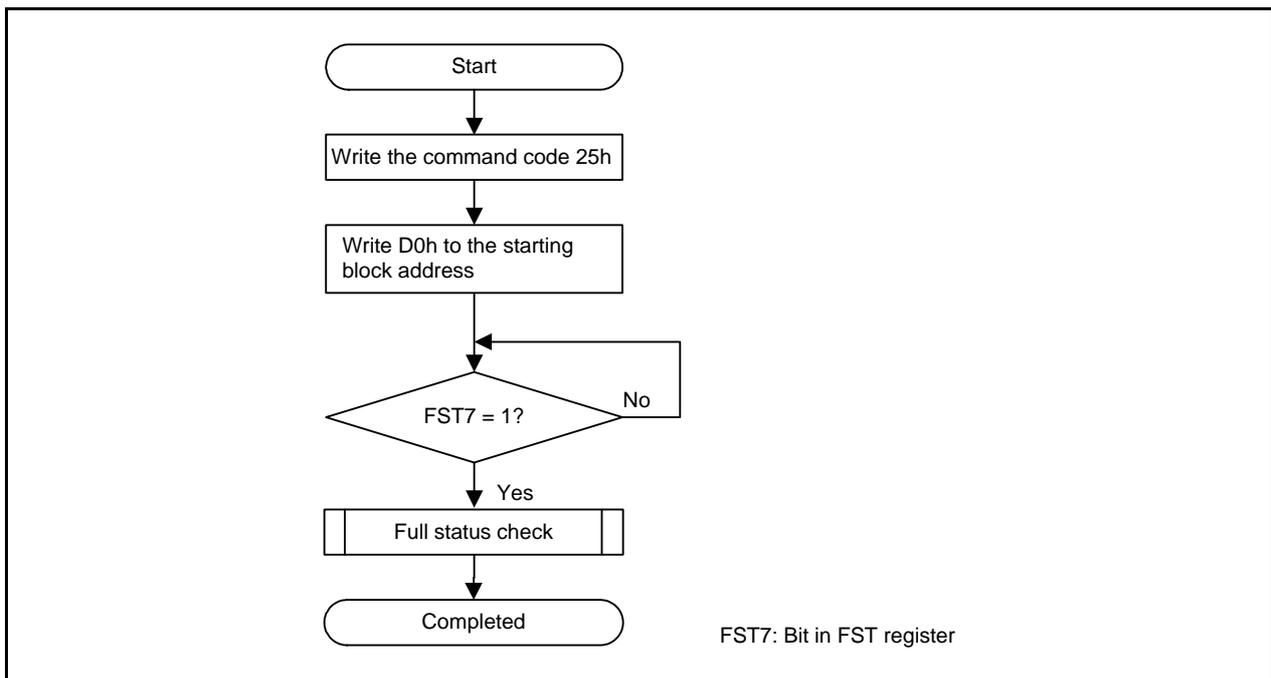
**Figure 24.14** Block Blank Check Flowchart
