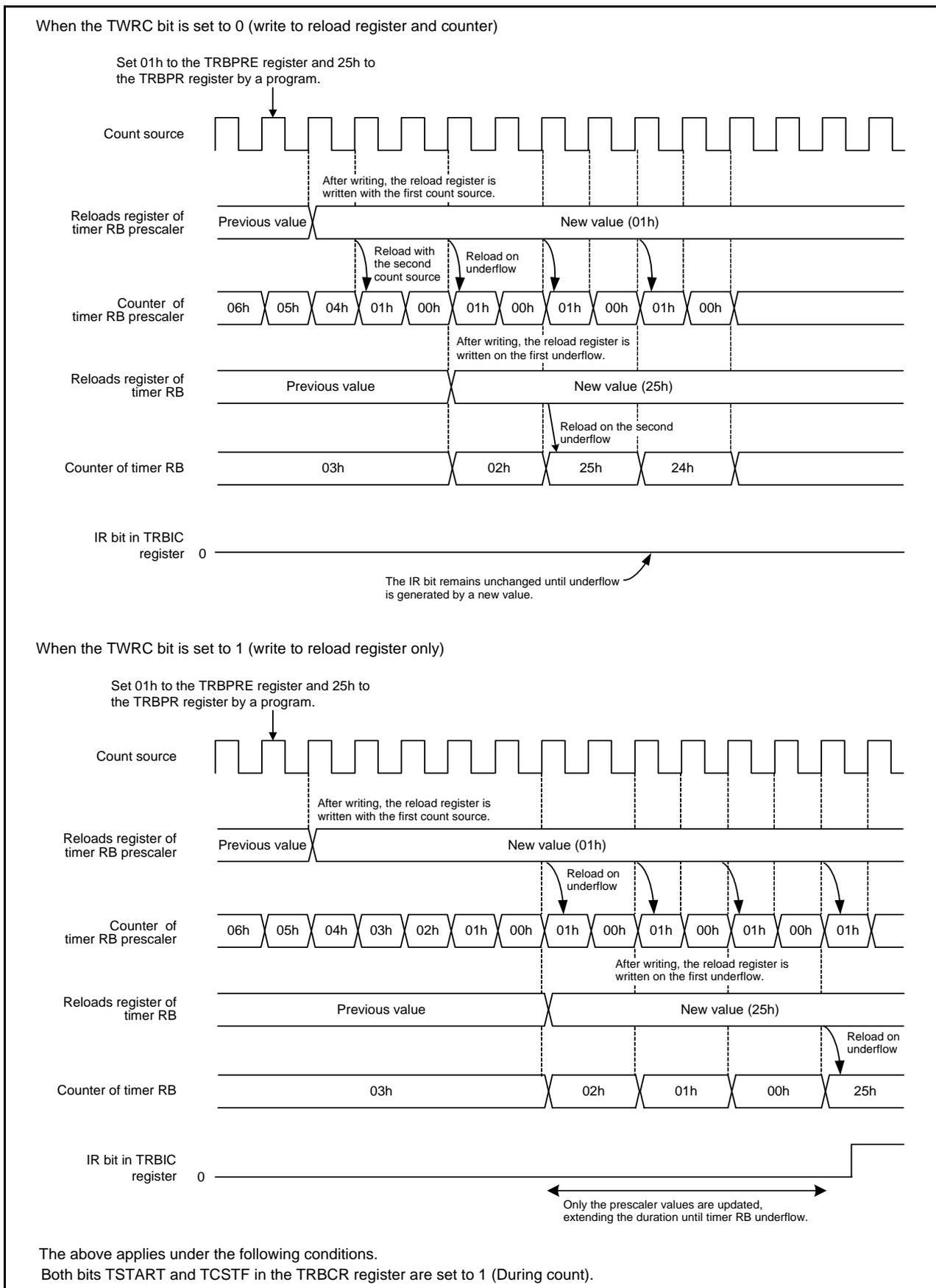
**Figure 17.2 Operating Example of Timer RB when Counter Value is Rewritten during Count Operation**
