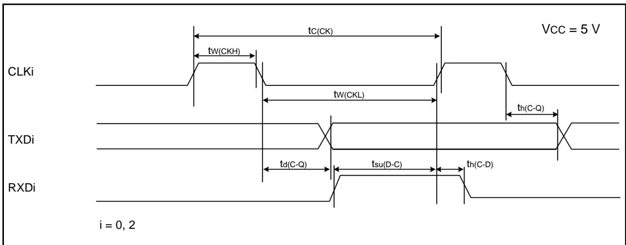
**Figure 26.6 Serial Interface Timing Diagram when Vcc = 5 V**
