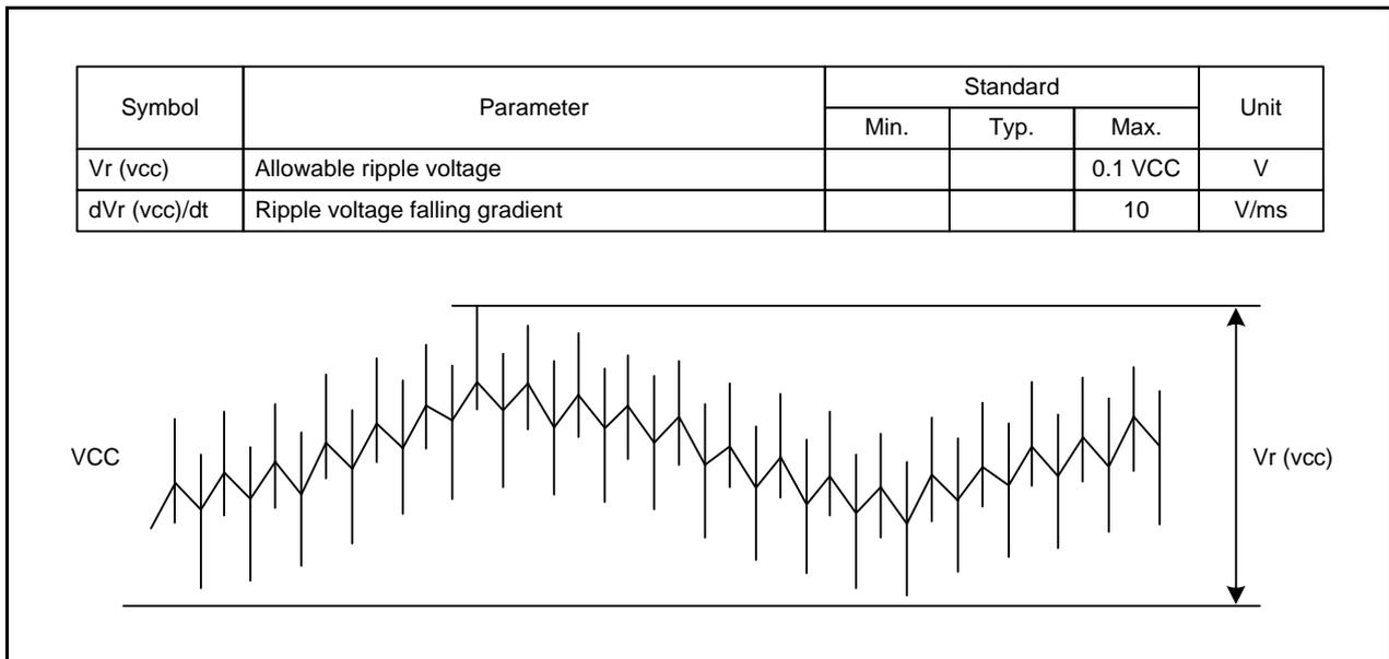
Figure 27.3 Definition of ripple voltage
