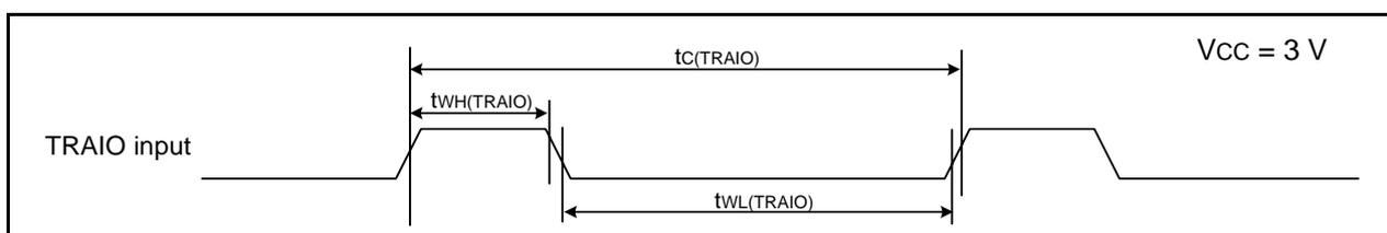
**Figure 26.9 TRAIO Input Timing Diagram when  $V_{CC} = 3\text{ V}$**
