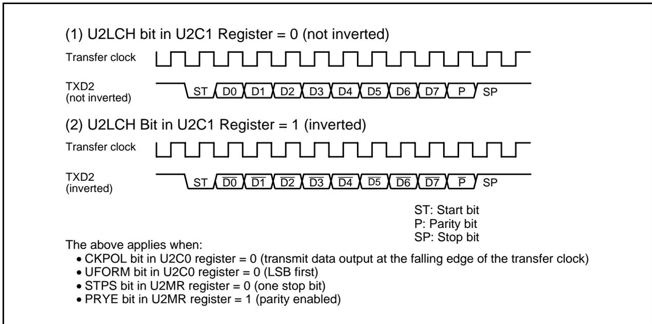
Figure 21.10 Serial Data Logic Switching
