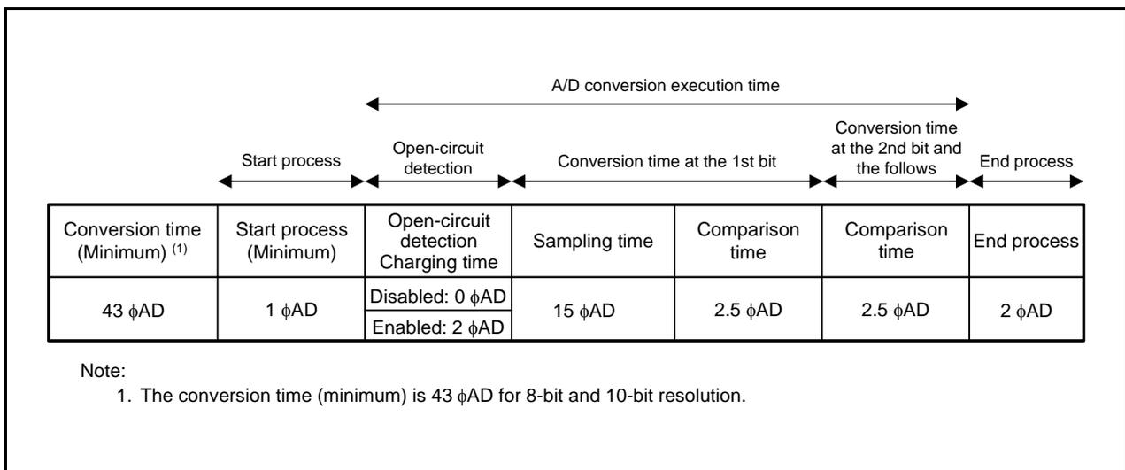
Figure 22.3 A/D Conversion Cycles ( $\phi_{AD} = f_{AD}$ )
