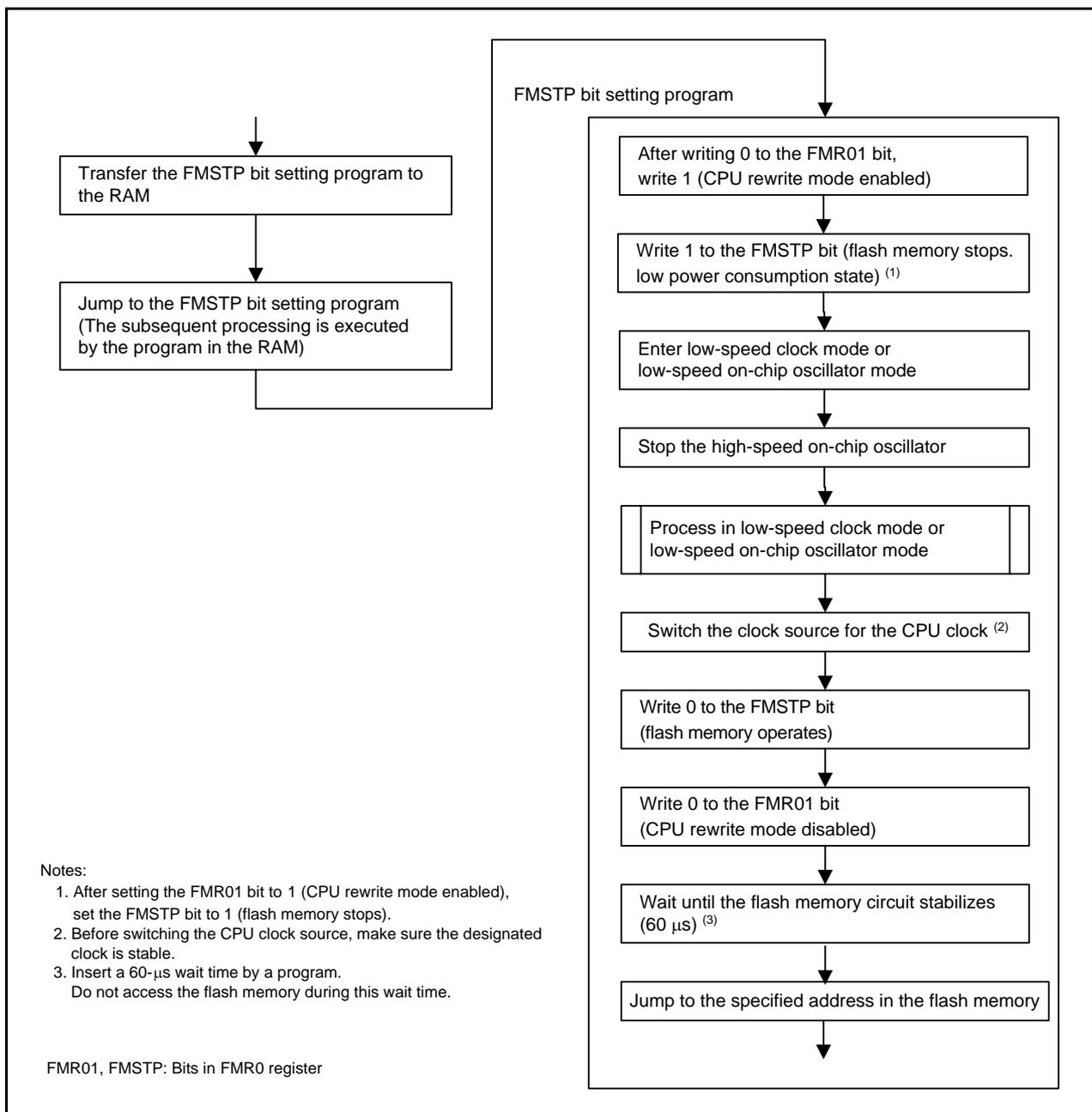
Figure 25.2 Handling Procedure Example for Reducing Power Consumption Using FMSTP Bit
