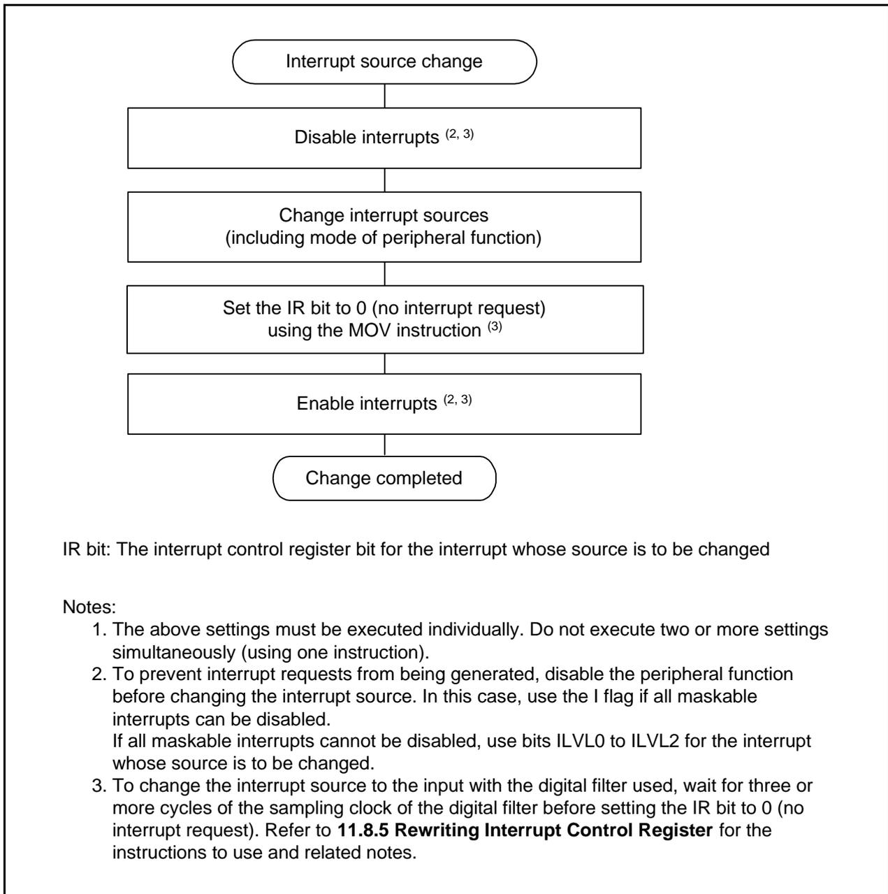
Figure 27.1 Procedure Example for Changing Interrupt Sources
