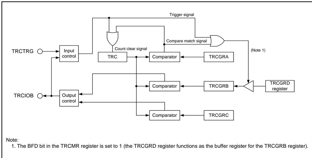
**Figure 18.16 PWM2 Mode Block Diagram**
