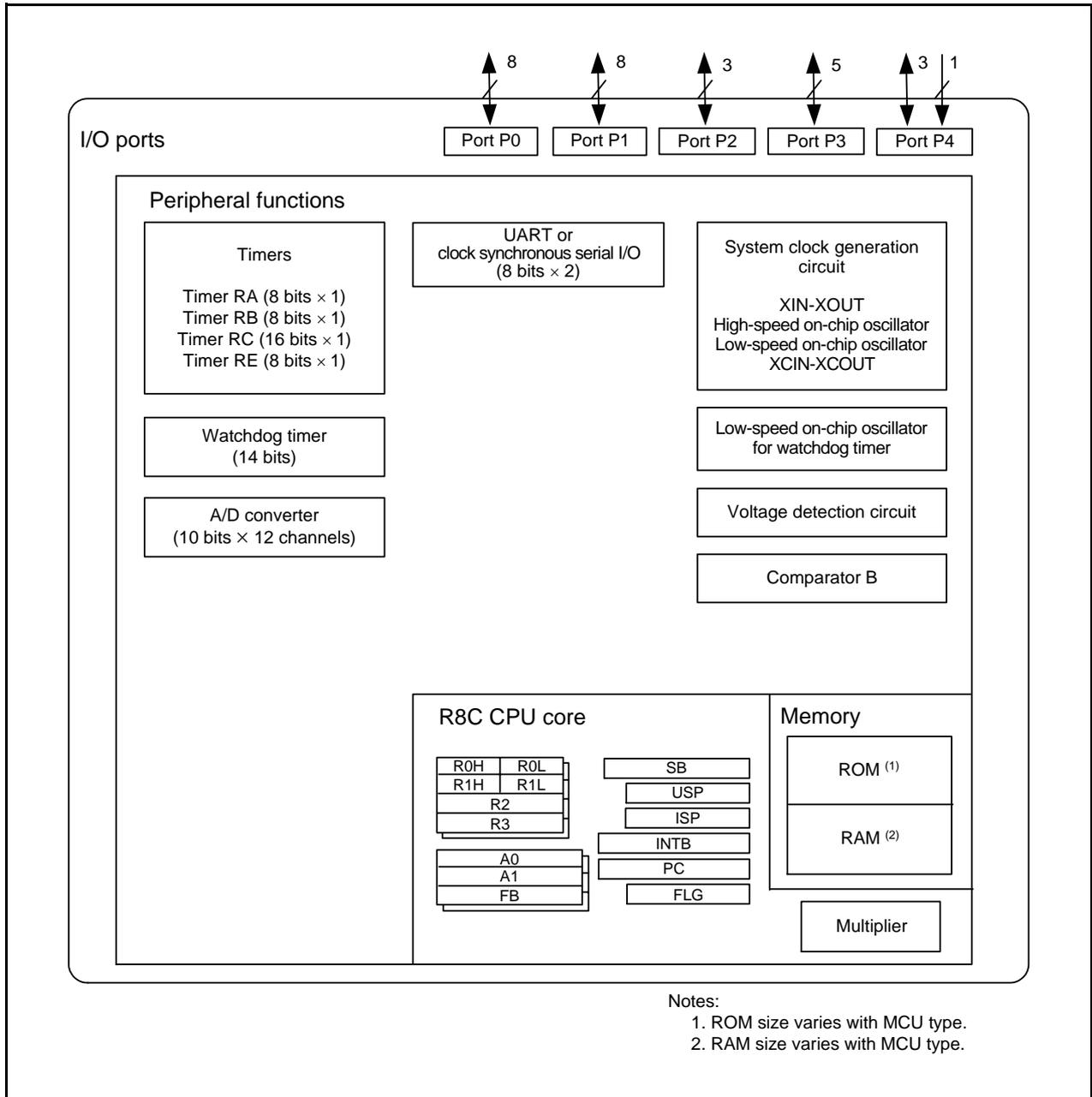
Figure 1.2 Block Diagram
