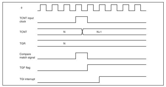
Figure 10.38 TGI Interrupt Timing (Compare Match)
