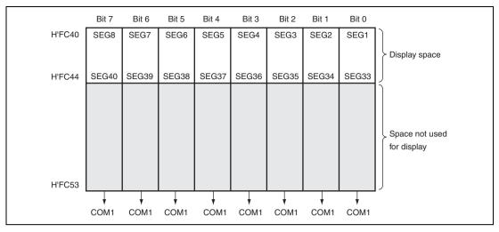
Figure 17.6 LCD RAM Map (Static Mode)
