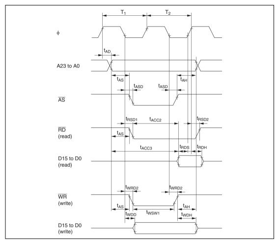
Figure 23.6 Basic Bus Timing (Two-State Access)
