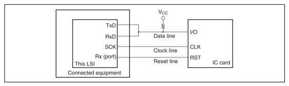
Figure 13.21 Schematic Diagram of Smart Card Interface Pin Connections
