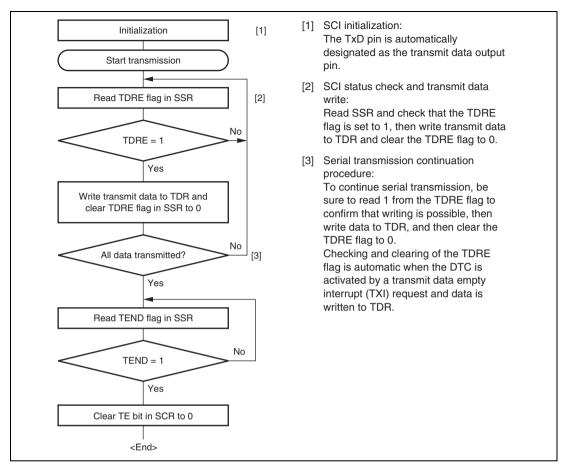
Figure 13.17 Sample Serial Transmission Flowchart
