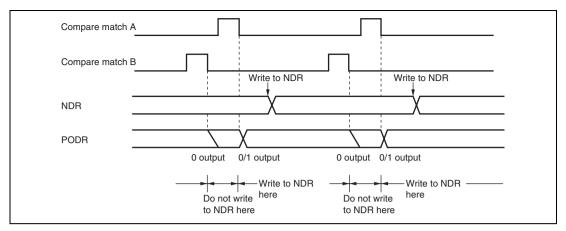
Figure 11.7 Non-Overlapping Operation and NDR Write Timing
