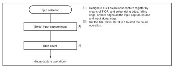
Figure 10.8 Example of Input Capture Operation Setting Procedure
