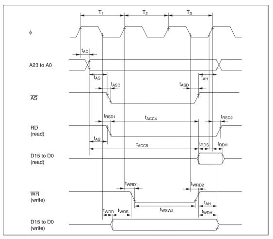
Figure 23.7 Basic Bus Timing (Three-State Access)
