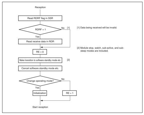
$Figure\ 13.37\quad Sample\ Flowchart\ for\ Mode\ Transition\ during\ Reception$
