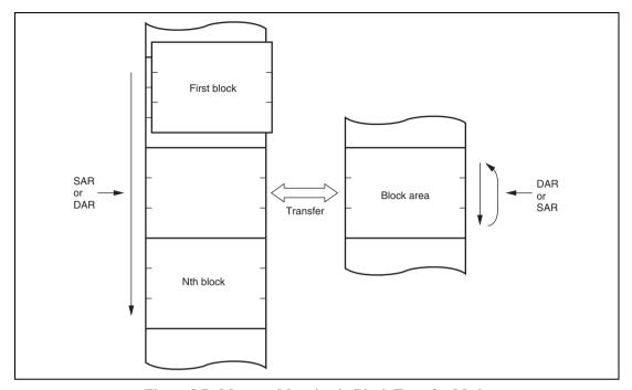
Figure 8.7 Memory Mapping in Block Transfer Mode
