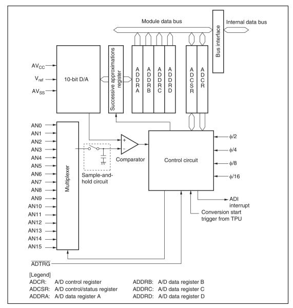
Figure 15.1 Block Diagram of A/D Converter
