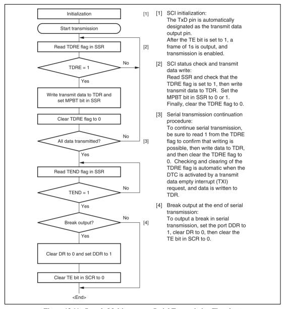
Figure 13.11 Sample Multiprocessor Serial Transmission Flowchart
