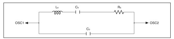
Figure 20.7 Equivalent Circuit for 32.768-kHz Crystal Resonator
