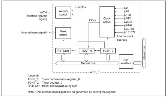
Figure 12.1 Block Diagram of WDT\_0
