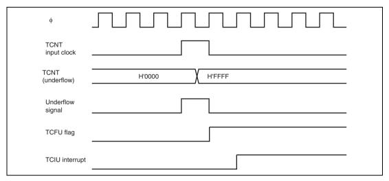
Figure 10.41 TCIU Interrupt Setting Timing
