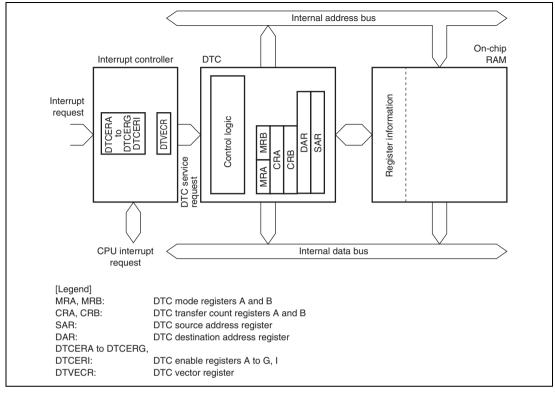
Figure 8.1 Block Diagram of DTC
