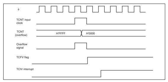
Figure 10.40 TCIV Interrupt Setting Timing
