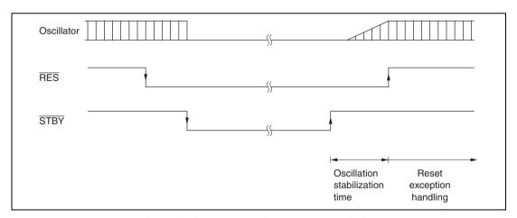
Figure 21.4 Hardware Standby Mode Timing
