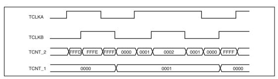
Figure 10.19 Example of Cascaded Operation (2)
