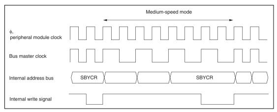
Figure 21.2 Medium-Speed Mode Transition and Clearance Timing
