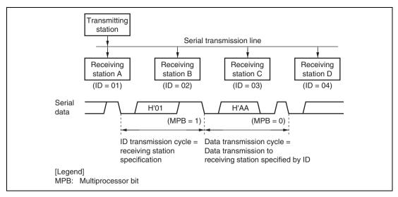
Figure 13.10 Example of Communication Using Multiprocessor Format (Transmission of Data H'AA to Receiving Station A)
