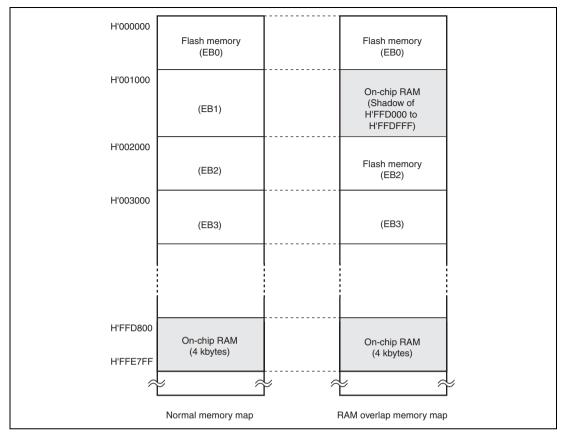
Figure 19.8 Example of RAM Overlap Operation
