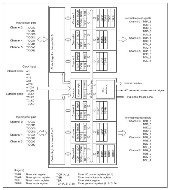
Figure 10.1 Block Diagram of TPU
