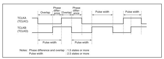
Figure 10.44 Phase Difference, Overlap, and Pulse Width in Phase Counting Mode
