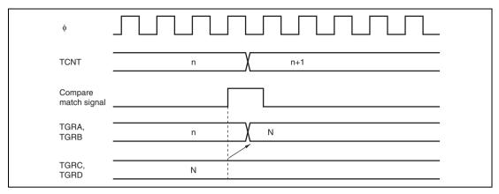
Figure 10.36 Buffer Operation Timing (Compare Match)
