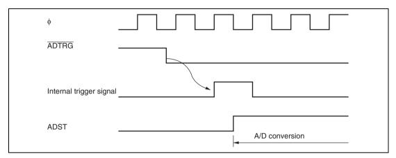
Figure 15.3 External Trigger Input Timing
