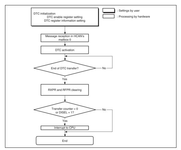
Figure 14.15 DTC Transfer Flowchart
