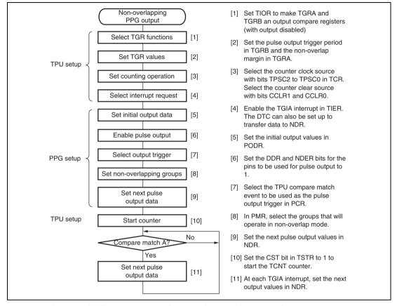
Figure 11.8 Setup Procedure for Non-Overlapping Pulse Output (Example)
