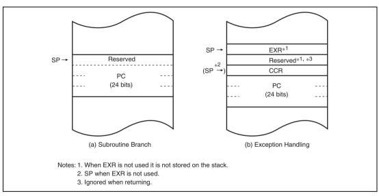
Figure 2.4 Stack Structure in Advanced Mode
