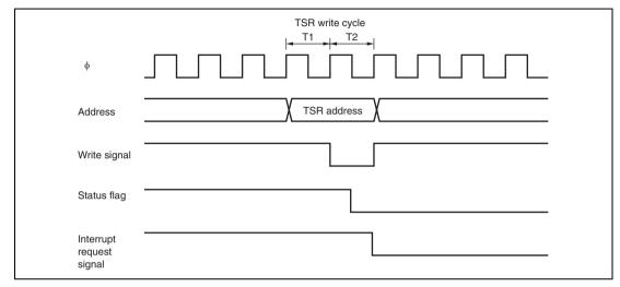
Figure 10.42 Timing for Status Flag Clearing by CPU
