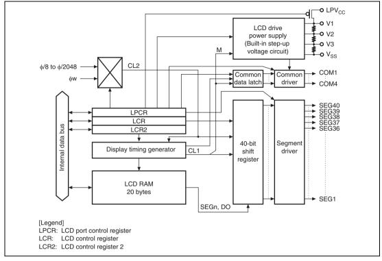
Figure 17.1 Block Diagram of LCD Controller/Driver
