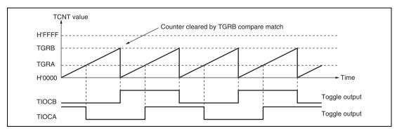
Figure 10.7 Example of Toggle Output Operation
