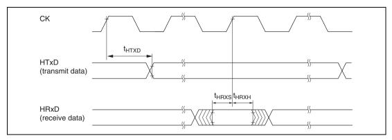
Figure 23.19 HCAN Input/Output Timing
