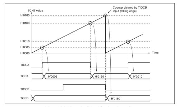
Figure 10.9 Example of Input Capture Operation
