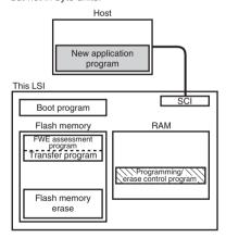
Programming/erase control program transfer When user program mode is entered, user software confirms this fact, executes transfer program in the flash memory, and transfers the programming/erase control program to RAM.
