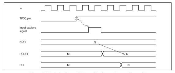
Figure 11.11 Pulse Output Triggered by Input Capture (Example)
