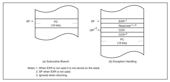
Figure 2.2 Stack Structure in Normal Mode
