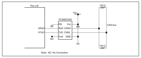
Figure 14.16 High-Speed Interface Using PCA82C250
