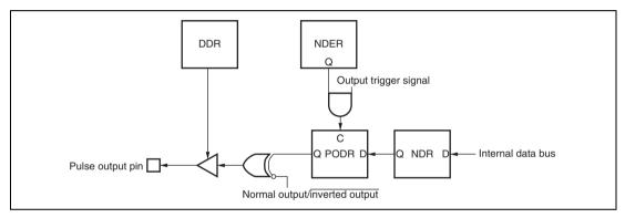
Figure 11.2 PPG Output Operation
