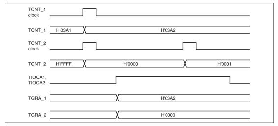
Figure 10.18 Example of Cascaded Operation (1)
