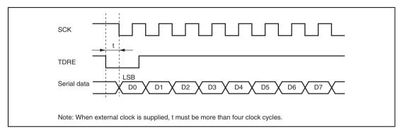
Figure 13.33 Sample Transmission using DTC in Clocked Synchronous Mode
