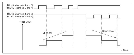
Figure 10.27 Example of Phase Counting Mode 3 Operation
