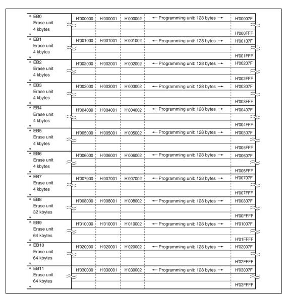
Figure 19.5 Flash Memory Block Configuration
