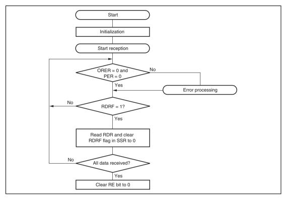
Figure 13.30 Example of Reception Processing Flow
