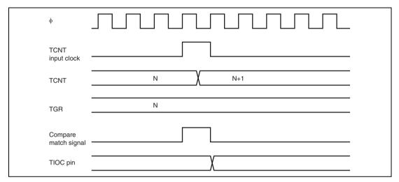
Figure 10.32 Output Compare Output Timing
