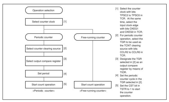
Figure 10.2 Example of Counter Operation Setting Procedure
