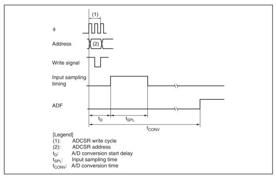
Figure 15.2 A/D Conversion Timing
