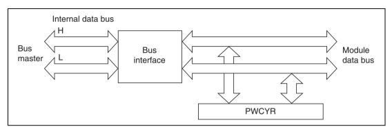
Figure 16.5 16-Bit Register Access Operation (Bus Master ↔ PWCYR (16 Bits))
