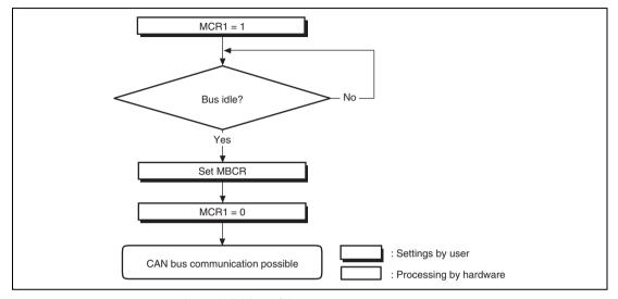
Figure 14.14 HCAN Halt Mode Flowchart
