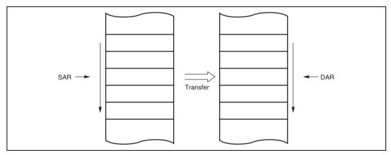
Figure 8.5 Memory Mapping in Normal Mode
