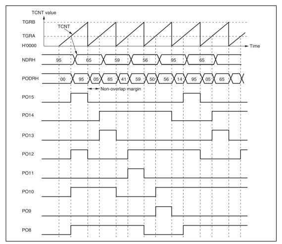
Figure 11.9 Non-Overlapping Pulse Output Example (Four-Phase Complementary)
