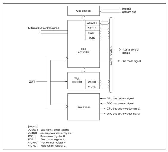
Figure 7.1 Block Diagram of Bus Controller
