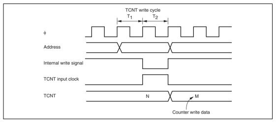
Figure 12.5 Contention between TCNT Write and Increment
