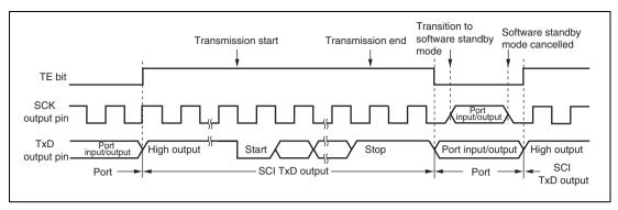
Figure 13.35 Pin States during Transmission in Asynchronous Mode (Internal Clock)
