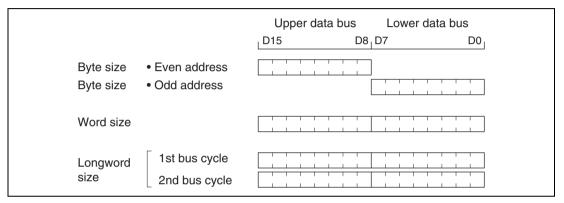
Figure 7.4 Access Sizes and Data Alignment Control (16-bit Access Space)
