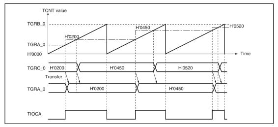
Figure 10.15 Example of Buffer Operation (1)
