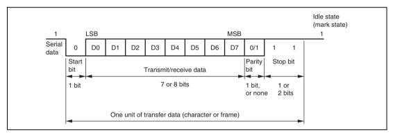
Figure 13.2 Data Format in Asynchronous Communication (Example with 8-Bit Data, Parity, Two Stop Bits)
