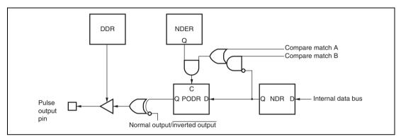
Figure 11.6 Non-Overlapping Pulse Output
