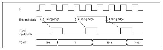
Figure 10.31 Count Timing in External Clock Operation
