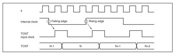
Figure 10.30 Count Timing in Internal Clock Operation
