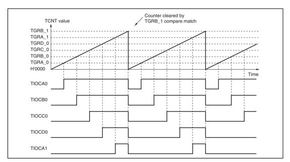
Figure 10.22 Example of PWM Mode Operation (2)
