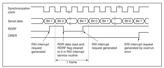
Figure 13.18 Example of SCI Operation in Reception
