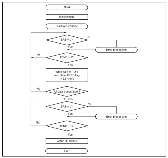
Figure 13.28 Example of Transmission Processing Flow
