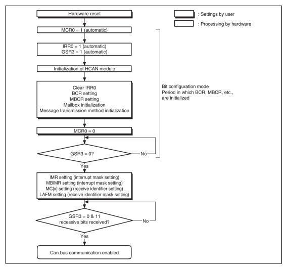
Figure 14.6 Hardware Reset Flowchart
