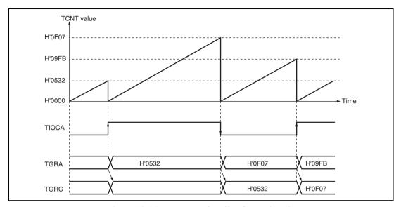
Figure 10.16 Example of Buffer Operation (2)
