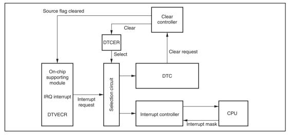
Figure 8.2 Block Diagram of DTC Activation Source Control
