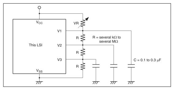
Figure 17.9 Connection of External Split-Resistance
