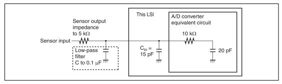
Figure 15.6 Example of Analog Input Circuit
