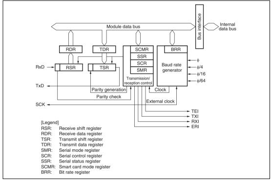
Figure 13.1 Block Diagram of SCI
