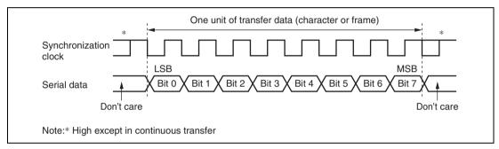
Figure 13.14 Data Format in Synchronous Communication (For LSB-First)
