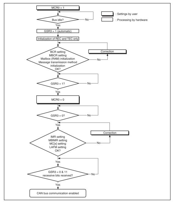
Figure 14.7 Software Reset Flowchart
