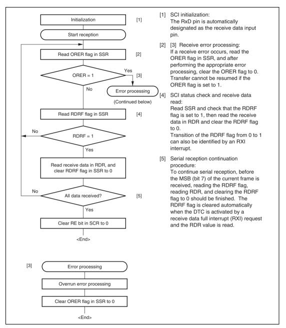
Figure 13.19 Sample Serial Reception Flowchart
