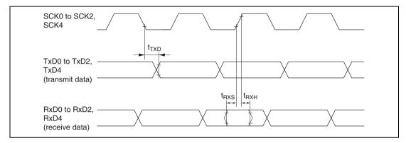
Figure 23.17 SCI Input/Output Timing (Clock Synchronous Mode)
