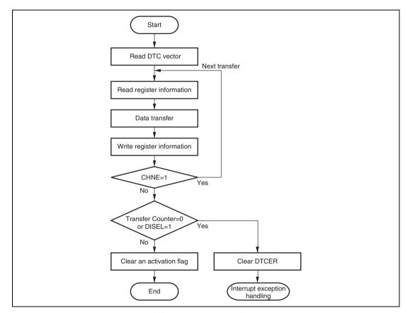
Figure 8.4 Flowchart of DTC Operation
