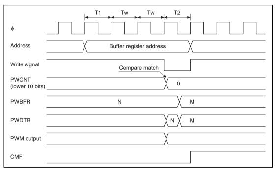
Figure 16.9 Conflict between Buffer Register Write and Compare Match
