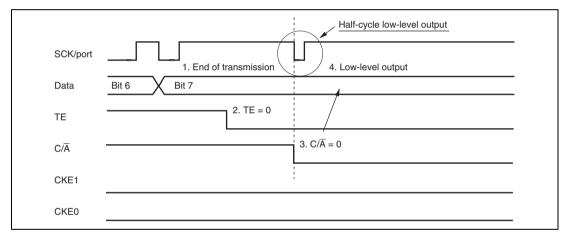
Figure 13.38 Operation when Switching from SCK Pin to Port Pin
