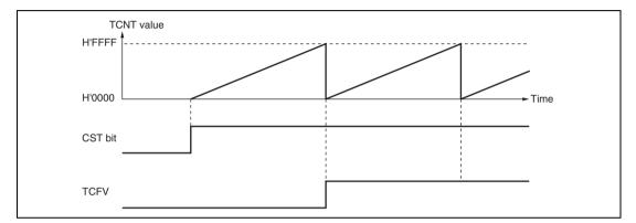
Figure 10.3 Free-Running Counter Operation
