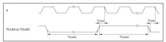
Figure 23.14 TPU Clock Input Timing
