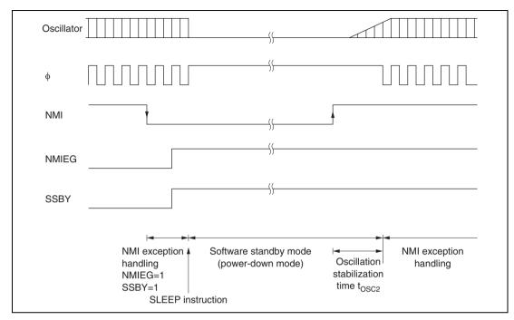
Figure 21.3 Software Standby Mode Application Example
