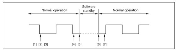
Figure 13.32 Clock Halt and Restart Procedure
