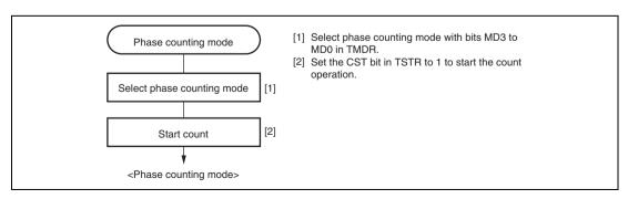
Figure 10.24 Example of Phase Counting Mode Setting Procedure
