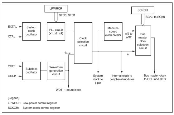
Figure 20.1 Block Diagram of Clock Pulse Generator
