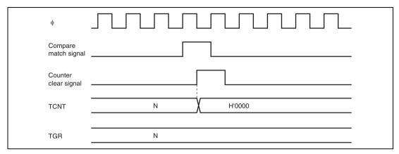
Figure 10.34 Counter Clear Timing (Compare Match)
