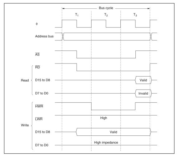
Figure 7.6 Bus Timing for 8-Bit, 3-State Access Space
