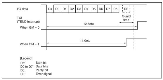
Figure 13.27 TEND Flag Generation Timing in Transmission Operation
