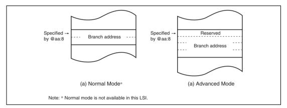
Figure 2.12 Branch Address Specification in Memory Indirect Mode
