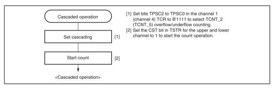
Figure 10.17 Cascaded Operation Setting Procedure
