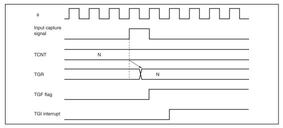
Figure 10.39 TGI Interrupt Timing (Input Capture)
