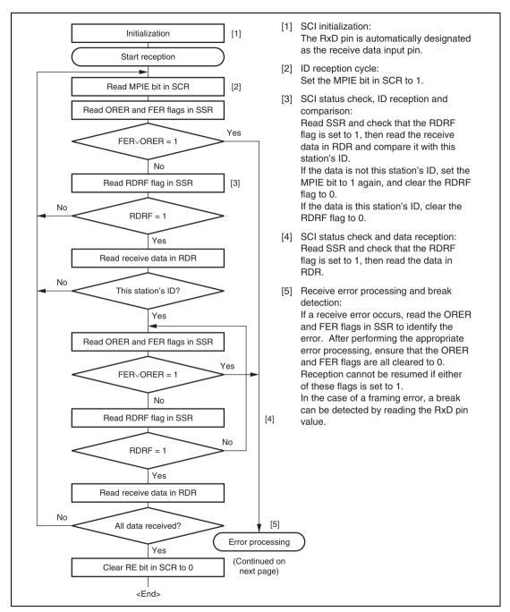
Figure 13.13 Sample Multiprocessor Serial Reception Flowchart (1)
