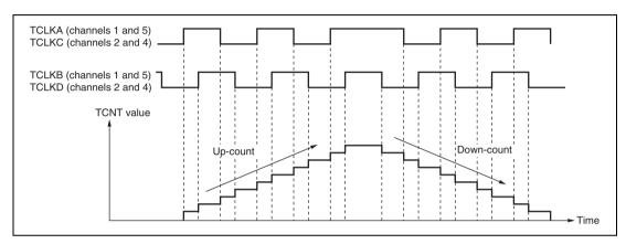
Figure 10.25 Example of Phase Counting Mode 1 Operation
