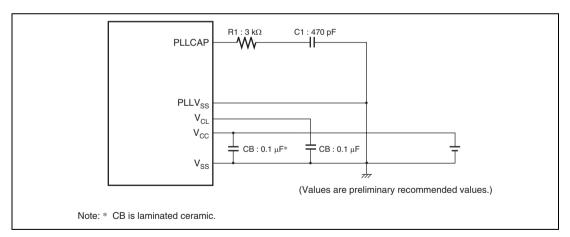
Figure 20.10 External Circuitry Recommended for PLL Circuit
