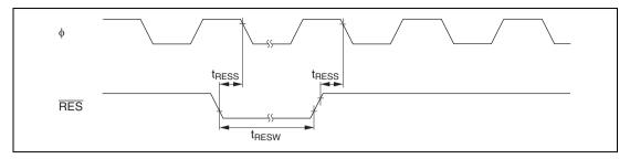
Figure 23.4 Reset Input Timing
