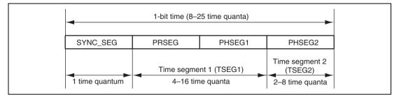
Figure 14.8 Detailed Description of One-Bit Time
