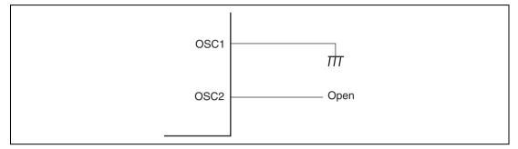
Figure 20.8 Pin Handling when Subclock is not Used
