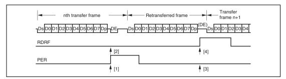
Figure 13.29 Retransfer Operation in SCI Receive Mode
