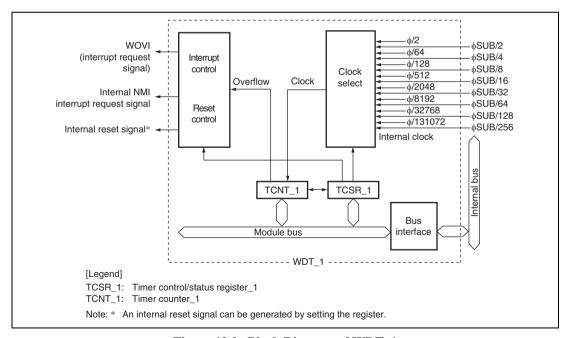
Figure 12.2 Block Diagram of WDT\_1
