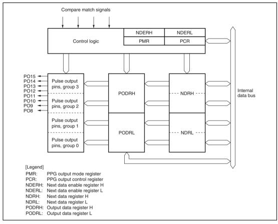
Figure 11.1 Block Diagram of PPG
