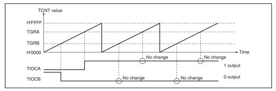
Figure 10.6 Example of 0 Output/1 Output Operation
