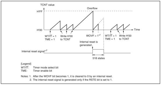
Figure 12.3 (a) WDT\_0 Operation in Watchdog Timer Mode
