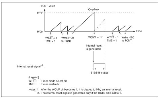
Figure 12.3 (b) WDT\_1 Operation in Watchdog Timer Mode
