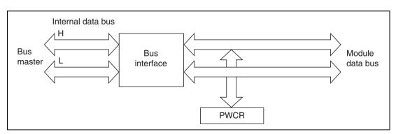
Figure 16.6 8-Bit Register Access Operation (Bus Master ↔ PWCR (Upper Eight Bits))
