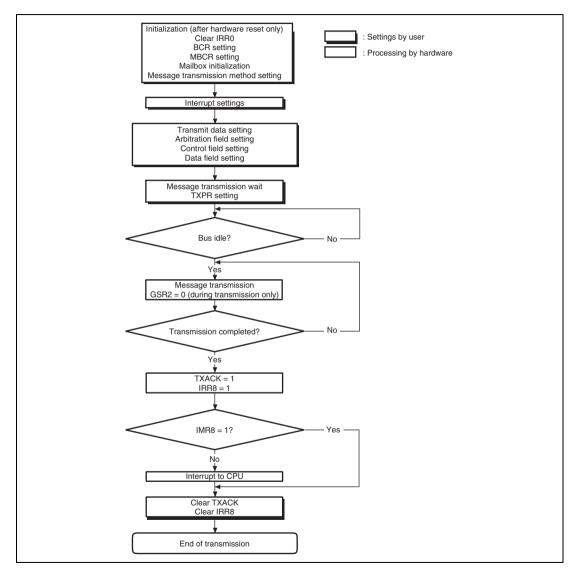
Figure 14.9 Transmission Flowchart
