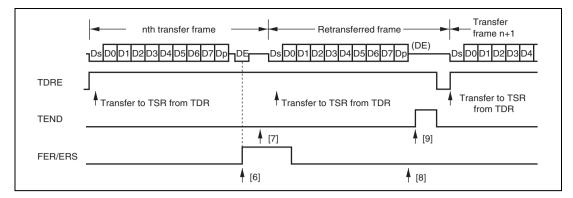
Figure 13.26 Retransfer Operation in SCI Transmit Mode
