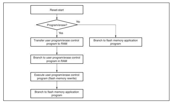
Figure 19.6 Programming/Erasing Flowchart Example in User Program Mode
