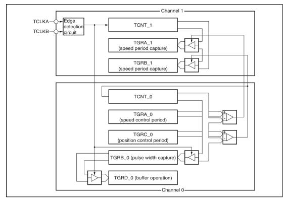
Figure 10.29 Phase Counting Mode Application Example
