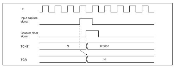
Figure 10.35 Counter Clear Timing (Input Capture)
