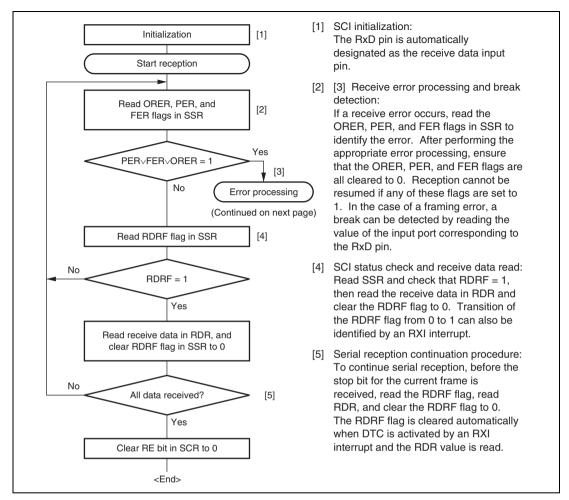
Figure 13.9 Sample Serial Reception Data Flowchart (1)
