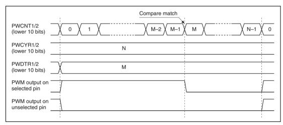
Figure 16.3 Duty Register Compare Match (OPS = 0 in PWPR)
