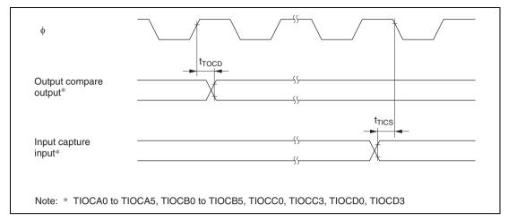
Figure 23.13 TPU Input/Output Timing
