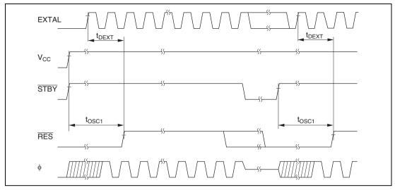
Figure 23.3 Oscillator Settling Timing
