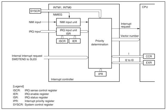
Figure 5.1 Block Diagram of Interrupt Controller
