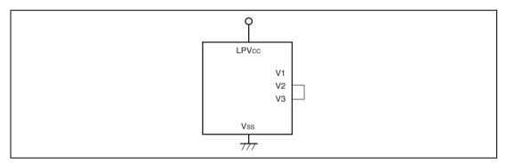
Figure 17.2 Handling of LCD Drive Power Supply when Using 1/2 Duty
