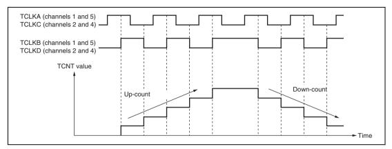
Figure 10.28 Example of Phase Counting Mode 4 Operation
