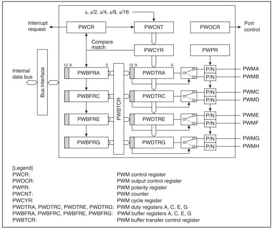
Figure 16.1 Block Diagram of PWM
