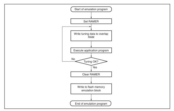
Figure 19.7 Flowchart for Flash Memory Emulation in RAM
