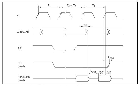
Figure 23.10 Burst ROM Access Timing (Two-State Access)
