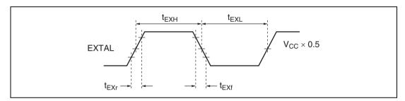
Figure 20.5 External Clock Input Timing
