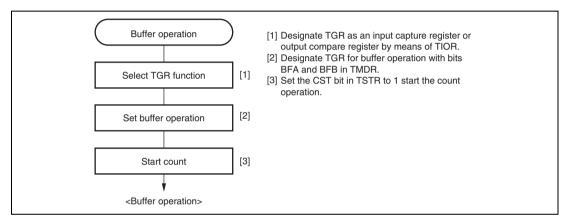
Figure 10.14 Example of Buffer Operation Setting Procedure
