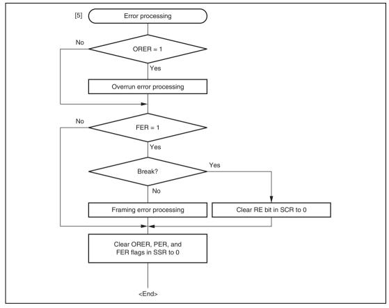
Figure 13.13 Sample Multiprocessor Serial Reception Flowchart (2)
