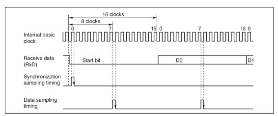
Figure 13.3 Receive Data Sampling Timing in Asynchronous Mode
