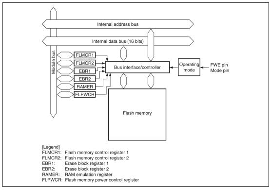
Figure 19.1 Block Diagram of Flash Memory
