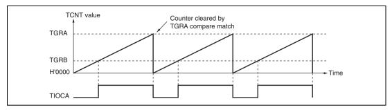
Figure 10.21 Example of PWM Mode Operation (1)
