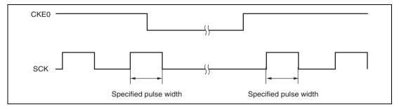
Figure 13.31 Timing for Fixing Clock Output Level
