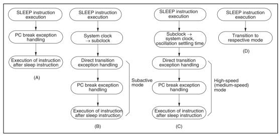
Figure 6.2 Operation in Power-Down Mode Transitions
