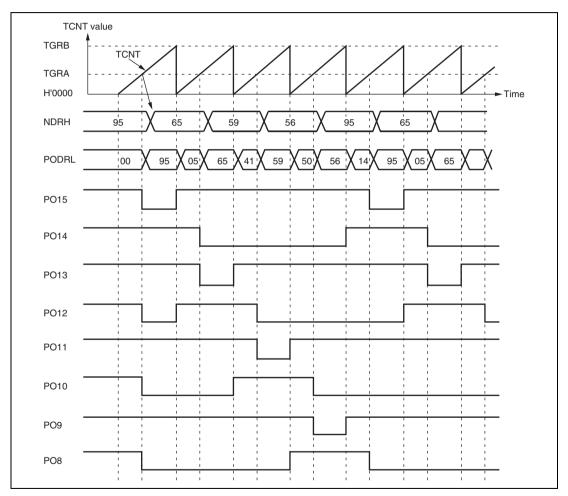
Figure 11.10 Inverted Pulse Output (Example)
