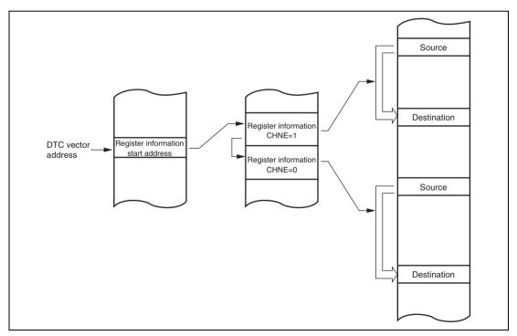
Figure 8.8 Chain Transfer Operation
