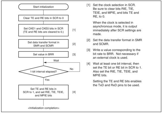
Figure 13.5 Sample SCI Initialization Flowchart
