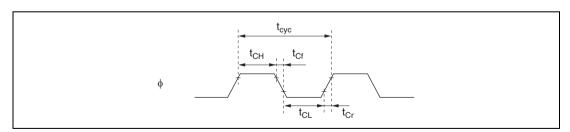
Figure 23.2 System Clock Timing
