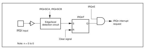
Figure 5.2 Block Diagram of Interrupts IRQ0 to IRQ5
