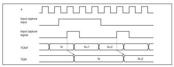
Figure 10.33 Input Capture Input Signal Timing
