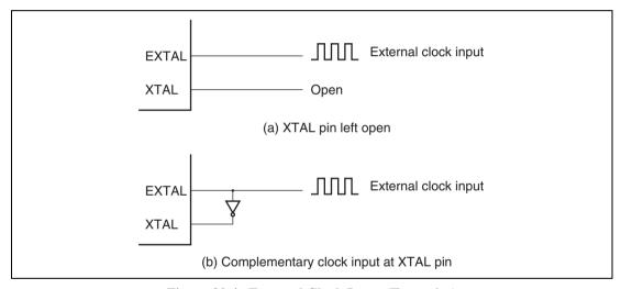
Figure 20.4 External Clock Input (Examples)
