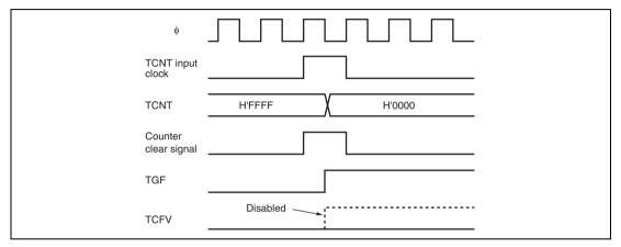
Figure 10.52 Conflict between Overflow and Counter Clearing
