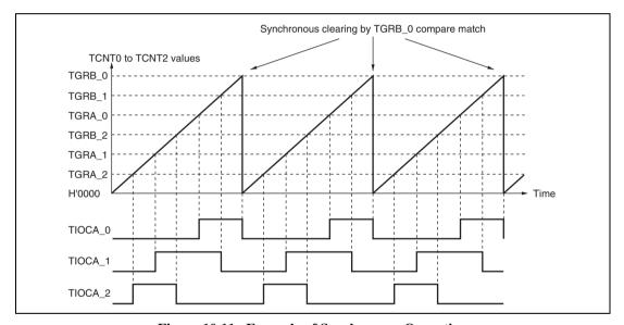
Figure 10.11 Example of Synchronous Operation
