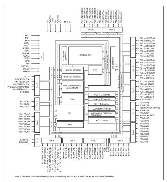
Figure 1.1 Internal Block Diagram
