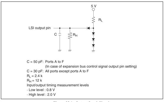
Figure 23.1 Output Load Circuit
