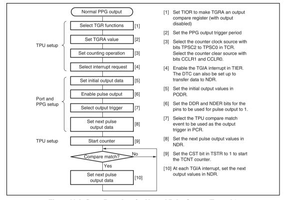
Figure 11.4 Setup Procedure for Normal Pulse Output (Example)
