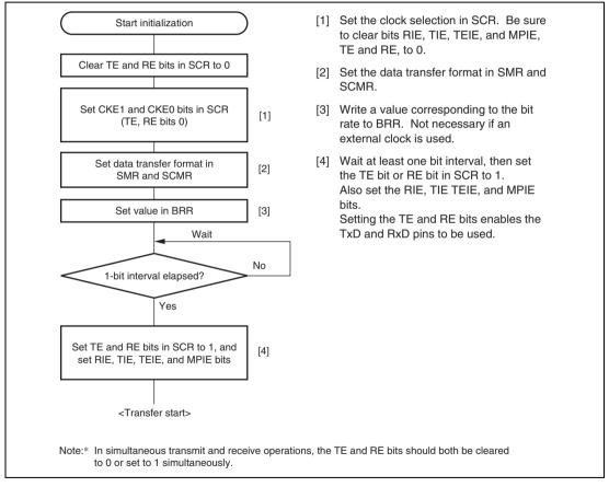
Figure 13.15 Sample SCI Initialization Flowchart
