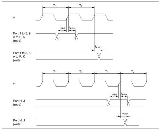
Figure 23.11 I/O Port Input/Output Timing
