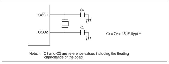
Figure 20.6 Connection Example of 32.768-kHz Crystal Resonator
