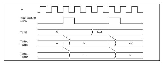
Figure 10.37 Buffer Operation Timing (Input Capture)
