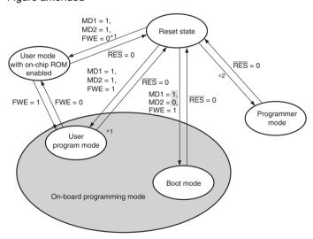
Notes: Only make a transition between user mode and user program mode when the CPU is not accessing the flash memory.
