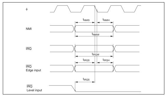
Figure 23.5 Interrupt Input Timing
