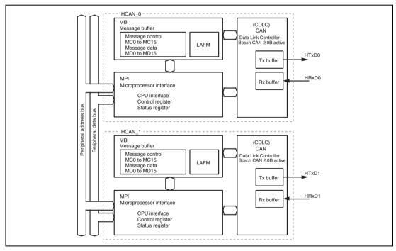
Figure 14.1 HCAN Block Diagram
