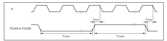
Figure 20.8 TPU Clock Input Timing
