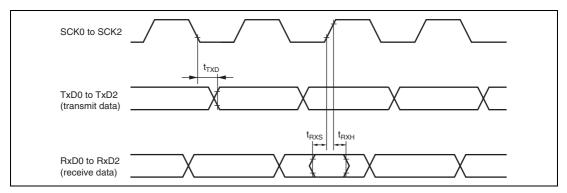
Figure 20.10 SCI Input/Output Timing (Clock Synchronous Mode)
