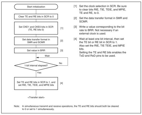
Figure 13.15 Sample SCI Initialization Flowchart
