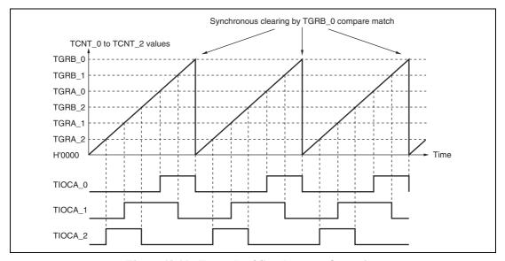
Figure 10.11 Example of Synchronous Operation
