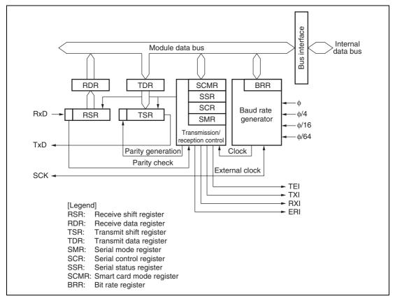
Figure 13.1 Block Diagram of SCI
