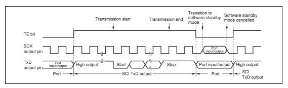
Figure 13.35 Pin States during Transmission in Asynchronous Mode (Internal Clock)
