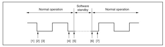
Figure 13.32 Clock Halt and Restart Procedure
