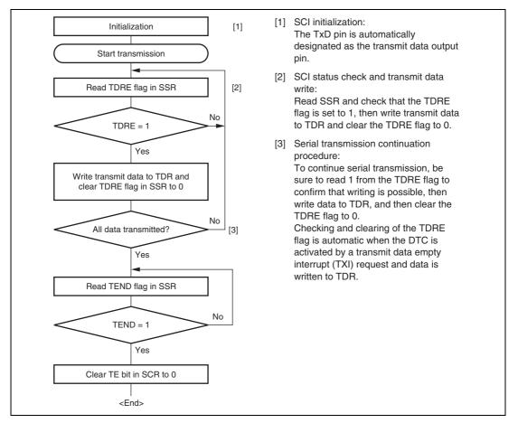
Figure 13.17 Sample Serial Transmission Flowchart
