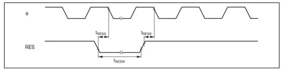
Figure 20.4 Reset Input Timing
