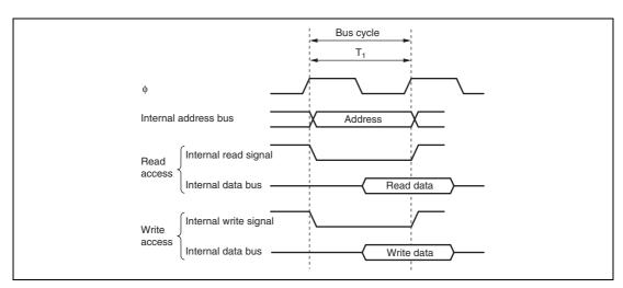
Figure 7.1 On-Chip Memory Access Cycle
