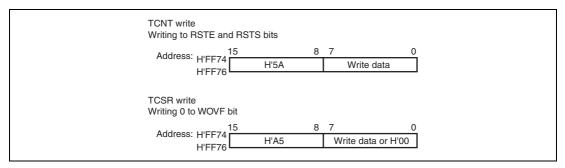
Figure 12.2 Writing to TCNT, TCSR, and RSTCSR (Example for WDT0)
