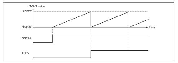
Figure 10.3 Free-Running Counter Operation
