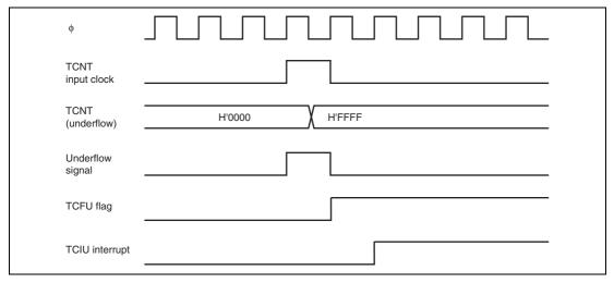
Figure 10.41 TCIU Interrupt Setting Timing
