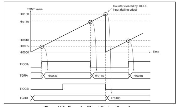
Figure 10.9 Example of Input Capture Operation
