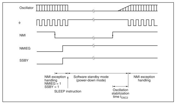
Figure 18.3 Software Standby Mode Application Example
