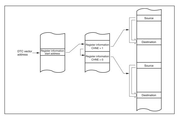
Figure 8.8 Chain Transfer Operation
