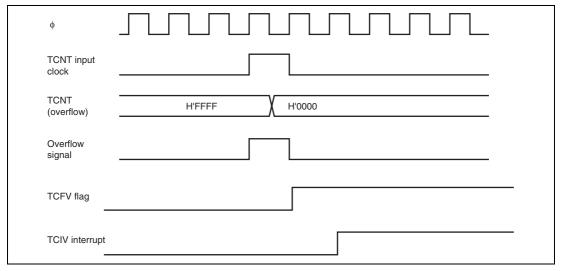
Figure 10.40 TCIV Interrupt Setting Timing
