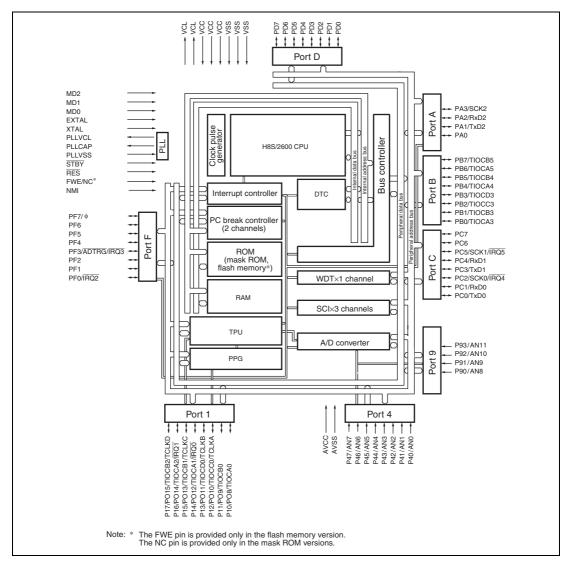
Figure 1.1 Block Diagram
