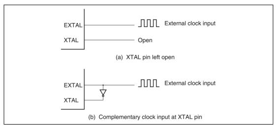
Figure 17.4 External Clock Input (Examples)
