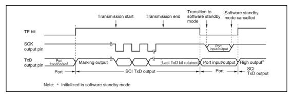
Figure 13.36 Pin States during Transmission in Clocked Synchronous Mode (Internal Clock)
