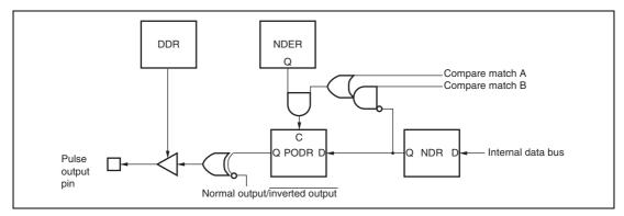
Figure 11.6 Non-Overlapping Pulse Output
