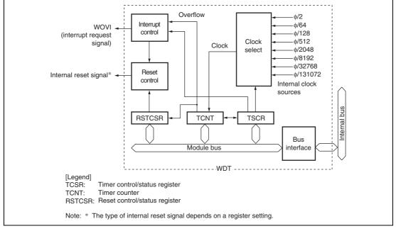
Figure 12.1 Block Diagram of WDT
