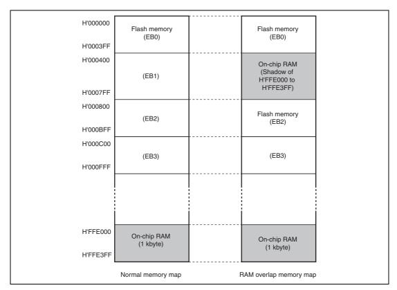
Figure 16.8 Example of RAM Overlap Operation
