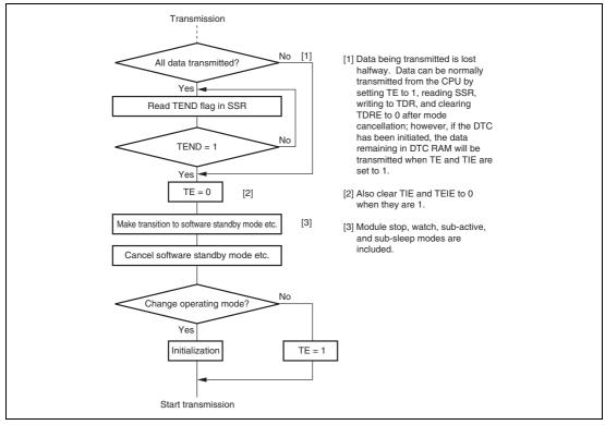
Figure 13.34 Sample Flowchart for Mode Transition during Transmission
