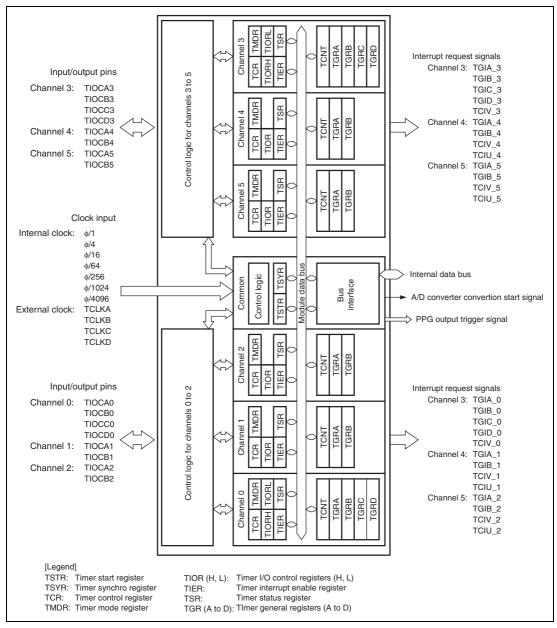
Figure 10.1 Block Diagram of TPU
