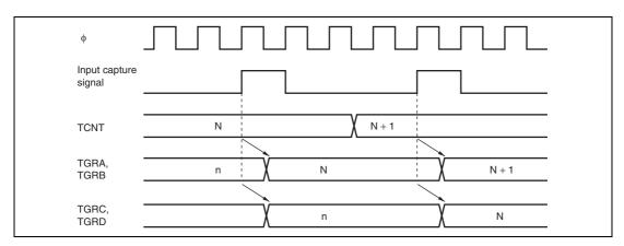
**Figure 10.37 Buffer Operation Timing (Input Capture)**
