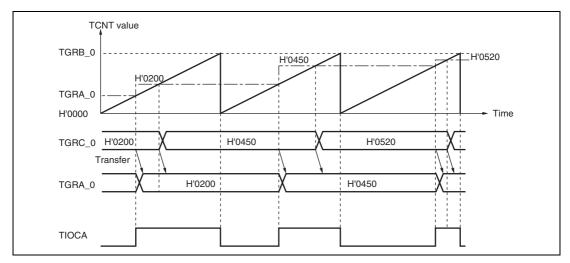
Figure 10.15 Example of Buffer Operation (1)
