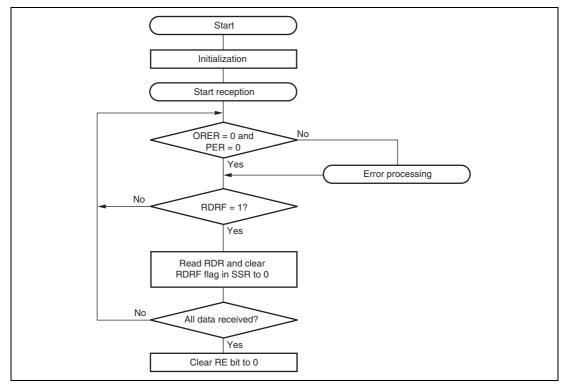
Figure 13.30 Example of Reception Processing Flow
