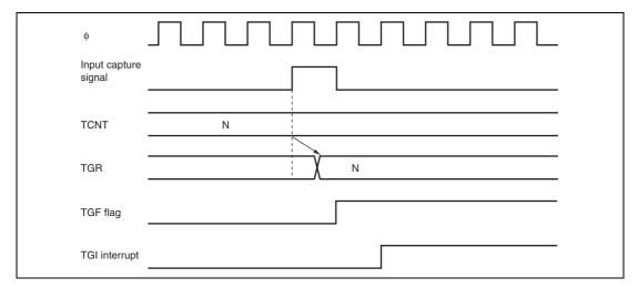
Figure 10.39 TGI Interrupt Timing (Input Capture)
