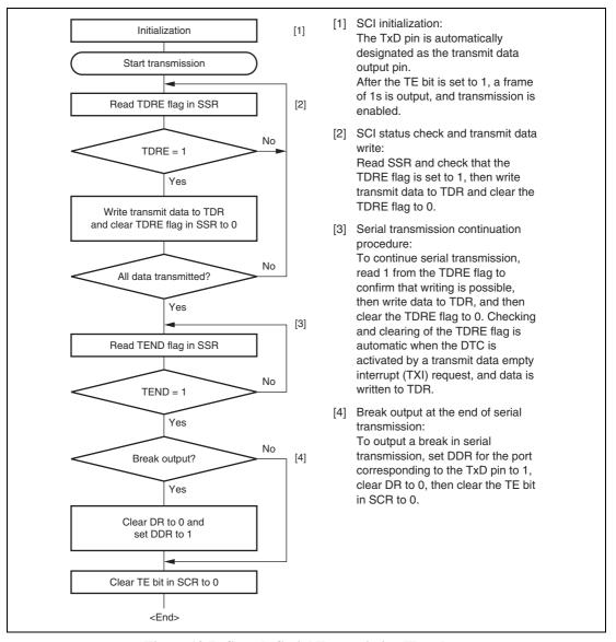
Figure 13.7 Sample Serial Transmission Flowchart
