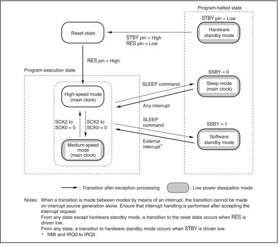
Figure 18.1 Mode Transition Diagram
