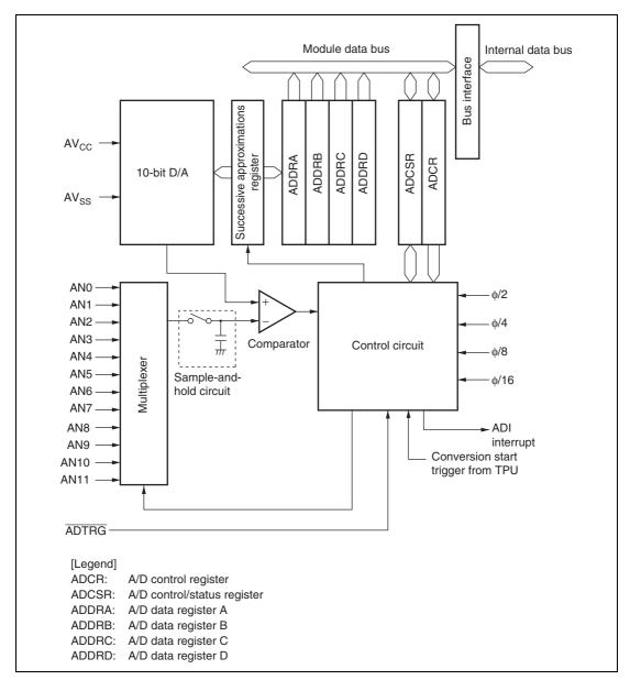
Figure 14.1 Block Diagram of A/D Converter
