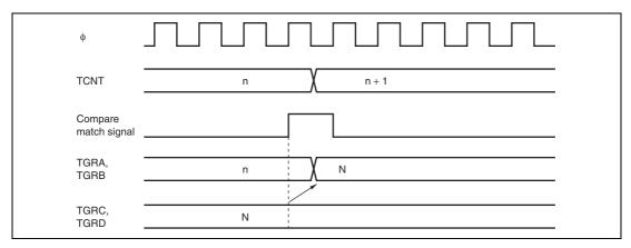
**Figure 10.36 Buffer Operation Timing (Compare Match)**
