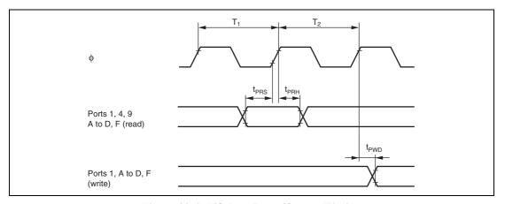
Figure 20.6 I/O Port Input/Output Timing
