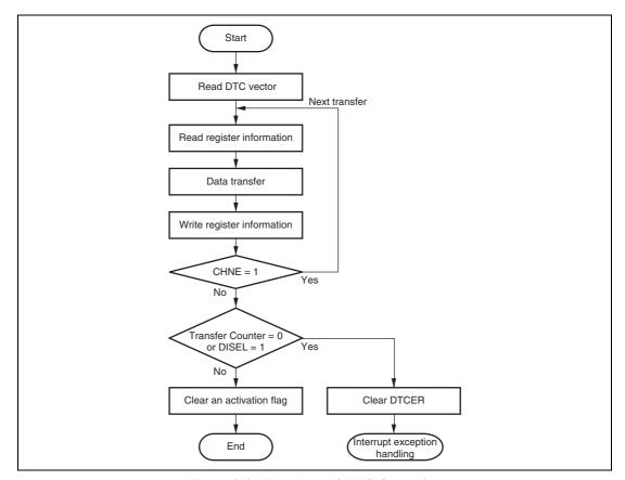
Figure 8.4 Flowchart of DTC Operation
