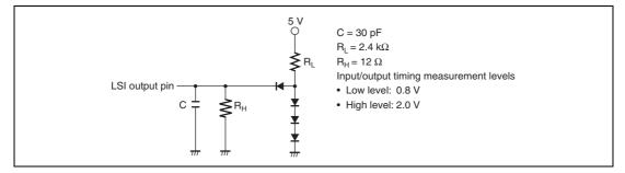
Figure 20.1 Output Load Circuit
