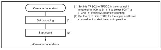
Figure 10.17 Cascaded Operation Setting Procedure
