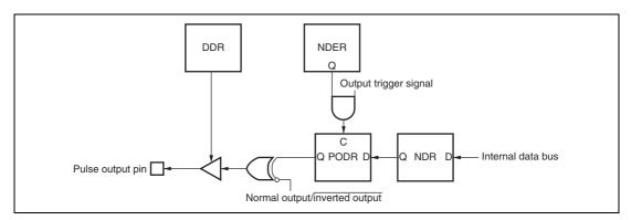
Figure 11.2 PPG Output Operation
