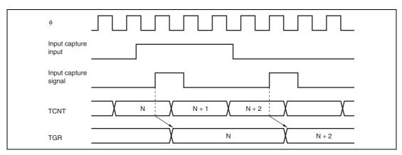
Figure 10.33 Input Capture Input Signal Timing
