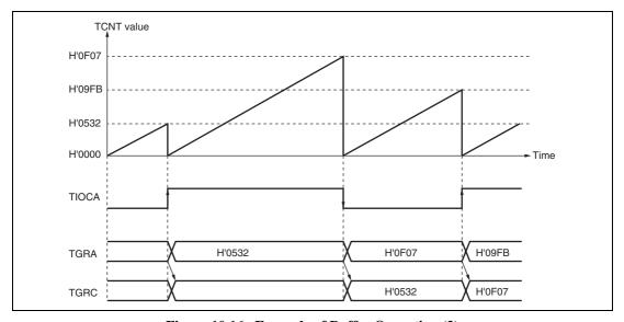
Figure 10.16 Example of Buffer Operation (2)
