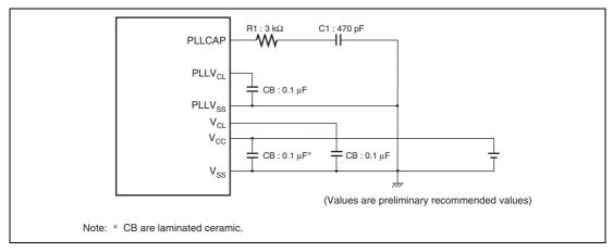
Figure 17.7 External Circuitry Recommended for PLL Circuit
