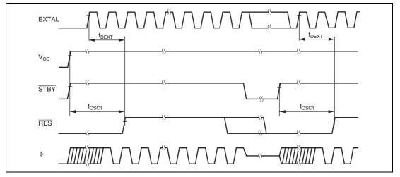
Figure 20.3 Oscillation Stabilization Timing
