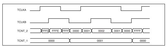
Figure 10.19 Example of Cascaded Operation (2)
