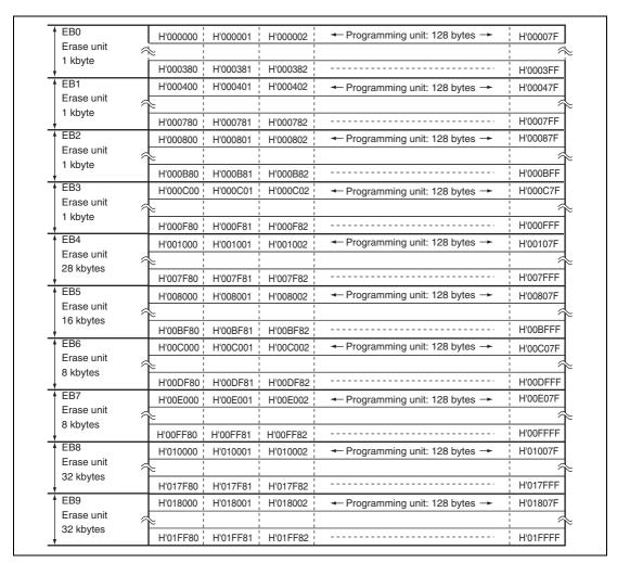
Figure 16.5 Flash Memory Block Configuration
