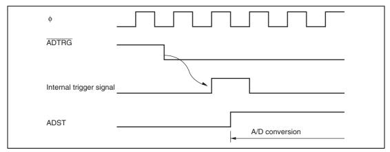
Figure 14.3 External Trigger Input Timing
