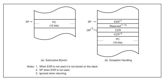
Figure 2.2 Stack Structure in Normal Mode
