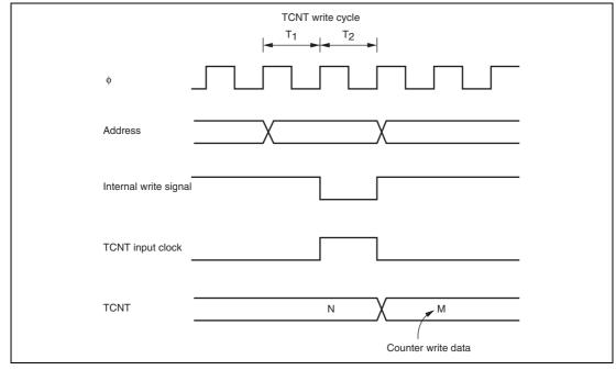
Figure 12.3 Contention between TCNT Write and Increment
