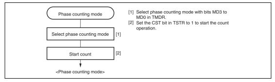
Figure 10.24 Example of Phase Counting Mode Setting Procedure
