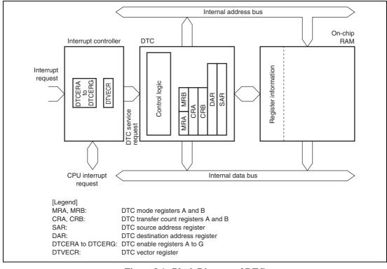
Figure 8.1 Block Diagram of DTC
