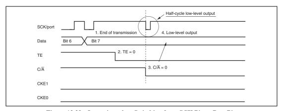
Figure 13.38 Operation when Switching from SCK Pin to Port Pin
