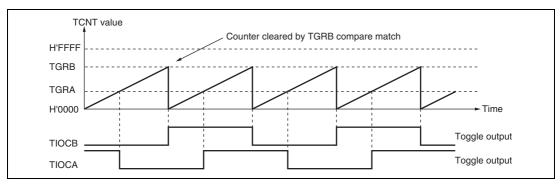
Figure 10.7 Example of Toggle Output Operation
