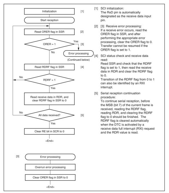
Figure 13.19 Sample Serial Reception Flowchart
