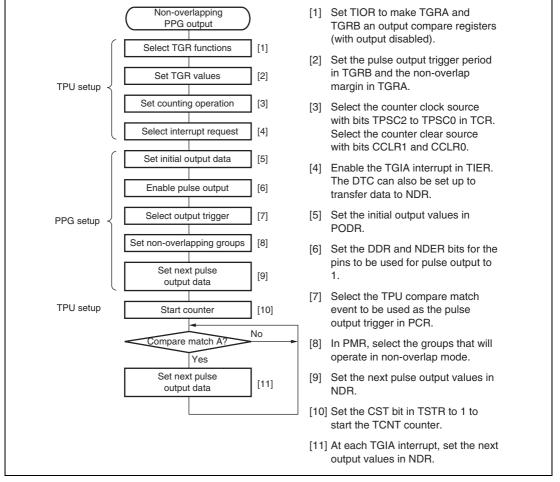
Figure 11.8 Setup Procedure for Non-Overlapping Pulse Output (Example)
