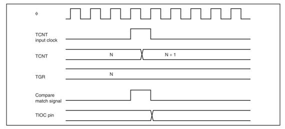
Figure 10.32 Output Compare Output Timing
