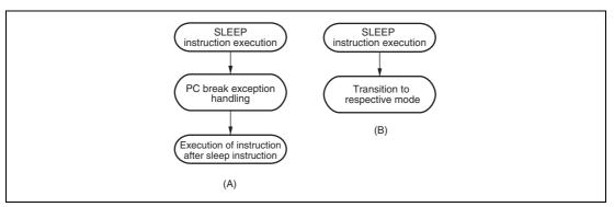
Figure 6.2 Operation in Power-Down Mode Transitions
