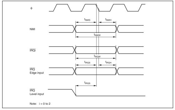
Figure 20.5 Interrupt Input Timing
