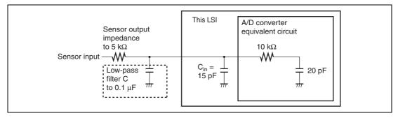
Figure 14.6 Example of Analog Input Circuit
