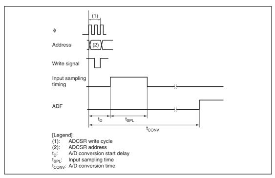
Figure 14.2 A/D Conversion Timing
