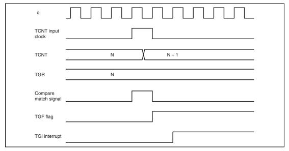
Figure 10.38 TGI Interrupt Timing (Compare Match)
