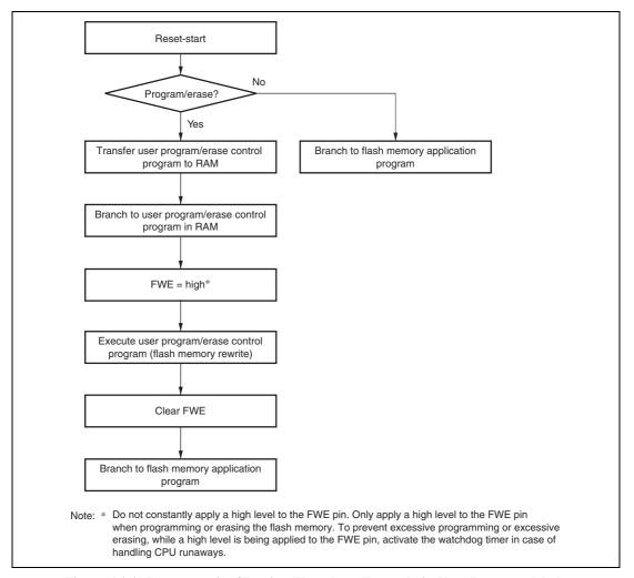
Figure 16.6 Programming/Erasing Flowchart Example in User Program Mode
