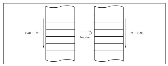
Figure 8.5 Memory Mapping in Normal Mode
