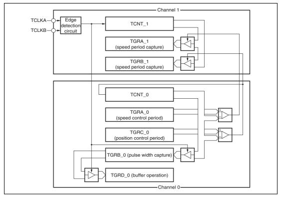
Figure 10.29 Phase Counting Mode Application Example
