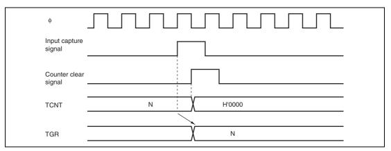
Figure 10.35 Counter Clear Timing (Input Capture)
