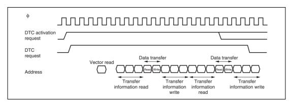
Figure 8.11 DTC Operation Timing (Example of Chain Transfer)
