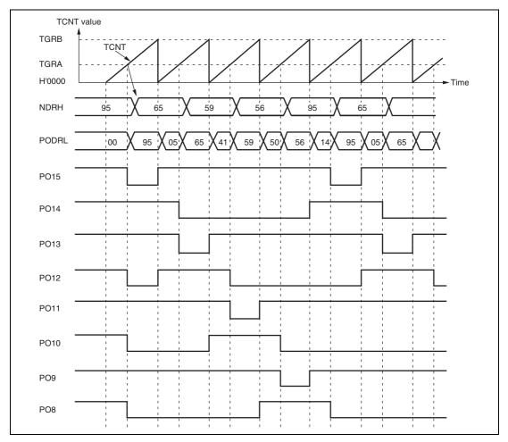
Figure 11.10 Inverted Pulse Output (Example)
