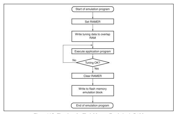
Figure 16.7 Flowchart for Flash Memory Emulation in RAM
