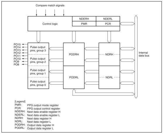
Figure 11.1 Block Diagram of PPG
