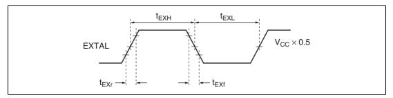
Figure 17.5 External Clock Input Timing
