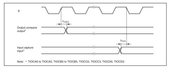
Figure 20.7 TPU Input/Output Timing
