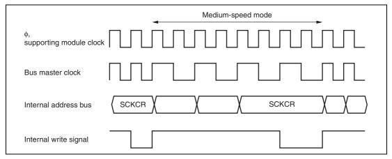
Figure 18.2 Medium-Speed Mode Transition and Clearance Timing
