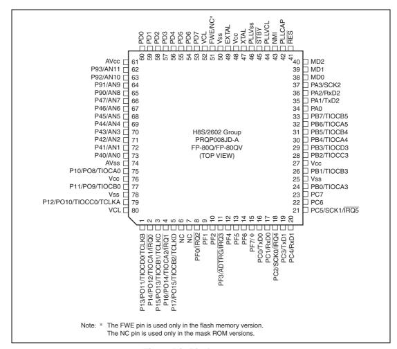
Figure 1.2 Pin Arrangement
