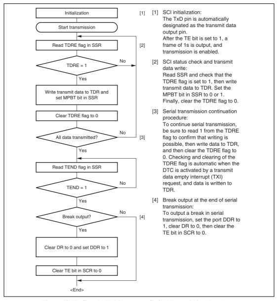
Figure 13.11 Sample Multiprocessor Serial Transmission Flowchart
