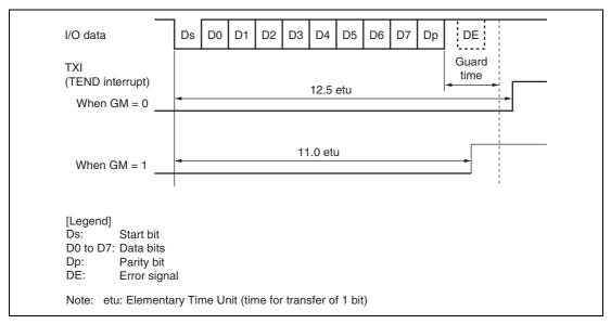
Figure 13.27 TEND Flag Generation Timing in Transmission Operation
