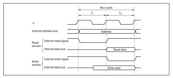
Figure 7.2 On-Chip Peripheral Module Access Cycle
