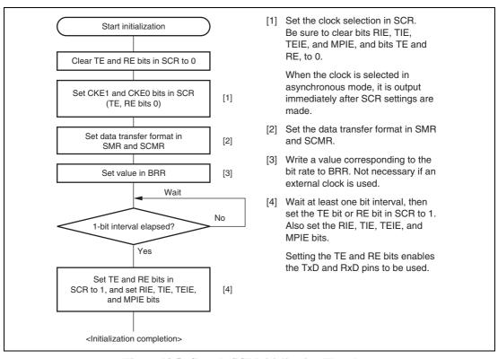
Figure 13.5 Sample SCI Initialization Flowchart
