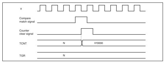
Figure 10.34 Counter Clear Timing (Compare Match)
