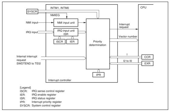
Figure 5.1 Block Diagram of Interrupt Controller
