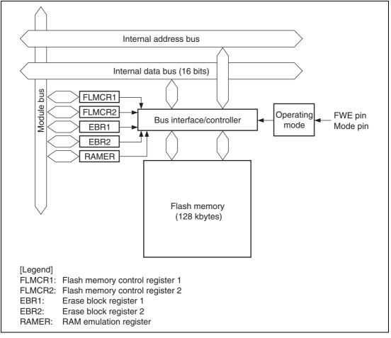
Figure 16.1 Block Diagram of Flash Memory
