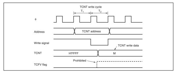
Figure 10.53 Contention between TCNT Write and Overflow
