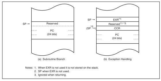
Figure 2.4 Stack Structure in Advanced Mode
