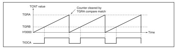
Figure 10.21 Example of PWM Mode Operation (1)
