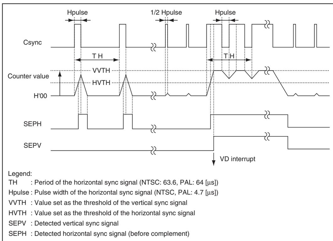
**Figure 26.73 Threshold Values and Separated Sync Signals**
