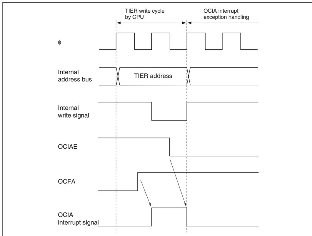
**Figure 6.9 Contention between Interrupt Generation and Disabling**
