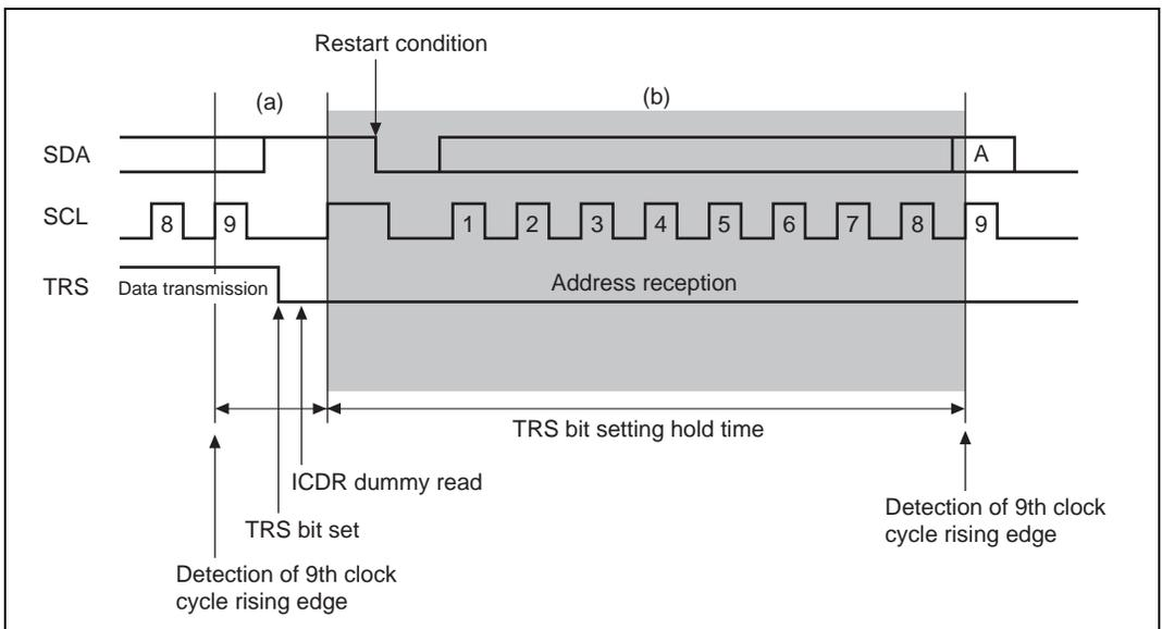
**Figure 23.23 TRS Bit Setting Timing in Slave Mode**
