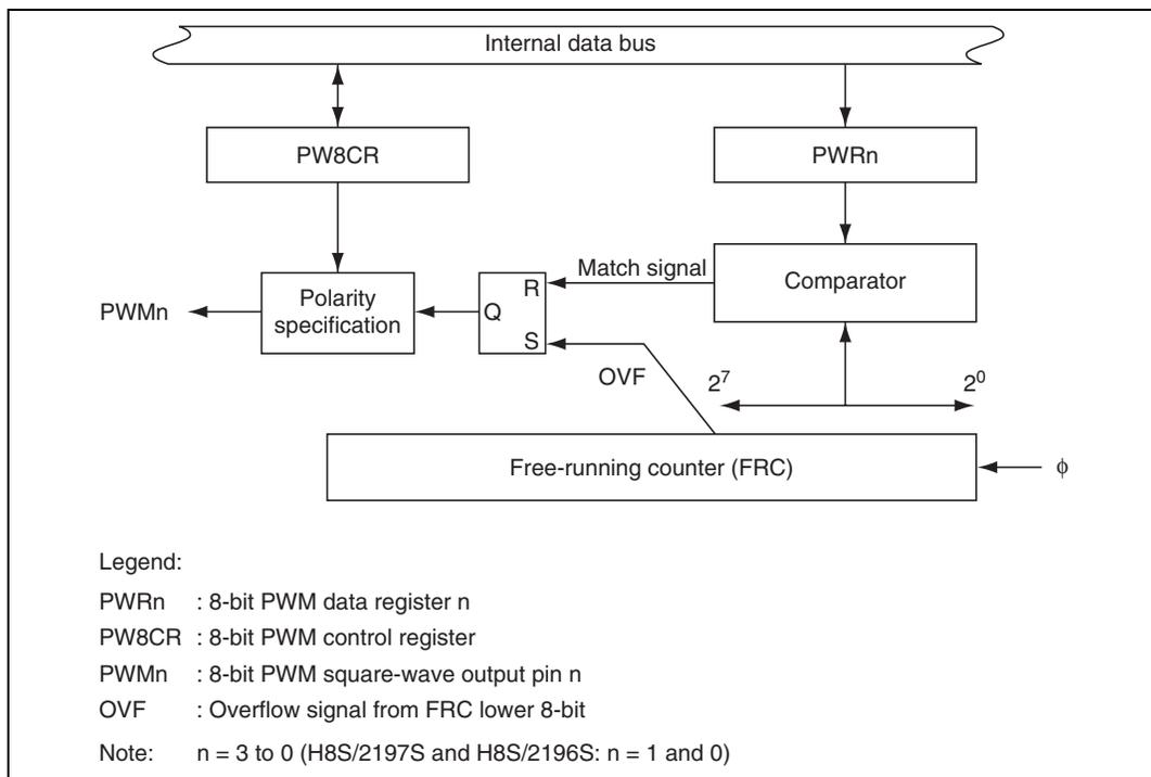
**Figure 18.1 Block Diagram of 8-Bit PWM (1 channel)**
