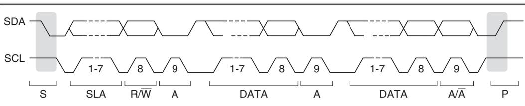
**Figure 23.5 I<sup>2</sup>C Bus Timing**
