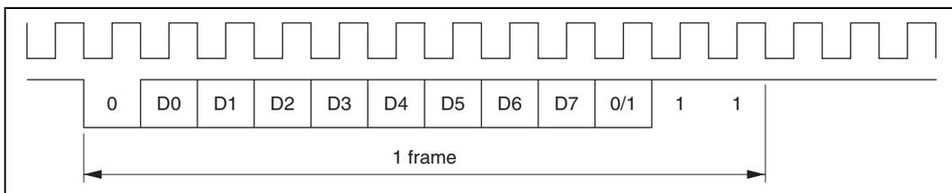
**Figure 22.3 Relation between Output Clock and Transfer Data Phase
