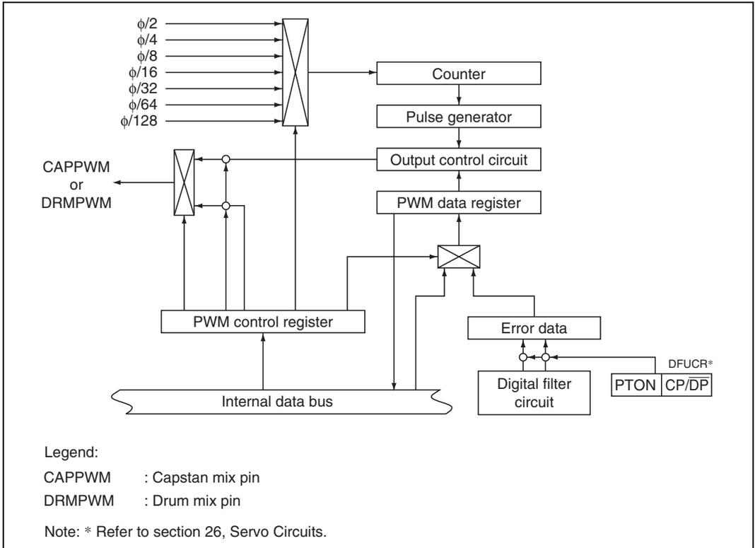
**Figure 19.1 Block Diagram of 12-Bit PWM (1 channel)**
