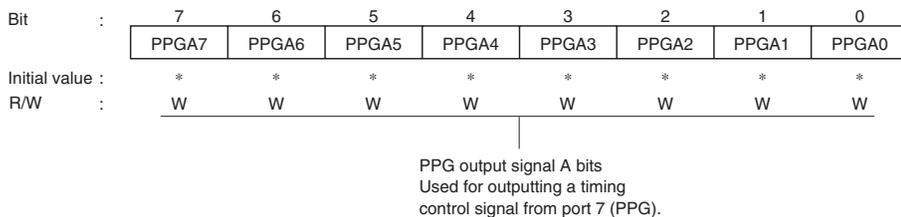
**H'D066 and H'D067: FIFO Timing Pattern Register 1 FTPRA\*: HSW Timing Generator**
