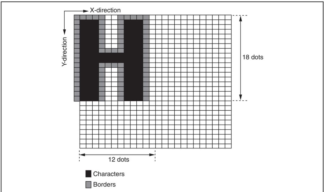
**Figure 29.16 Border Extending beyond the Display Frame (Example)**
