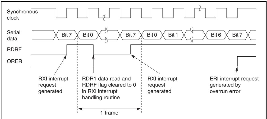
**Figure 22.21 Example of SCI Operation in Reception**
