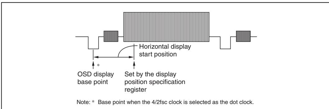
**Figure 29.11 Base Point for Horizontal Display Start Position**
