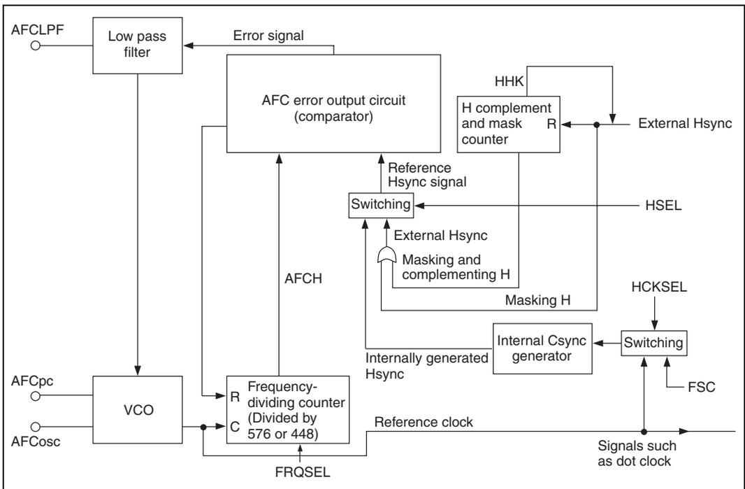
**Figure 27.22 AFC Configuration**
