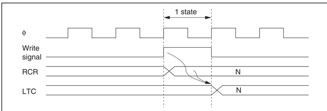
**Figure 14.4 Timing of Writing and Reloading of RCR**
