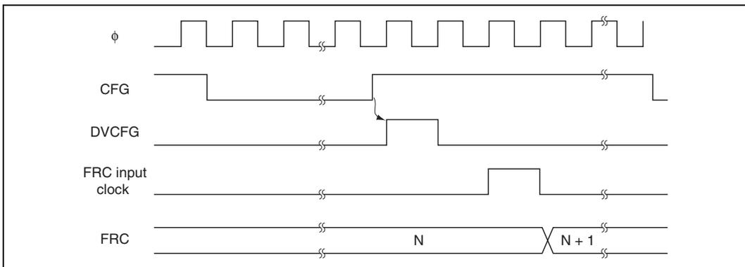
**Figure 16.4 Count Timing for CFG Clock Operation**
