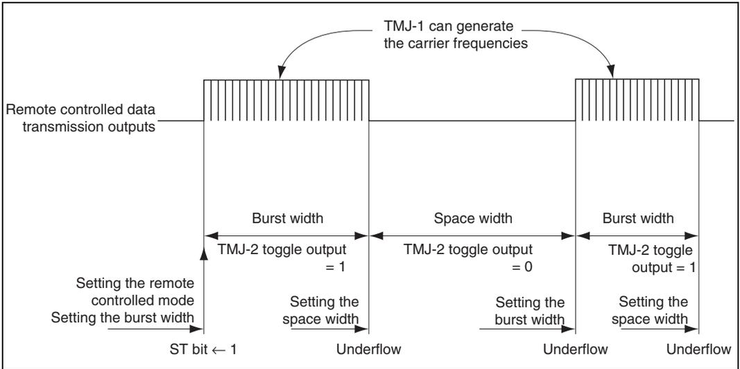
**Figure 13.2 Remote Controlled Data Transmission Output Waveform**
