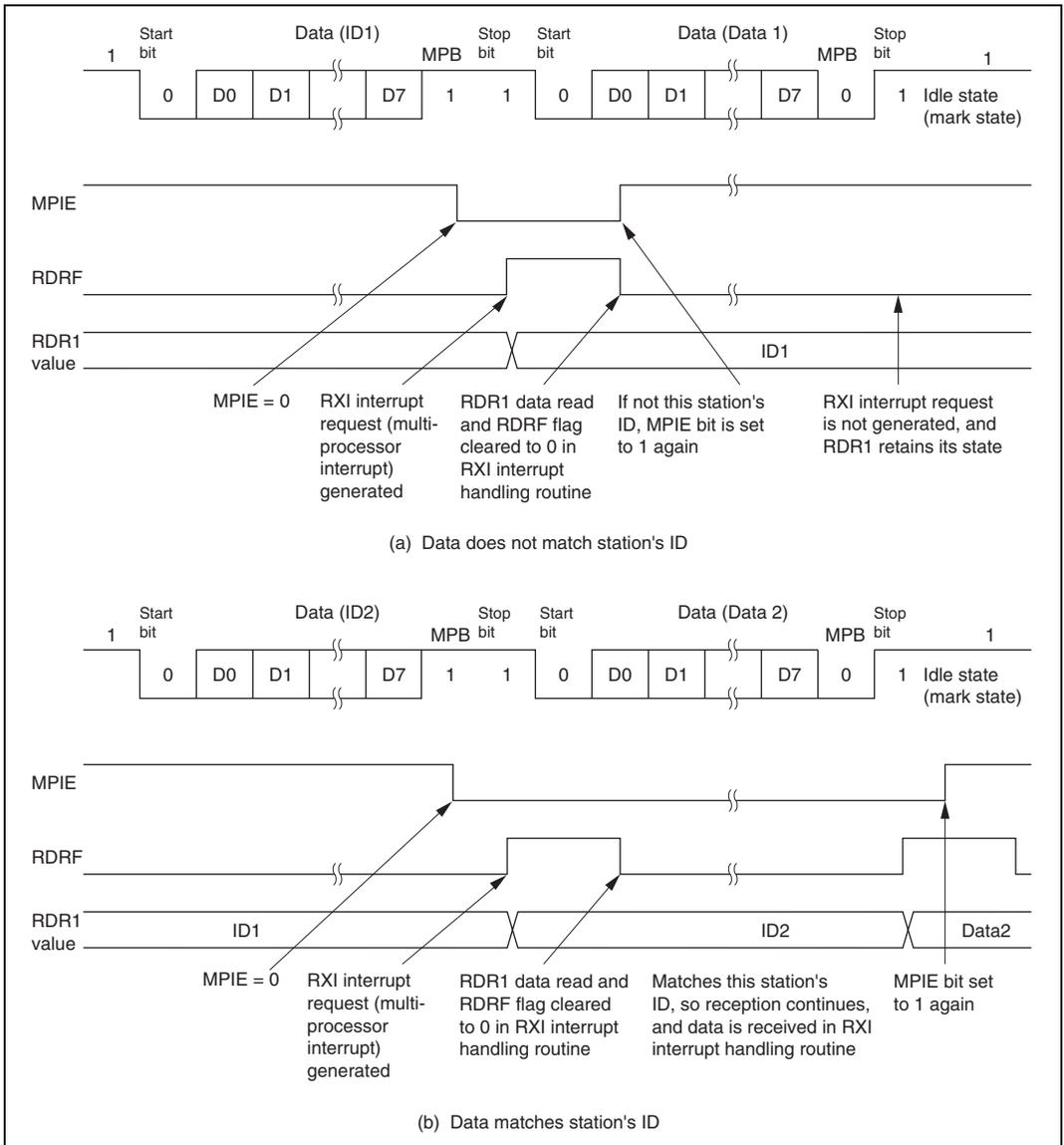
**Figure 22.15 Example of SCI Operation in Reception
