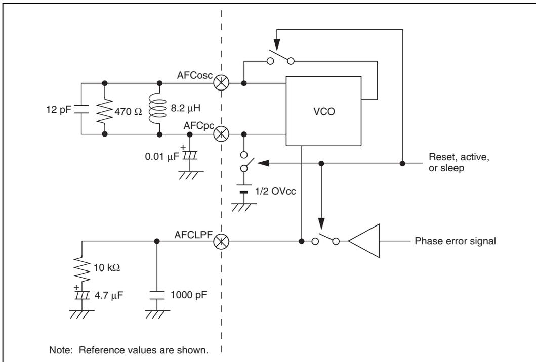
**Figure 27.23 Circuit Example for a 576 × fh Reference Clock**
