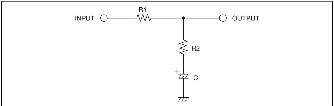
**Figure 26.40 Lag-Lead Filter**
