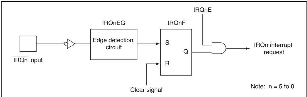
**Figure 6.2 Block Diagram of Interrupts IRQ5 to IRQ0**
