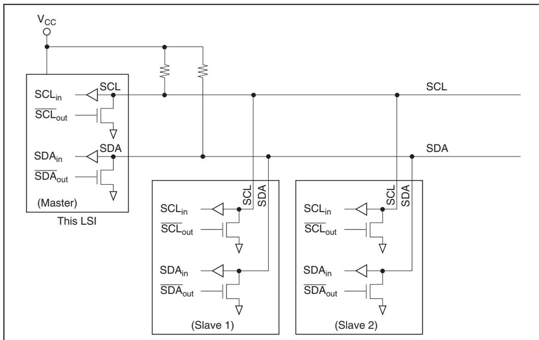
**Figure 23.2 I<sup>2</sup>C Bus Interface Connections (Example: This Chip as Master)**
