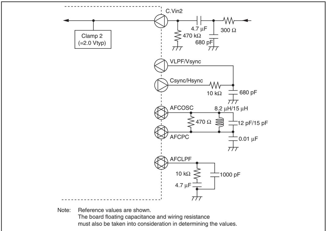
**Figure E.8 Example of External Circuit for Sync Separator and Data Slicer
