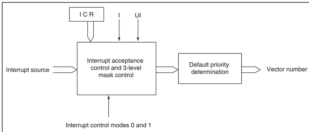
**Figure 6.4 Block Diagram of Interrupt Priority Determination Operation**
