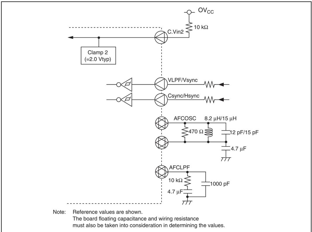
**Figure E.10 Example of External Circuit for Sync Separator and Data Slicer
