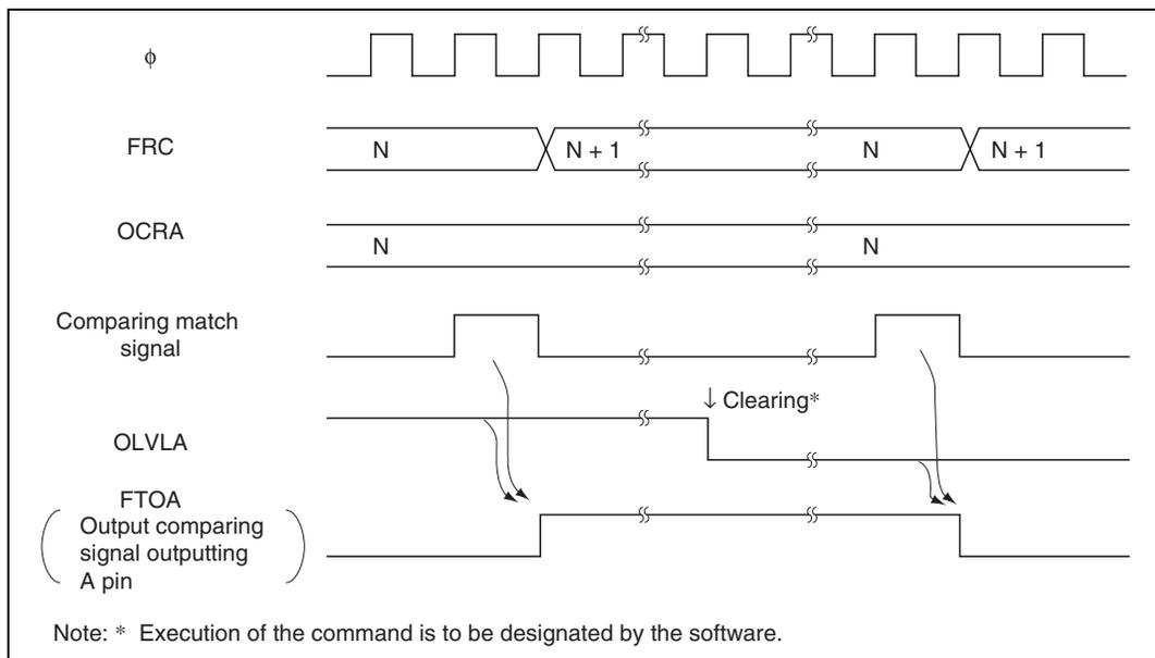
**Figure 16.5 Output Comparing Signal Outputting A Timing**
