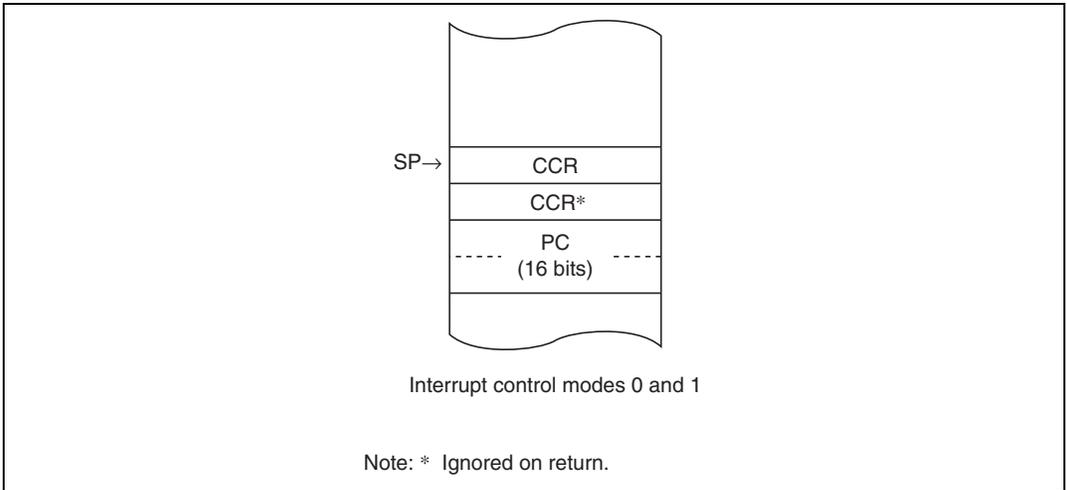
**Figure 5.4 Stack Status after Exception Handling (Normal Mode)\***
