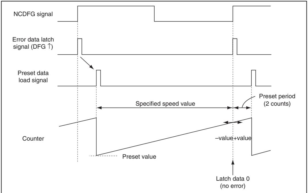
**Figure 26.28 Example of the Drum Speed Error Detection
