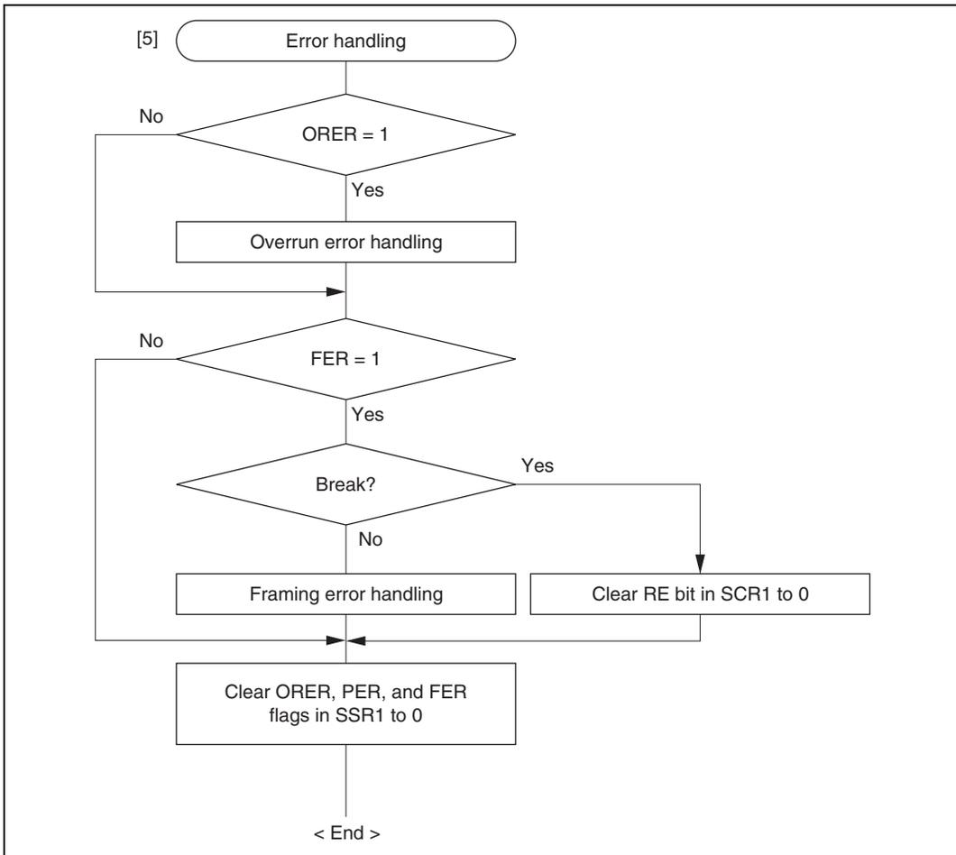
**Figure 22.14 Sample Multiprocessor Serial Reception Flowchart (2)**
