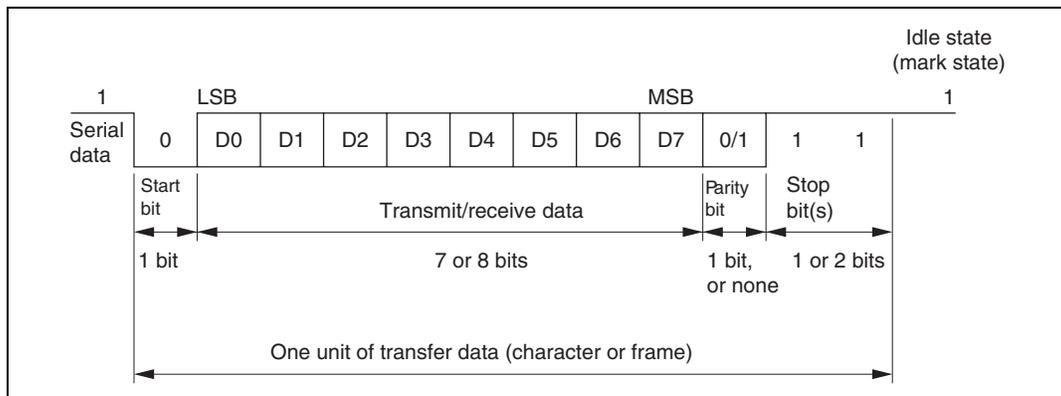
**Figure 22.2 Data Format in Asynchronous Communication**
