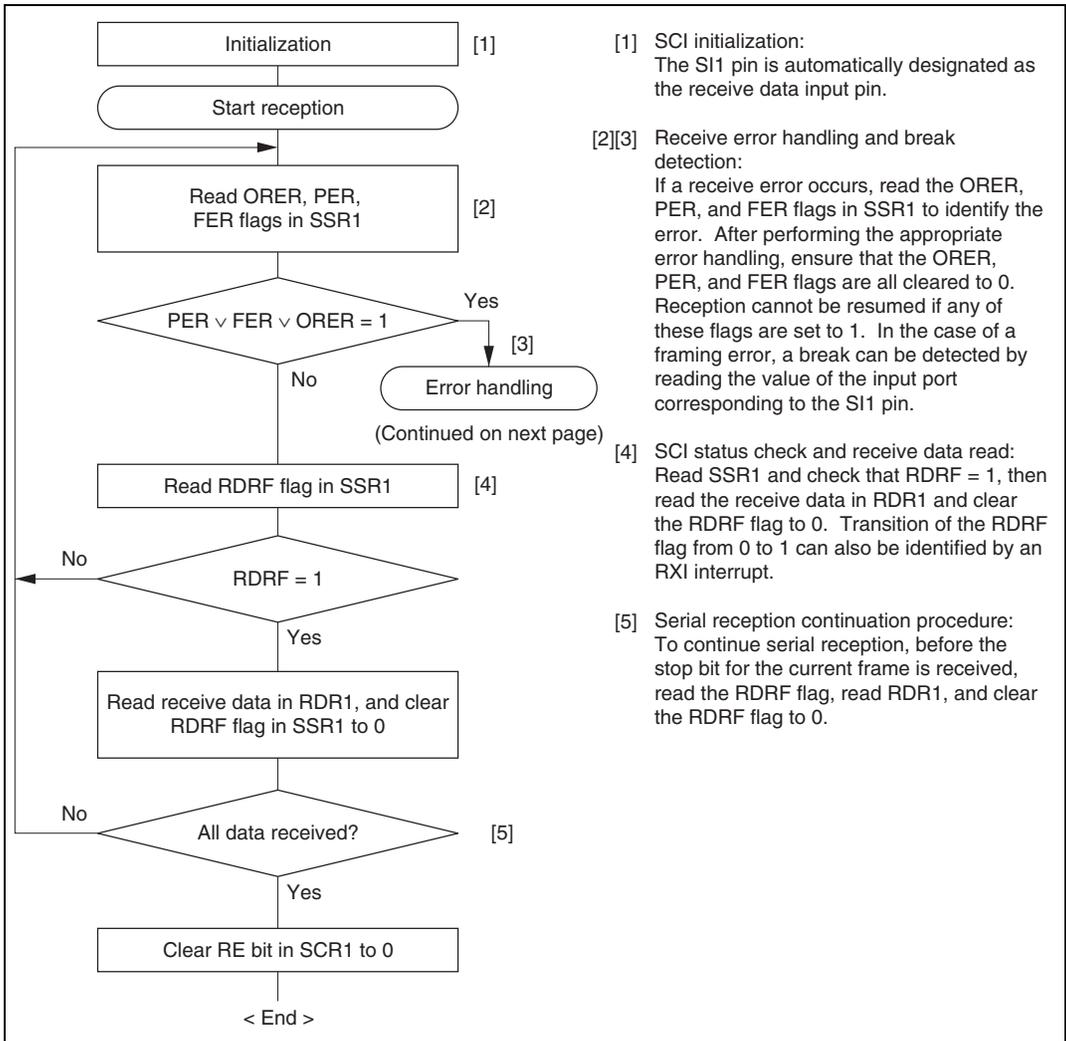
**Figure 22.7 Sample Serial Reception Data Flowchart (1)**
