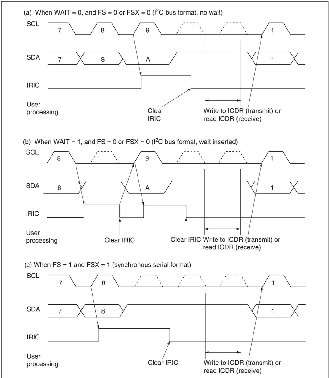
**Figure 23.12 IRIC Setting Timing and SCL Control**
