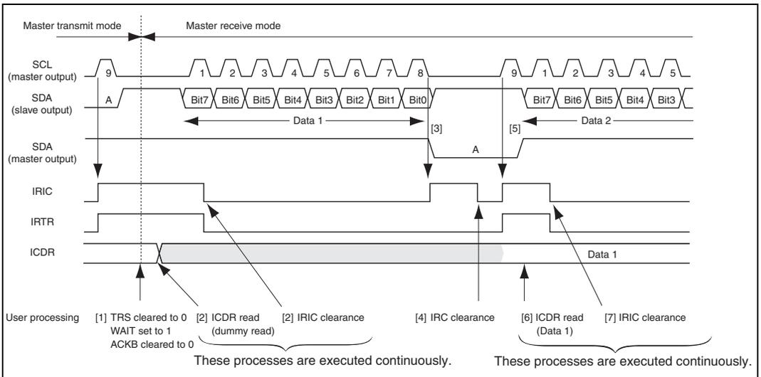
**Figure 23.7 Example of Master Receive Mode Operation Timing**
