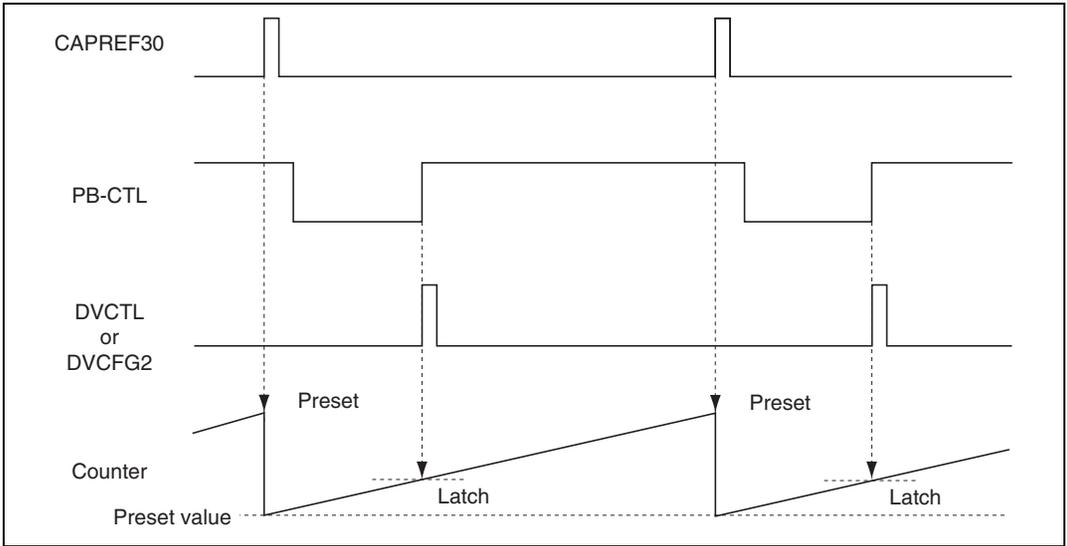
**Figure 26.35 Capstan Phase Control in Playback Mode**
