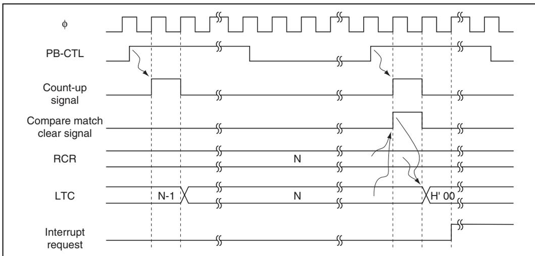
**Figure 14.3 Compare Match Clearing Timing Chart**
