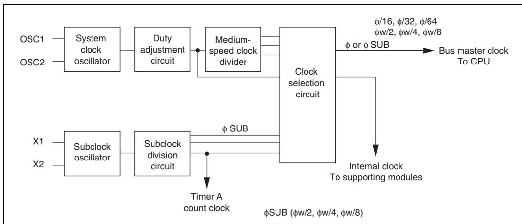
**Figure 9.1 Block Diagram of Clock Pulse Generator**
