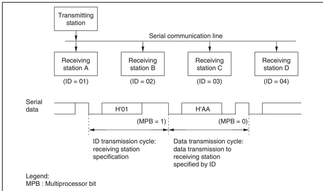
**Figure 22.10 Example of Inter-Processor Communication Using Multiprocessor Format
