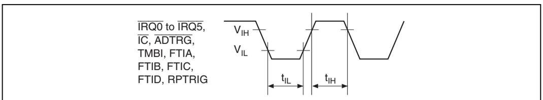
Figure 31.20 Input Timing
