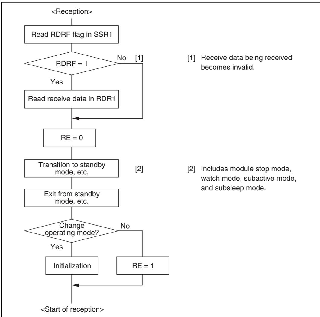
**Figure 22.27 Sample Flowchart for Mode Transition during Reception**
