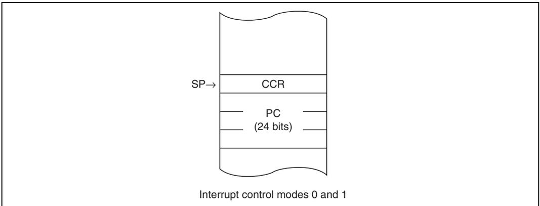
**Figure 5.5 Stack Status after Exception Handling (Advanced Mode)**
