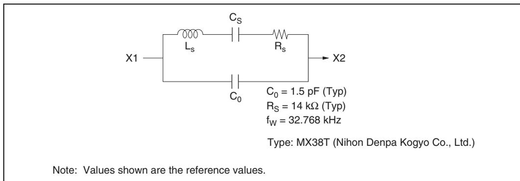
**Figure 9.9 32.768 kHz Crystal Resonator Equivalent Circuit**
