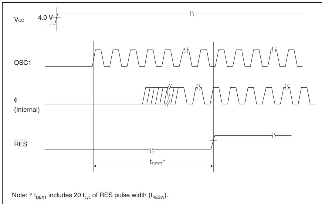
**Figure 9.7 External Clock Output Settling Delay Timing**
