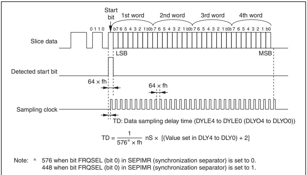
Figure 28.13 Sampling Clock when Bit DSL32B Is 1
