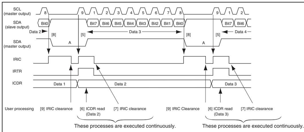
**Figure 23.8 Example of Master Receive Mode Operation Timing
