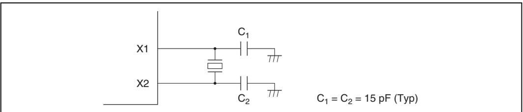
**Figure 9.8 Connecting a 32.768 kHz Crystal Resonator (Example)**
