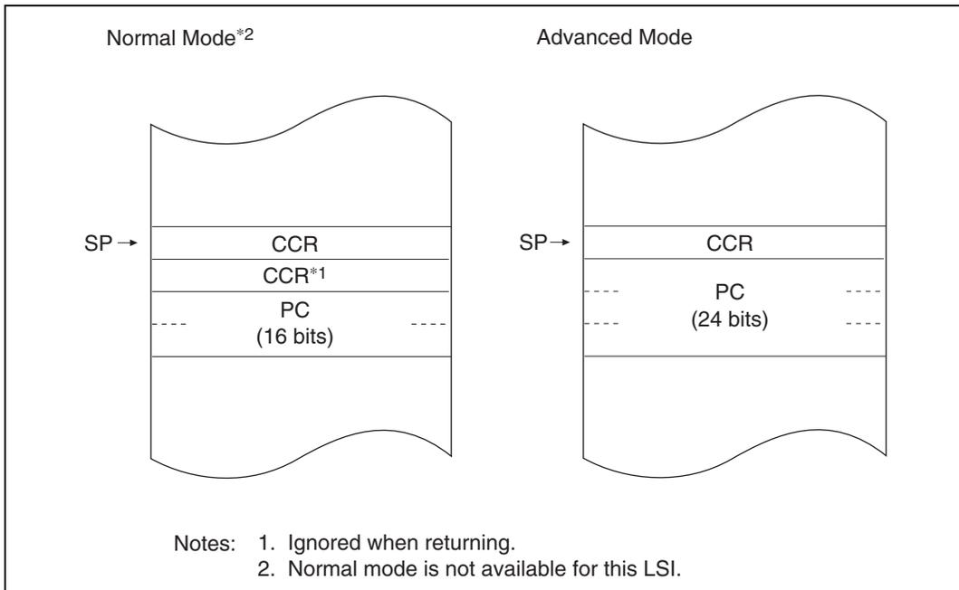
**Figure 2.17 Stack Structure after Exception Handling (Examples)**
