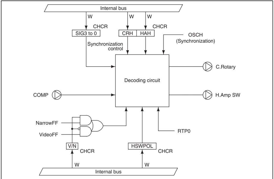
**Figure 26.26 High-Speed Switching Circuit for Four-Head Special Playback**
