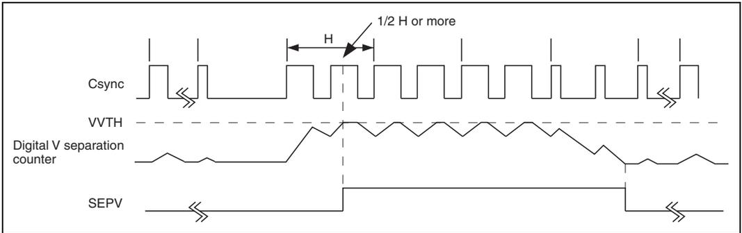
**Figure 27.10 VVTH Value and SEPV Generation Timing**
