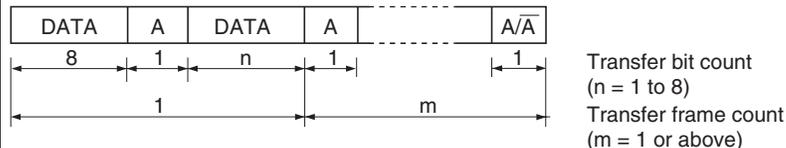
**Figure 23.3 I<sup>2</sup>C Bus Data Formats (I<sup>2</sup>C Bus Formats)**
