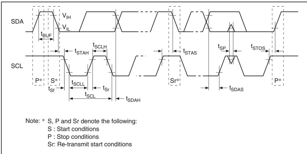
**Figure 31.8 I<sup>2</sup>C Bus Interface I/O Timing**
