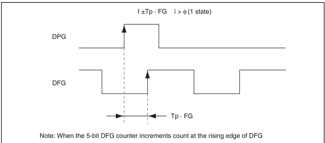
**Figure 26.25 Input Timing of DPG and DFG**
