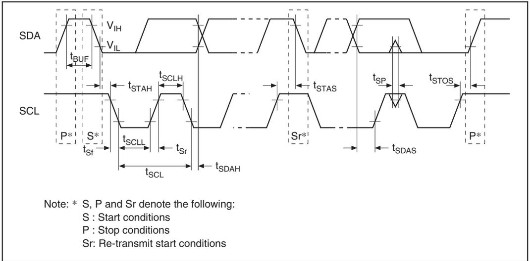
**Figure 31.24 I<sup>2</sup>C Bus Interface I/O Timing**
