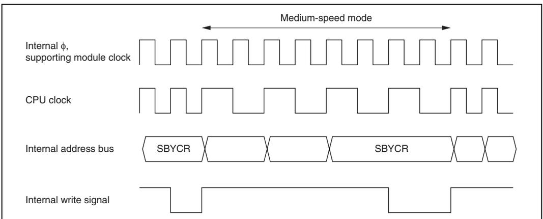
**Figure 4.2 Medium-Speed Mode Transition and Clearance Timing**
