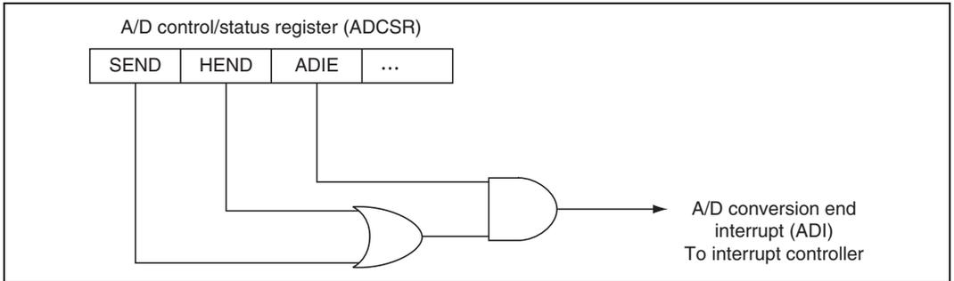
**Figure 24.4 Block Diagram of A/D Conversion End Interrupt**
