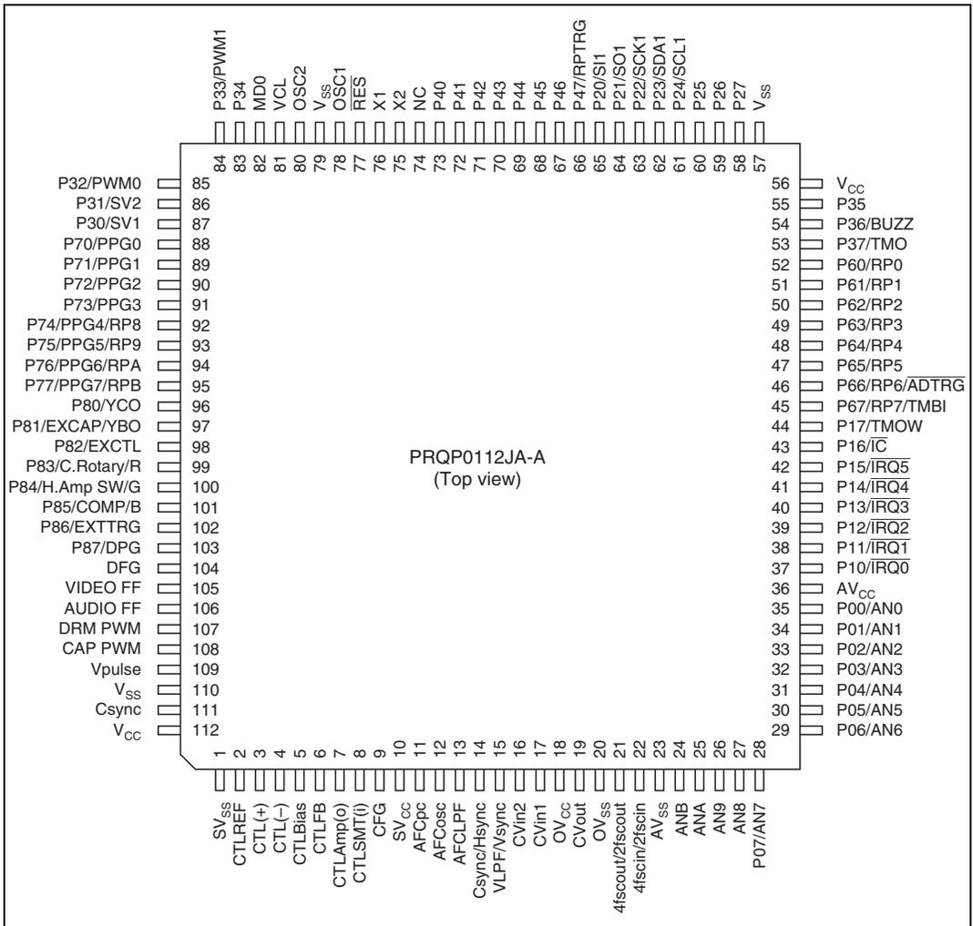
**Figure 1.4 Pin Arrangement of H8S/2197S and H8S/2196S**
