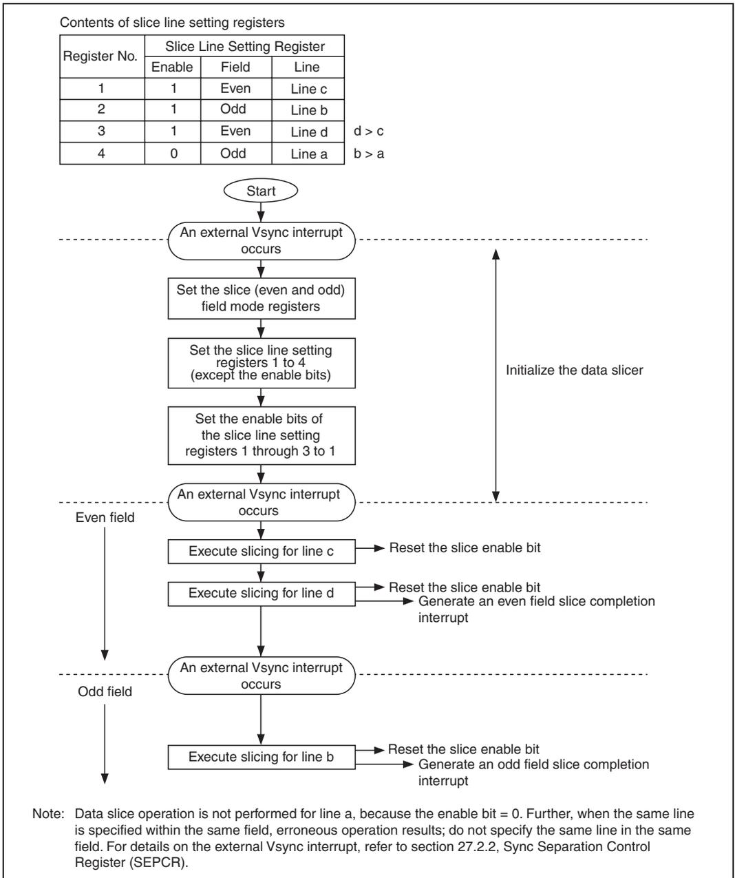
**Figure 28.9 Example of Slice Line Specification and Operation (1)**
