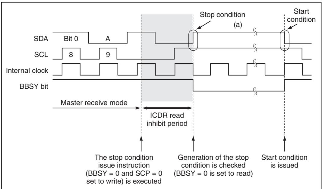
**Figure 23.18 Precautions on Reading the Master Receive Data**
