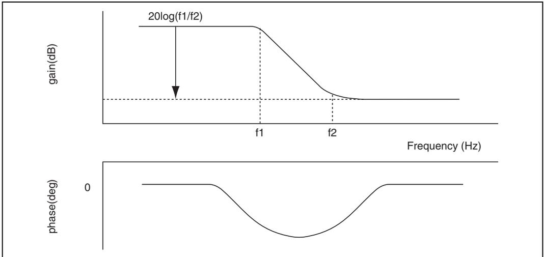
**Figure 26.41 Frequency Characteristics of the Lag-Lead Filter**
