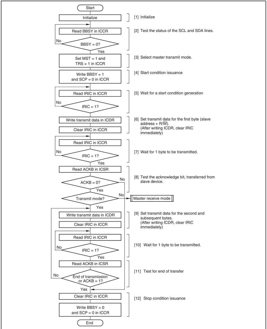
Figure 23.14 Flowchart for Master Transmit Mode (Example)
