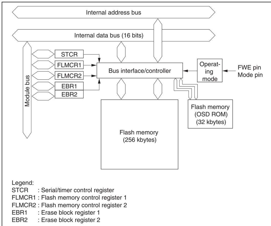
**Figure 7.2 Block Diagram of Flash Memory (H8S/2199R Only)**
