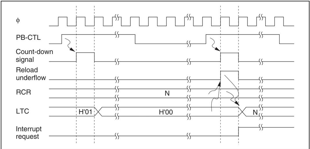
**Figure 14.5 Reload Timing (Rising Edge of PB-CTL Selected)**
