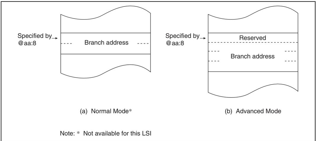
**Figure 2.14 Branch Address Specification in Memory Indirect Mode**
