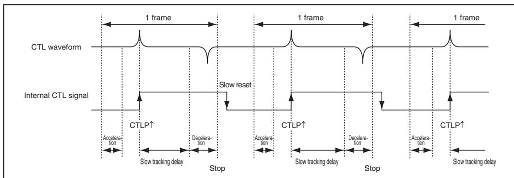
**Figure 26.54 PB-CTL Waveform in Slow Mode Operation**
