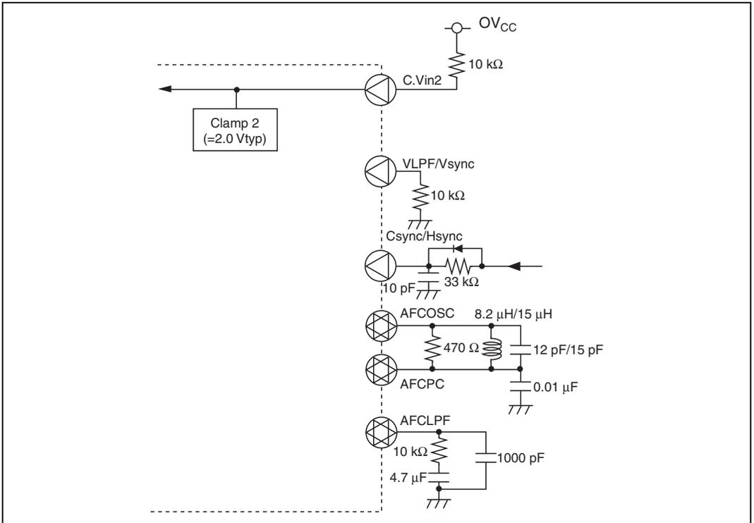
**Figure E.9 Example of External Circuit for Sync Separator and Data Slicer
