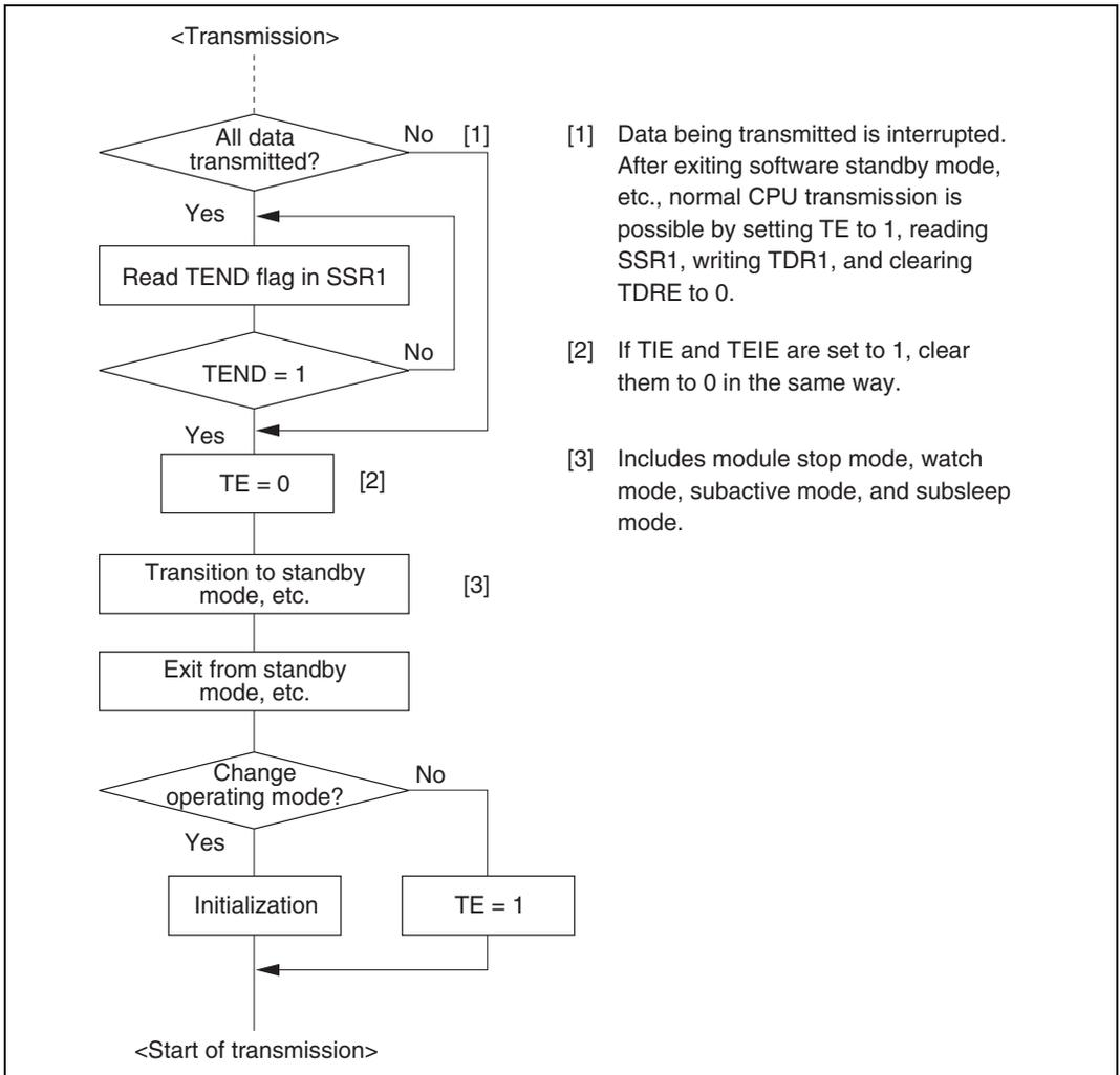
**Figure 22.24 Sample Flowchart for Mode Transition during Transmission**
