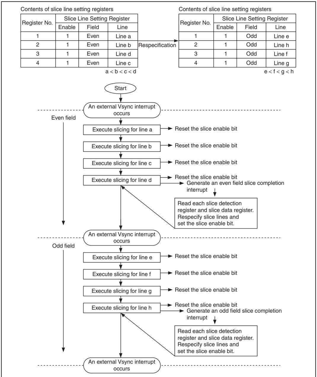
**Figure 28.10 Example of Slice Line Specification and Operation (2)**
