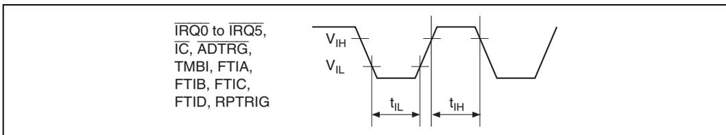
**Figure 31.4 Input Timing**
