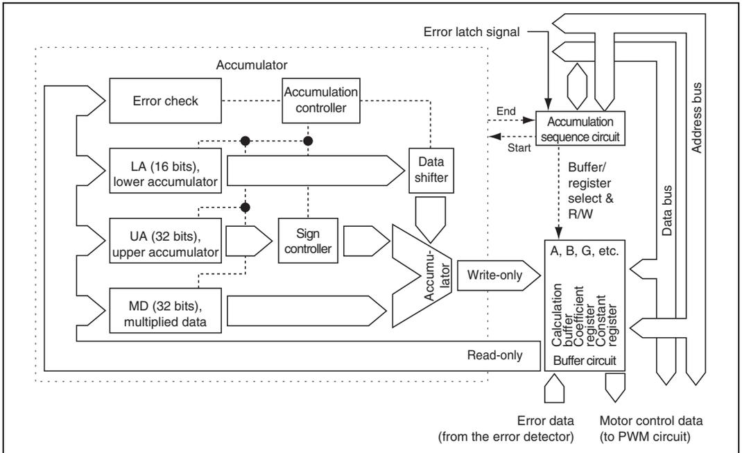
Figure 26.38 Block Diagram of Digital Filter Circuit
