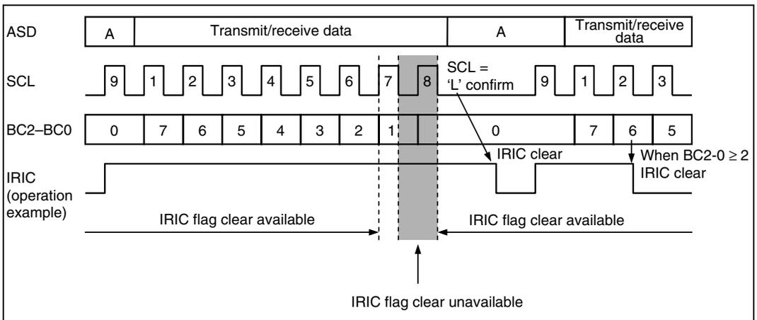
**Figure 23.21 IRIC Flag Clear Timing on WAIT Operation**
