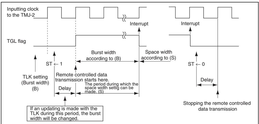
**Figure 13.4 Controls of the Remote Controlled Data Transmission**
