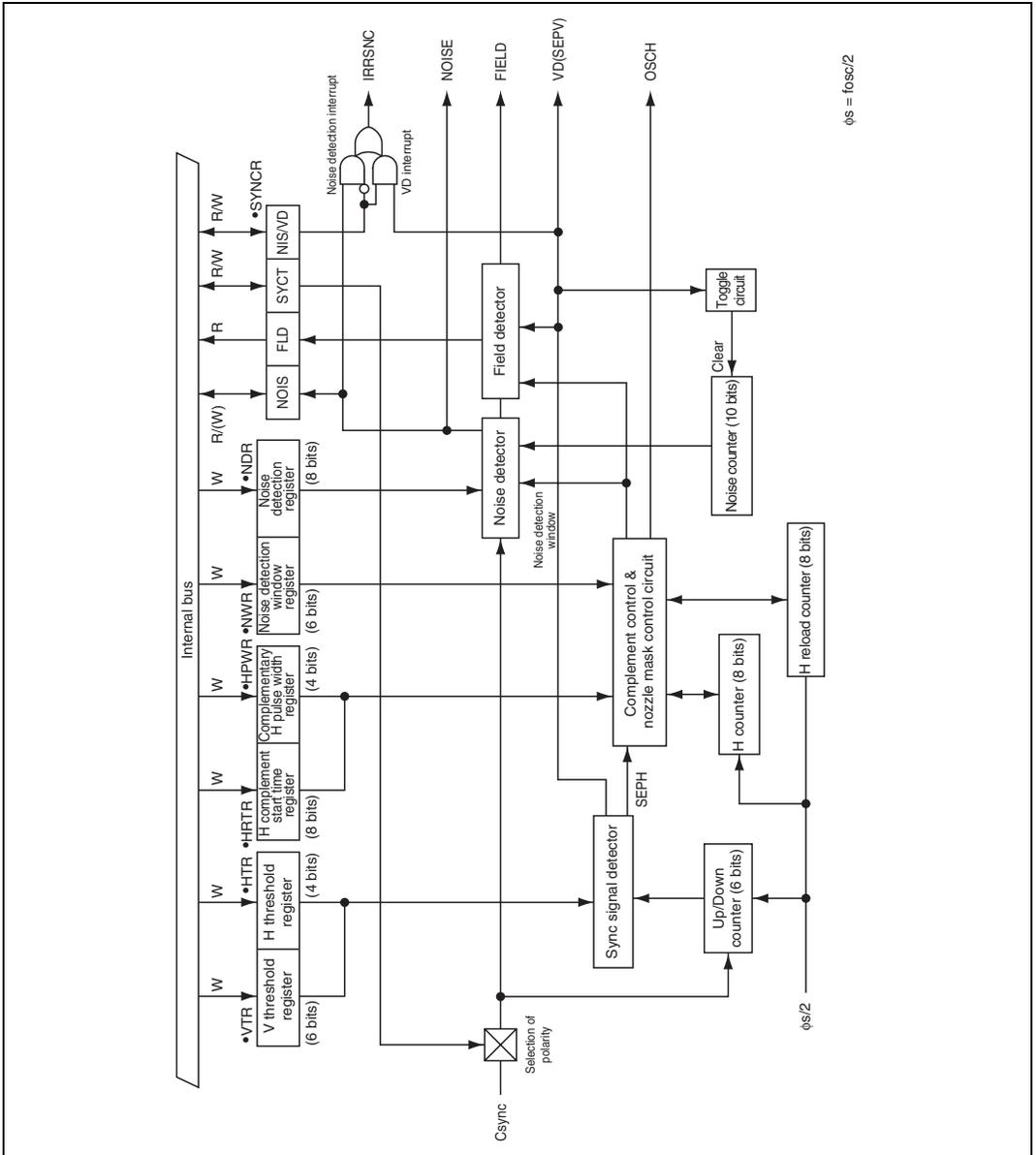
Figure 26.72 Block Diagram of the Sync Signal Detector
