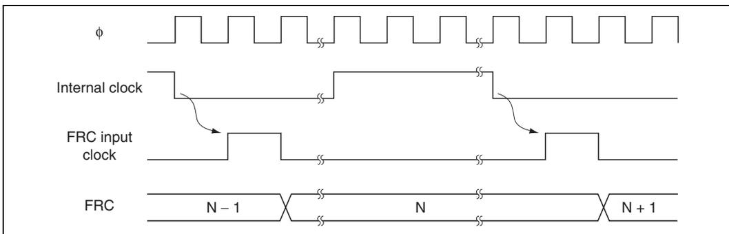
**Figure 16.3 Count Timing for Internal Clock Operation**
