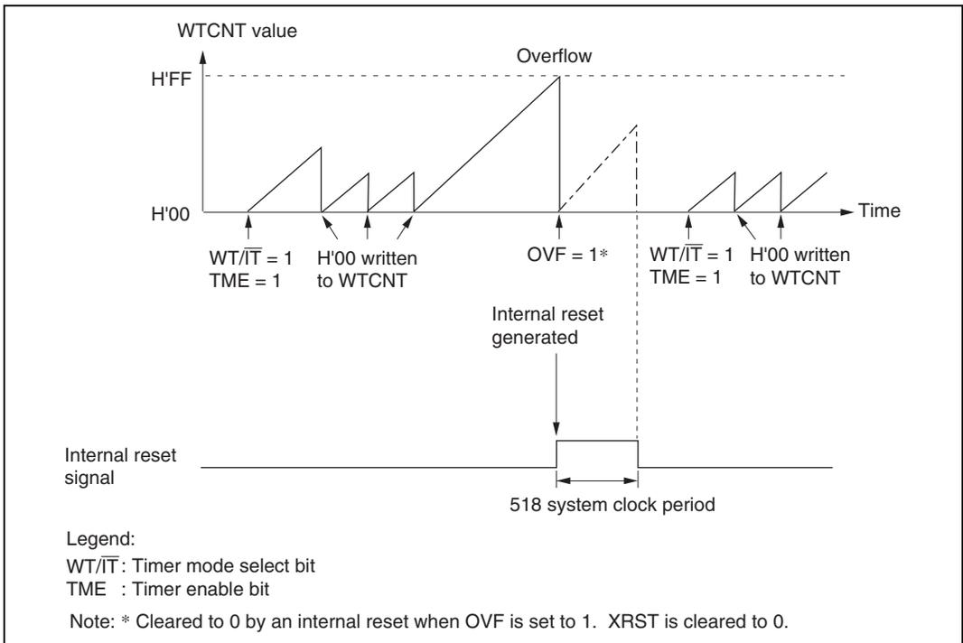
**Figure 17.3 Operation in Watchdog Timer Mode (when Reset)**
