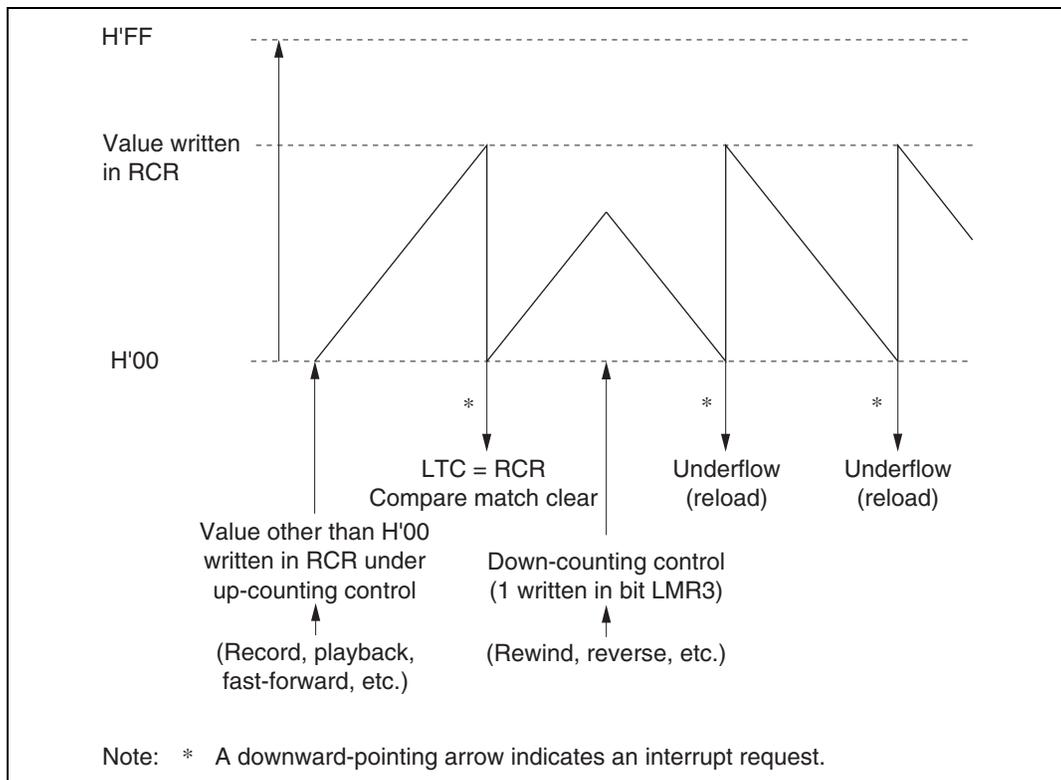
**Figure 14.6 Typical Usage of Linear Time Counter**
