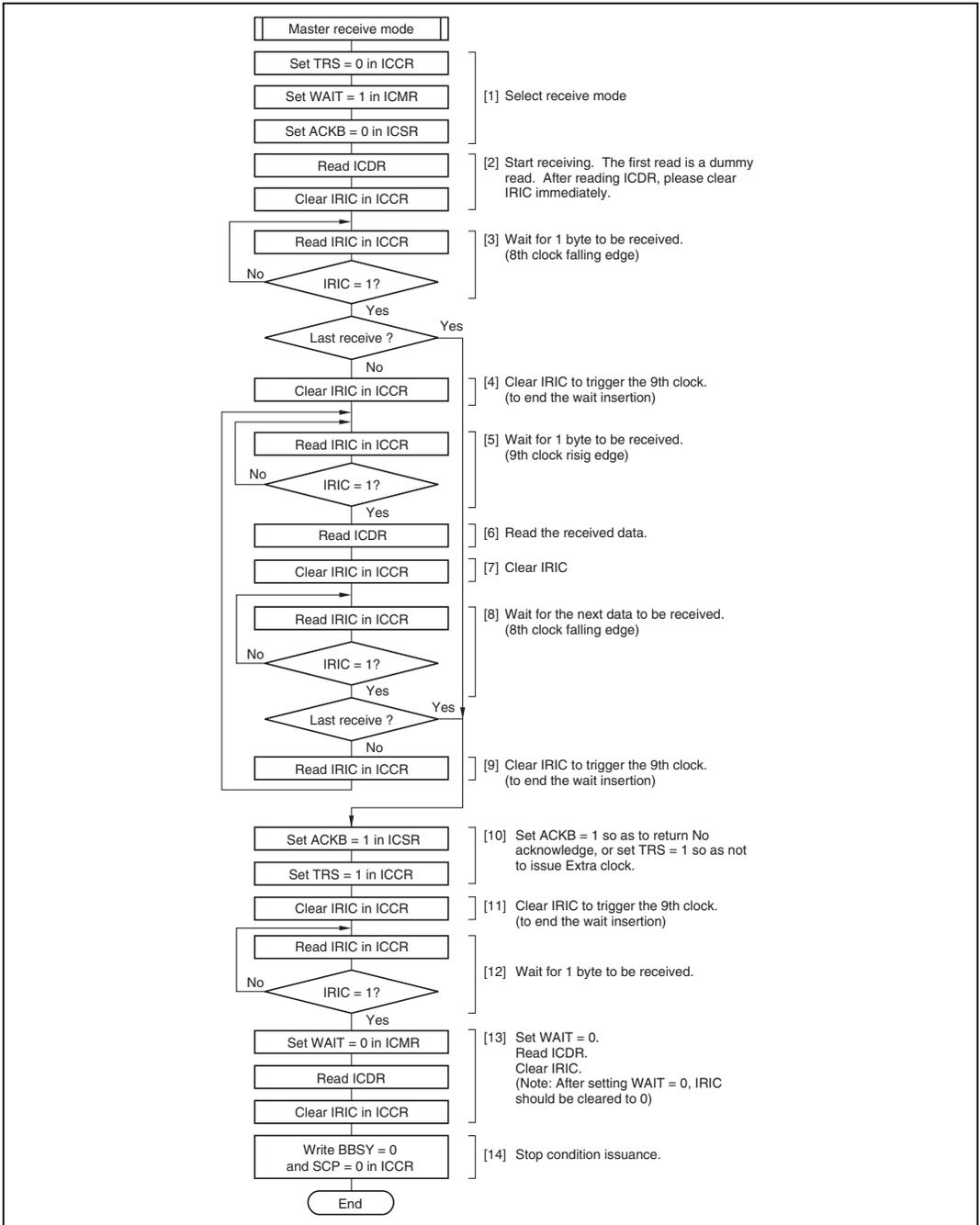
Figure 23.15 Flowchart for Master Receive Mode (Example)
