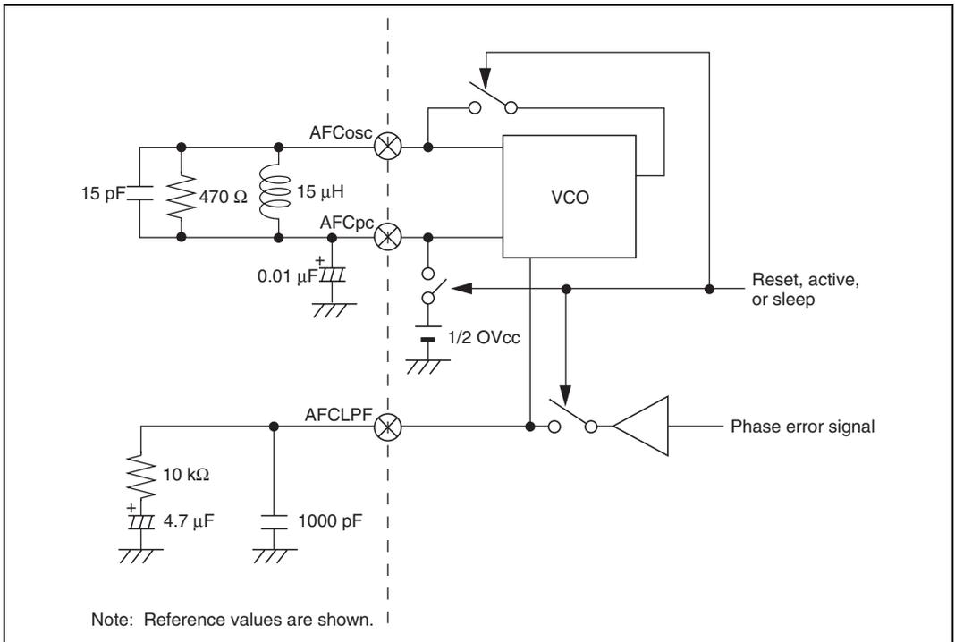
**Figure 27.24 Circuit Example for a 448 × fh Reference Clock**
