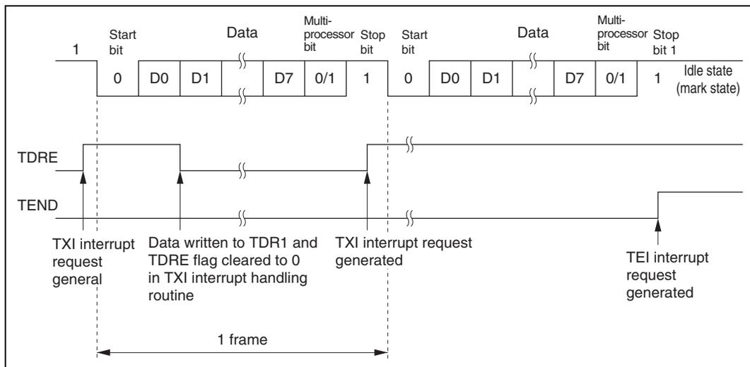
**Figure 22.12 Example of SCI Operation in Transmission
