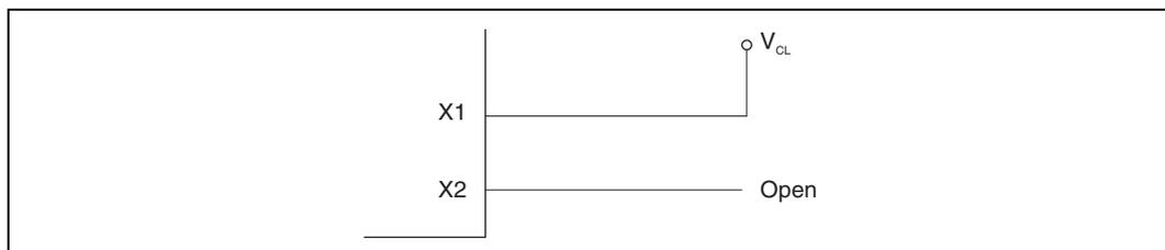
**Figure 9.10 Terminal When Subclock Is Not Needed**
