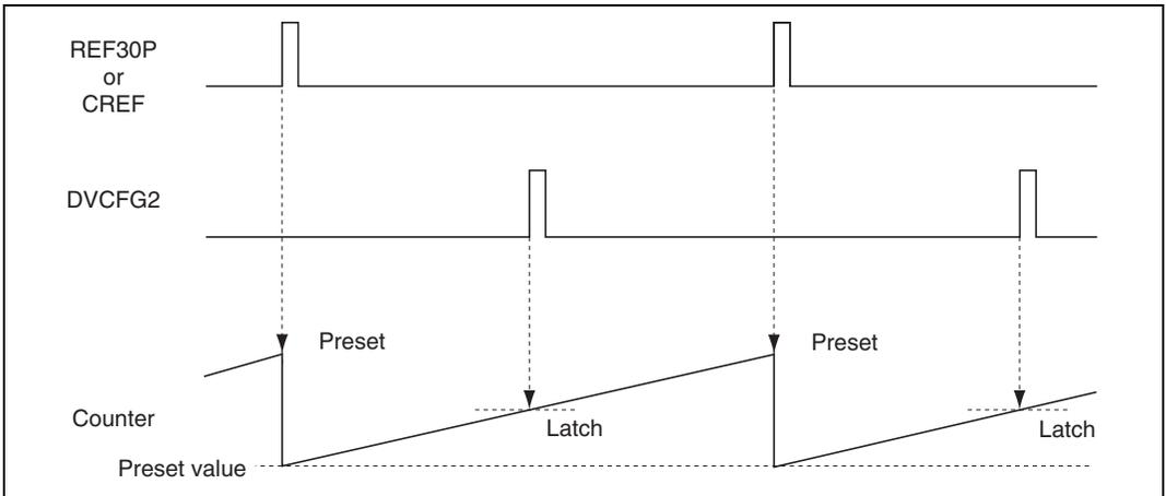
**Figure 26.36 Capstan Phase Control in Record Mode**
