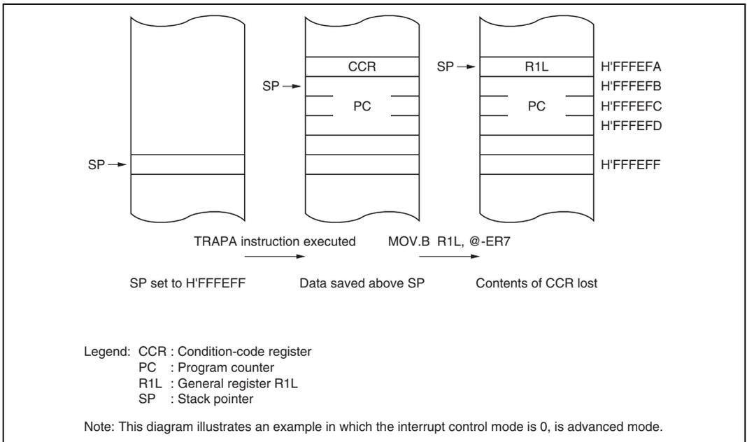
**Figure 5.6 Operation when SP Value Is Odd**
