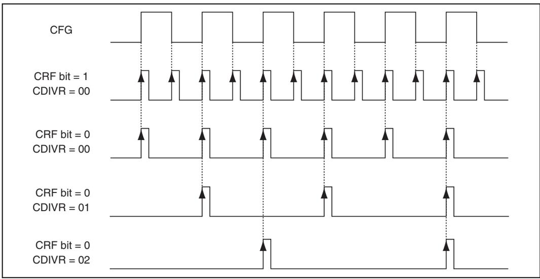
**Figure 26.66 CFG Frequency Division Waveforms**
