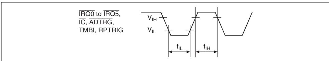
**Figure 31.12 Input Timing**
