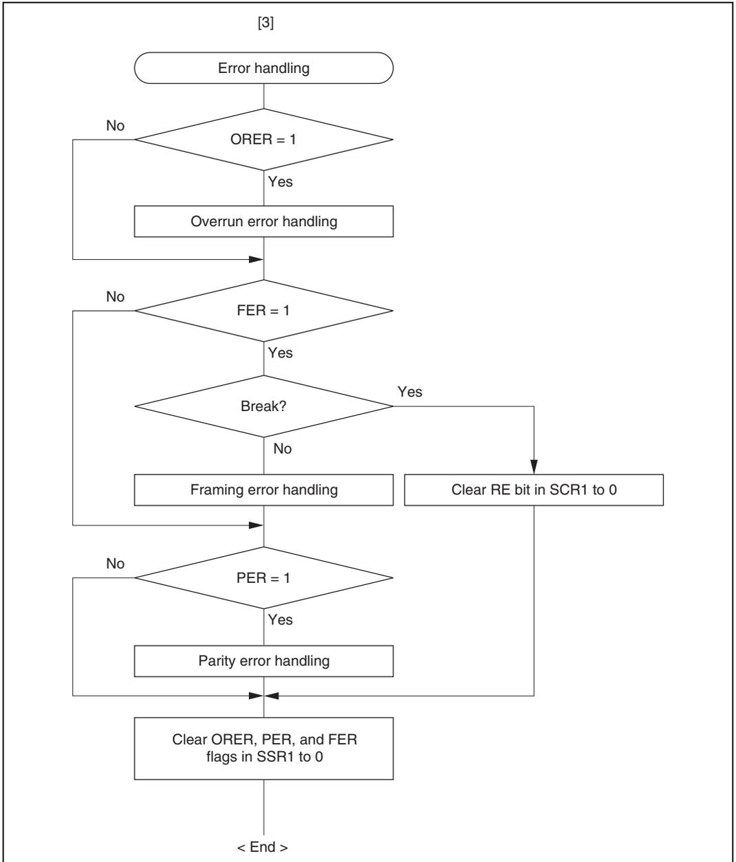
Figure 22.8 Sample Serial Reception Data Flowchart (2)
