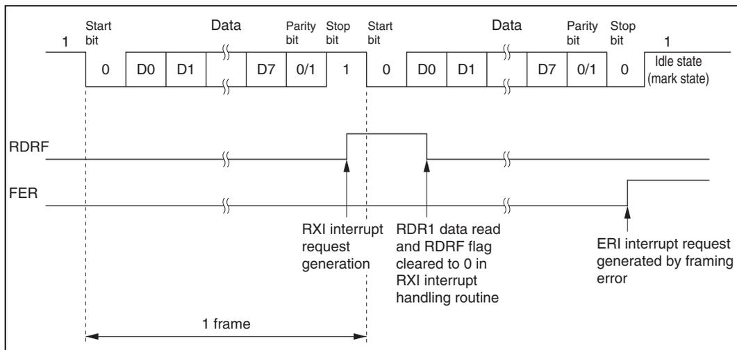
**Figure 22.9 Example of SCI Operation in Reception
