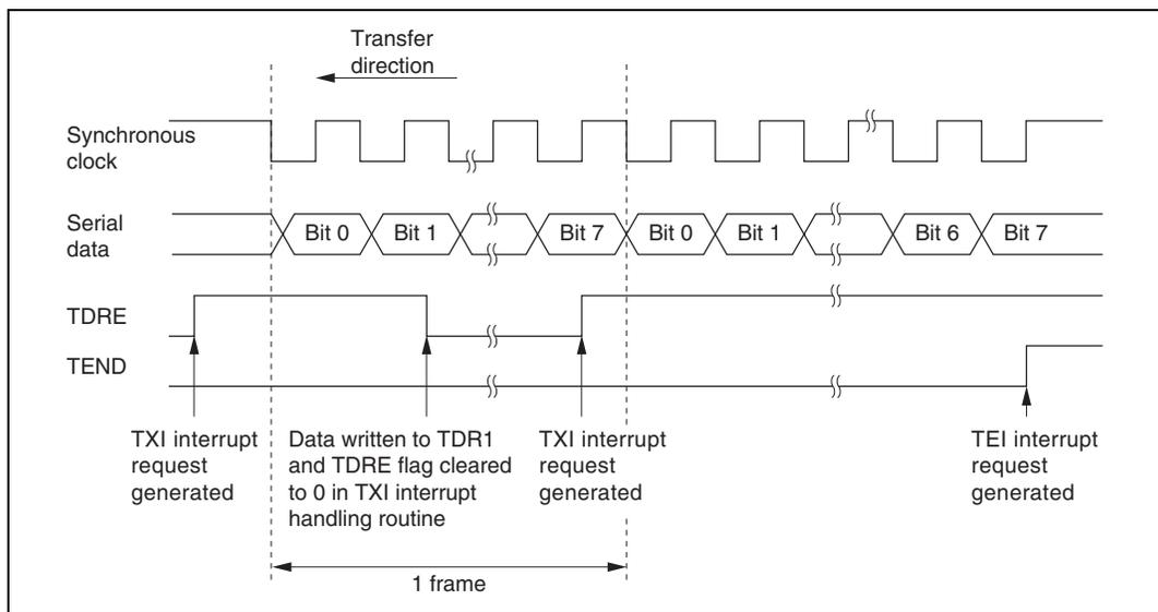
**Figure 22.19 Example of SCI Operation in Transmission**
