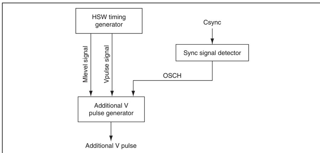
**Figure 26.43 Additional V Pulse Control Circuit**
