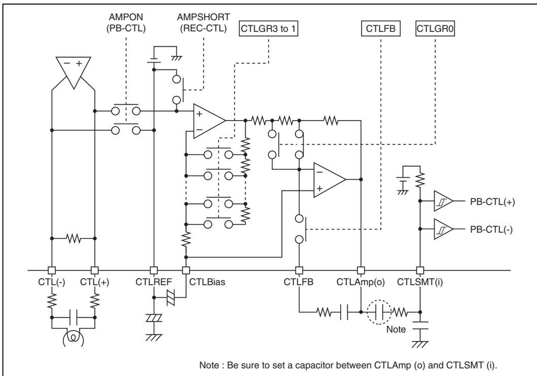
**Figure 26.52 Block Diagram of CTL Input Amplifier**
