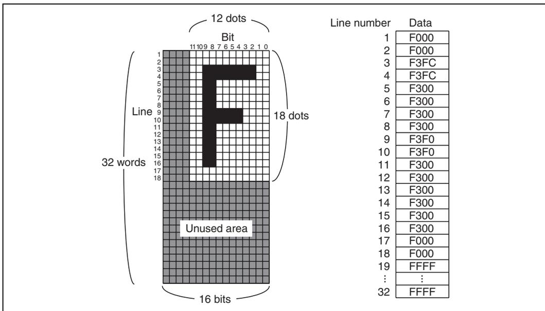
**Figure 29.8 OSDROM Data Configuration (for the letter “F”)**
