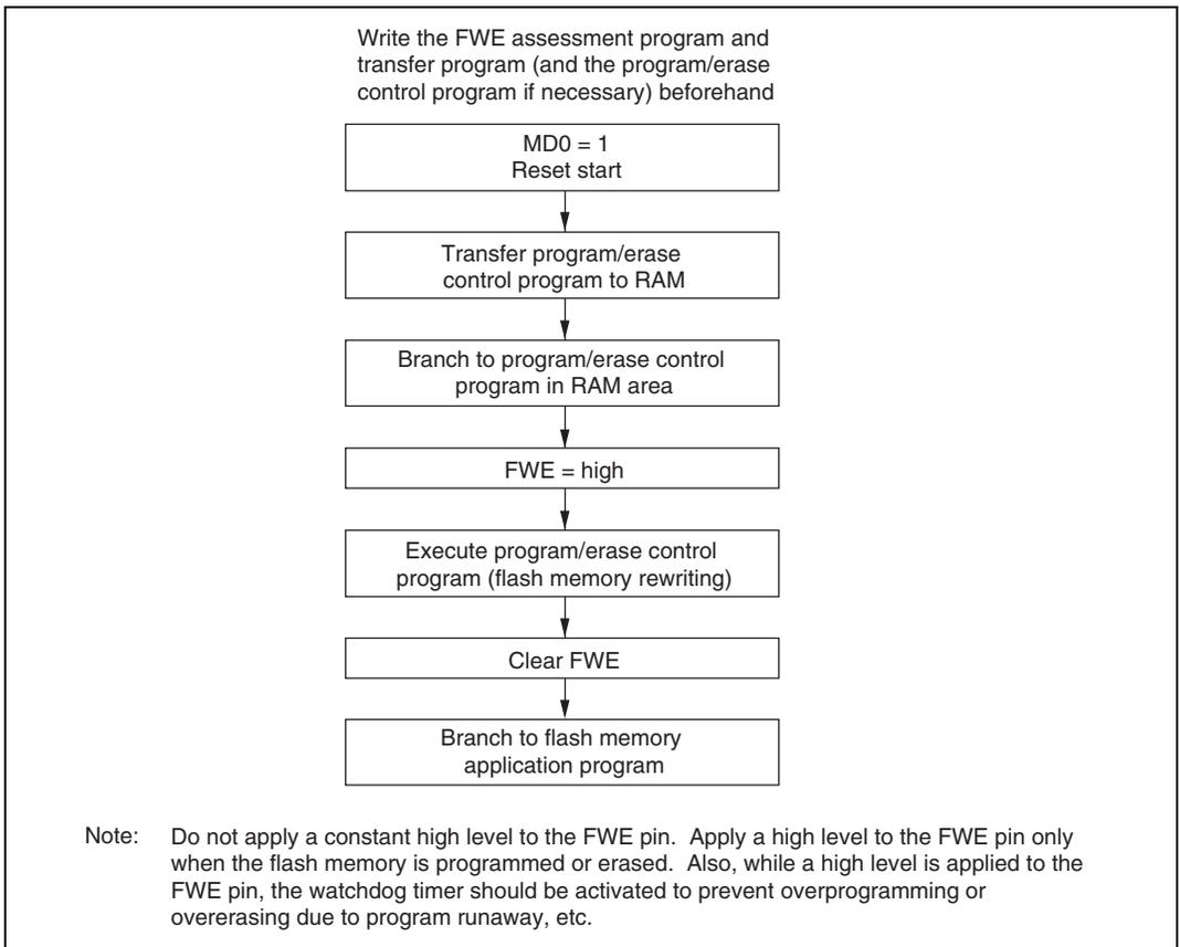
**Figure 7.11 User Program Mode Execution Procedure**
