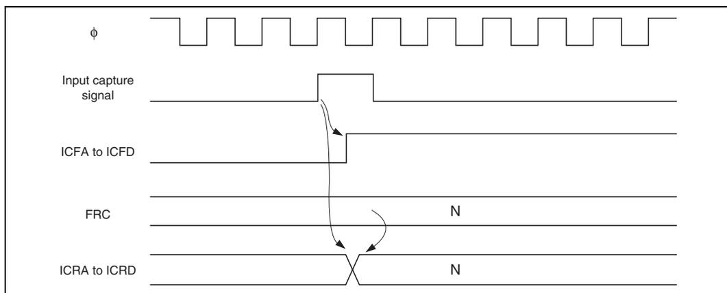
**Figure 16.9 ICFA through ICFD Setting Up Timing**
