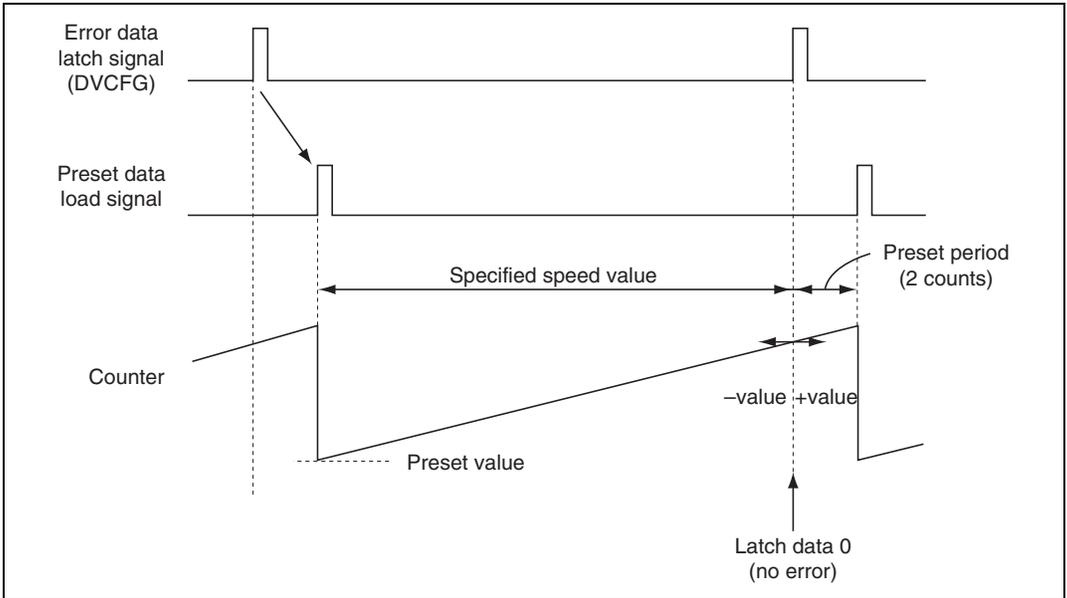
**Figure 26.33 Example of the Capstan Speed Error Detection**
