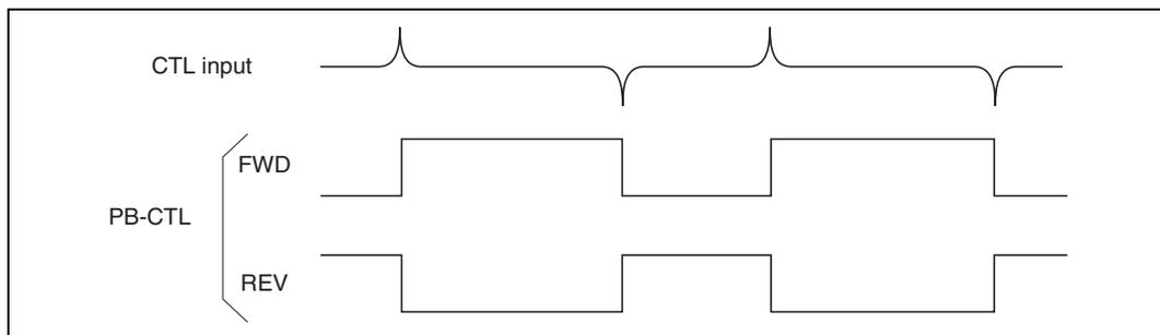
**Figure 26.48 Internal PB-CTL Signal in Forward and Reverse**
