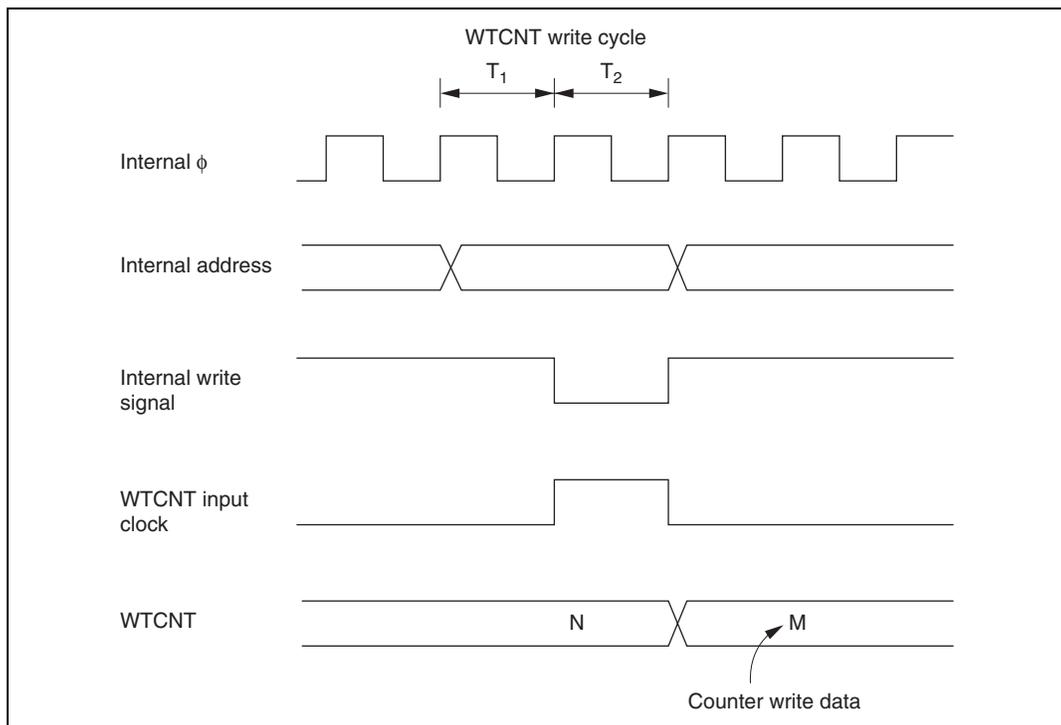
**Figure 17.6 Contention between WTCNT Write and Increment**
