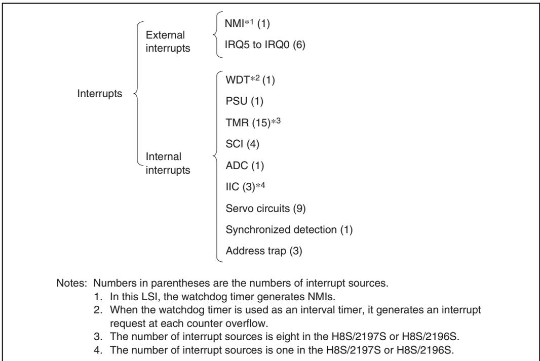
**Figure 5.3 Interrupt Sources and Number of Interrupts**
