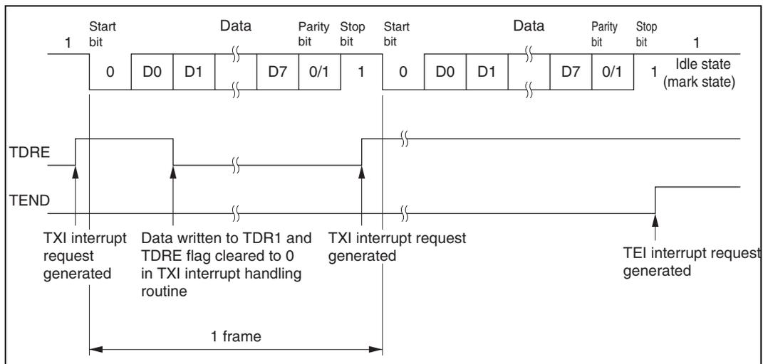
**Figure 22.6 Example of Operation in Transmission in Asynchronous Mode
