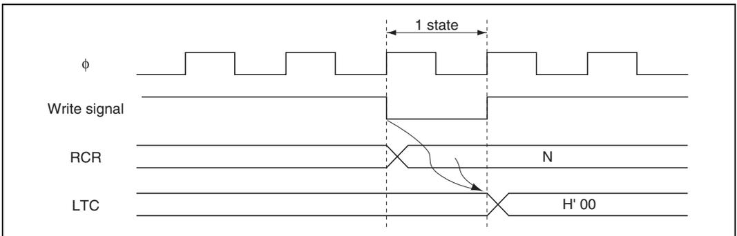
Figure 14.2 RCR Writing and LTC Clearing Timing Chart
