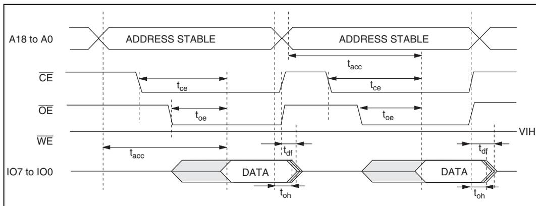
Figure 7.19 Timing Waveforms for  $\overline{CE}/\overline{OE}$  Clocked Read
