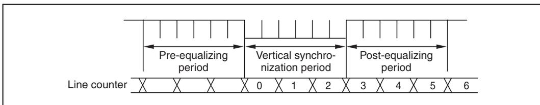
**Figure 29.10 Base Point for Vertical Display Start Positions**
