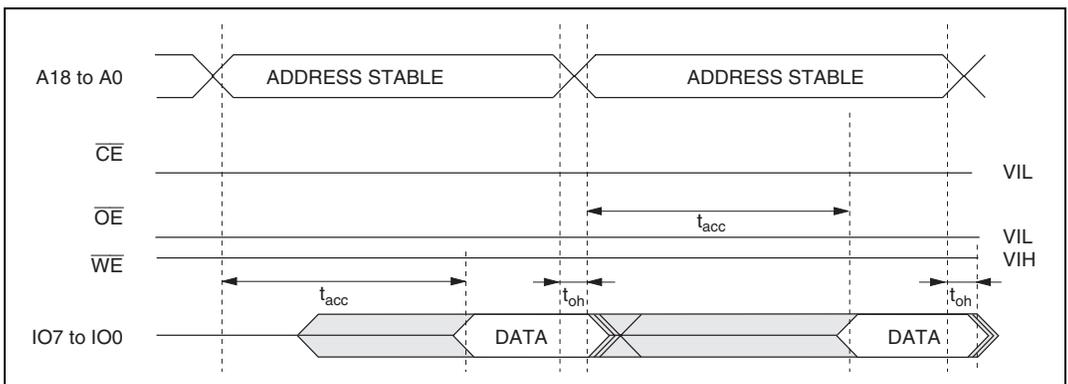
**Figure 7.18 Timing Waveforms for  $\overline{CE}/\overline{OE}$  Enable State Read**
