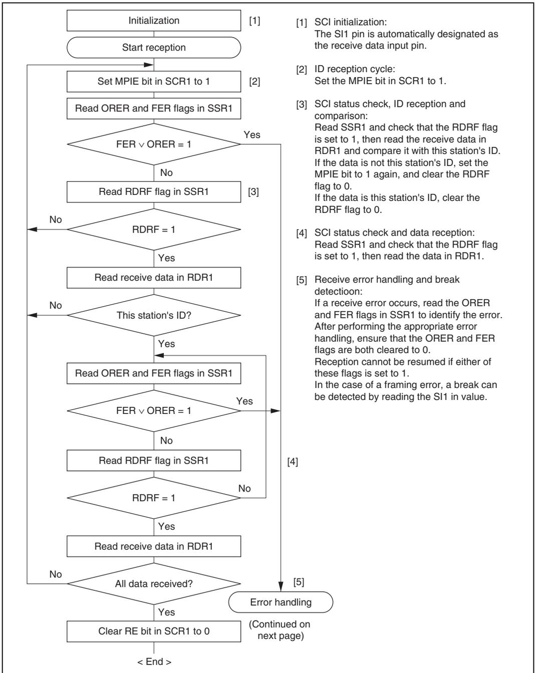
Figure 22.13 Sample Multiprocessor Serial Reception Flowchart (1)
