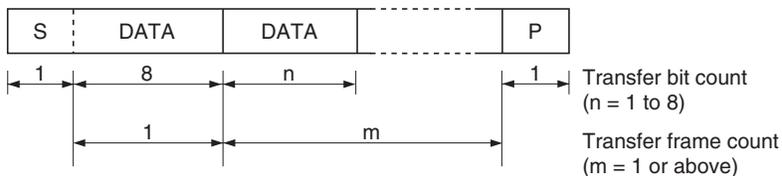
**Figure 23.4 I<sup>2</sup>C Bus Data Format (Serial Format)**
