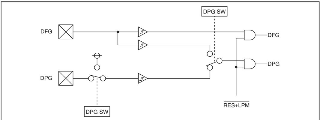
**Figure 26.2 Input Circuit of DFG and DPG**
