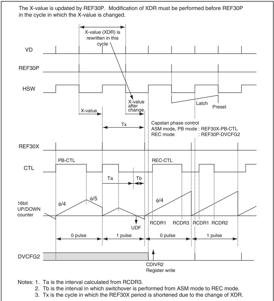
**Figure 26.50 Example of CTLM Switchover Timing**
