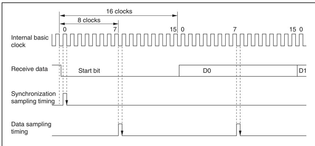
**Figure 22.23 Receive Data Sampling Timing in Asynchronous Mode**
