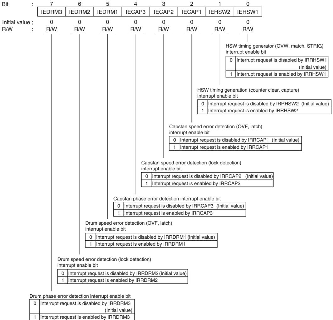
**H'D0B9: Servo Interrupt Enable Register 2 SIENR2: Servo Interrupt**
