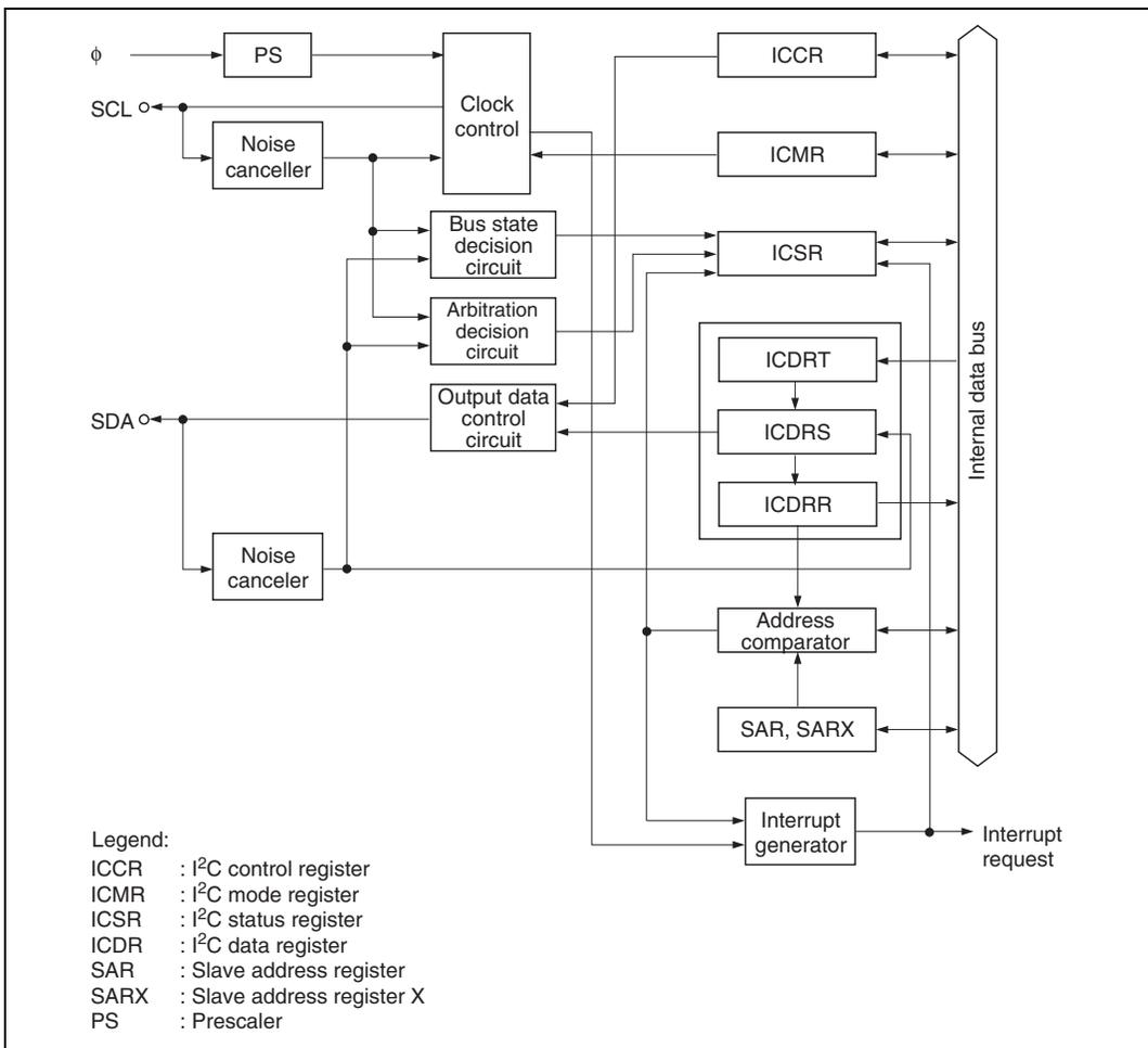
**Figure 23.1 Block Diagram of I<sup>2</sup>C Bus Interface**
