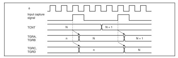
Figure 10.37 Buffer Operation Timing (Input Capture)
