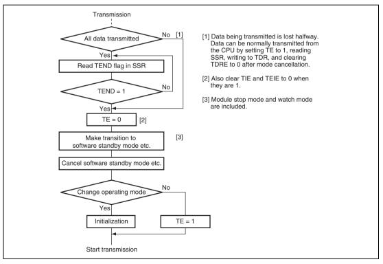
Figure 14.33 Sample Flowchart for Mode Transition during Transmission
