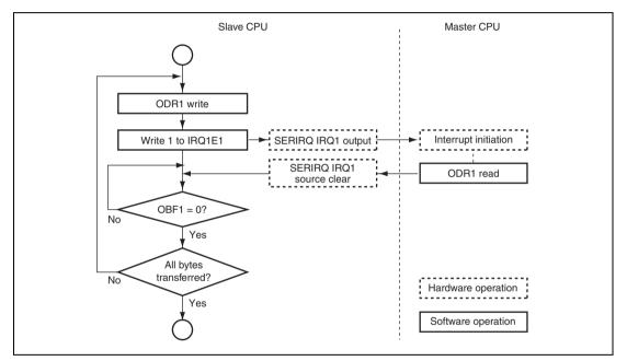
Figure 19.8 HIRQ Flowchart (Example of Channel 1)
