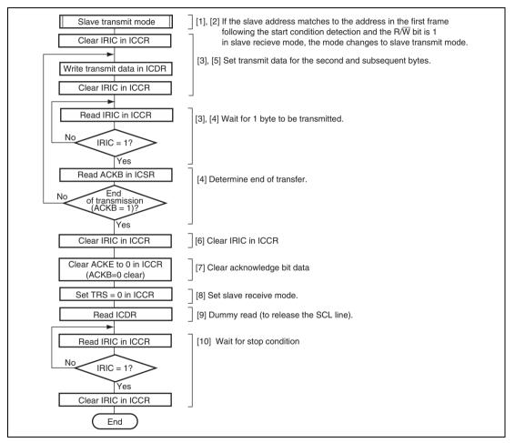
Figure 16.16 Sample Flowchart for Slave Transmit Mode
