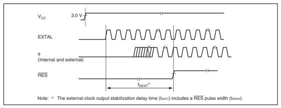
Figure 23.6 Timing of External Clock Output Stabilization Delay Time
