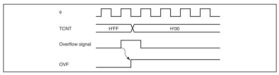
Figure 12.10 Timing of OVF Flag Setting
