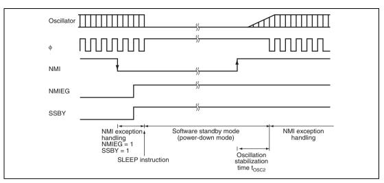
Figure 24.3 Software Standby Mode Application Example
