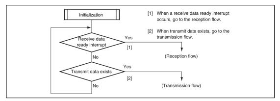
Figure 15.7 Example of Data Transmission/Reception Standby Flowchart
