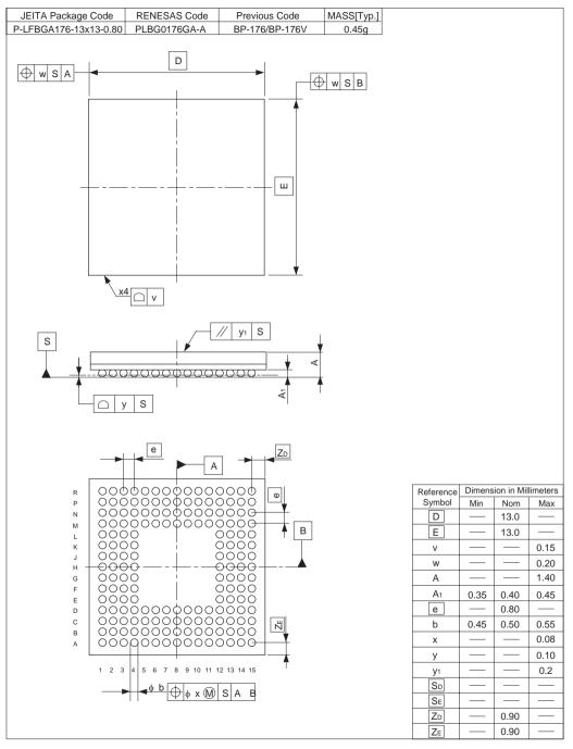
Figure C.2 Package Dimensions (BP-176V)
