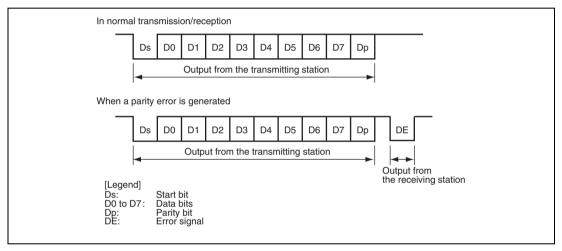
Figure 14.22 Data Formats in Normal Smart Card Interface Mode
