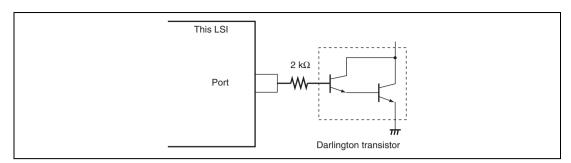
Figure 26.1 Darlington Transistor Drive Circuit (Example)
