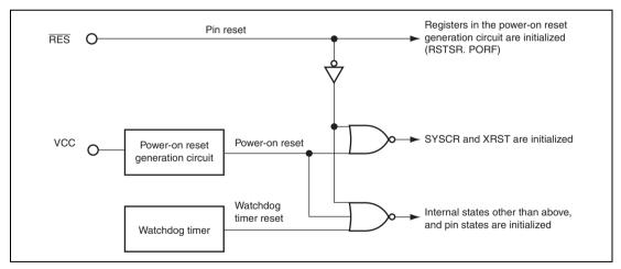
Figure 4.1 Block Diagram of Reset Circuit
