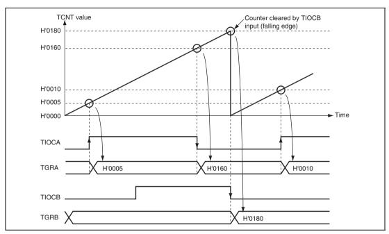
Figure 10.13 Example of Input Capture Operation
