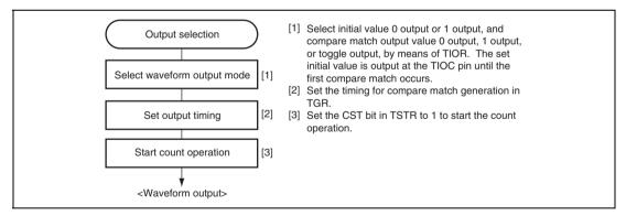
Figure 10.9 Example of Setting Procedure for Waveform Output by Compare Match
