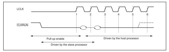
Figure 19.7 Clock Start Request Timing
