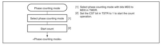
Figure 10.25 Example of Phase Counting Mode Setting Procedure
