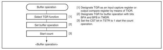
Figure 10.18 Example of Buffer Operation Setting Procedure
