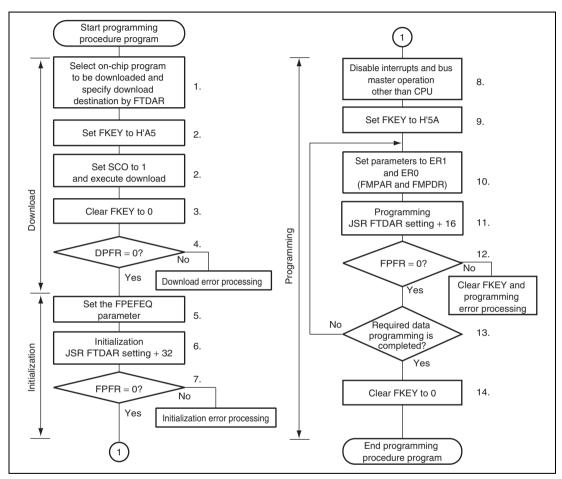
Figure 22.12 Programming Procedure in User Program Mode
