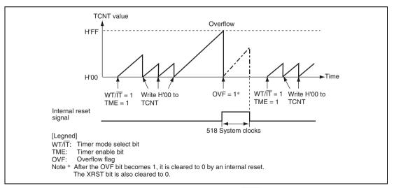
Figure 13.2 Watchdog Timer Mode (RST/<u>NMI</u> = 1) Operation
