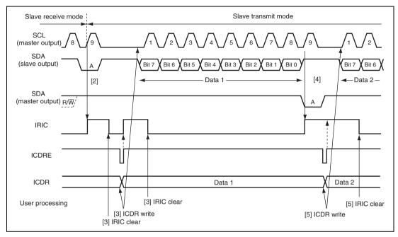
Figure 16.17 Example of Slave Transmit Mode Operation Timing (MLS = 0)
