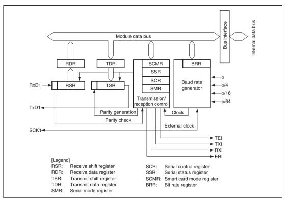
Figure 14.1 Block Diagram of SCI
