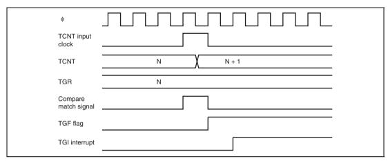
Figure 10.38 TGI Interrupt Timing (Compare Match)
