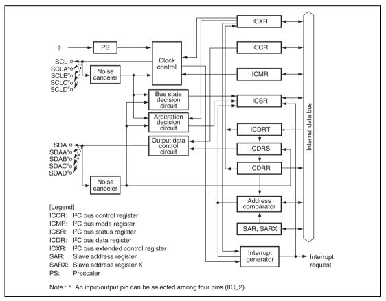
Figure 16.1 Block Diagram of I<sup>2</sup>C Bus Interface
