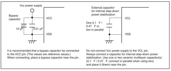
Figure 26.28 Connection of VCL Capacitor
