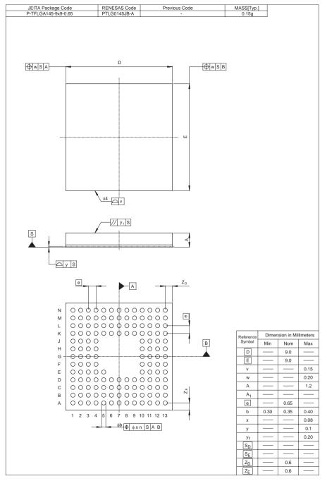
Figure C.3 Package Dimensions (TLP-145V)
