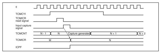
Figure 11.15 Conflict between TCMICR Read and Input Capture
