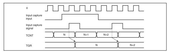
Figure 10.33 Input Capture Input Signal Timing
