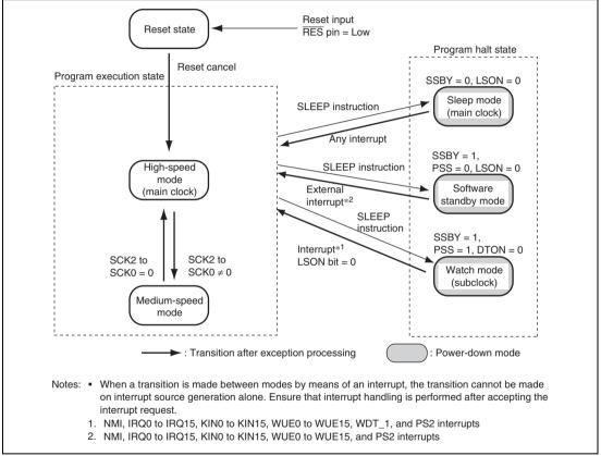
Figure 24.1 Mode Transition Diagram
