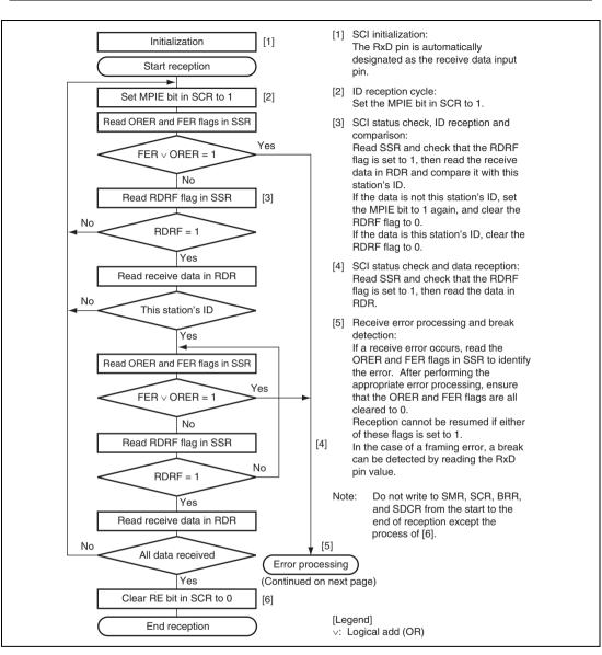
Figure 14.13 Sample Multiprocessor Serial Reception Flowchart (1)
