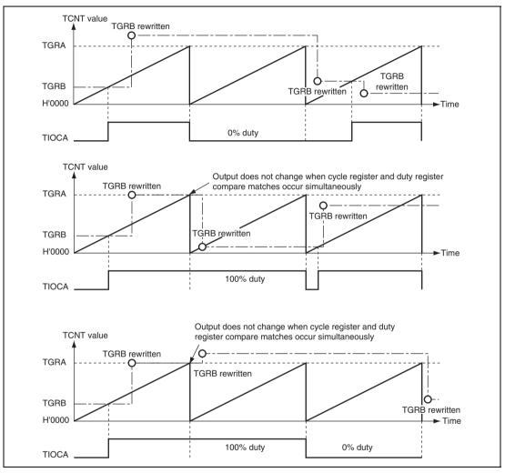
Figure 10.24 Example of PWM Mode Operation (3)
