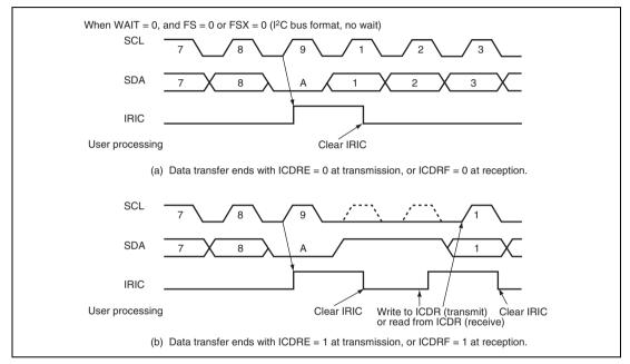
Figure 16.18 IRIC Setting Timing and SCL Control (1)
