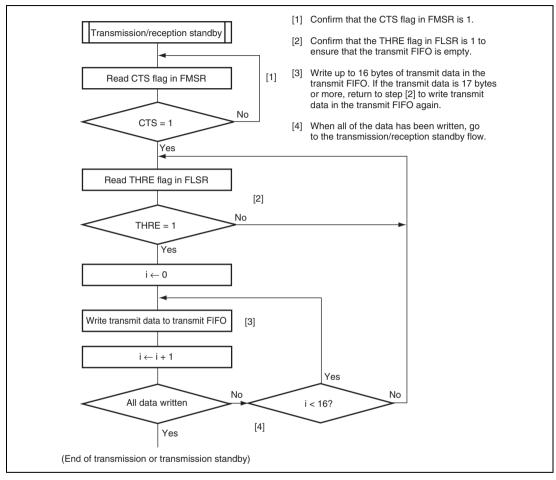
Figure 15.8 Example of Data Transmission Flowchart
