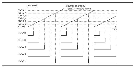
Figure 10.23 Example of PWM Mode Operation (2)
