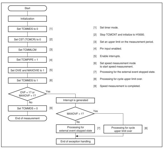
Figure 11.12 Example of Cycle Measurement Mode Settings
