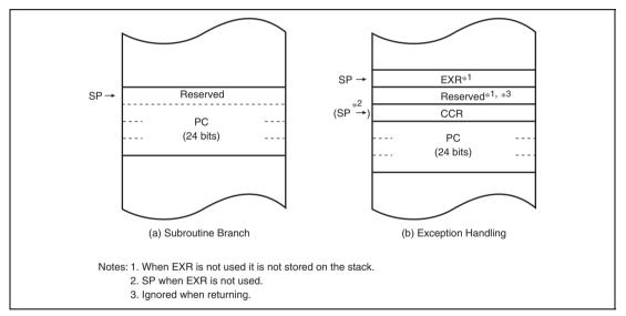
Figure 2.2 Stack Structure
