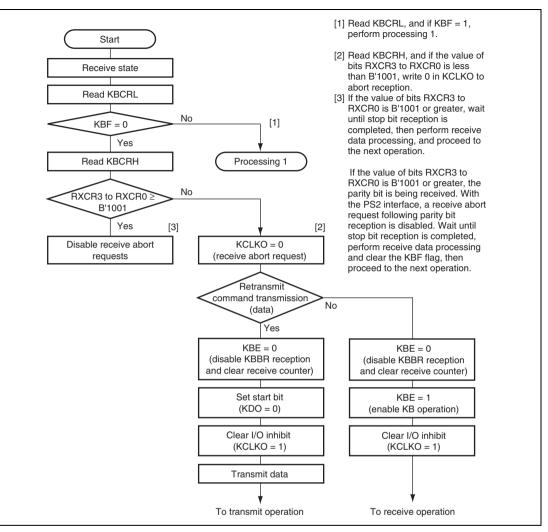
Figure 18.7 Sample Receive Abort Processing Flowchart (1)
