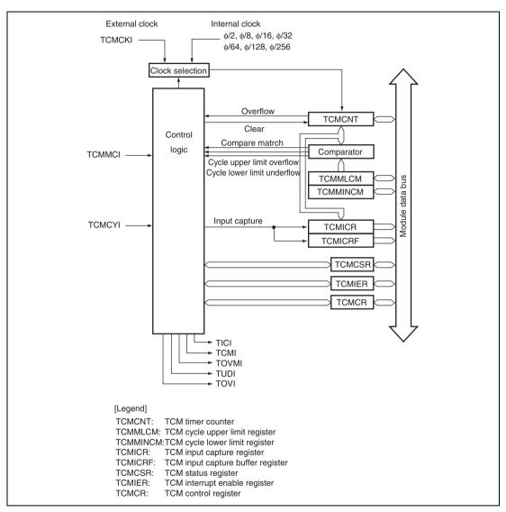
Figure 11.1 Block Diagram of the TCM
