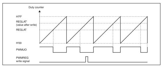
Figure 9.6 PWMU Output Waveform When PWMREG Value is Changed
