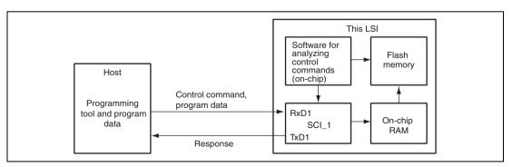
Figure 22.6 System Configuration in Boot Mode
