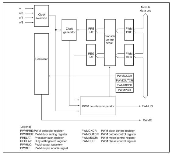
Figure 9.1 Block Diagram of PWMU Timer
