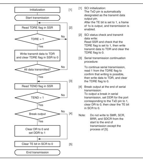
Figure 14.7 Sample Serial Transmission Flowchart
