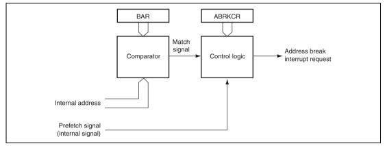
Figure 6.11 Block Diagram of Address Break Function
