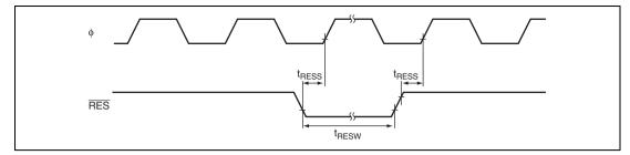
Figure 26.7 Reset Input Timing
