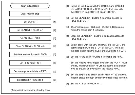
Figure 15.6 Example of Initialization Flowchart
