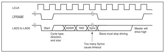
Figure 19.3 Abort Mechanism
