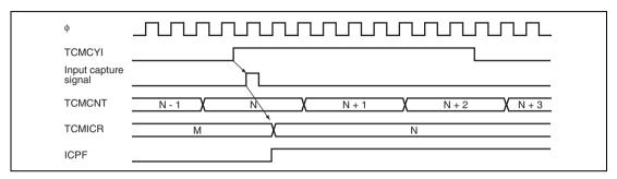
Figure 11.4 Input Capture Operation Timing (Sensing of Rising Edges)
