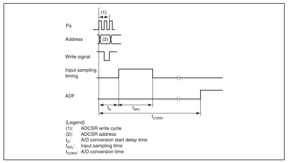
Figure 20.2 A/D Conversion Timing
