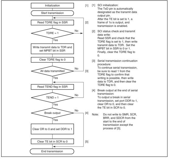
Figure 14.11 Sample Multiprocessor Serial Transmission Flowchart
