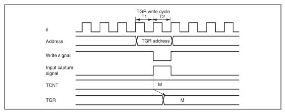
Figure 10.49 Conflict between TGR Write and Input Capture
