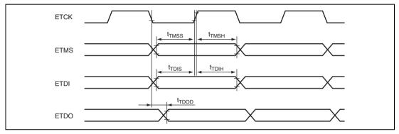
Figure 26.26 JTAG Input/Output Timing
