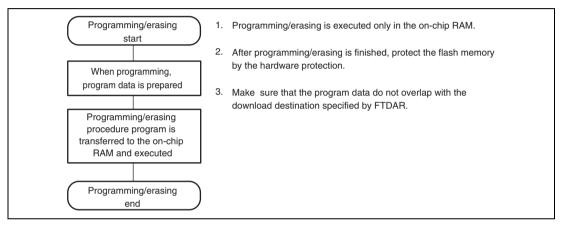
Figure 22.10 Programming/Erasing Flow
