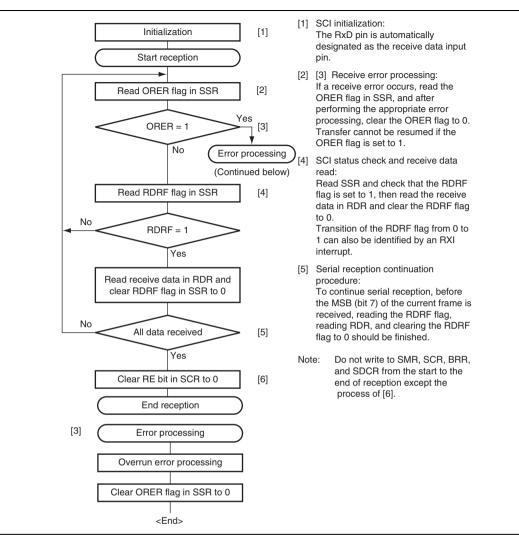
Figure 14.19 Sample Serial Reception Flowchart
