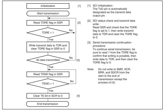
Figure 14.17 Sample Serial Transmission Flowchart
