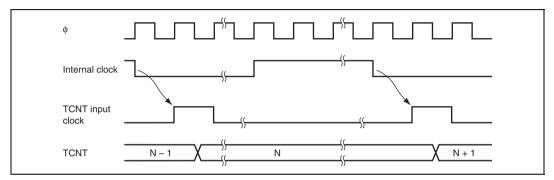
Figure 12.4 Count Timing for Internal Clock Input
