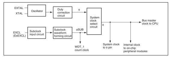
Figure 23.1 Block Diagram of Clock Pulse Generator
