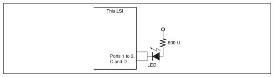
Figure 26.2 LED Drive Circuit (Example)
