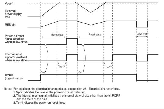
Figure 4.2 The Operation of the Power-On Reset
