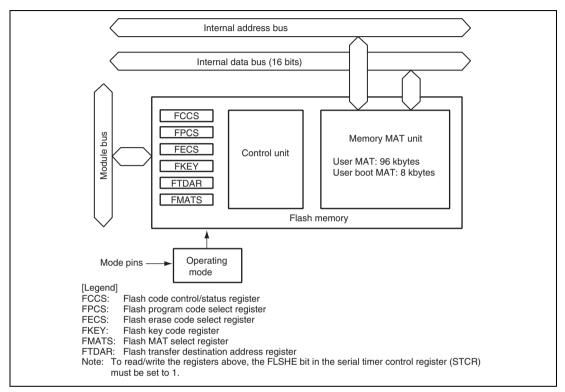
Figure 22.1 Block Diagram of Flash Memory
