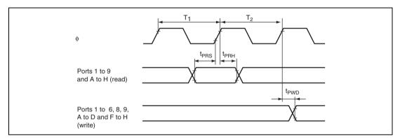
Figure 26.9 I/O Port Input/Output Timing
