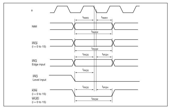
Figure 26.8 Interrupt Input Timing
