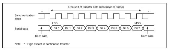
Figure 14.14 Data Format in Synchronous Communication (LSB-First)
