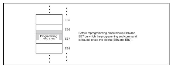
Figure 22.9 Example of Erase Block Including Programmed Area
