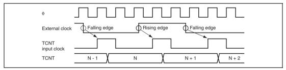
Figure 10.31 Count Timing in External Clock Operation
