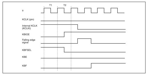
Figure 18.19 KBIOE Setting and KCLK Falling Edge Detection Timing
