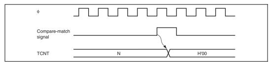
Figure 12.8 Timing of Counter Clear by Compare-Match
