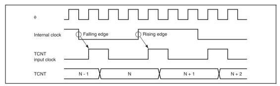
Figure 10.30 Count Timing in Internal Clock Operation
