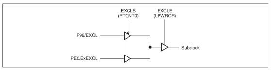
Figure 23.7 Subclock Input from EXCL Pin and ExEXCL Pin
