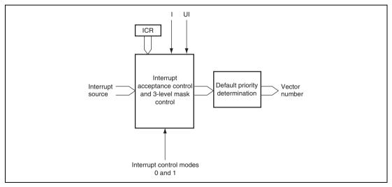
Figure 6.6 Block Diagram of Interrupt Control Operation
