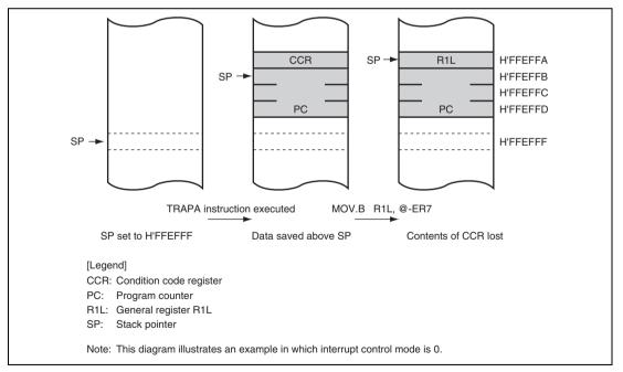
Figure 5.3 Operation when SP Value Is Odd
