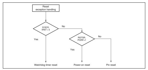
Figure 4.3 Example of Reset Generation Source Determination Flow
