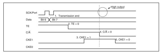
Figure 14.38 Prevention of Low Pulse Output at Switching from SCK Pins to Port Pins
