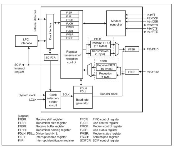
Figure 15.1 shows a block diagram of the SCIF.
