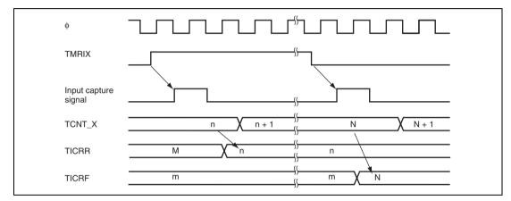
Figure 12.11 Timing of Input Capture Operation
