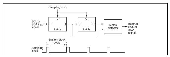
Figure 16.21 Block Diagram of Noise Canceller
