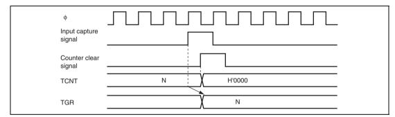
Figure 10.35 Counter Clear Timing (Input Capture)
