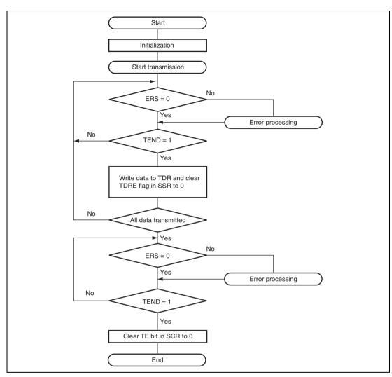
Figure 14.28 Sample Transmission Flowchart
