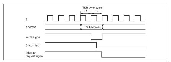
Figure 10.42 Timing for Status Flag Clearing by CPU
