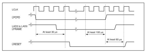
Figure 19.5 Power-Down State Termination Timing
