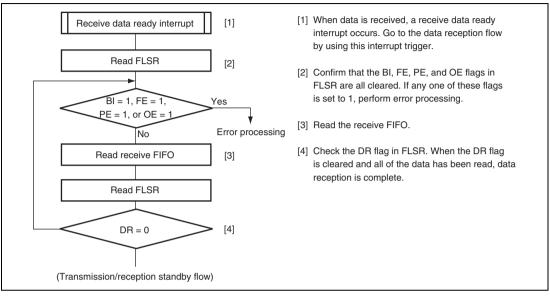
Figure 15.10 Example of Data Reception Flowchart
