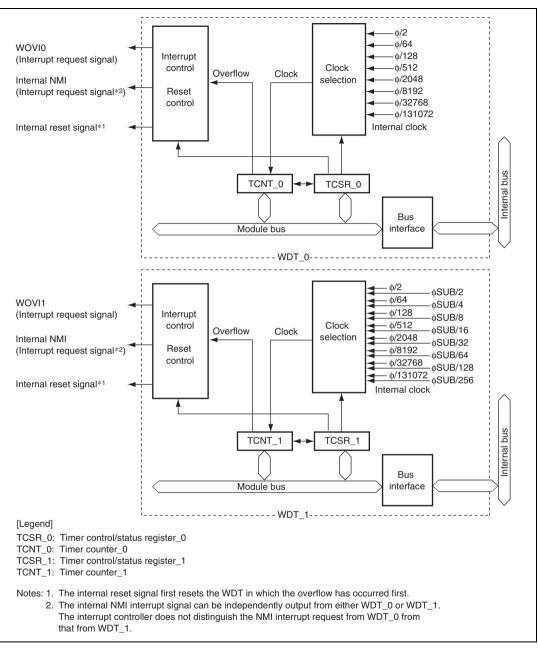
Figure 13.1 Block Diagram of WDT
