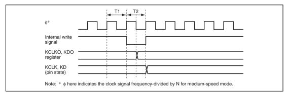
Figure 18.10 KCLKO and KDO Write Timing
