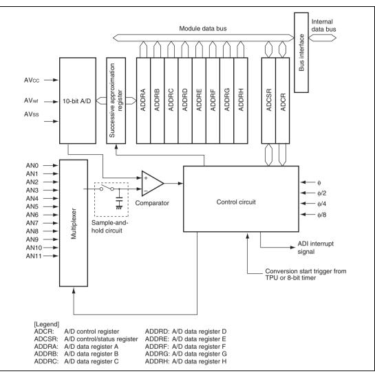
Figure 20.1 Block Diagram of A/D Converter
