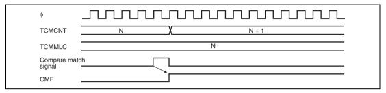
Figure 11.6 Timing of CMF Flag Setting on a Compare Match
