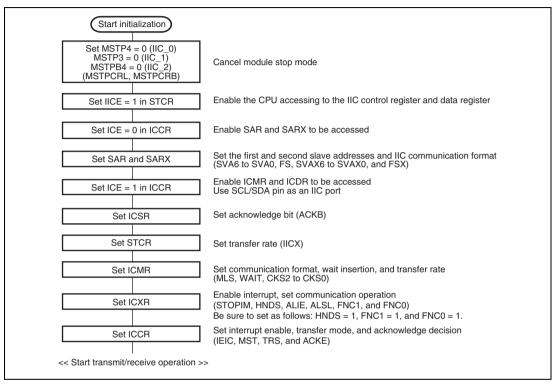
Figure 16.6 Sample Flowchart for IIC Initialization
