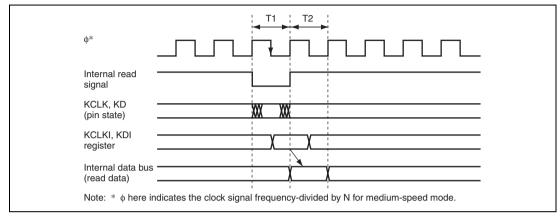
Figure 18.9 KCLKI and KDI Read Timing
