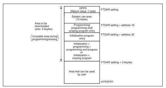
Figure 22.11 RAM Map when Programming/Erasing is Executed
