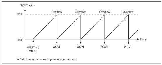
Figure 13.3 Interval Timer Mode Operation
