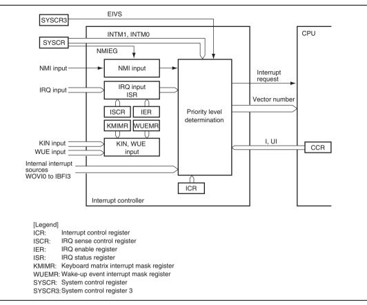
Figure 6.1 Block Diagram of Interrupt Controller
