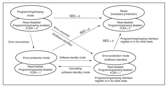
Figure 22.16 Transitions to Error Protection State
