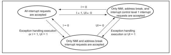
Figure 6.8 State Transition in Interrupt Control Mode 1
