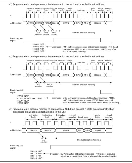
Figure 6.12 Examples of Address Break Timing
