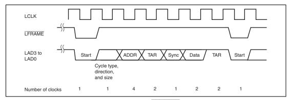
Figure 19.2 Typical LFRAME Timing
