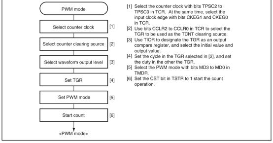
Figure 10.21 Example of PWM Mode Setting Procedure
