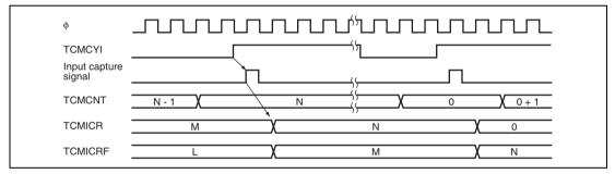
Figure 11.5 Buffer Operation of Input Capture
