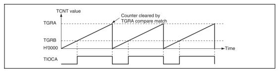
Figure 10.22 Example of PWM Mode Operation (1)
