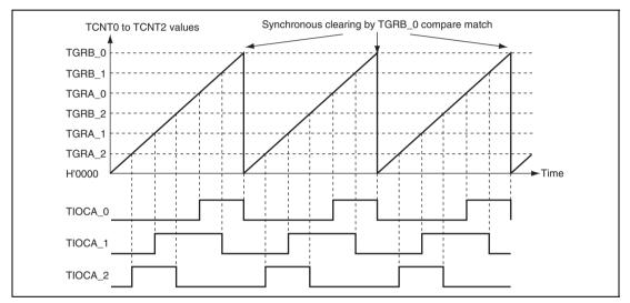
Figure 10.15 Example of Synchronous Operation
