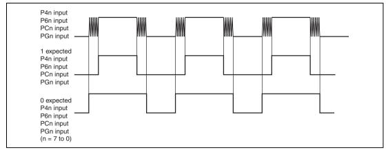
Figure 8.2 Schematic View of Noise Cancel Operation
