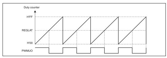
Figure 9.5 Duty Counter Value and PWMU Output Timing
