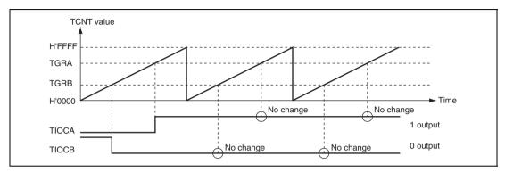
Figure 10.10 Example of 0 Output/1 Output Operation
