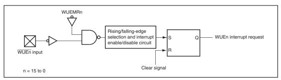
Figure 6.5 Block Diagram of Interrupts WUE15 to WUE0
