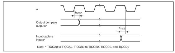
Figure 26.10 TPU Input/Output Timing
