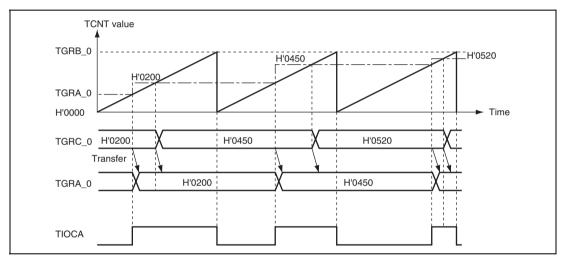
Figure 10.19 Example of Buffer Operation (1)
