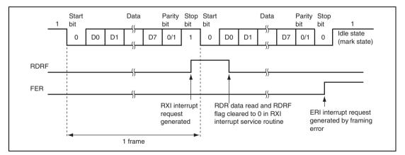
Figure 14.8 Example of SCI Operation in Reception (Example with 8-Bit Data, Parity, One Stop Bit)
