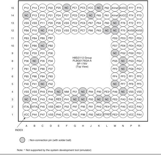
Figure 1.4 Pin Assignments (BP-176V)
