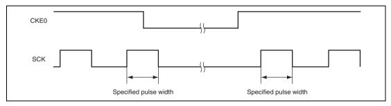
Figure 14.31 Clock Output Fixing Timing
