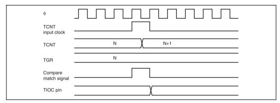
Figure 10.32 Output Compare Output Timing
