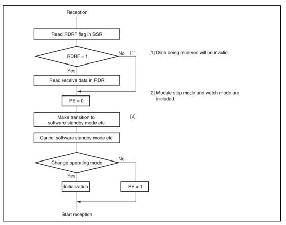
Figure 14.36 Sample Flowchart for Mode Transition during Reception
