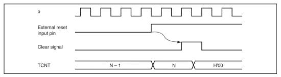
Figure 12.9 Timing of Counter Clear by External Reset Input
