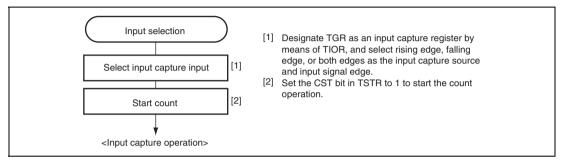
Figure 10.12 Example of Input Capture Operation Setting Procedure
