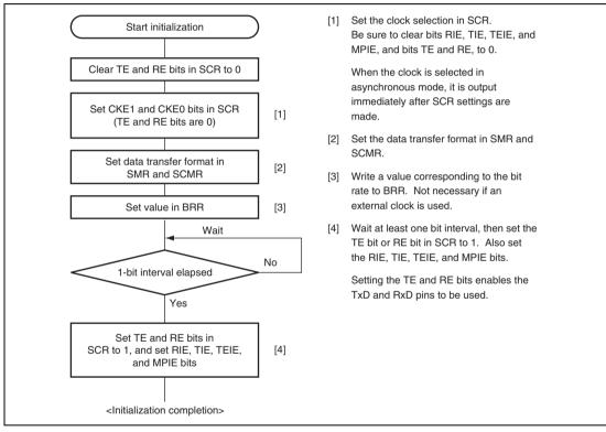
Figure 14.5 Sample SCI Initialization Flowchart
