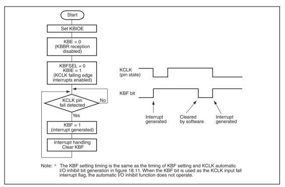
Figure 18.14 Example of KCLK Input Fall Interrupt Operation
