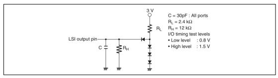
Figure 26.3 Output Load Circuit
