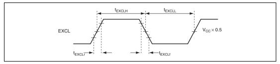
Figure 23.8 Subclock Input Timing
