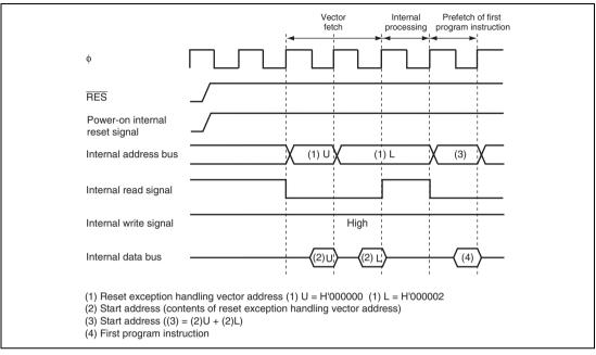
Figure 5.1 shows an example of the reset sequence.
