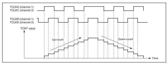
Figure 10.26 Example of Phase Counting Mode 1 Operation
