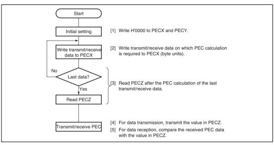
Figure 17.4 Sample Flowchart of PEC Calculation
