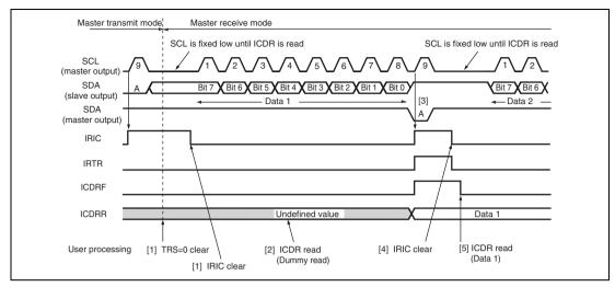
Figure 16.11 Example of Operation Timing in Master Receive Mode (MLS = WAIT = 0)
