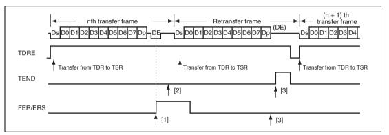
Figure 14.26 Data Re-transfer Operation in SCI Transmission Mode
