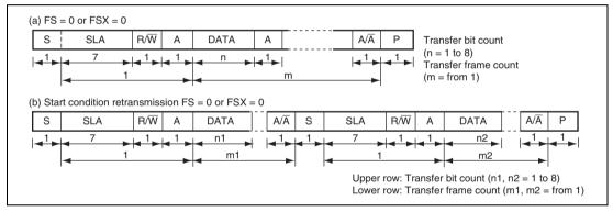
Figure 16.3 I<sup>2</sup>C Bus Data Format (I<sup>2</sup>C Bus Format)
