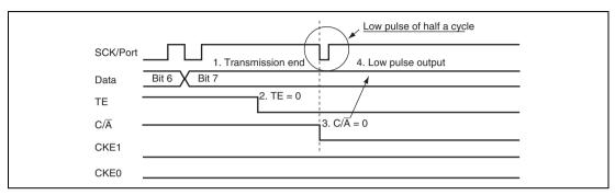
Figure 14.37 Switching from SCK Pins to Port Pins
