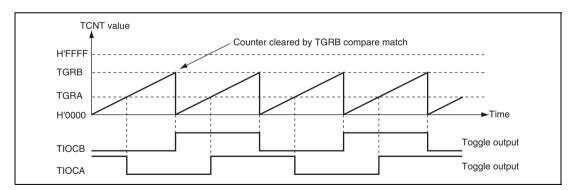
Figure 10.11 Example of Toggle Output Operation
