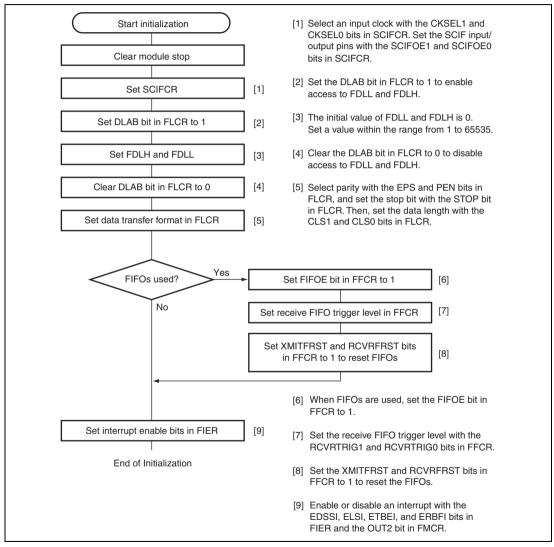
Figure 15.3 Example of Initialization Flowchart
