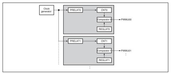
Figure 9.2 Block Diagram of 8-Bit Single Pulse Mode
