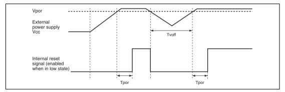
Figure 26.27 Electrical Characteristics of the Power-on Reset Circuit
