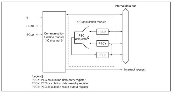
Figure 17.1 Block Diagram of SMBus Interface
