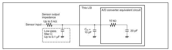
Figure 20.5 Example of Analog Input Circuit
