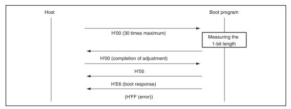
Figure 22.19 Bit-Rate-Adjustment Sequence
