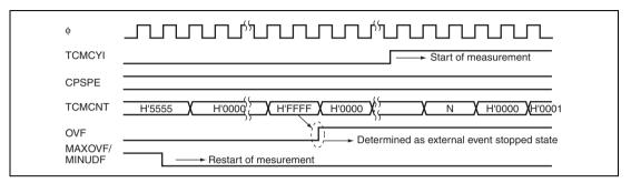
Figure 11.11 Example of Timing in External Event Stopped State (2)
