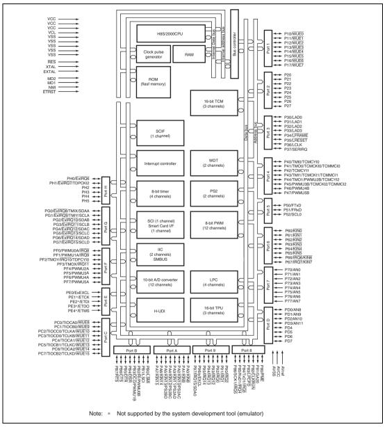
Figure 1.2 Internal Block Diagram
