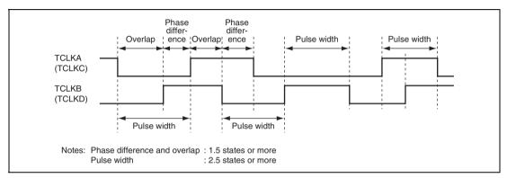
Figure 10.43 Phase Difference, Overlap, and Pulse Width in Phase Counting Mode
