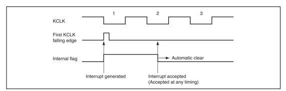
Figure 18.18 Internal Flag of First KCLK Falling Interrupt in Software Standby Mode and Watch Mode
