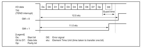
Figure 14.27 TEND Flag Set Timings during Transmission
