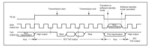
Figure 14.34 Pin States during Transmission in Asynchronous Mode (Internal Clock)
