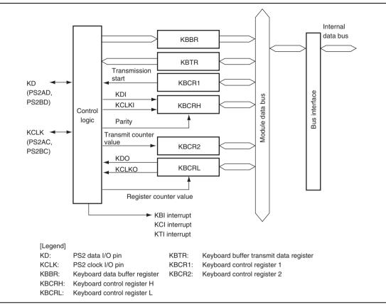
Figure 18.1 Block Diagram of PS2
