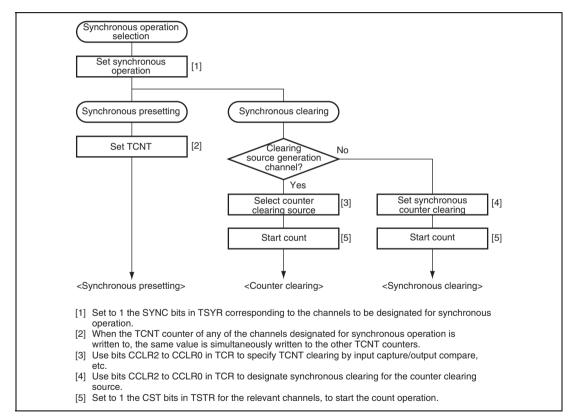
Figure 10.14 Example of Synchronous Operation Setting Procedure
