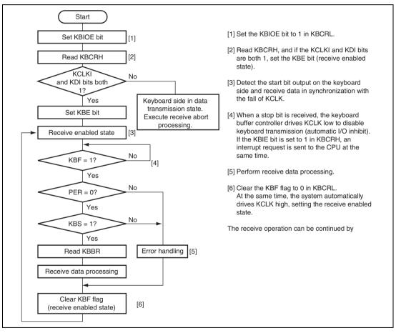
Figure 18.3 Sample Receive Processing Flowchart
