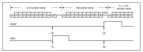
Figure 14.29 Data Re-transfer Operation in SCI Reception Mode
