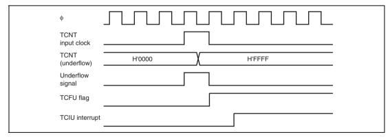
Figure 10.41 TCIU Interrupt Setting Timing
