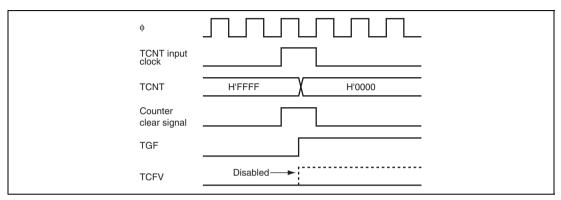
Figure 10.51 Conflict between Overflow and Counter Clearing
