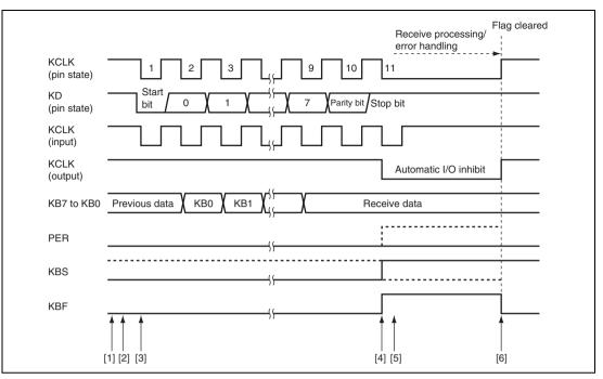
Figure 18.4 Receive Timing
