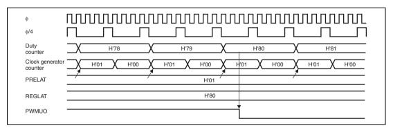
Figure 9.4 Example of Duty Counter and Clock Generator Counter Operation (When PWMPRE = H'01 and PWMREG = H'80 with  $\phi/4$  Selected as Count Clock Source) The following shows the duty counter value and PWMU output timing.
