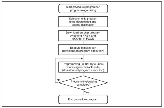
Figure 22.5 Procedure for Creating Procedure Program
