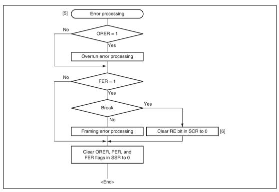
Figure 14.13 Sample Multiprocessor Serial Reception Flowchart (2)
