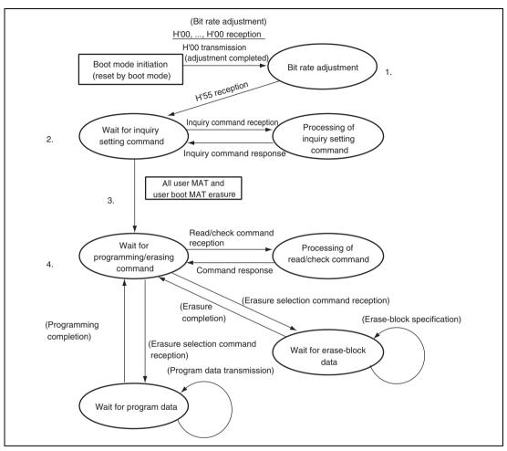
Figure 22.8 Boot Mode State Transition Diagram
