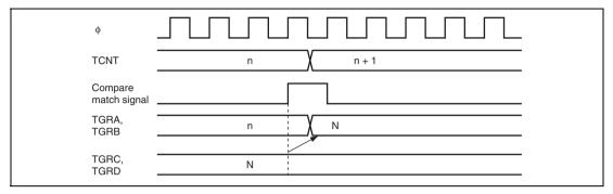
Figures 10.36 and 10.37 show the timing in buffer operation.
