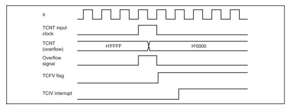
Figure 10.40 TCIV Interrupt Setting Timing
