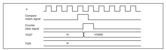
Figure 10.34 Counter Clear Timing (Compare Match)
