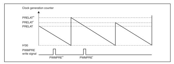
Figure 9.7 PRELAT Update Timing When PWMPRE Value is Changed
