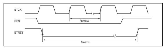
Figure 26.25 Reset Hold Timing
