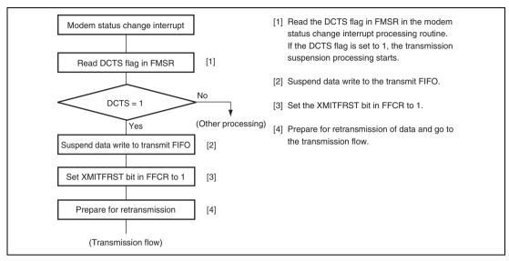
Figure 15.9 Example of Data Transmission Suspension Flowchart
