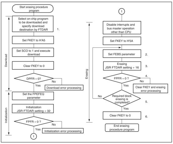
Figure 22.13 Erasing Procedure in User Program Mode
