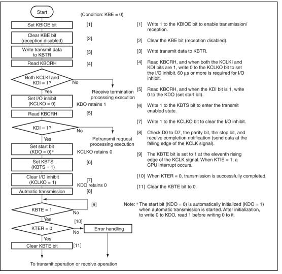
Figure 18.5 Sample Transmit Processing Flowchart
