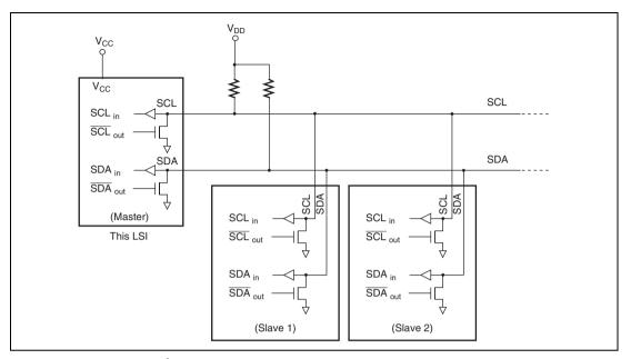
Figure 16.2 I<sup>2</sup>C Bus Interface Connections (Example: This LSI as Master)
