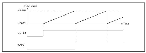
Figure 10.7 Free-Running Counter Operation
