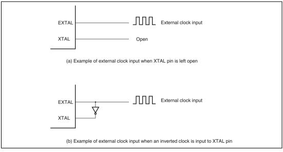
Figure 23.4 Example of External Clock Input
