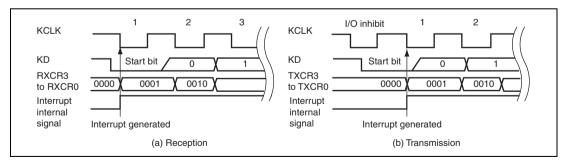
Figure 18.15 Timing of First KCLK Interrupt
