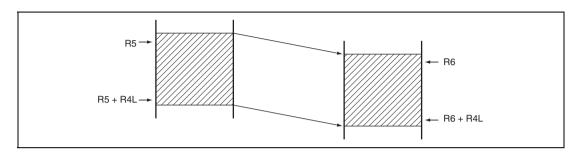
2. R4L and R6 must be set so that the last address of the destination (R6 +R4L) must be H'FFFF or lower. That is, the value of R6 in the middle of execution must not be H'FFFF  $\rightarrow$  H'0000.
