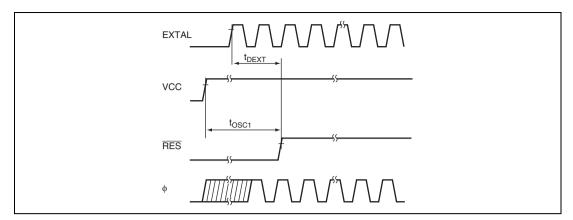
Figure 26.5 Oscillation Stabilization Timing
