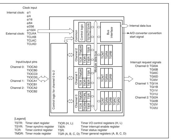
Figure 10.1 Block Diagram of TPU
