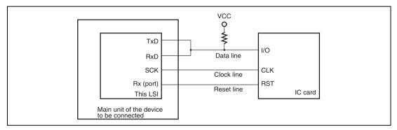
Figure 14.21 Pin Connection for Smart Card Interface
