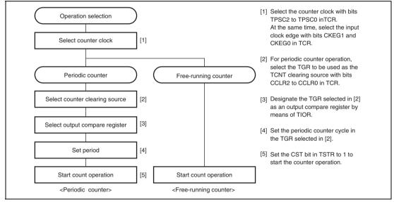
Figure 10.6 Example of Counter Operation Setting Procedure
