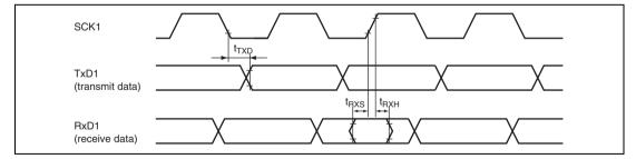
Figure 26.19 SCI Input/Output Timing (Clock Synchronous Mode)
