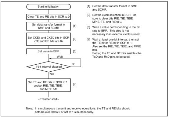
Figure 14.15 Sample SCI Initialization Flowchart
