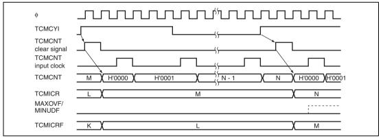
Figure 11.8 shows an example of timing in speed measurement.
