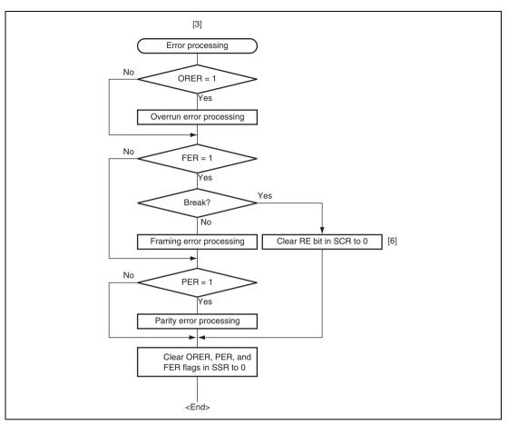
Figure 14.9 Sample Serial Reception Flowchart (2)
