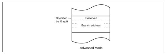
Figure 2.10 Branch Address Specification in Memory Indirect Mode
