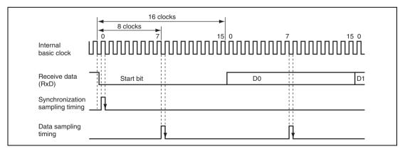
Figure 14.3 Receive Data Sampling Timing in Asynchronous Mode
