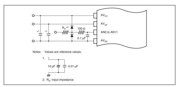
Figure 20.6 Example of Analog Input Protection Circuit
