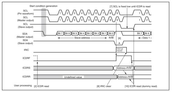
Figure 16.14 Example of Slave Receive Mode Operation Timing (1) (MLS = 0)
