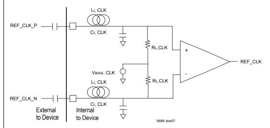
Figure 7.1 Reference Clock Representative Circuit
