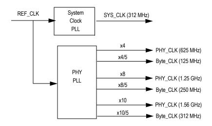
Figure 7.2 Internal PLL Clock Generator
