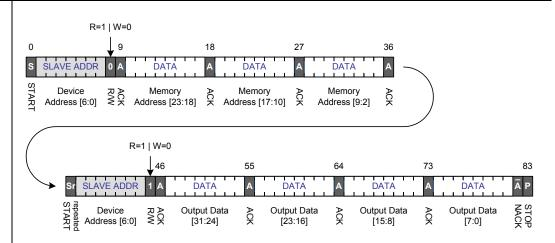
Figure 4.15 Read Protocol with 7-bit Slave Address (ADS is 0)
