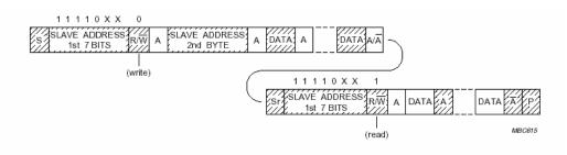
Figure 4.10 Combined Format: Master Addresses a Slave with 10-bit Address<sup>1</sup>
