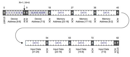
Figure 4.12 Write Protocol with 10-bit Slave Address (ADS is 1)
