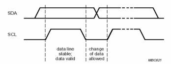
Figure 4.1 Bit Transfer on the I<sup>2</sup>C Bus
