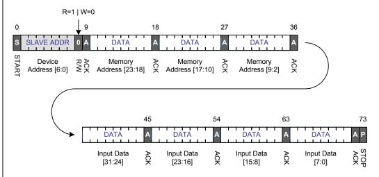
Figure 4.14 Write Protocol with 7-bit Slave Address (ADS is 0)
