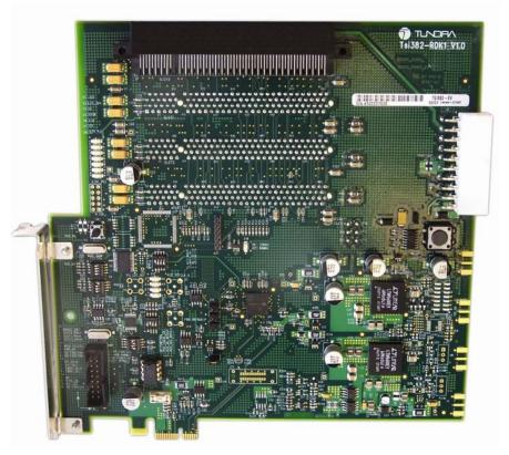
The evaluation board uses the Tsi382A to bridge between x1 PCIe on the card edge to four 32-bit PCI slots on the board.
