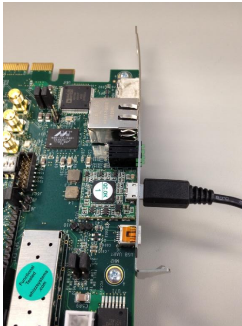
Fig 5. Xilinx KC705 JTAG connector
