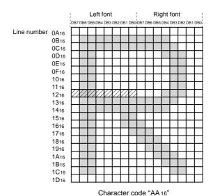
Notes 1: The 80-byte addresses corresponding to the character code "7F16" and "8016" in OSD ROM are the test data storning area. Set "FF16" to the area (We stores the test data to this area and the different data from "FF16" is stored for the actual products.)
