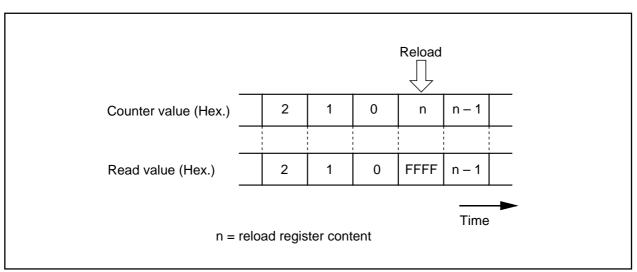
Figure 2.2.28. Reading timer Ai register
