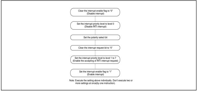
Figure 1.11.13. Switching condition of INT interrupt request
