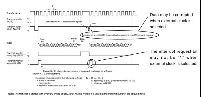
Example of transmit with UART mode, Transfer data 8 bits long.
