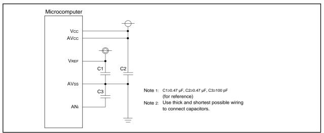
Figure 2.7.22. Use of capacitors to reduce noise
