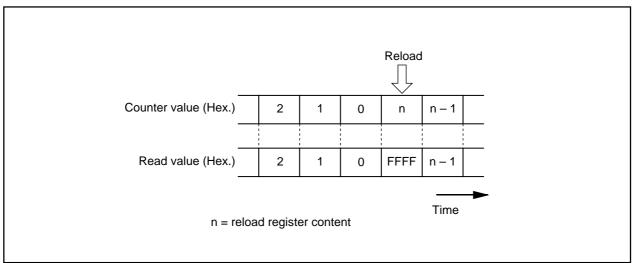
Figure 2.3.12. Reading timer Bi register
