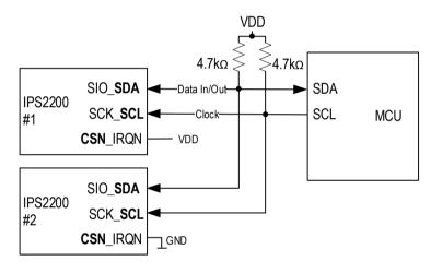
Figure 28. I2C Interface with Address Select
