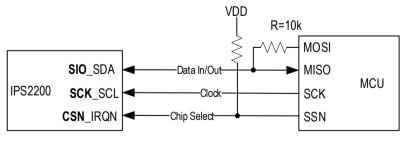
Figure 7. Half Duplex 3-4 Wire SPI Interface
