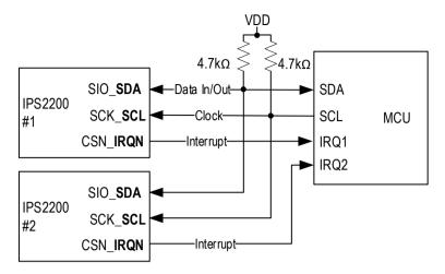
Note: In this mode, several I2C slaves are connected in parallel, all of them must have an individual I2C address.
