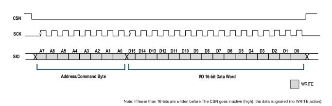
Figure 10. SPI Single Word Write
