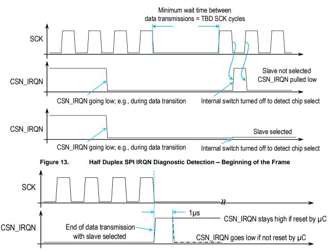
Figure 14. Half Duplex SPI IRQN Diagnostic Detection – End of the Frame
