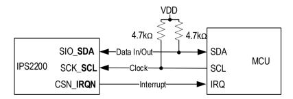
Figure 29. I2C Interface Configuration with Interrupt on a Single Slave
