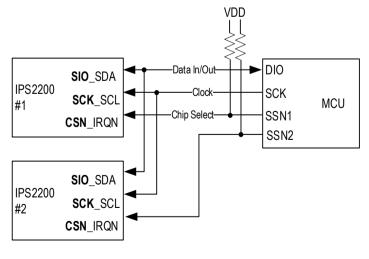
Figure 5. Half Duplex 3-3 Wire SPI Multi-slave Interface
