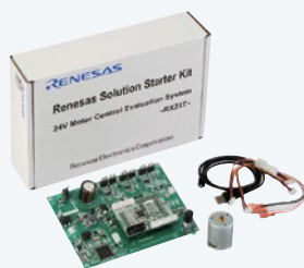
RX motor control starter kit (24V Motor Control Evaluation System for RX)
