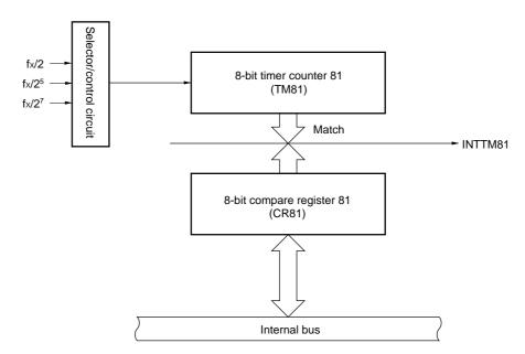
Figure 5-4. Block Diagram of 8-Bit Timer 81
