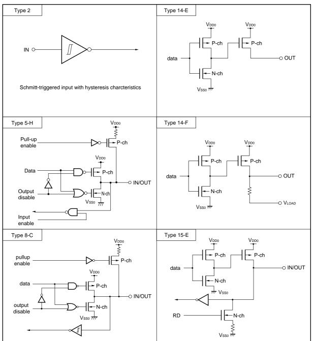
Figure 3-1. Pin Input/Output Circuits
