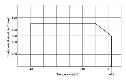
**Note** Total power dissipation differs depending on the temperature (see the following figure).
