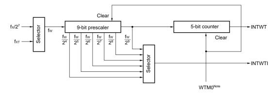
Note Bit 0 of the Watch timer mode control register (WTM)
