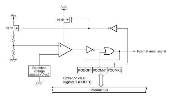
Figure 6-18. Block Diagram of Low-Voltage Detection Circuit
