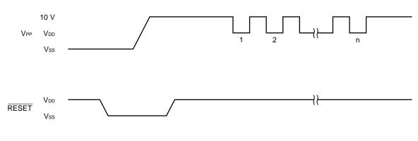
Figure 10-1. Communication Mode Selection Format
