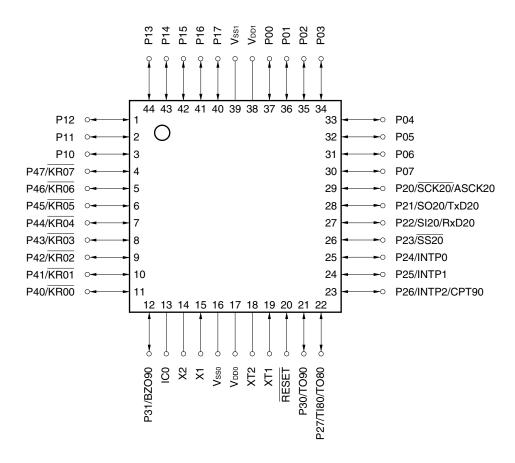
Caution Connect the IC0 (Internally Connected) pin directly to Vsso or Vss1 pin.
