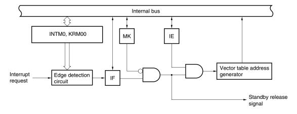
INTM0: External interrupt mode register 0 KRM00: Key return mode register 00
