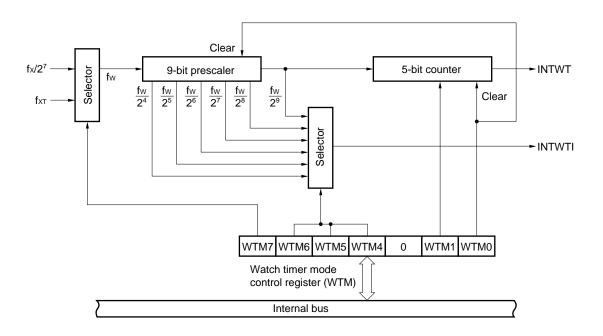
Figure 5-6. Block Diagram of Watchdog Timer
