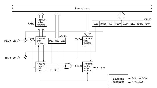
Figure 5-9. Block Diagram of Serial Interface UART0
