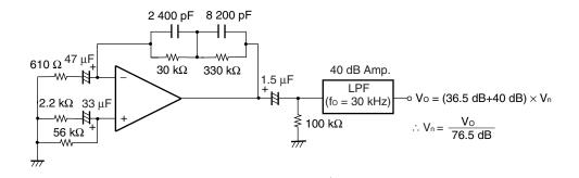
Figure 3 Noise Measurement Circuit (FLAT+JIS A)
