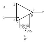
★ Remark The OFFSET NULL pins should be left open or connected to V<sup>-</sup> via a resistor as shown in the left figure. Don't connect to any lines other than V<sup>-</sup>, otherwise mulfunction, degradation, or failure may occur.
