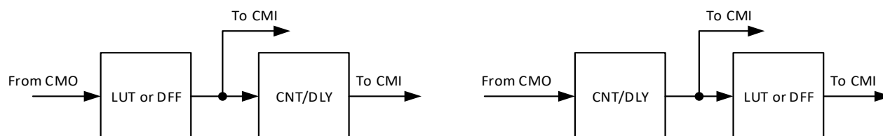
Figure 32. Possible Connections inside Multi-Function Macrocell
