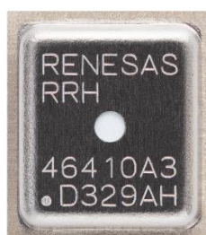
Figure 1. RRH46410 Gas Sensor
