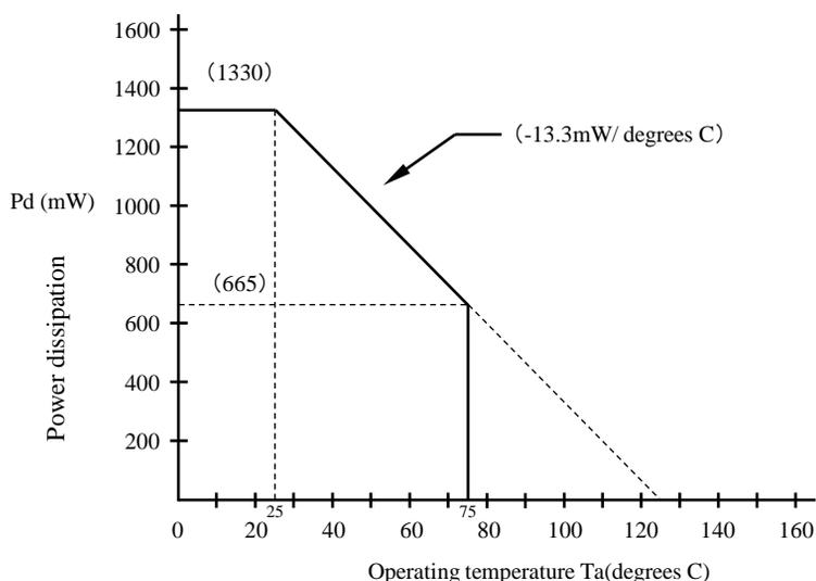
Notes The power consumption of this IC has the dominant electric power which each output transistor consumes.
