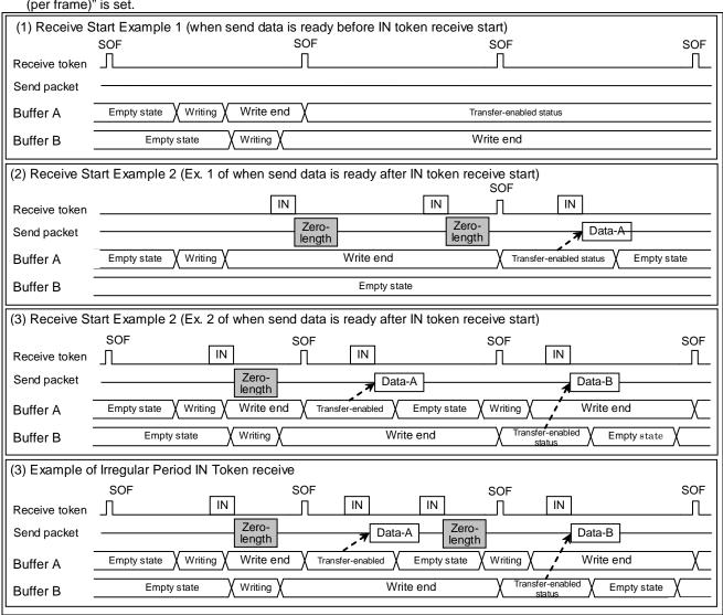
Figure 3.21 Data Setup Function Operation
