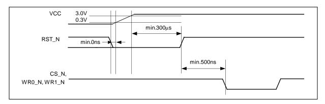
Note: Simultaneous Power-on and Power-off is recommended for VCC and AVCC. VIF Power-on timing is recommended to be simultaneous with VCC and AVCC, or to be earlier than VCC and AVCC. The VIF Power-off timing is recommended to be simultaneous with VCC and AVCC, or to be later than VCC and AVCC.
