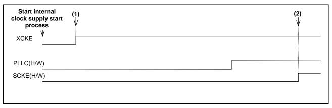
Figure 3.2 Clock Supply Start Control Timing Diagram
