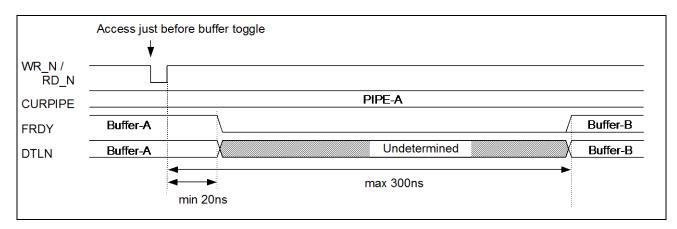
Figure 3.19 Figure 3.18 FRDY, DTLN Confirmation Timing after Double Buffer Read/Write Complete
