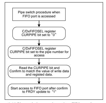
Figure 3.16 Pipe switch procedure when FIFO port is accessed
