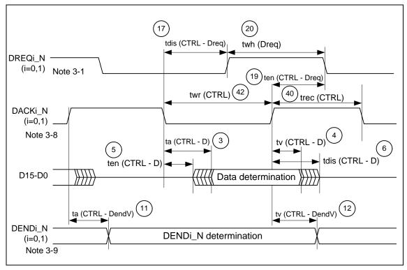
Note 3-1: The control signal is the inactive condition for DREQi\_N (i=0, 1). When the next DMA transfer exists, the delay ratings for twh (Dreq) and ten (CTRL-Dreq) will be valid until DREQi\_N becomes active is twh (Dreq).
