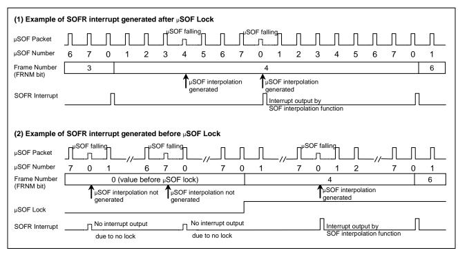
Figure 3.12 SOFR Interrupt Output Timing Example
