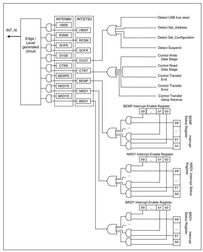
**Figure 3.6 Interrupt Configuration Diagram**
