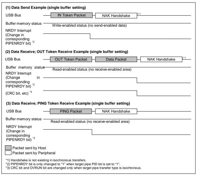
**Figure 3.8 NRDY Interrupt Generation Timing**
