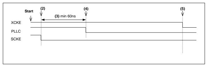
Figure 3.3 Internal Clock Supply Stop Process Timing Diagram
