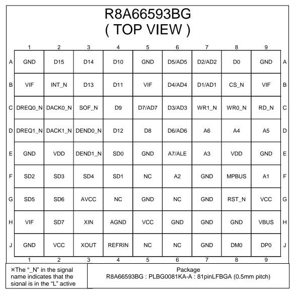
Figure 1.2 R8A66593BG Pin Layout
