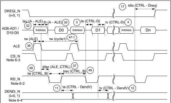
Note 6-1: The control signal when writing data is a combination of CS\_N, WR0\_N and WR1\_N.
