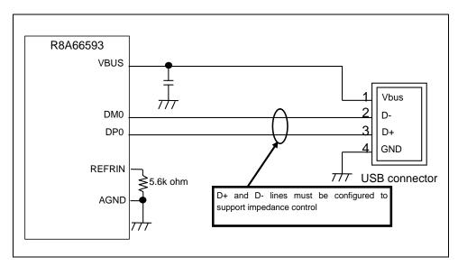
Figure 3.25 USB Connector Connection Example
