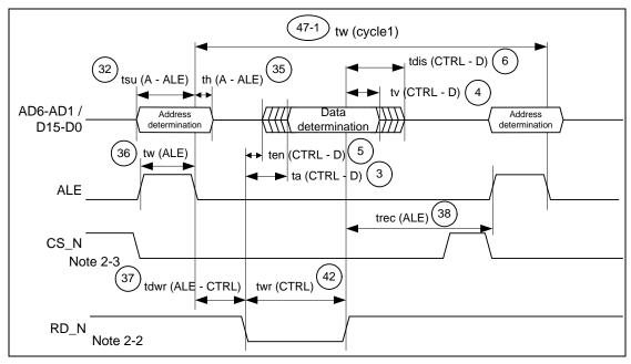
Note 2-1: The control signal when writing data is a combination of CS\_N, WR1\_N, and WR0\_N.
