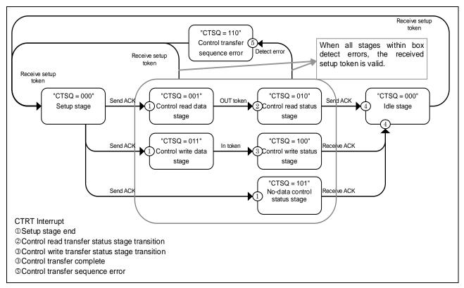
Figure 3.11 Control Transfer Stage Transition
