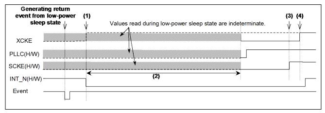
Figure 3.4 Control Timing Diagram for Returning from Low-Power Sleep State
