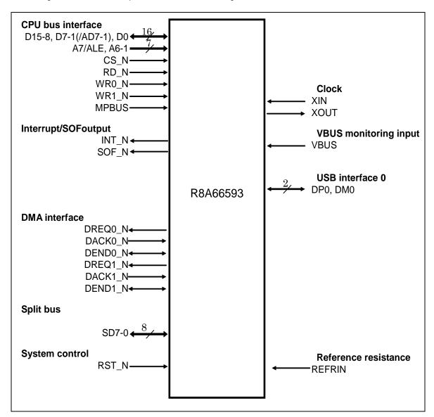
Figure 1.3 Block Diagram of Pin Functions
