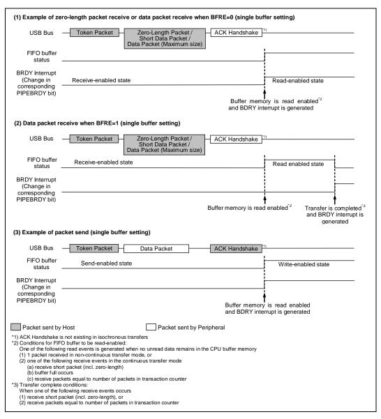
Figure 3.7 BRDY Interrupt Generation Timing Diagram
