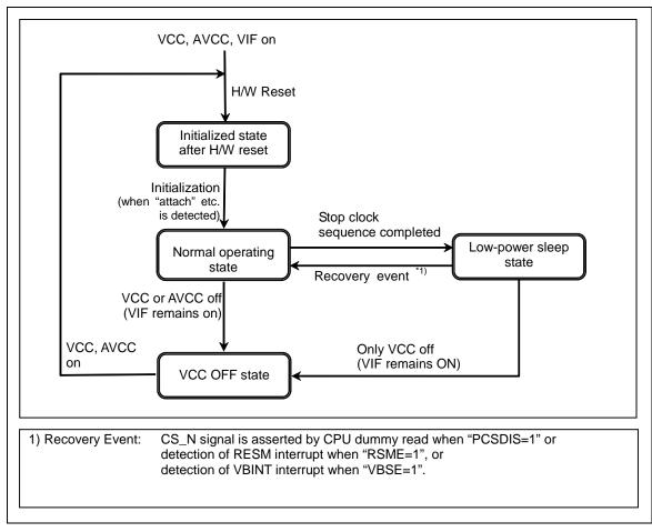
Figure 3.1 Controller State Transition Diagram
