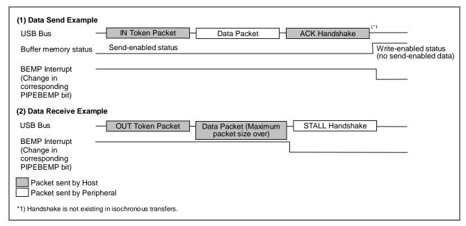
Figure 3.9 BEMP Interrupt Generation Timing Diagram
