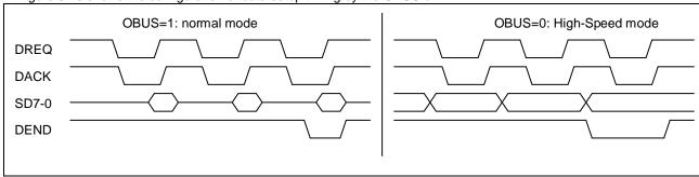
Figure 3.20 Data Setup Timing Configuration
