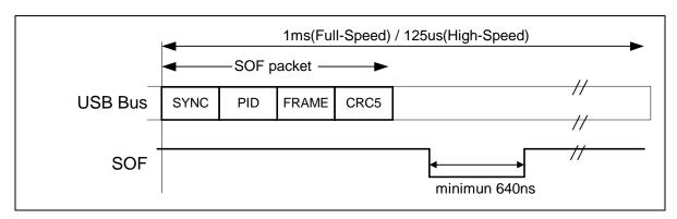
Figure 3.24 SOF Output Timing
