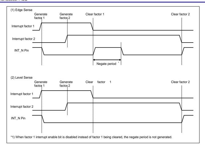
Figure 3.5 INT\_N Pin Operating Diagram (example when "INTA=0" is set)
