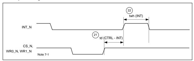
Note7-1: Writing using the combination of CS\_N, WR0\_N and WR1\_N takes place during the active ("L") overlap period. The ratings from the rising edge are valid starting from the earliest change in the inactive signal.
