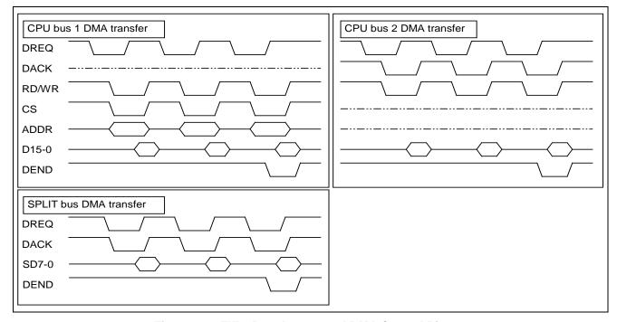
Figure 3.17 FIFO Port Access and DMA Control Pin
