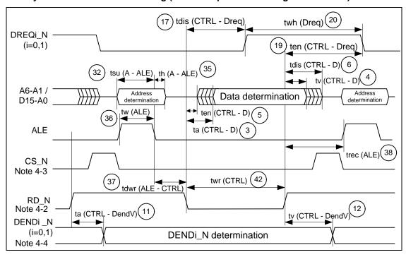
Note 4-1: The control signal when writing data is a combination of CS\_N, WR0\_N, and WR1\_N.
