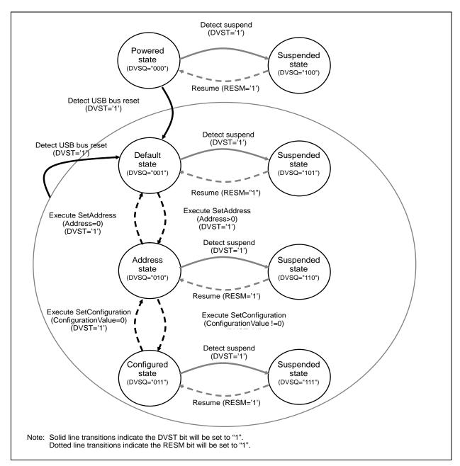
Figure 3.10 Device State Transitions
