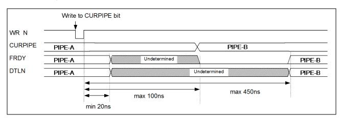
Figure 3.18 FRDY, DRLN Fix Timing after Pipe Switch
