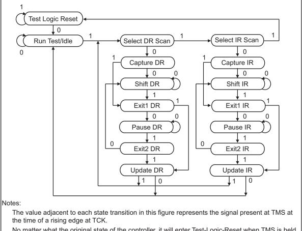
No matter what the original state of the controller, it will enter Test-Logic-Reset when TMS is held high for at least five rising edges of TCK.
