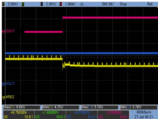
Figure 11. Load Transient: V OUT = 5V, 0A → 1.2A
