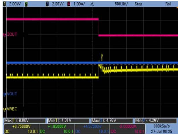
Figure 14. Load Transient: V_{OUT} = 4.5V, 1.2A \rightarrow 0A
