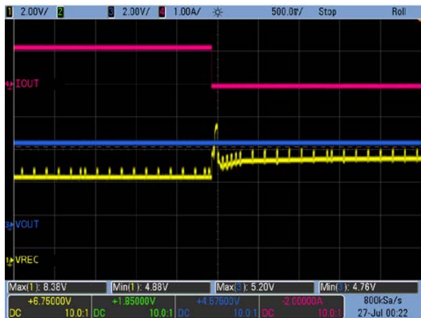
Figure 12. Load Transient: V OUT = 5V, 1.2A → 0A
